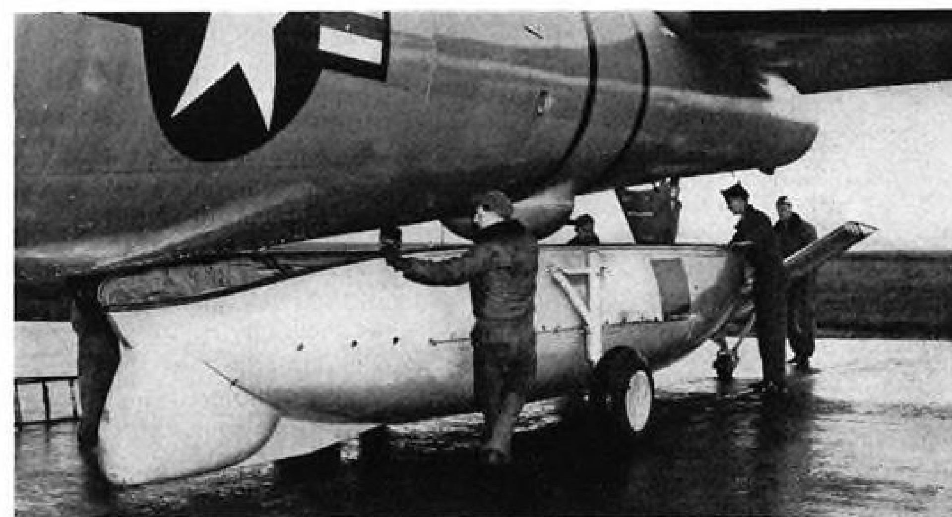
OFF TO THE RESCUE! Airmen wheel an Edo A-3 lifeboat into position under SB-29 after which wheels are detached, 100 foot parachute lowers boat.
