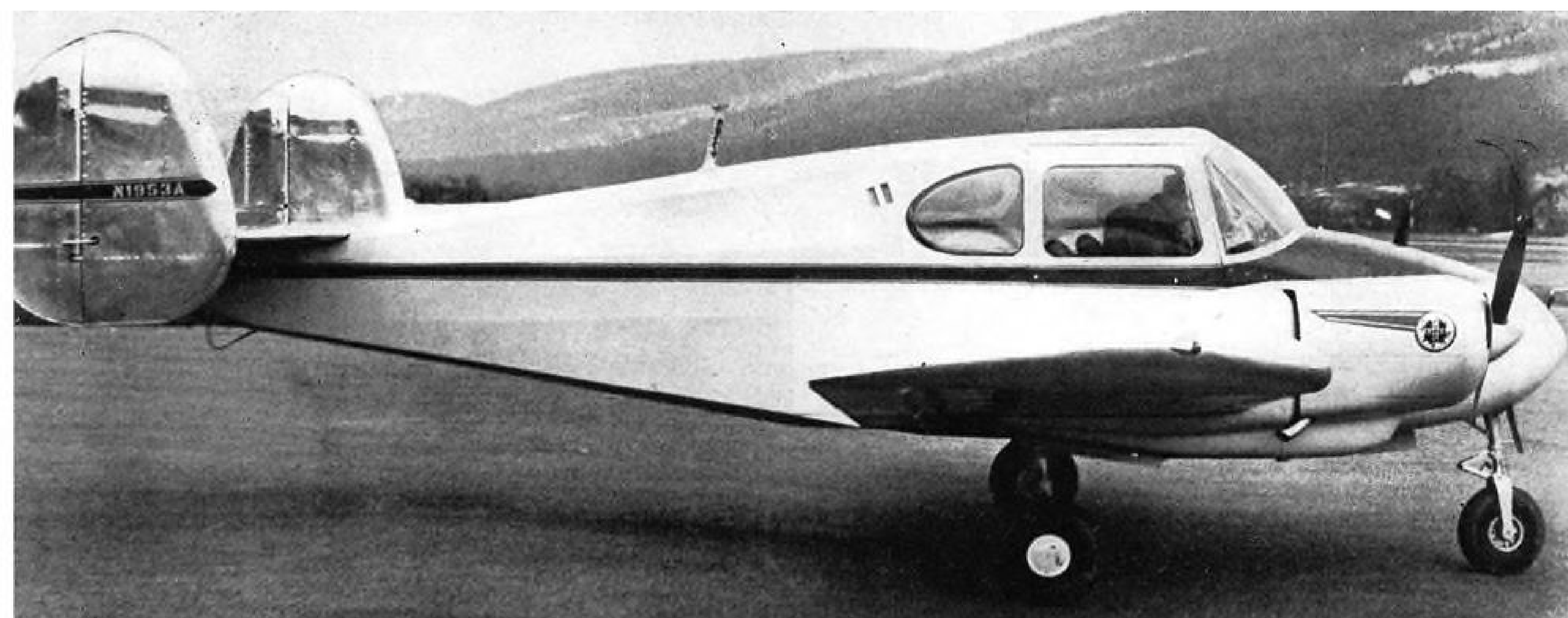
PIPER TRANSPORT —First photo (above) shows new Piper PA-23 Twin-Stinson low-wing four-place light transport powered by two 135-hp. Lycoming O-290-D2 engines, which began its flight test program Mar. 2. It's designed to sell for less than $25,000 (Aviation Week Mar. 3, p. 16).
