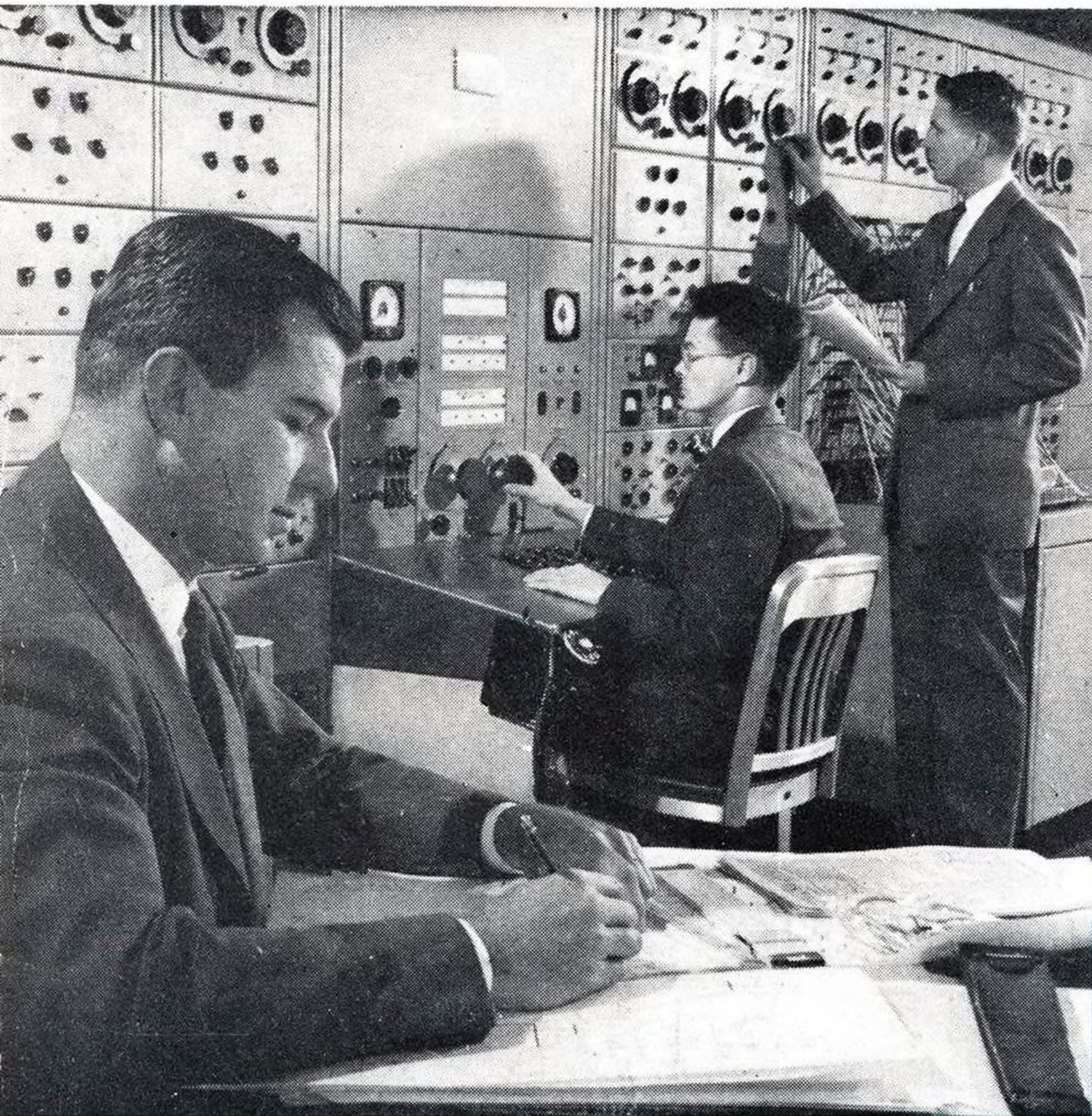
Complete electrical systems for any given aircraft can be simulated on this network analyzer.
