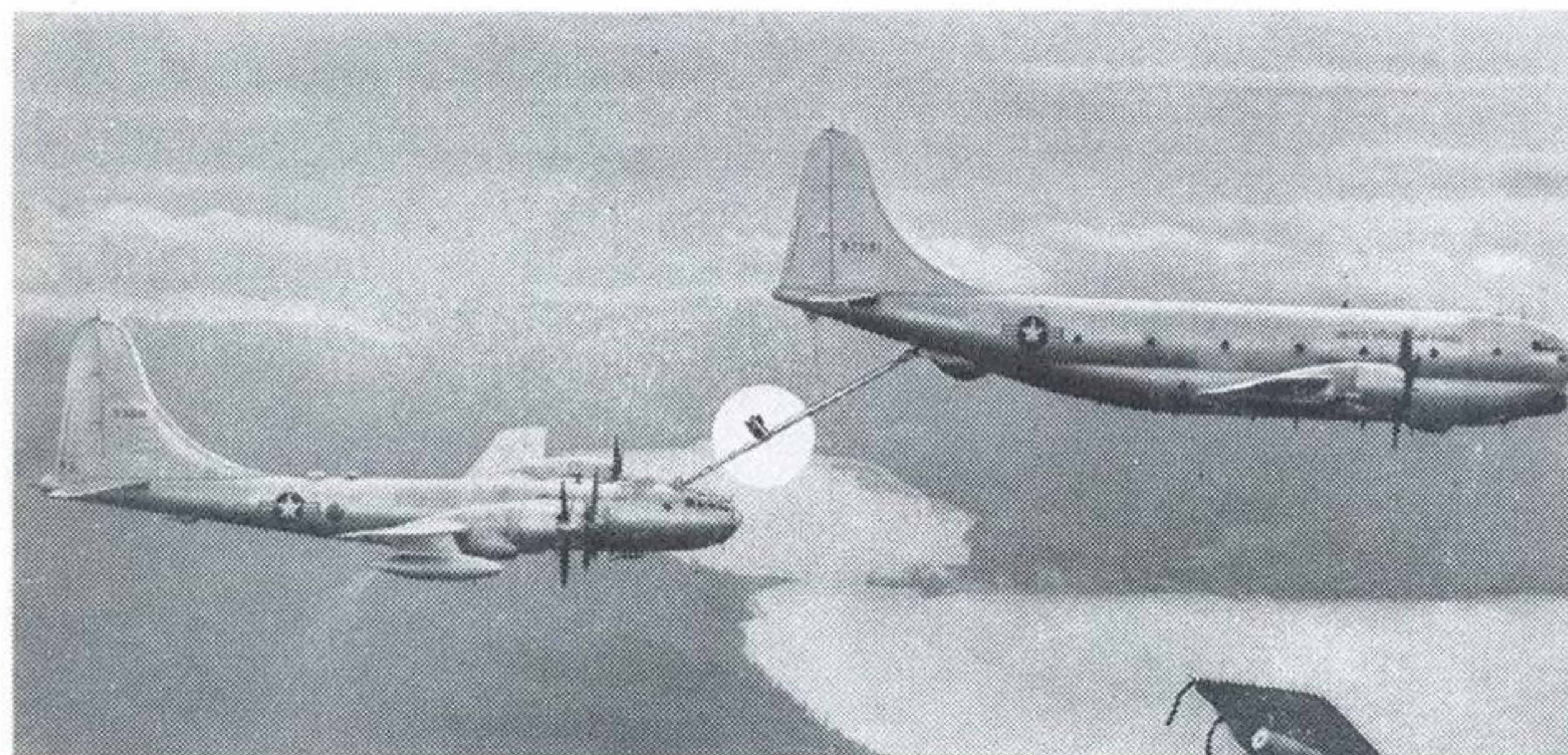
ICEGUARD PROTECTION on rudder surfaces controlling refueling boom. Smaller picture shows KC-97A in flight refueling of B-50.
