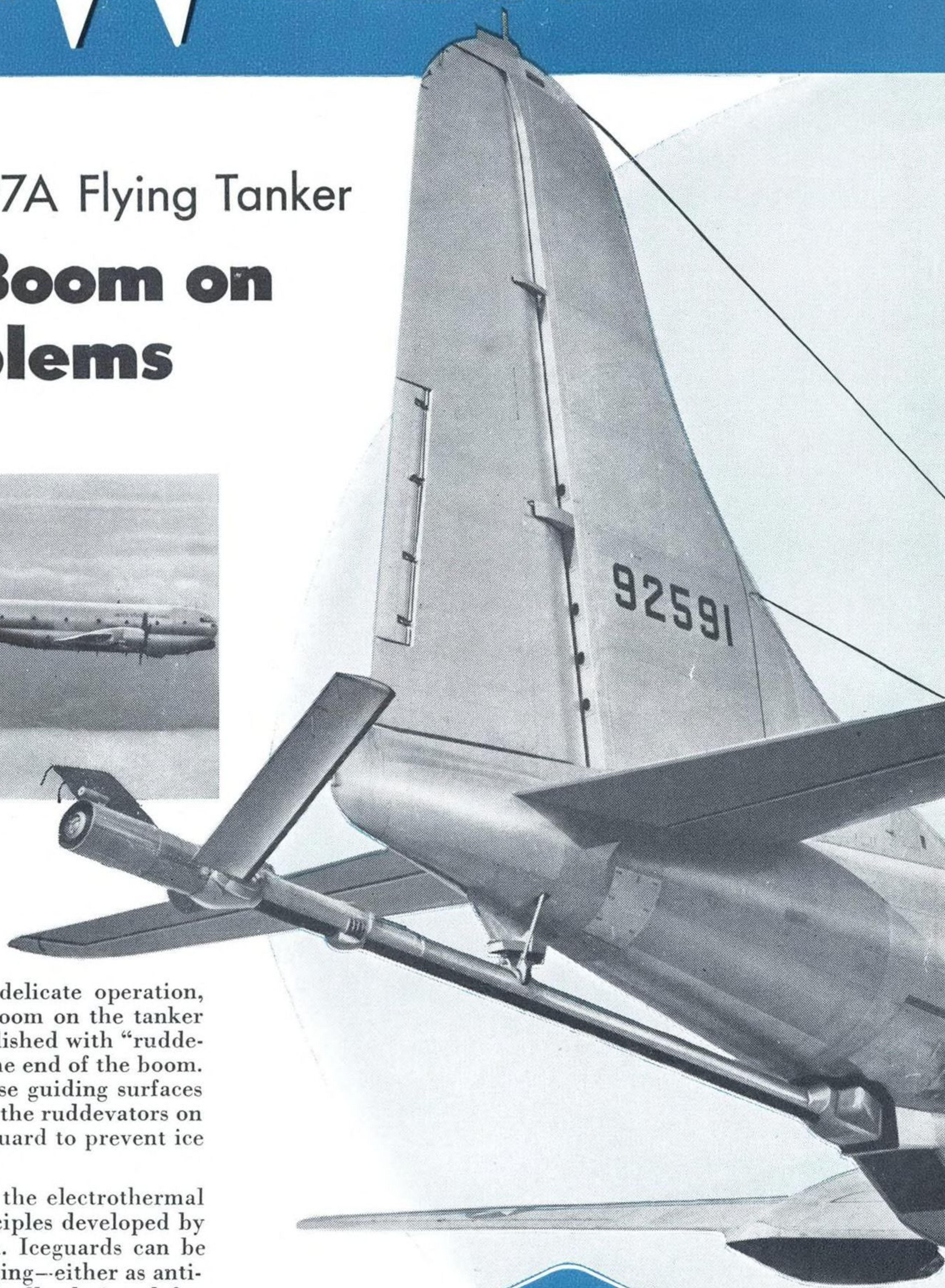
ICEGUARD PROTECTION on rudder surfaces controlling refueling boom. Smaller picture shows KC-97A in flight refueling of B-50.
