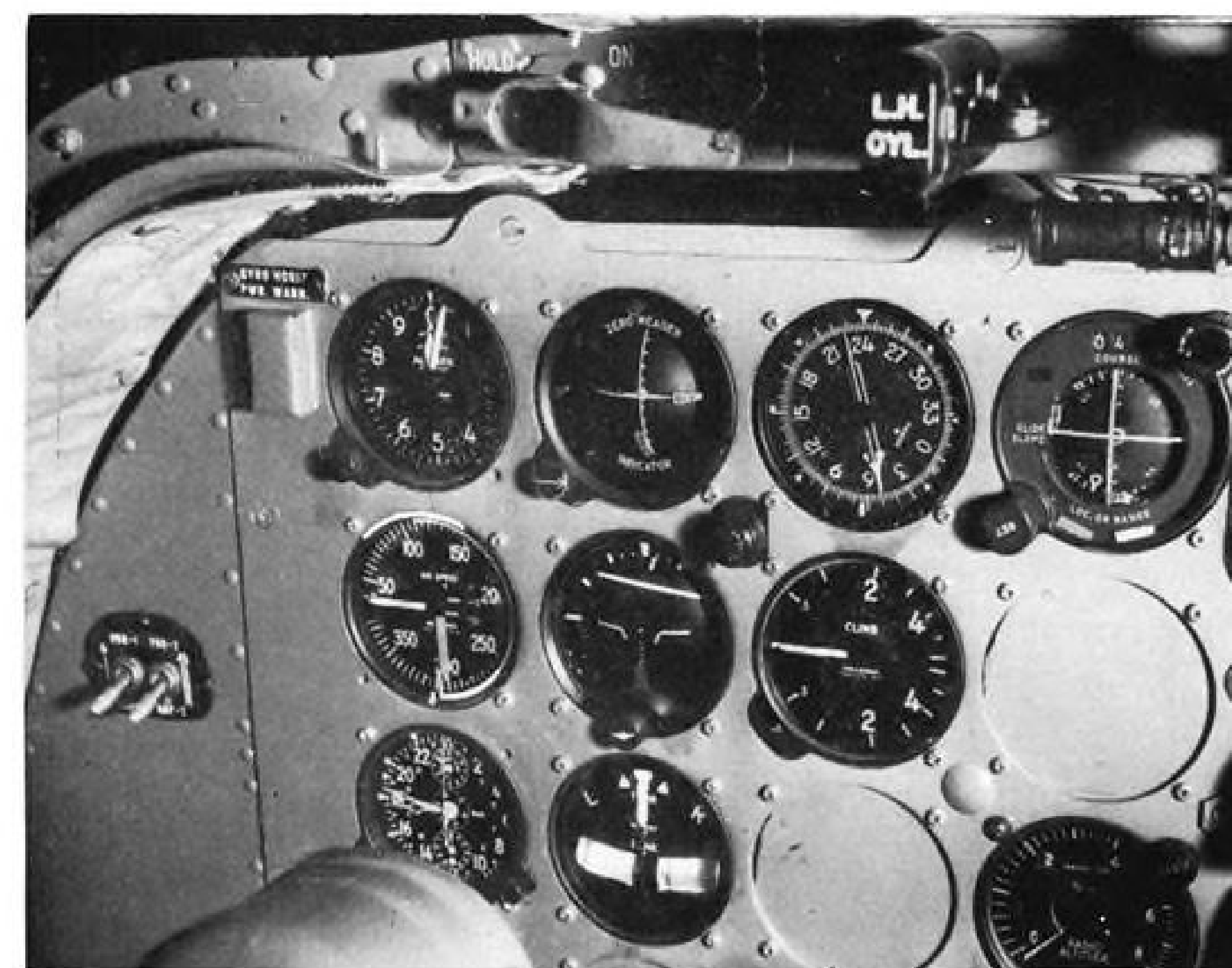
ZERO READER gets choice spot on PanAm panel (top row, second from left). Bendix Omnimag is at extreme right, with space below it for DME indicator.
