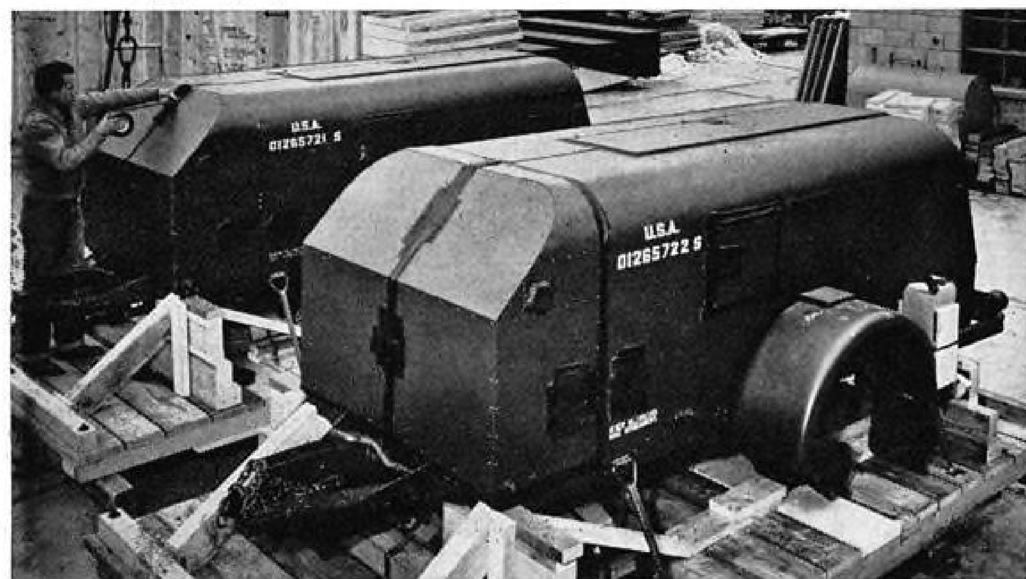
COMPLYING WITH GOV'T SPECS , these army mobile shower trailer units are sealed with Polyken No. 214, ready for overseas shipment.
