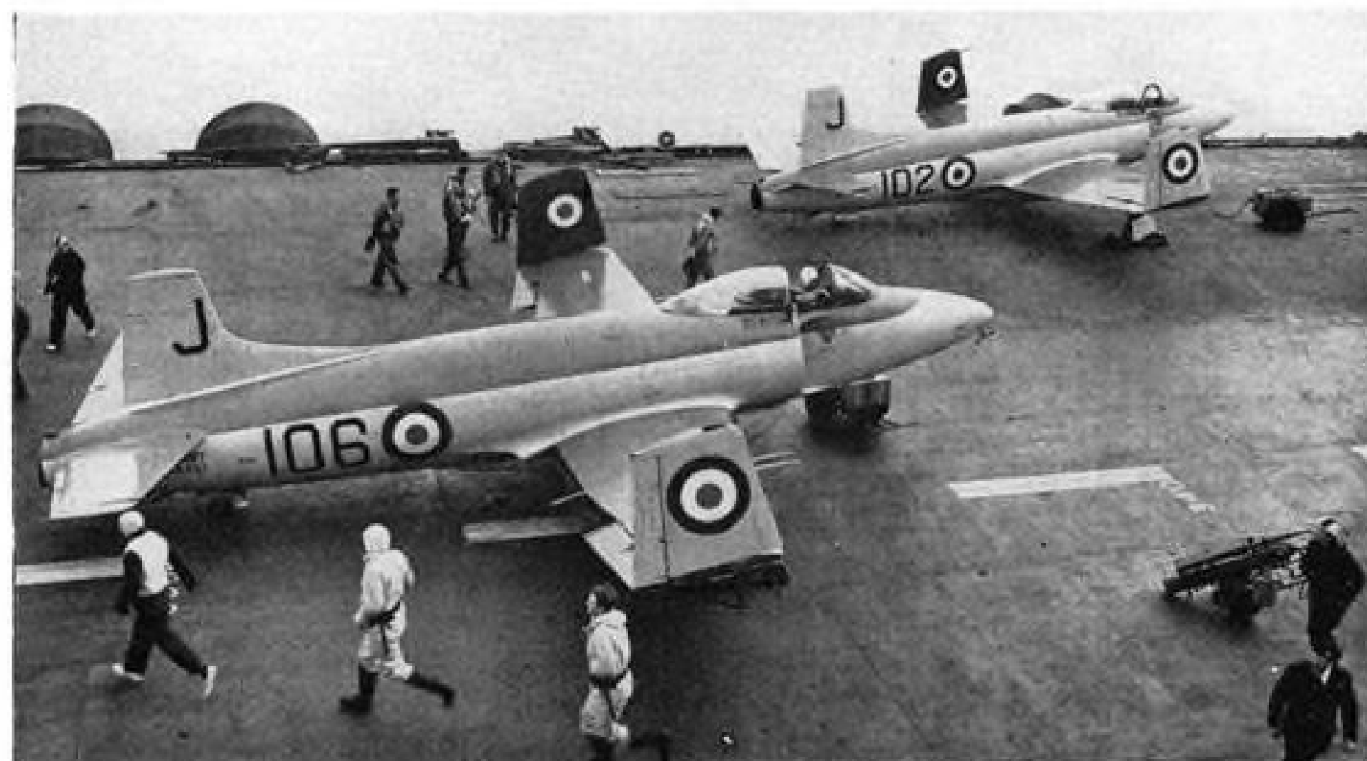
STUB WINGS FOLDED, two Attackers are ranged on deck awaiting further flight duty.
