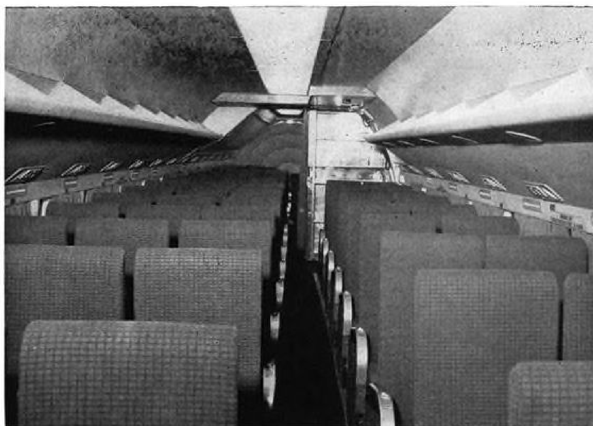
MAIN TOURIST CABIN accommodates 71 with five-abreast seating. Removable seats are lighter and narrower than counterparts in the luxury version.
