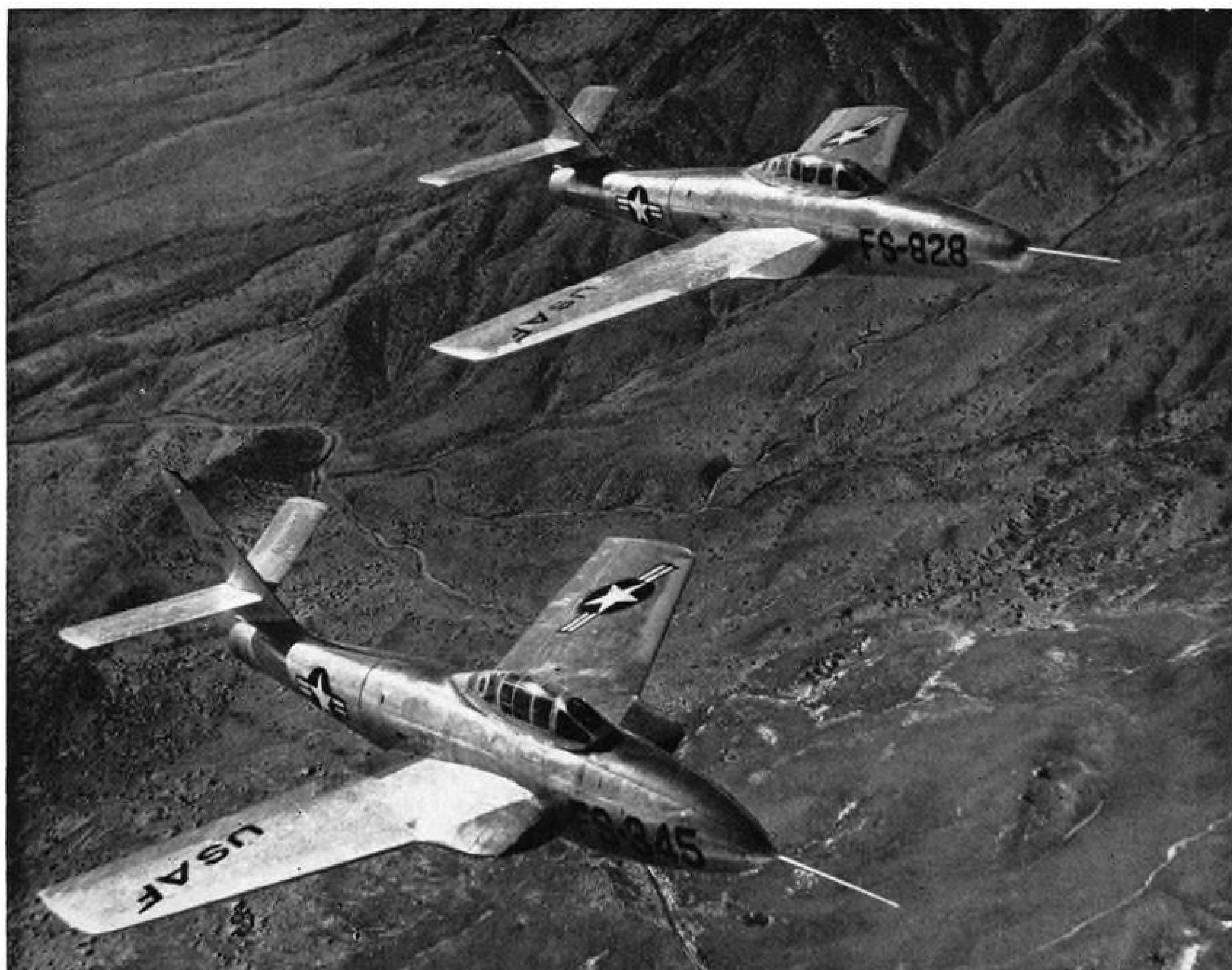
NEW THUNDERJETS, the fighter-bomber version of the F-84F (foreground) and the photo reconnaissance F-84F, shown in test flights over Edwards AFB, Calif. Both are equipped with Wright-built J65 Sapphire jet engines.
