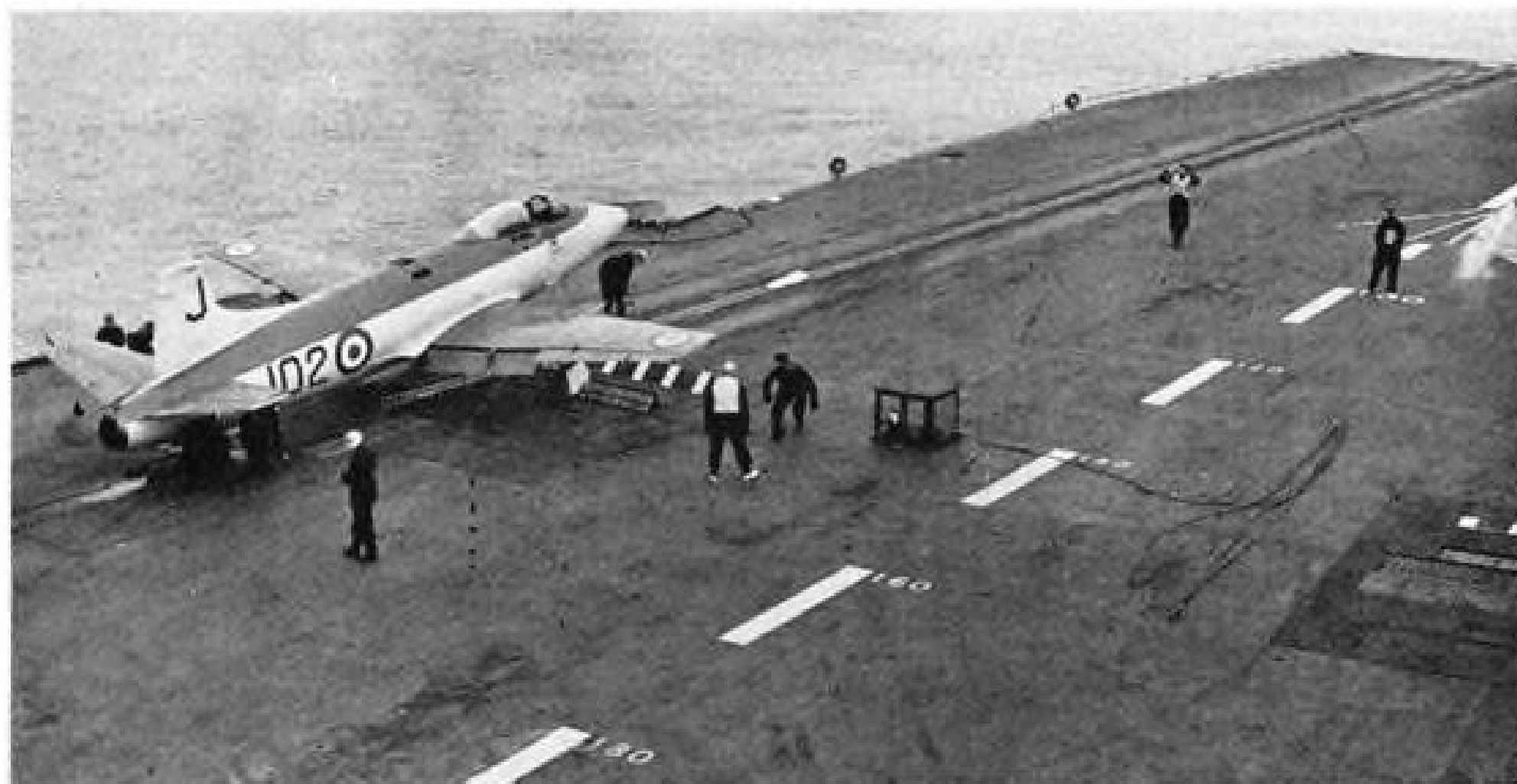
TIED TO CATAPULT, Attacker will be "fired off" by controller in enclosure.
