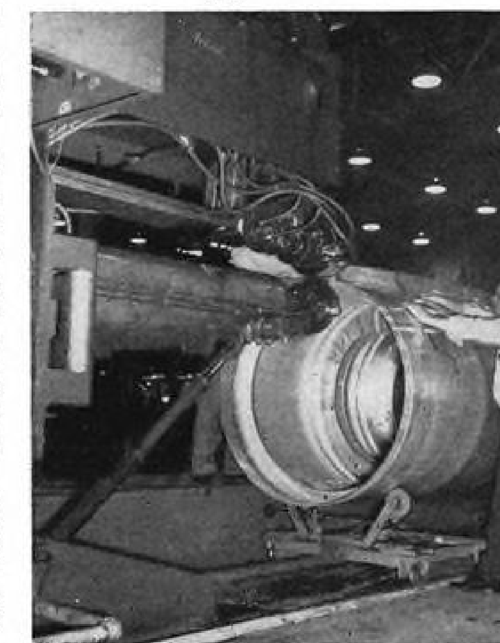
FEDERAL WELDERS, used on the giant fuel tanks, have deep 60-in. throat, can spot nine welds per inch at a rate of 200 per min.
