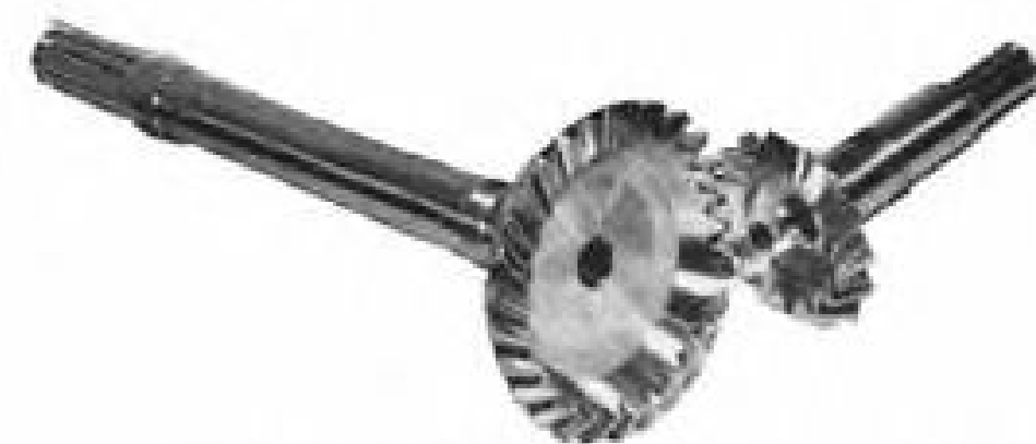
The driven gear shown here is 5" in pitch diameter and 15" long overall. It is carburized and hardened with heat-treating distortion held within .001".
