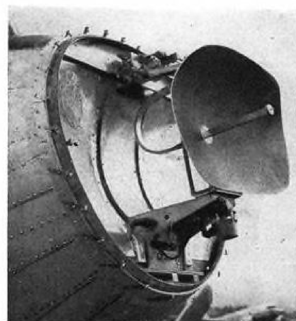
AIRCRAFT aerial with cover removed.
