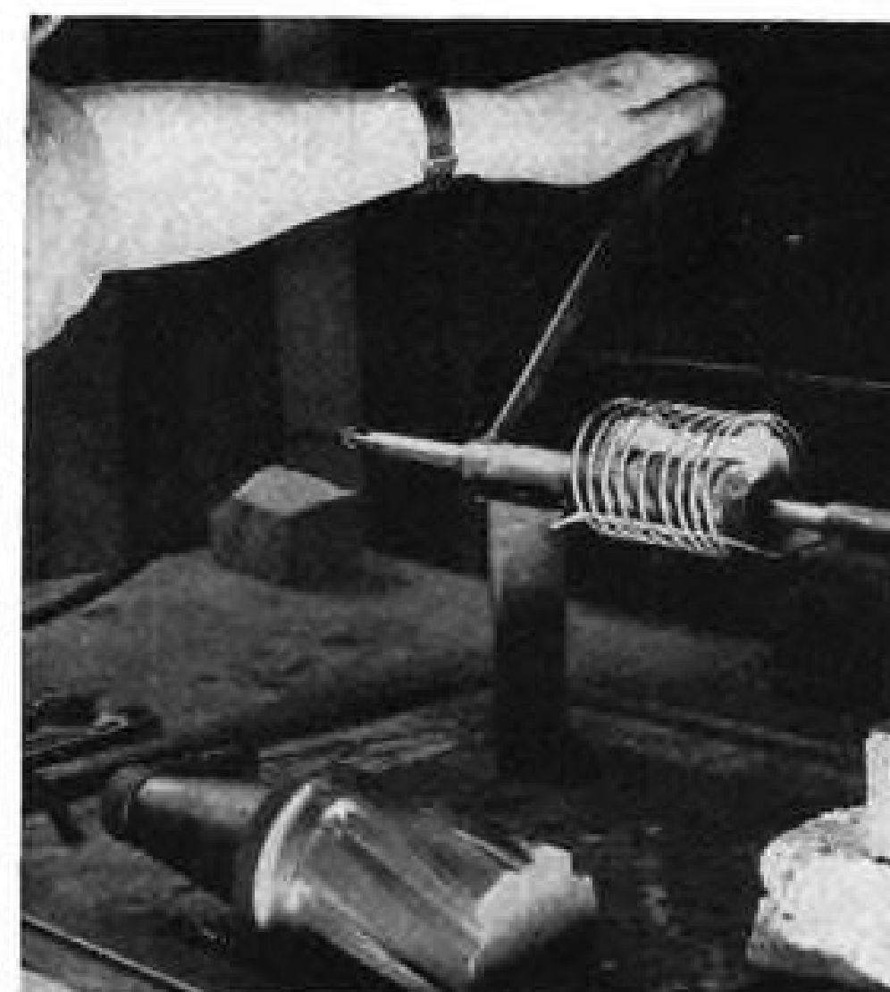
CARBIDE INSERT, at 2,200F in induction heater coil, is manually twisted and bent by Boeing-designed tool to proper angle.
