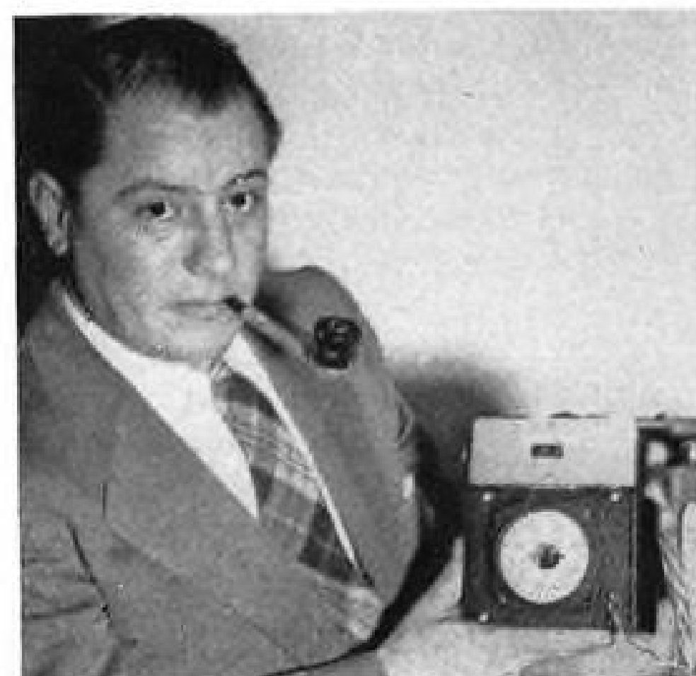
DME includes frequency selector (top) and distance indicator (dial, bottom).
