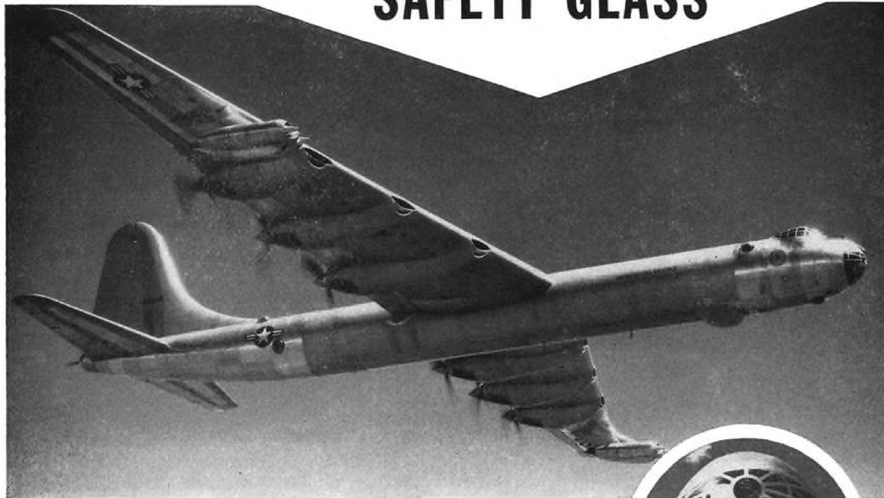
Six 3800-hp piston engines, plus four jet engines, power the Convair B-36, the world's largest bomber. The pilot's and bombardier's compartments are glazed with 85 separate pieces of Pittsburgh Flexseal Safety Glass.
