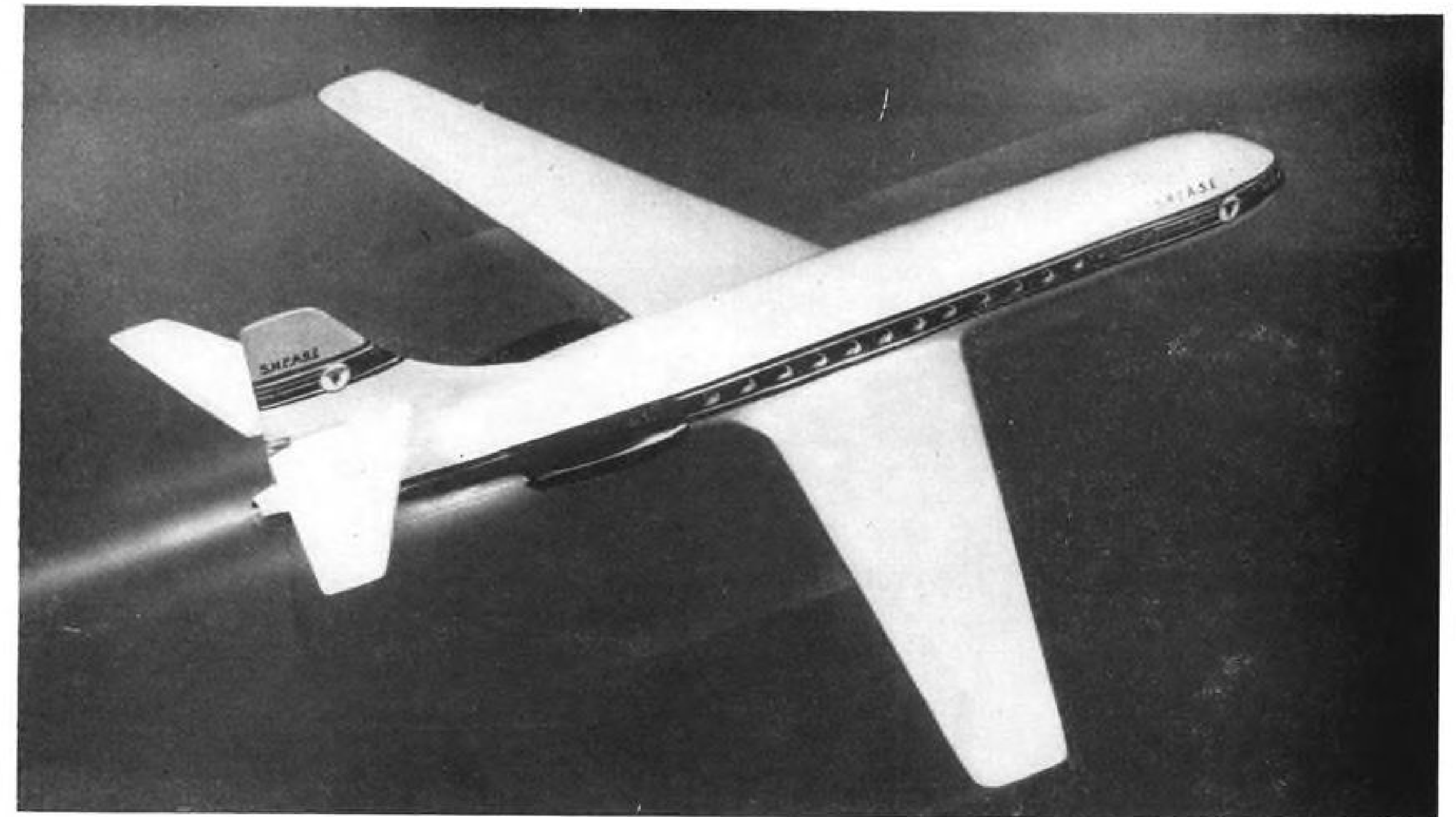
THREE-JET SNCASE medium transport, shown in model form, would have two 6,000-lb.-thrust Atar jets located behind the passenger cabin, another in the tail. Exhausts thus would not impinge on cabin. Freight would be stowed behind the cockpit.
