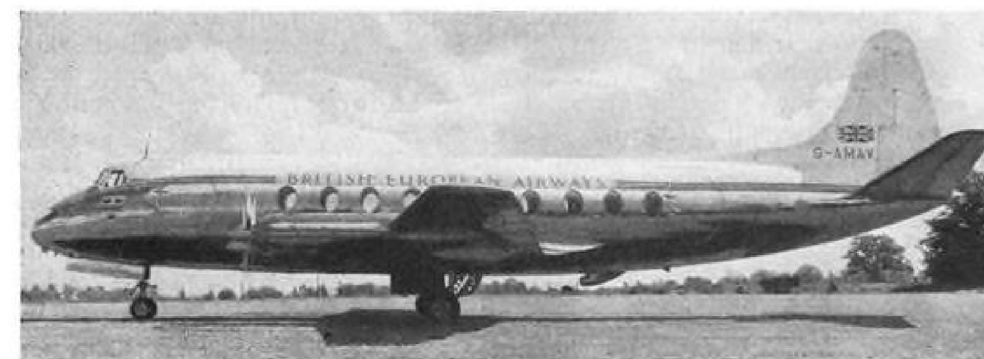
VISCOUNT 700 in colors of British European Airways is pre-production prototype of entire series. Ventral scoop is for cabin comfortization system.
