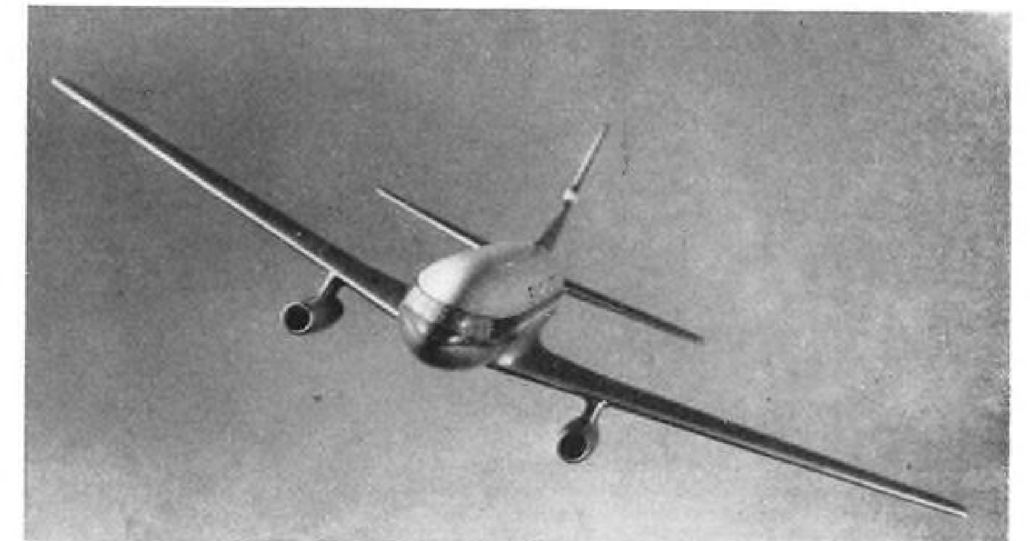
THREE-JET SNCASE medium transport, shown in model form, would have two 6,000-lb.-thrust Atar jets located behind the passenger cabin, another in the tail. Exhausts thus would not impinge on cabin. Freight would be stowed behind the cockpit.
