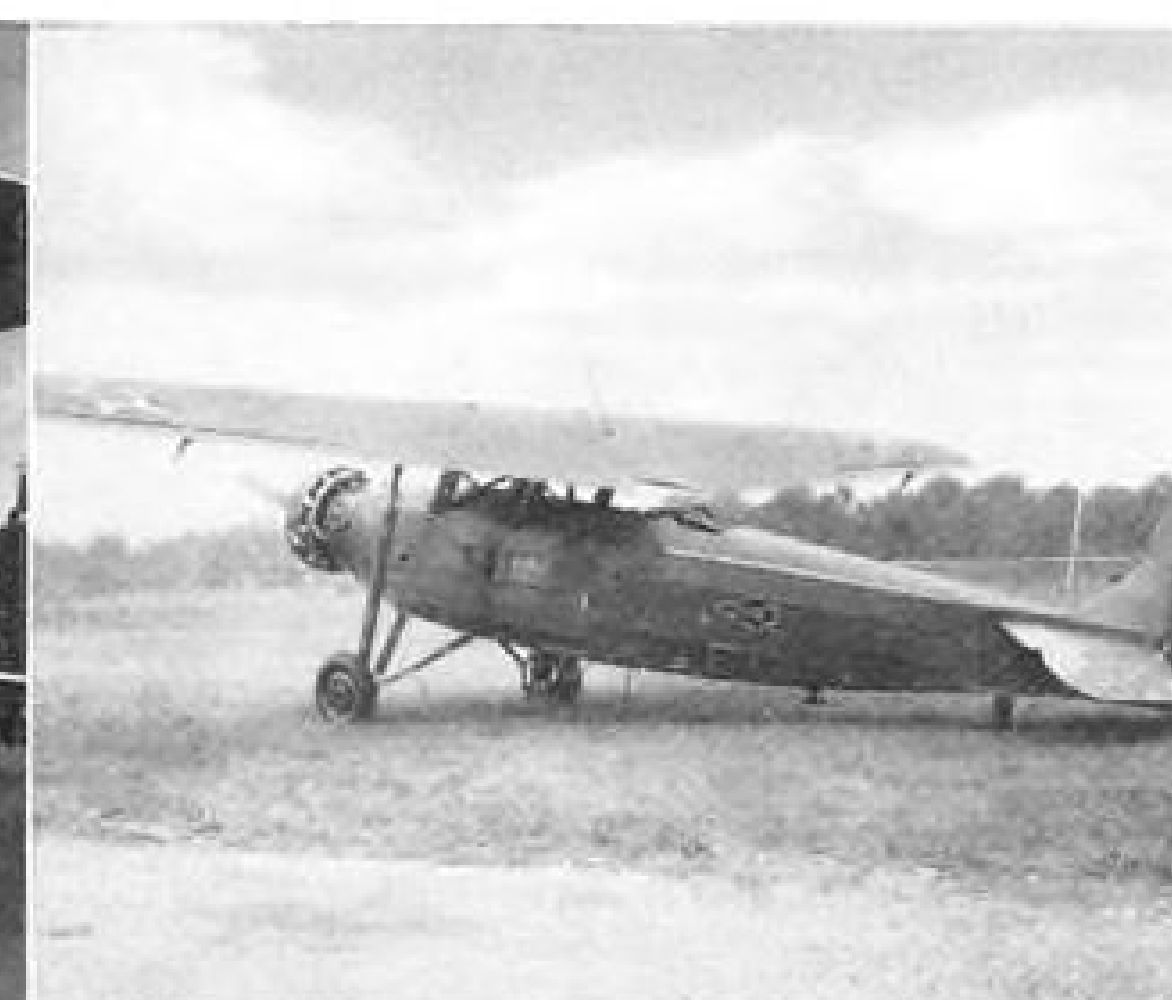
1937 First completely automatic landings were made by the U.S. Army Air Corps in 1937 by coupling radio aids to the Sperry automatic pilot.
