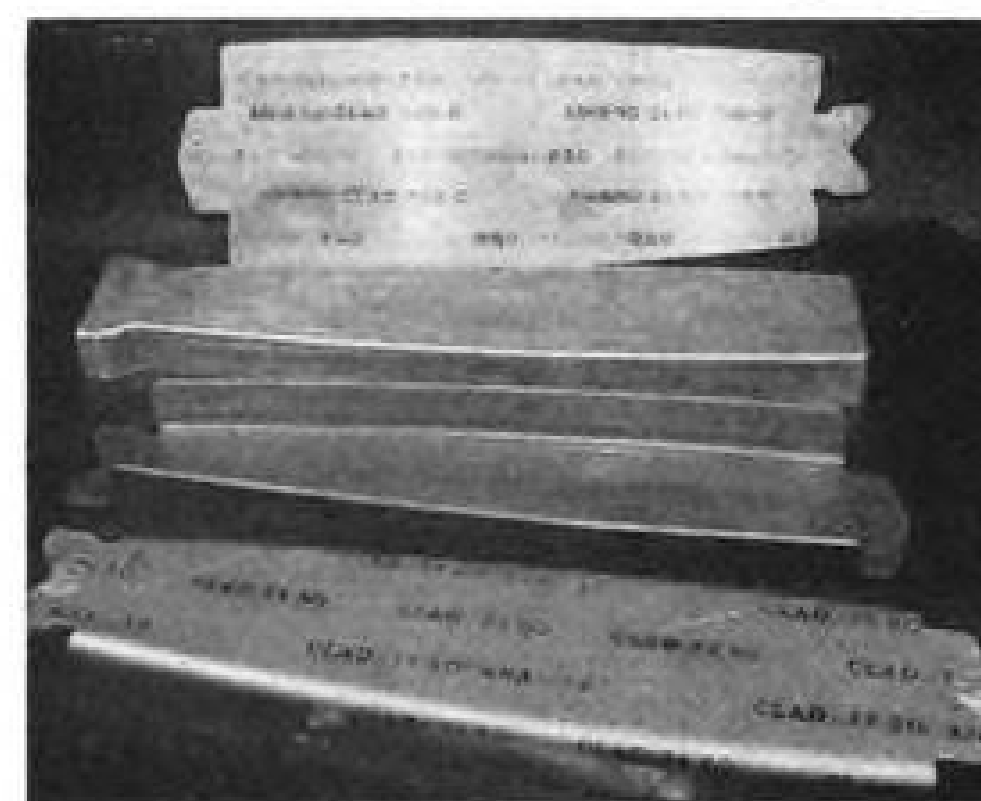
METAL BLANK of precut 75S aluminum (top) is formed on Wheelon press by Kirk-site block shown under the blank into parts in lower half of picture.
