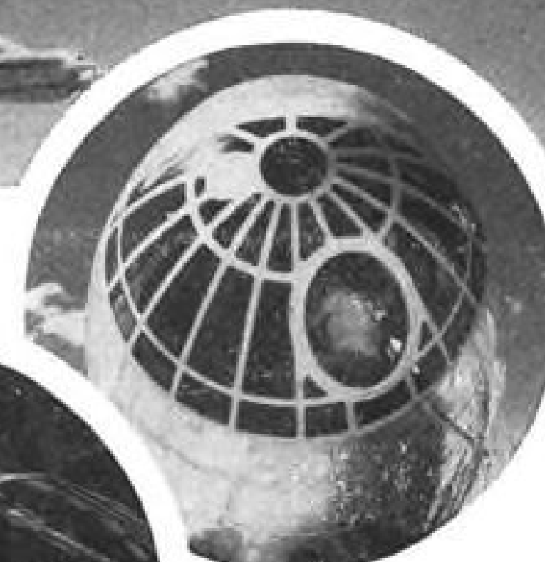
Bombardier's compartment of the B-36 is glazed with optically-excellent Pittsburgh Flexseal.
