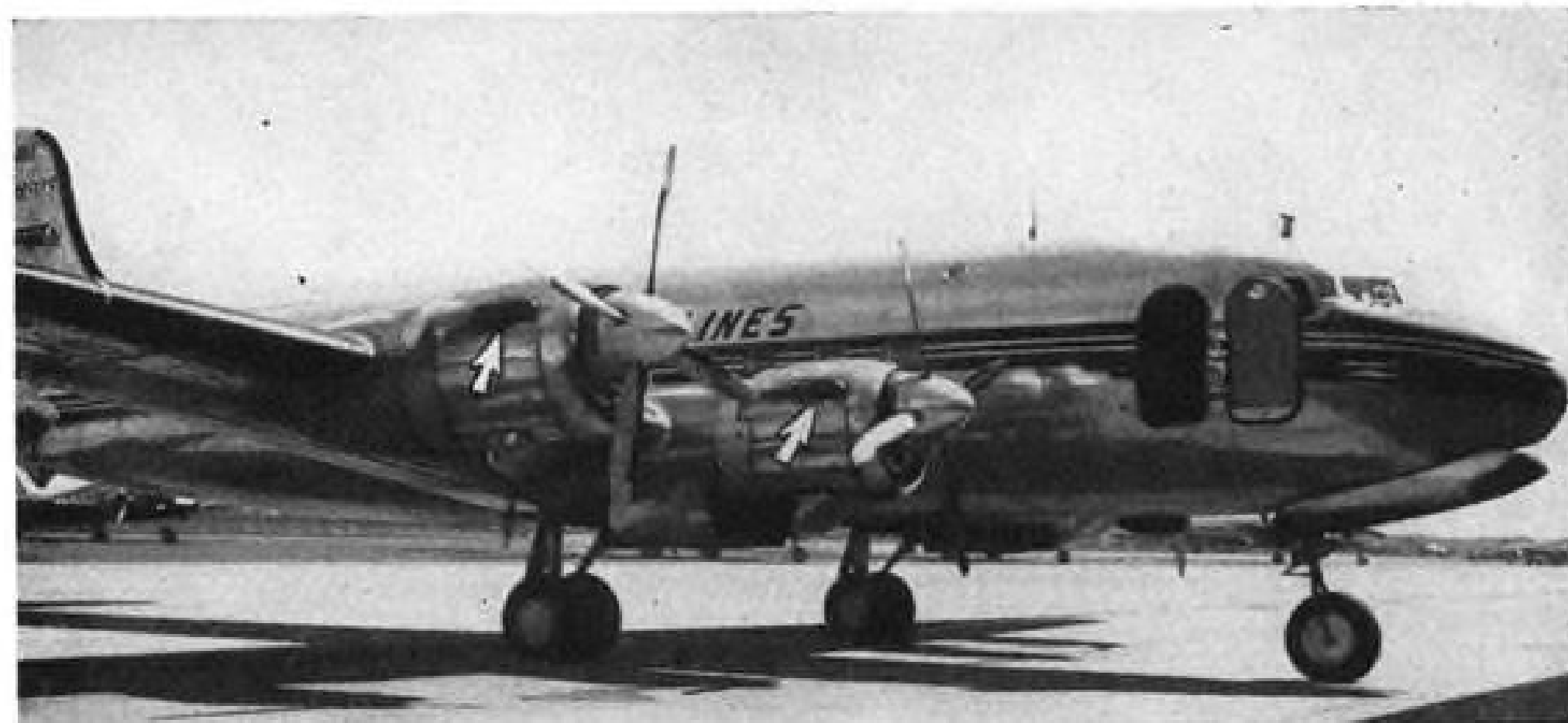
CROSS-OVER EXHAUST stacks (arrows) give TCA passengers a quieter ride.
