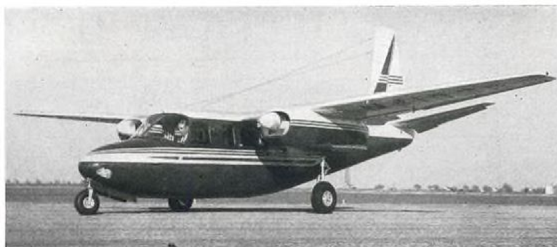
HIGH WING means good visibility and low step out of cabin of Aero Commander. Note exhaust augmentor system on outboard side of nacelle, and extremely clean cowlings.
