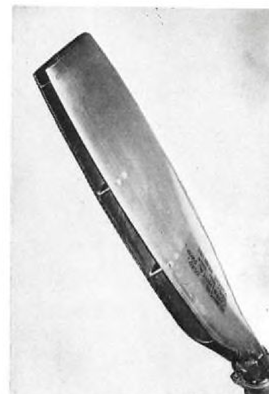
SLOTTED STRIP keeps air from hitting prop blade flatly, eliminates zoom.
