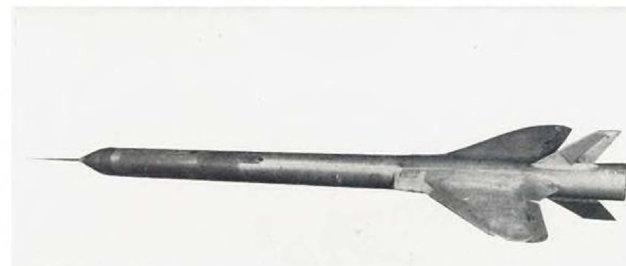
SCALE-MODEL WING of delta fighter is fixed near tail of 5-in. rocket for . . .
