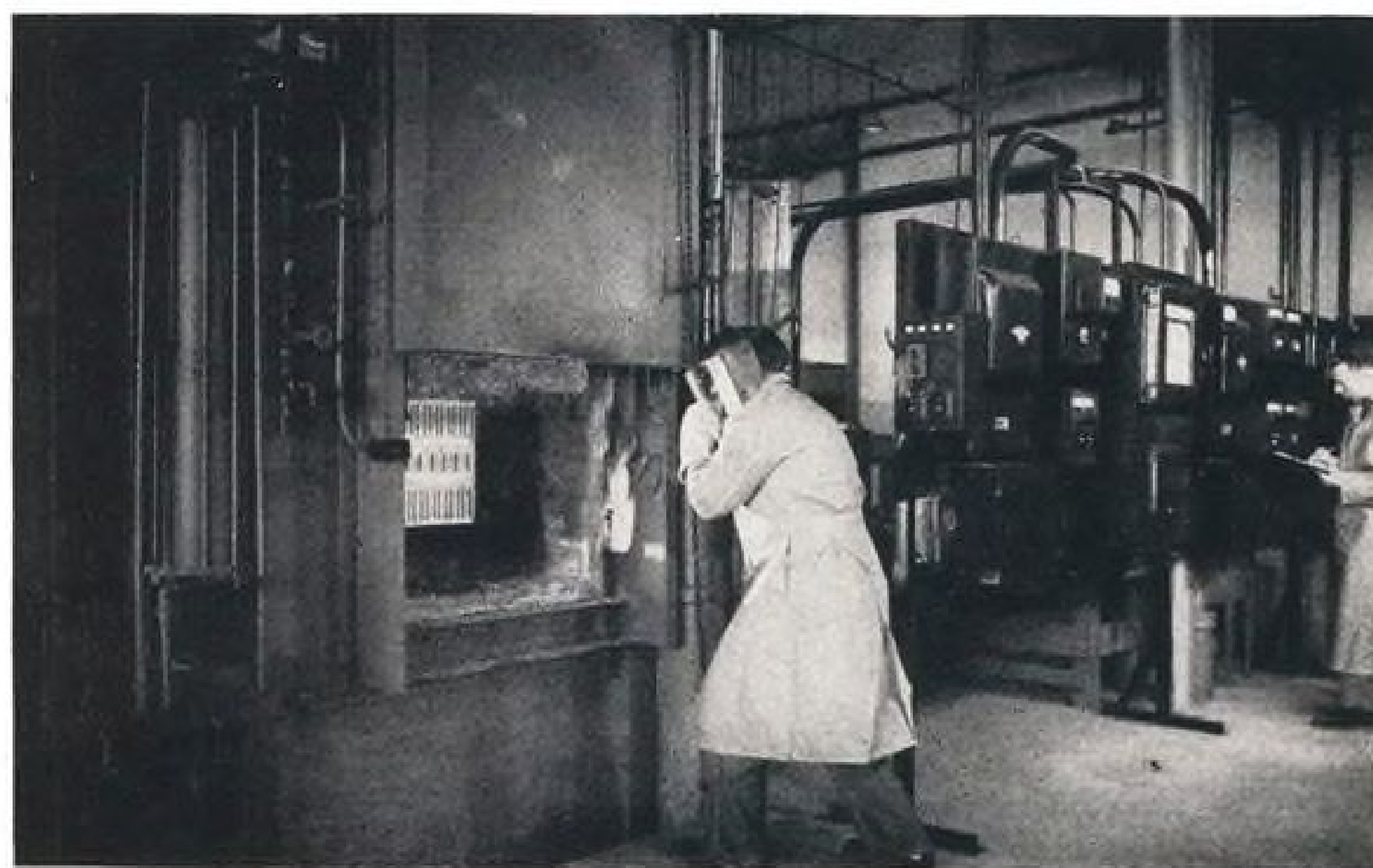
ASSEMBLED CORE is brazed in furnace after carefully controlled preheat.
