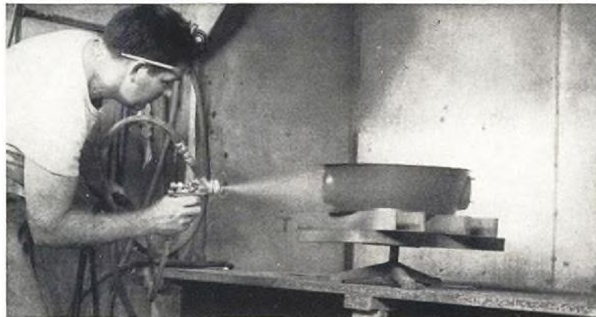
SPRAYED ceramic coats turbosupercharger exhaust hood (other methods of application are dipping and hand-brushing), preparing part to be . . .
