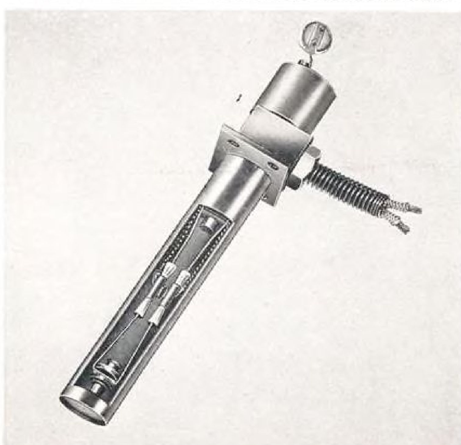
CUTAWAY VIEW of Fenwal THERMOSWITCH control shows enclosed electrical contacts. The temperature-sensitive shell expands or contracts instantly with temperature changes, thus making or breaking the contacts. Fenwal units are compact, highly resistant to shock, vibration and extreme temperature conditions. For complete data on these and other Fenwal aircraft controls, write FENWAL, INCORPORATED, 126 Pleasant Street, Ashland, Mass.
