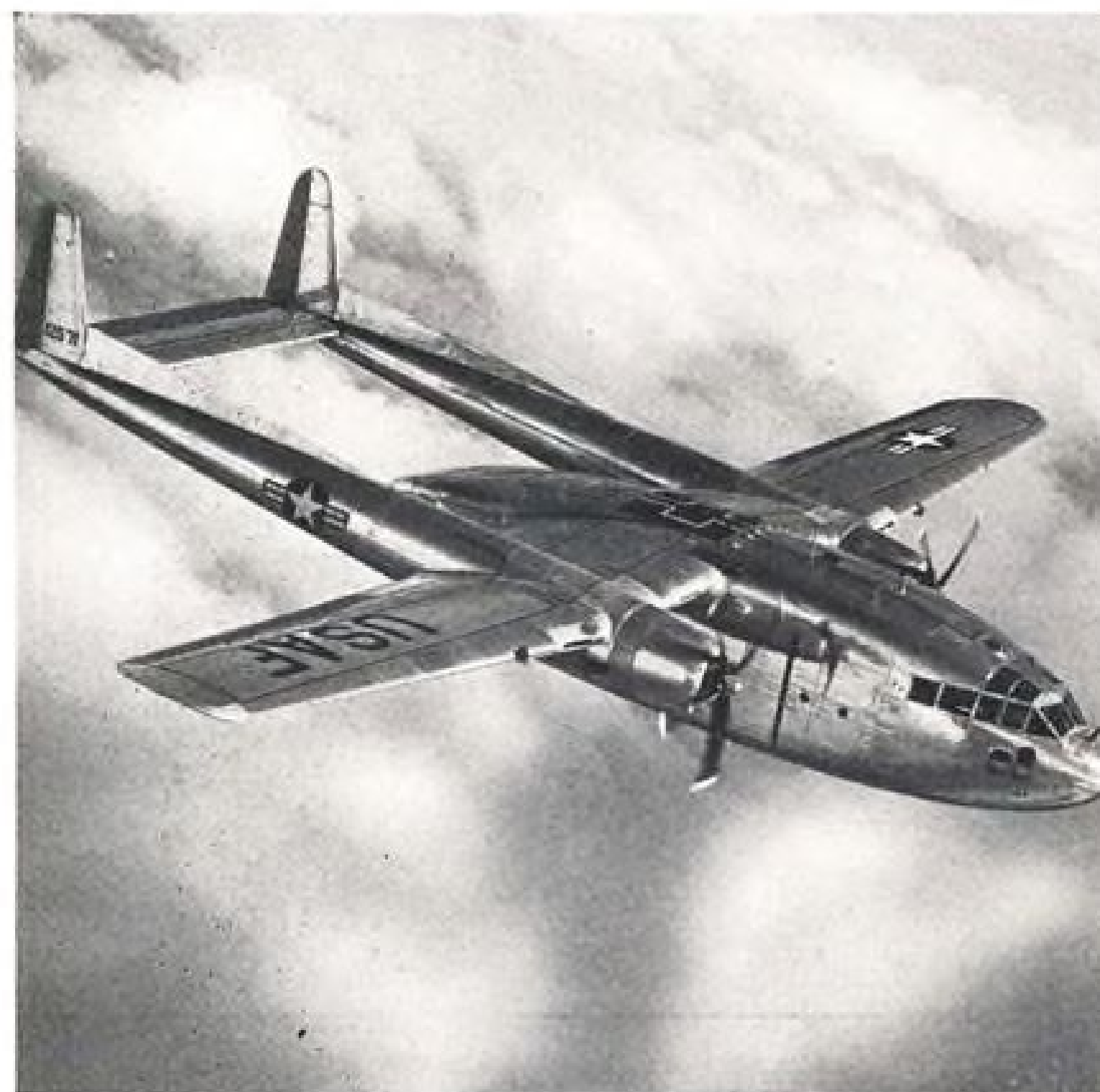
IN THIS C-119 FAIRCHILD "FLYING BOXCAR," hot air heats the crews' quarters and provides anti-icing protection for wing and tail surfaces. Eight unit heaters produce the hot air which must be maintained at a constant temperature. That job is effectively handled by 32 Fenwal THERMOSWITCH® controls . . . four to each heater.
