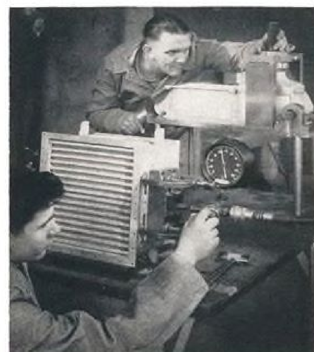
STRAIGHT FIN is equal to round tube in heat exchanger properties.
