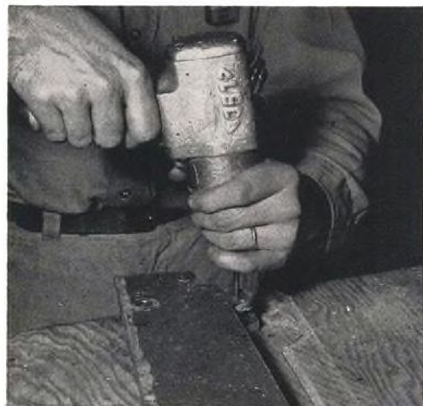
LEFT: CLECO A-3 Impact Wrench driving 1/4" x 3" screws into router table at Douglas Aircraft Company's Santa Monica plant.
