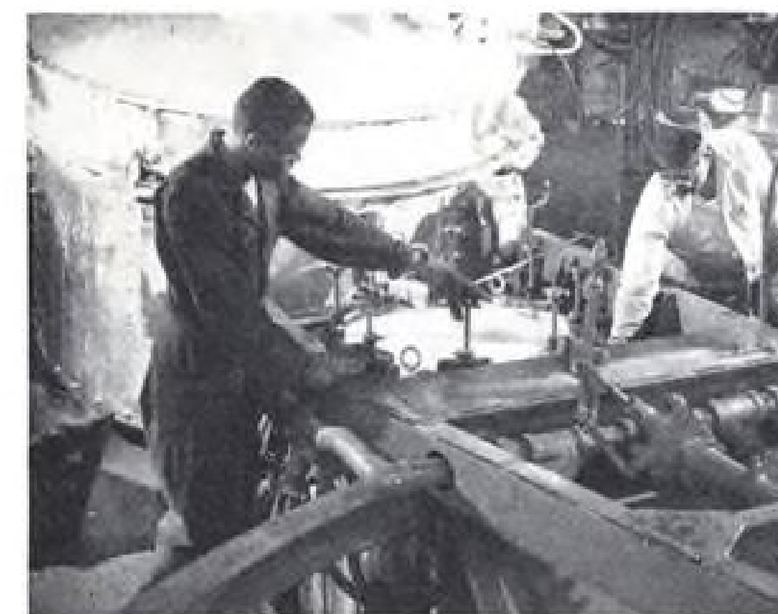
Here the direct casting process turns out ingot logs of any aluminum alloy. Harvey produces aluminum extrusions in special shapes, bar stock, forging stock, tubing and related mill products under the most exacting metallurgical control.
