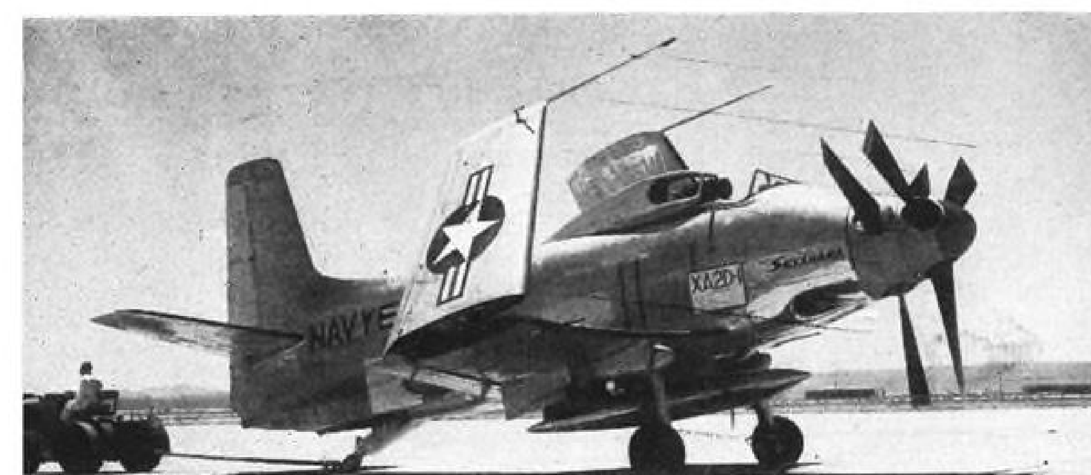
DOUGLAS XA2D-1 SKYSHARK—Big, attack plane (left) with wings folded being towed before Aviation Writers at Edwards AFB, Calif. Powered by Allison T40 turboprop engine turning contrarotating three-blade Aeroproducts props, the Skyshark is one of the planes being pushed for production by APB (see p. 13). It was initially ordered on limited scale. This plane is fitted with a streamlined auxiliary tank under the fuselage, carries two 20-mm. cannon in each center wing section.
