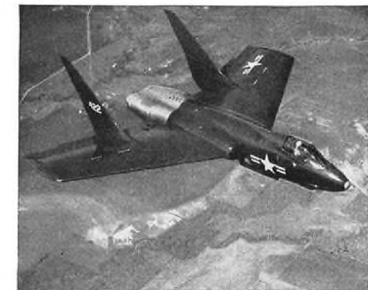
Flight of the Chance Vought Cutlass, seventh in a line of outstanding fighters and "potentially capable" of flying faster than any other service type jet aircraft in production, land or carrier-based. Substantial surface areas of the Cutlass are constructed of painted Alodized aluminum.
