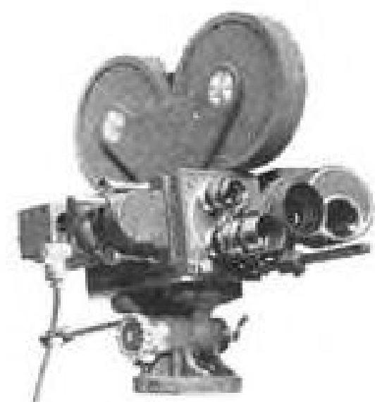
THE MAURER 16MM. , designed specifically for professional use, equipped with precision high-power focusing and view-finder. Standard equipment includes: 235" dissolving shutter, automatic fade control, view-finder, sunshade and filter holder, one 400-foot gear-driven film magazine, a 60-cycle 115-volt synchronous motor, one 8-frame handcrank, power cable and a lightweight carrying case.
