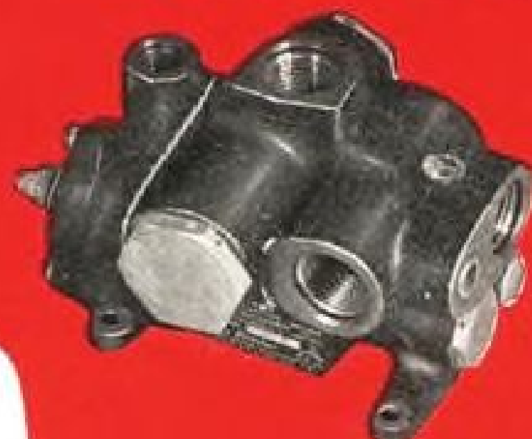
COMPENSATED PRESSURE REDUCER ... Outlet pressure is varied as a function of a secondary system. Example: Hydraulic pressure is proportional to fuel pressure — etc.
