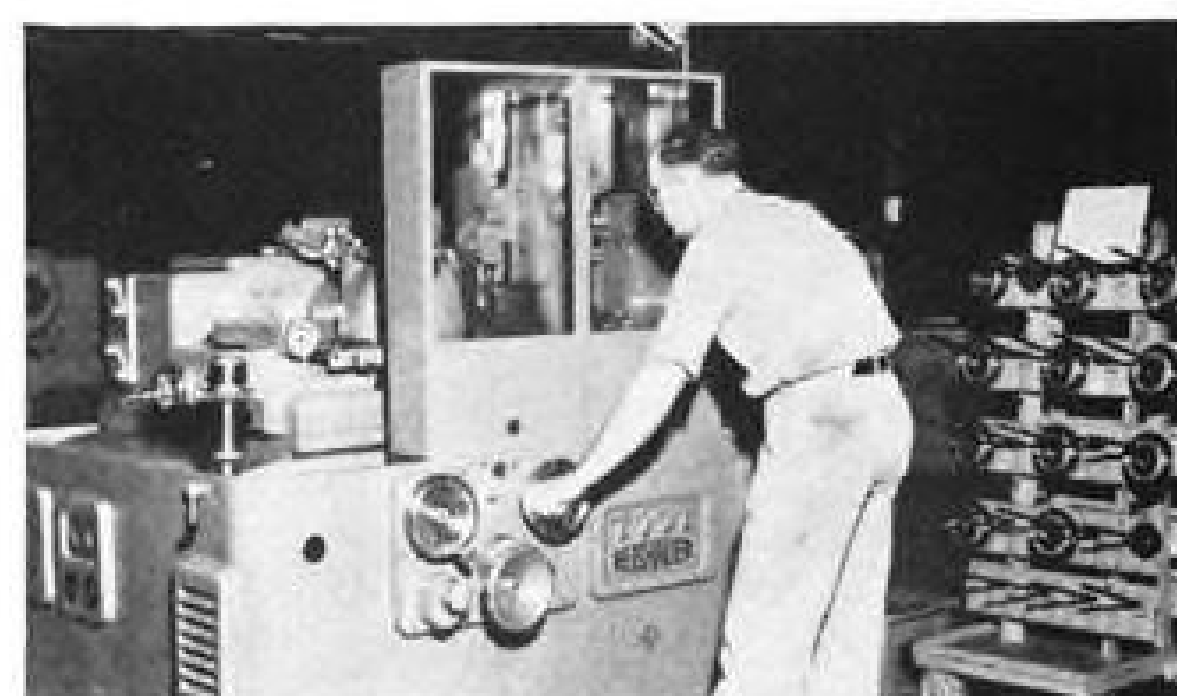
NEW MACHINE grinds gears to tolerances of .0003 inches. Modern machinery like this speeds jet manufacture.
