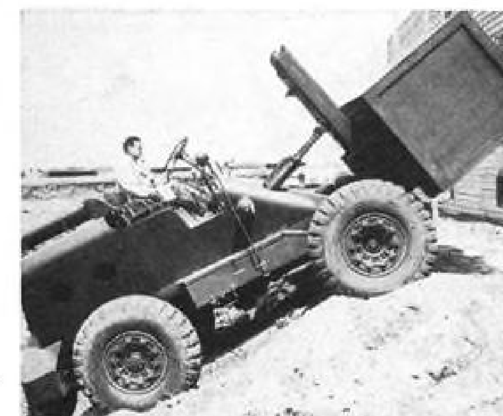
ALL-AROUND fork lift truck climbs 45 deg.
