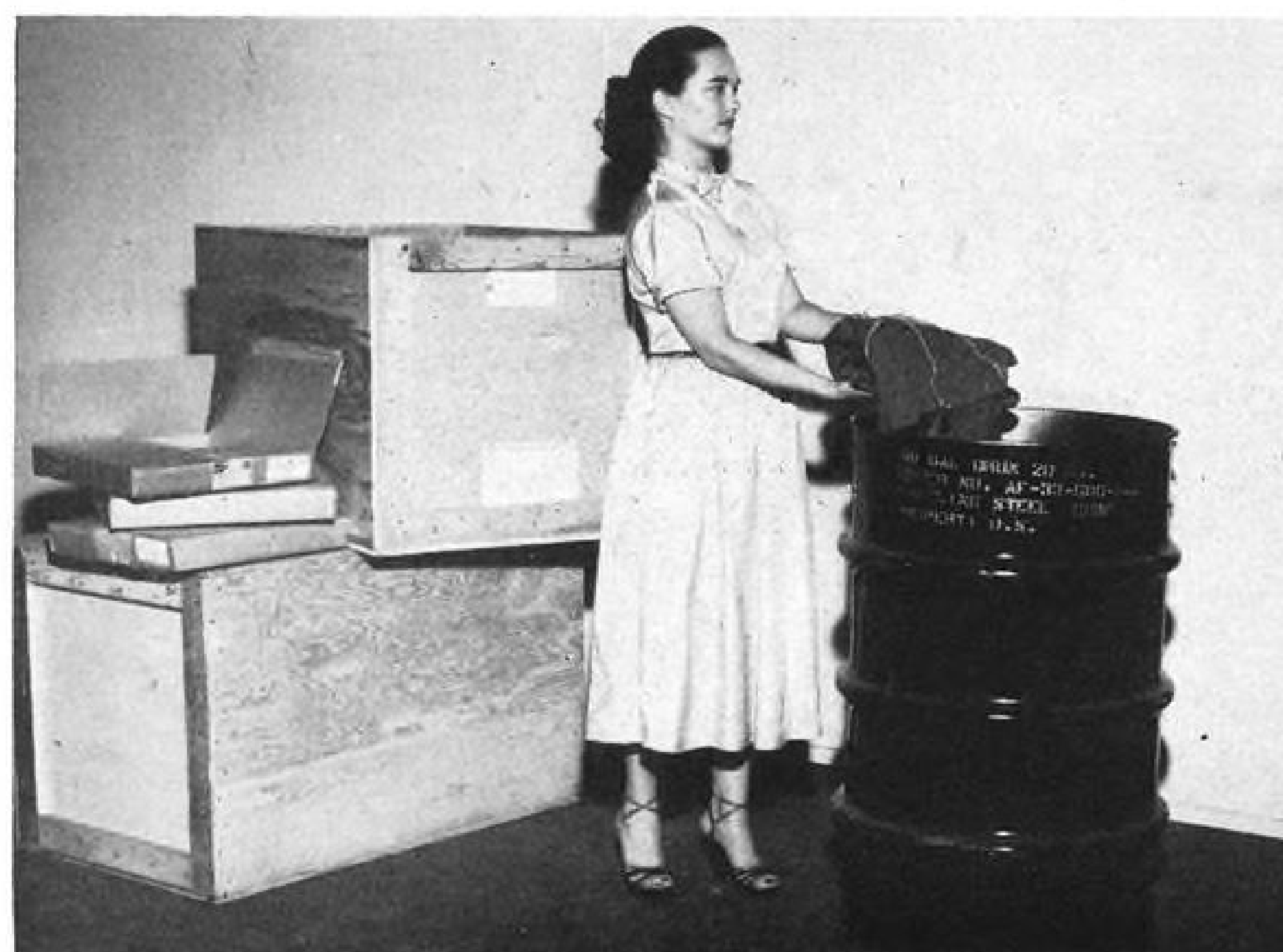
FULLY PACKED cans of clothing are cheaper to ship than large wooden crates, give better protection, and can be re-used.
