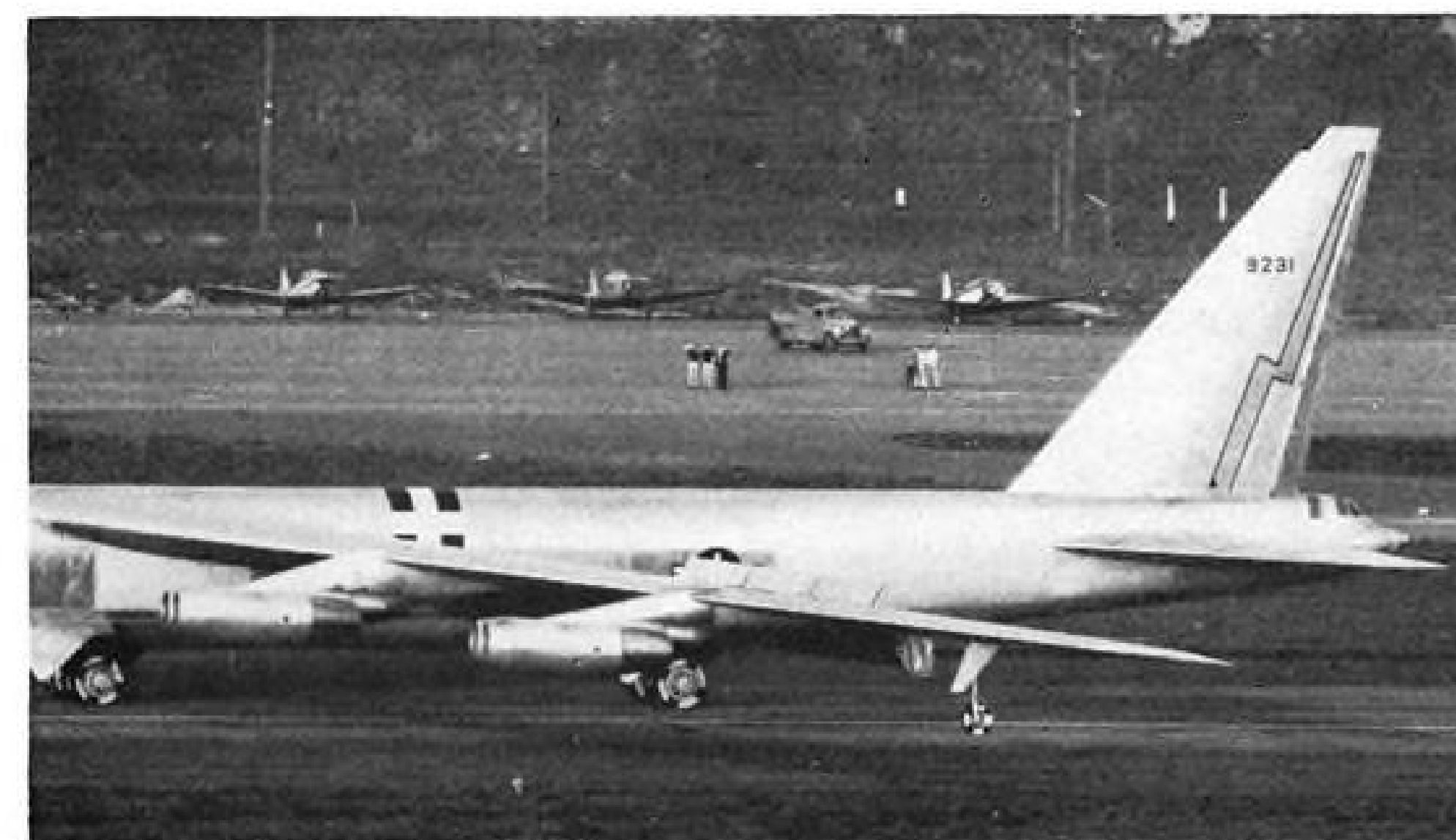
SPOILERS break the clean lines of the Boeing B-52's swept wing. These surfaces, made up of three sections probably capable of independent operation, form part of the lateral control system. Spoilers replace adverse yaw characteristics with favorable ones.
