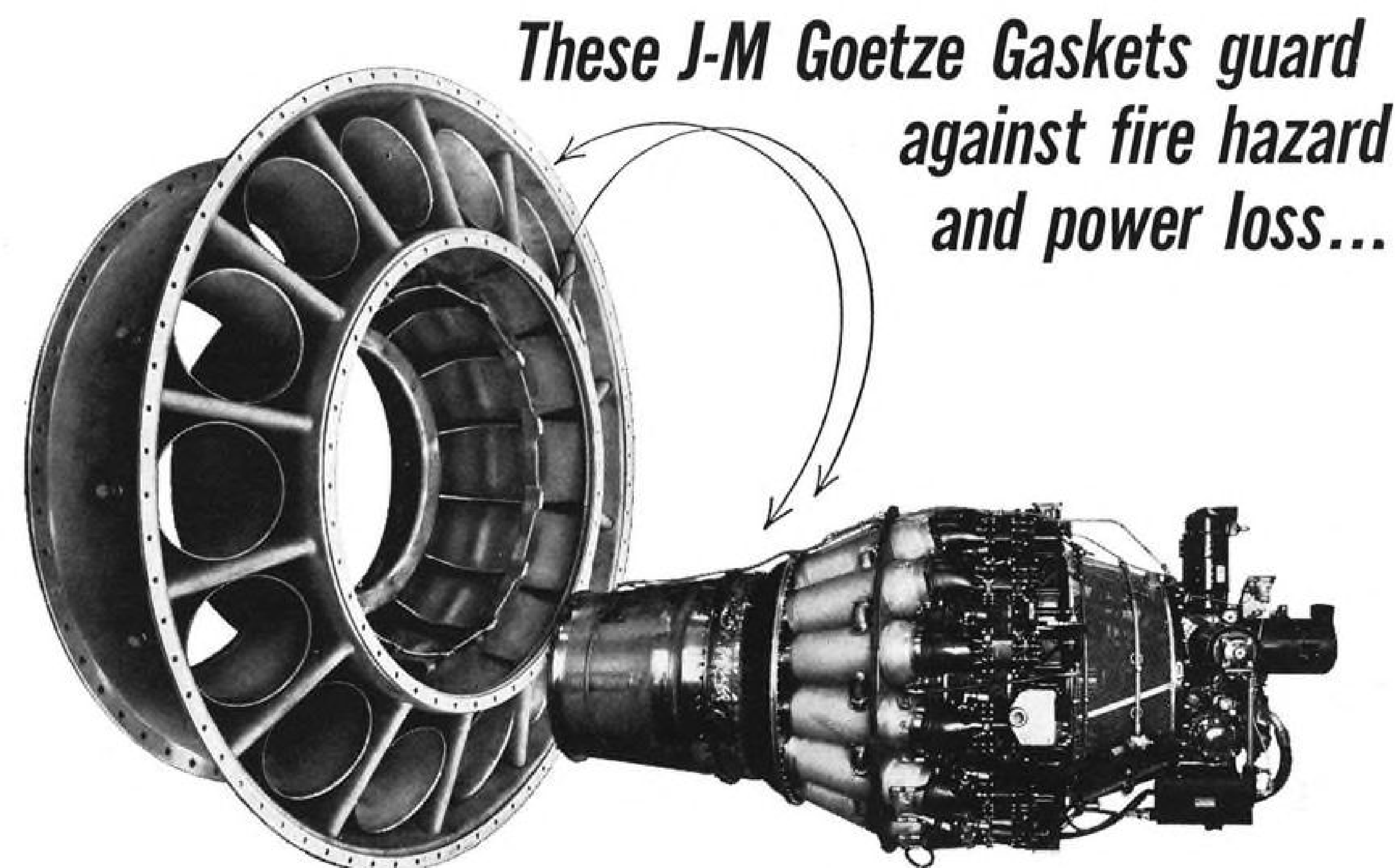
Arrows point to J-M Goetze metallic gaskets on the inner and outer annulus, and their approximate location on the J33 turbojet engine turbine frame.
