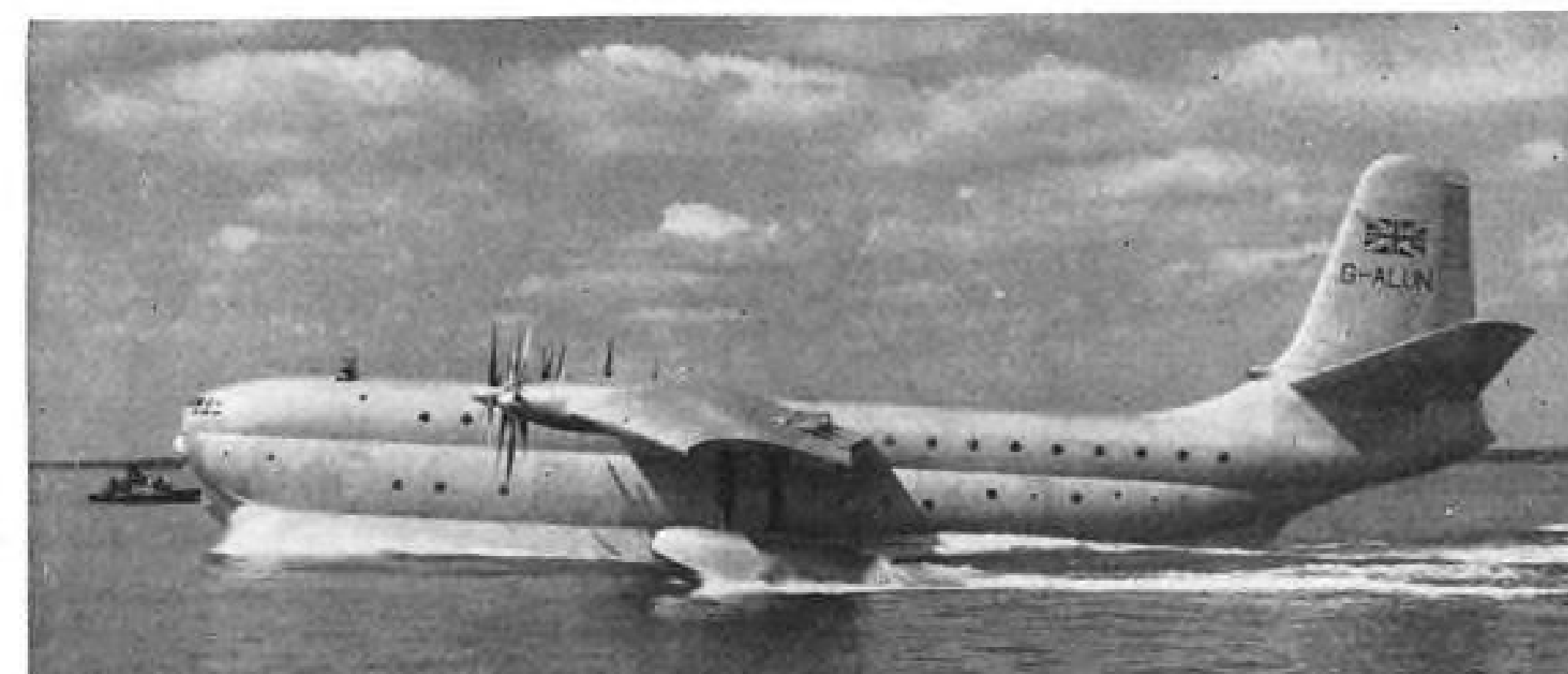
SAUNDERS-ROE PRINCESS is 140-ton flying boat powered by ten Bristol turboprops.
