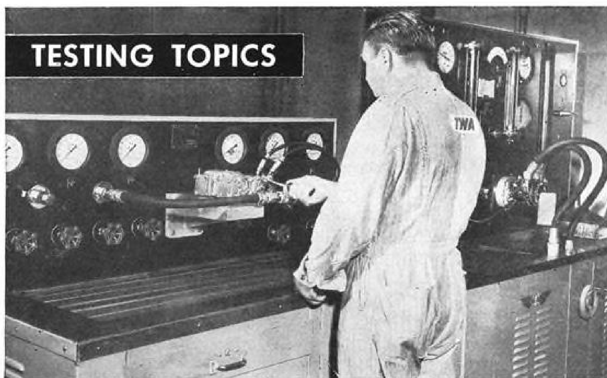
TESTING TOPICS GREER OIL RADIATOR TEMPERATURE CONTROL VALVE STAND is shown here checking operation of thermostatic control and surge relief valve used with aircraft oil radiators under low, normal and high temperatures. At right is the Greer Vacuum Pump Tester for testing complete performance of vacuum pumps.
