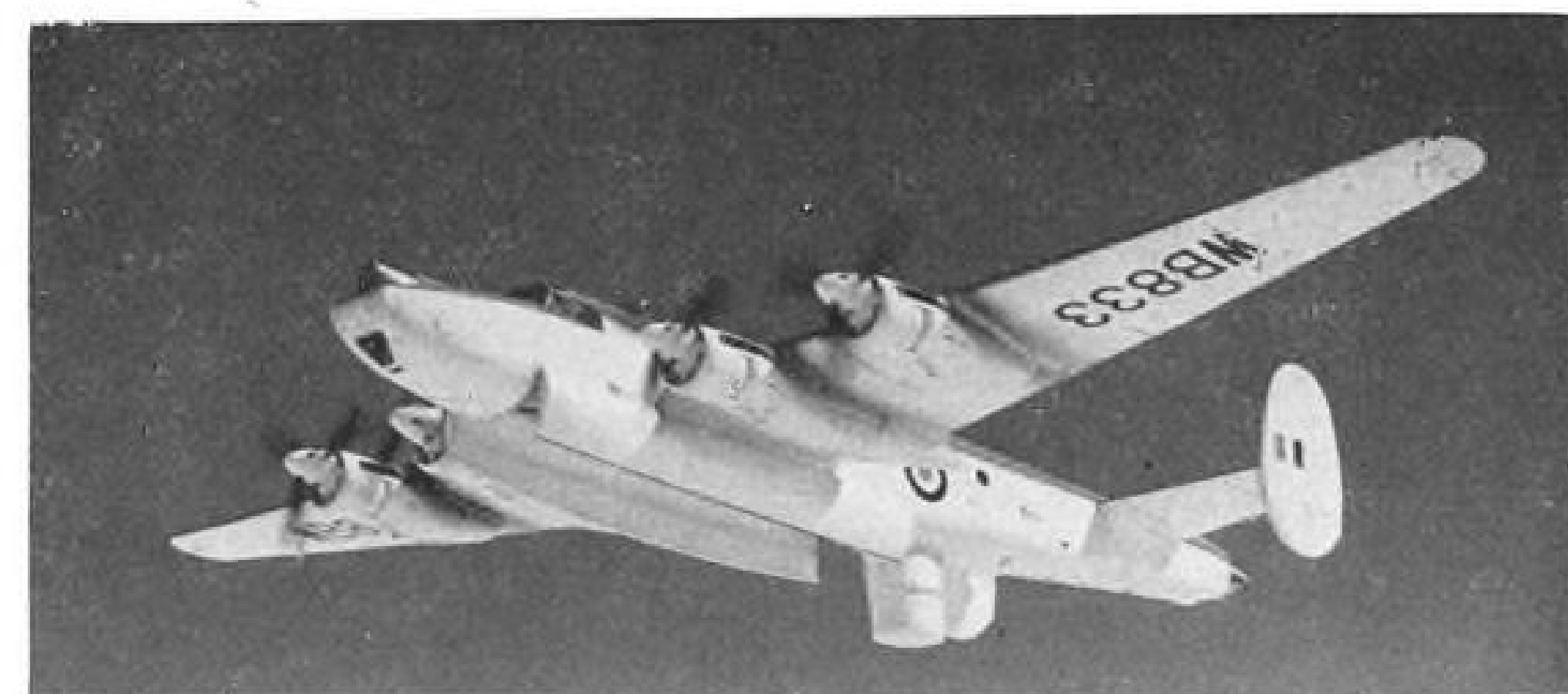
AVRO SHACKLETON 2 sub hunter-killer shows cleaner nose, relocation of radome.
