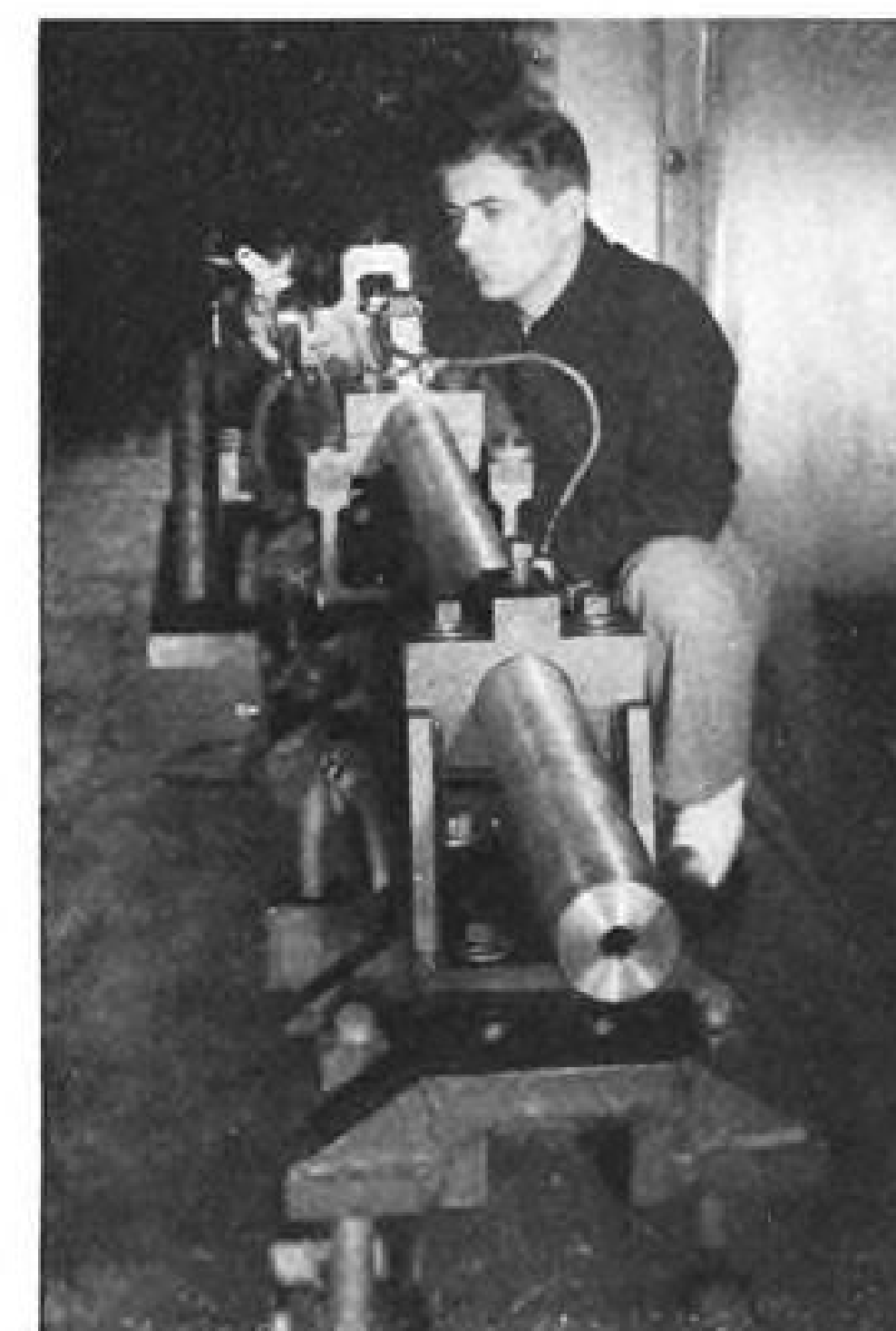
LAUNCHER fires models of missiles into supersonic gale to add velocities of bullet and wind for higher Mach numbers. Model of missile (right) enclosed in plastic sabot is ready for firing. Clear plastic portion breaks away radially from missile after leaving muzzle of launcher; base of sabot tumbles and lags far behind model.
