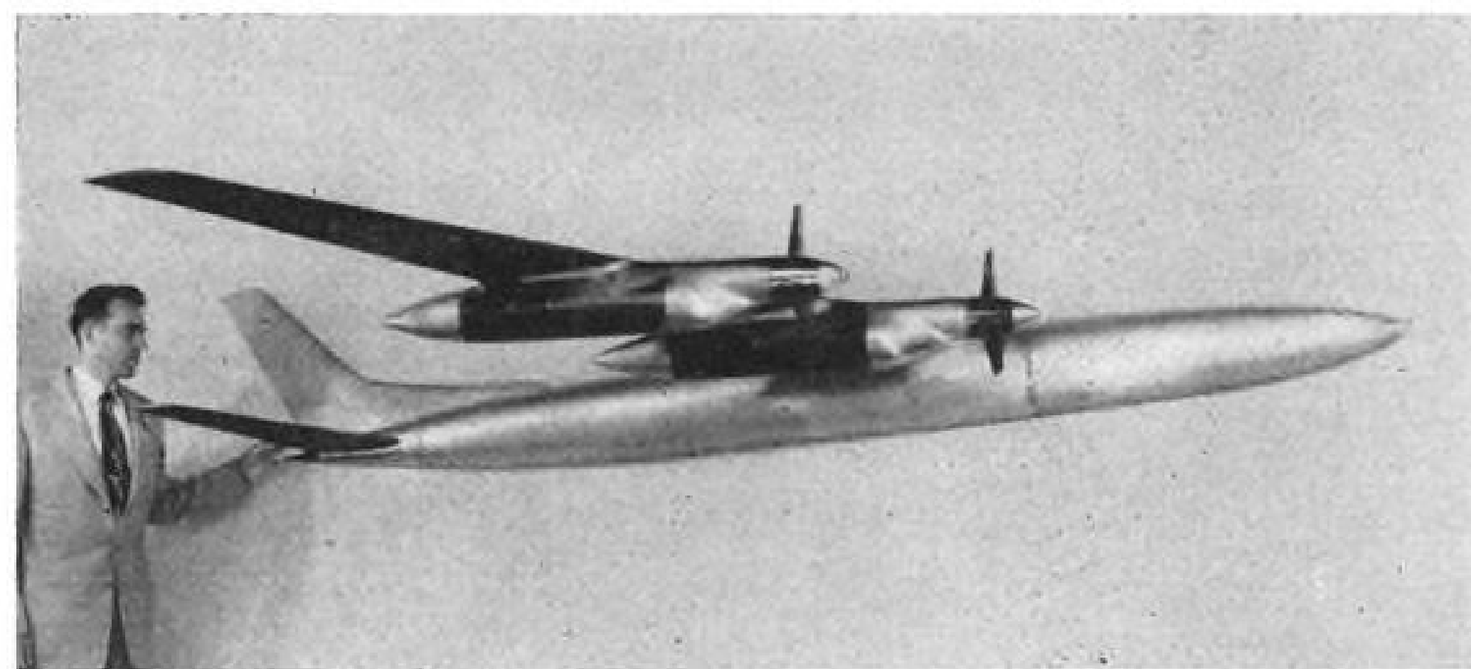
NACA MODEL of sweptwing turboprop-powered plane undergoing tunnel tests.
