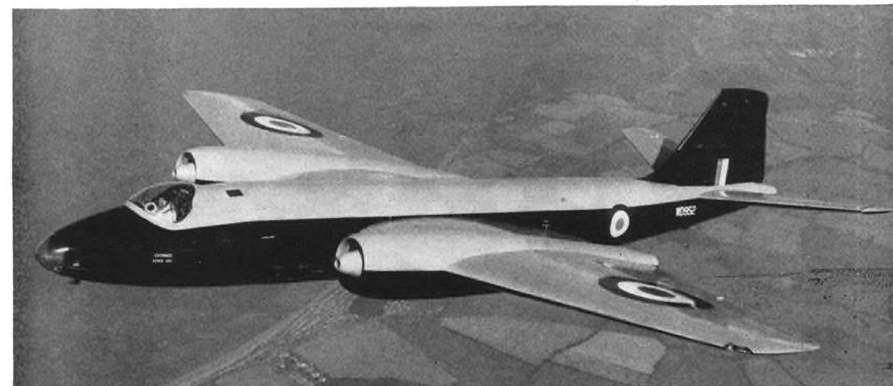
BRISTOL OLYMPUS TESTBED is this twin-engine English Electric Canberra which is gathering flight data on the powerful split-compressor engines. Installation problems have prevented engineers from pulling full thrust capabilities from the Canberra experimental rig.
