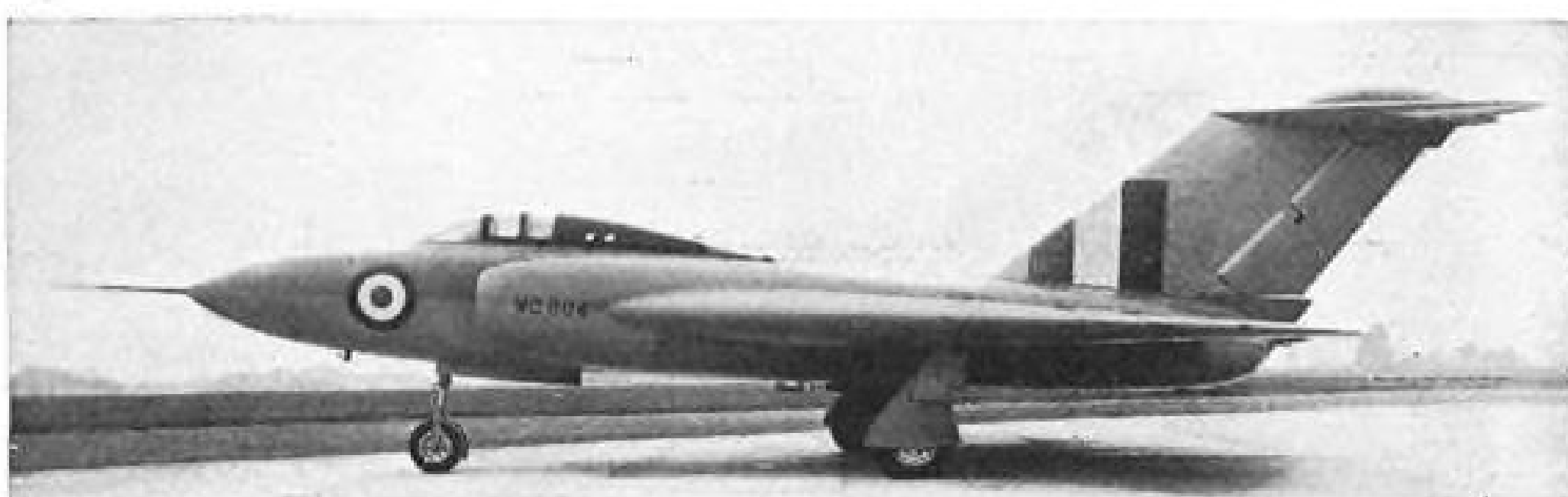
STANDING JAVELIN shows low angle of incidence. Contrast tailpipe lines in this early picture of prototype with later picture of same plane, p. 21.
