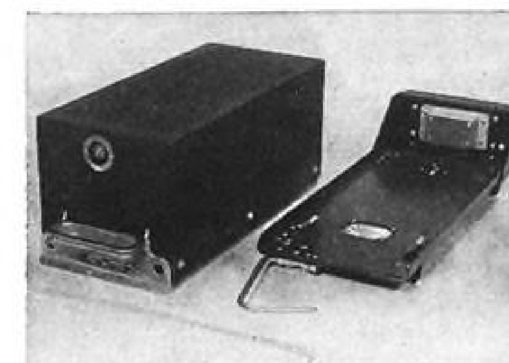
AVR-22 UNIT can be mounted compactly in a standard plug-in type of tray.
