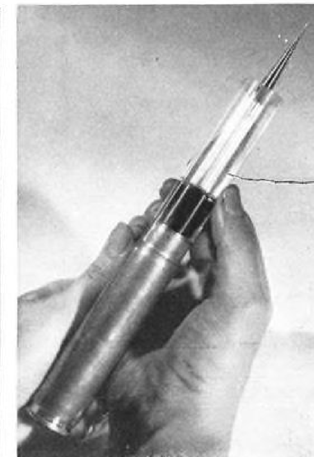
LAUNCHER fires models of missiles into supersonic gale to add velocities of bullet and wind for higher Mach numbers. Model of missile (right) enclosed in plastic sabot is ready for firing. Clear plastic portion breaks away radially from missile after leaving muzzle of launcher; base of sabot tumbles and lags far behind model.
