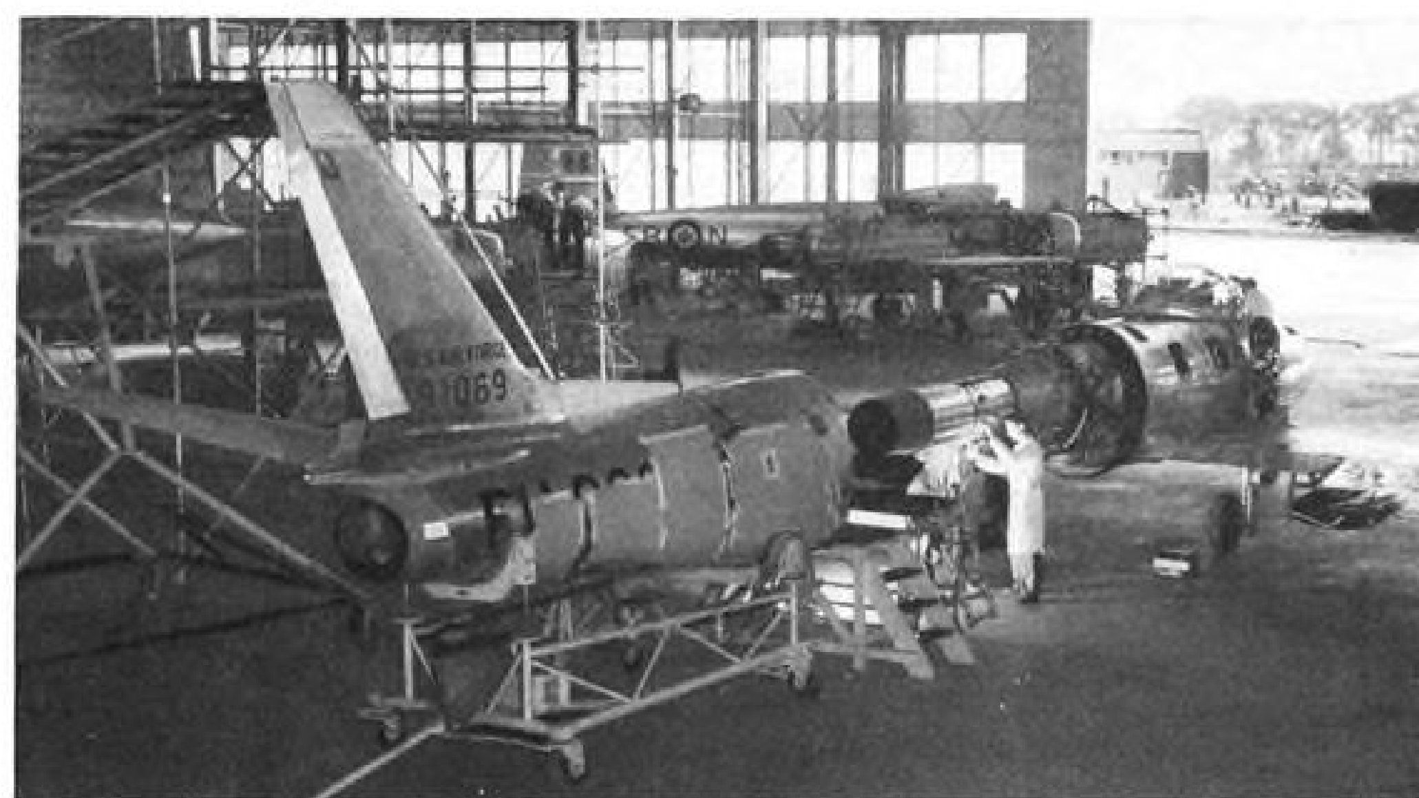
ORENDA POWERPLANT will be mass-produced in Avro's new Malton plant. It will drive Canadair-built F-86 (foreground) and Avro CF-100 twin-jet fighter (background). Thrust of Orenda has been reported as slightly over 7,000 lb.
