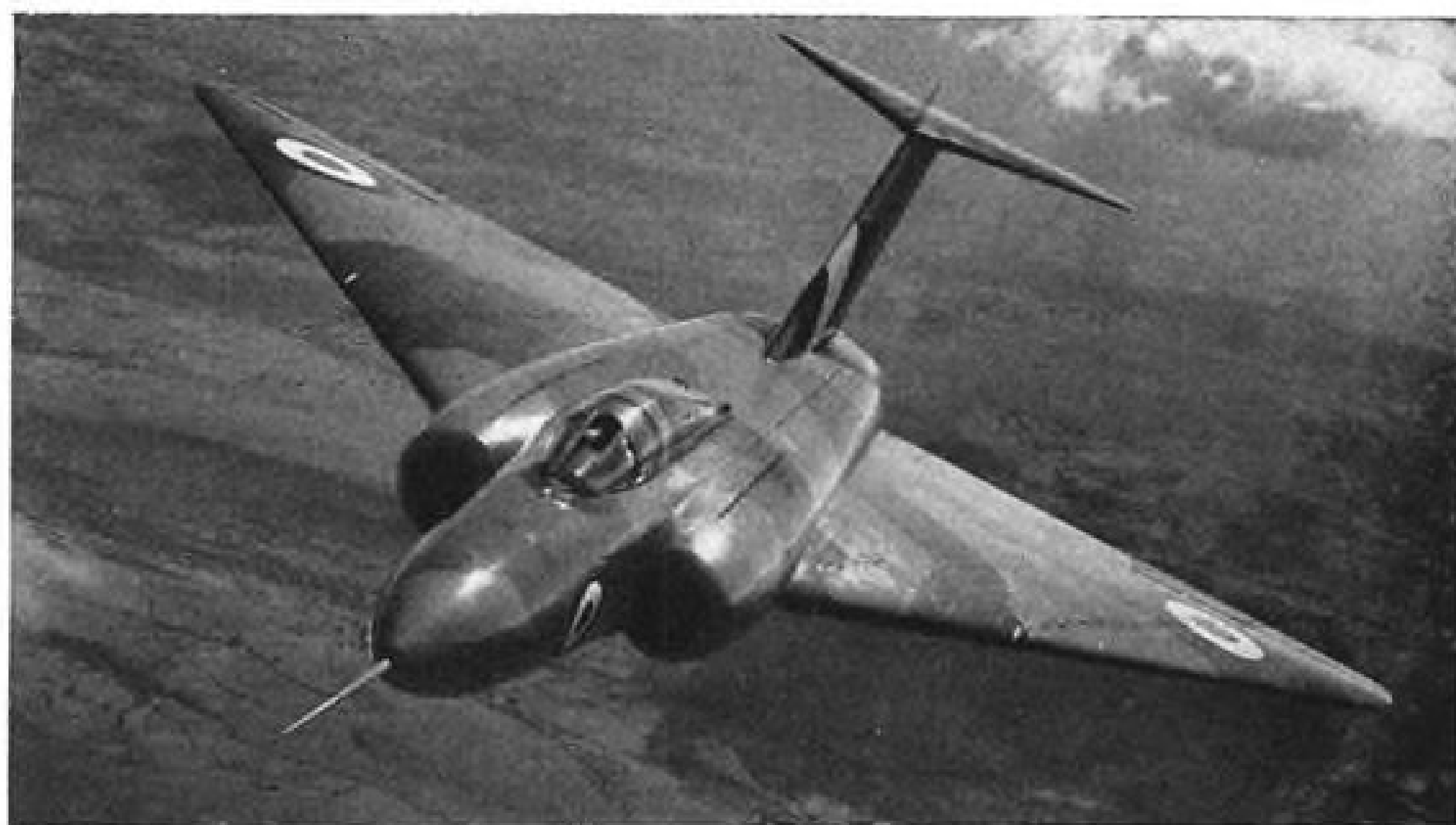
BANKING JAVELIN shows flat, wide-beamed fuselage and round air intakes.
