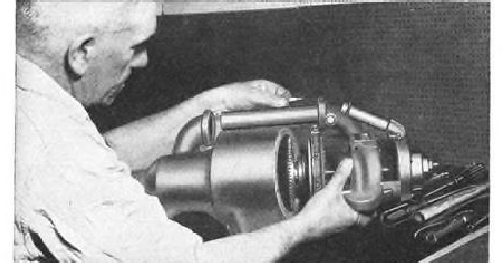
REHEAT FUEL PUMP bleeds air from jet engine to supply extra flow of fuel for afterburner operation.
