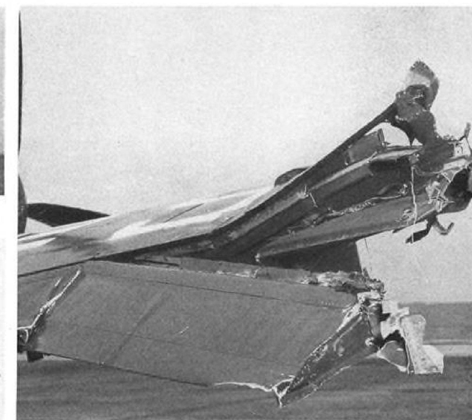
DAMAGED WINGTIP having some five feet shorn off and the aileron torn from its starboard hinge.
