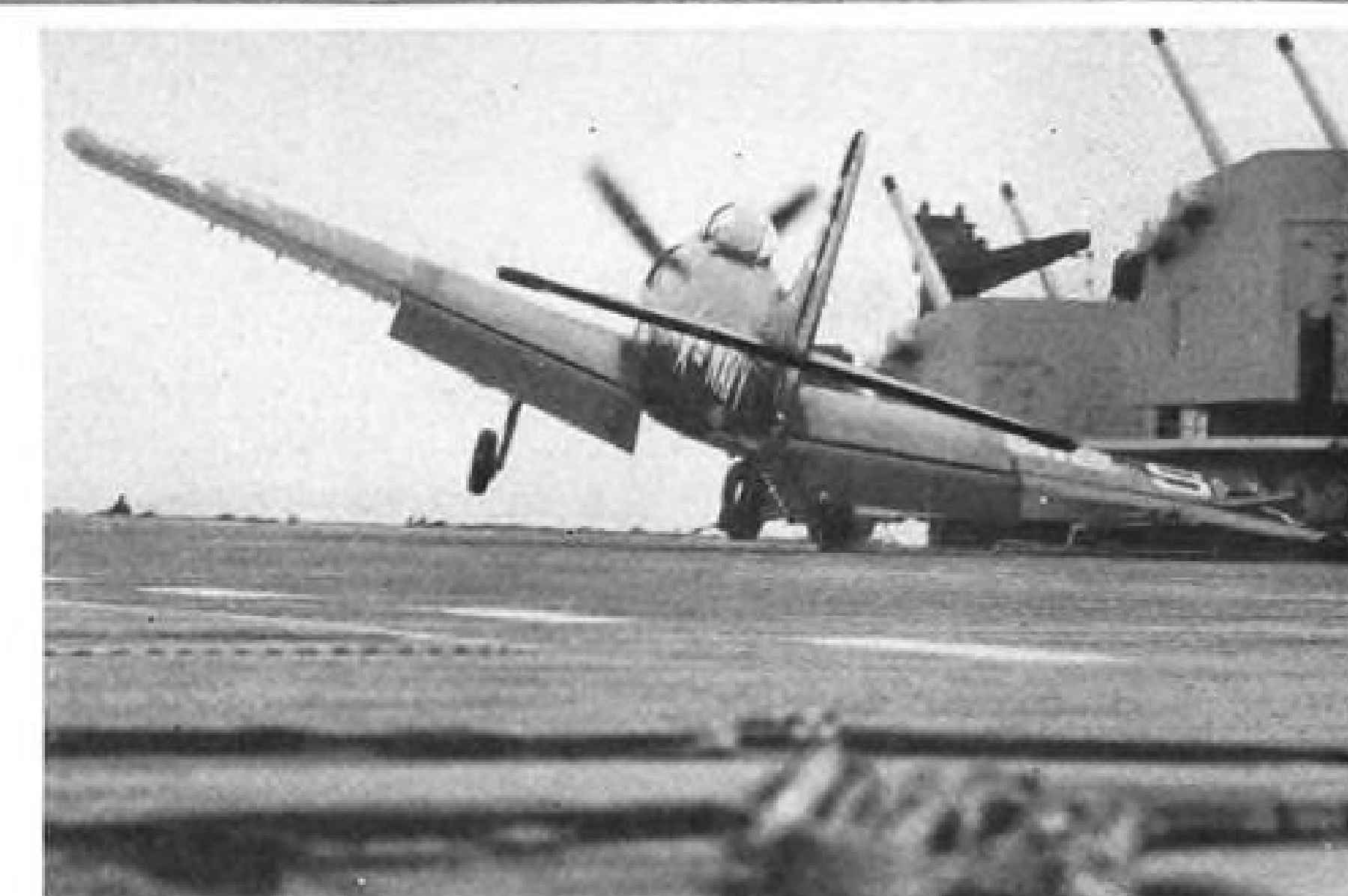
HAVING BOUNCED over the barriers, AD-4 Skyraider (above) strikes the carrier's island with its right wing and pieces fly. Then it . . .
