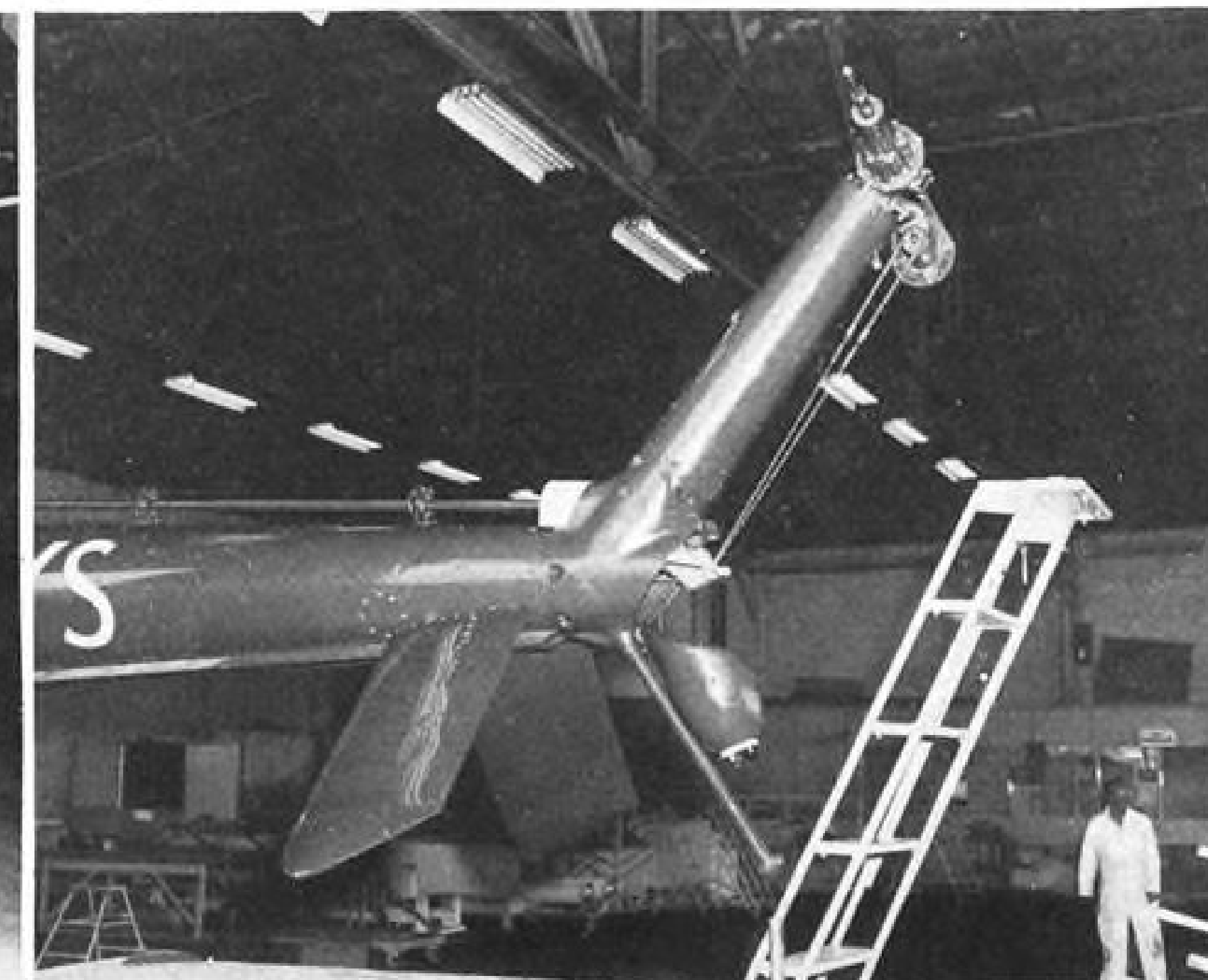
ACCESS DOORS removed, S-55 undergoes 240-hr. check. AUTO TRIM stabilizer fins which caused one maintenance problem.
