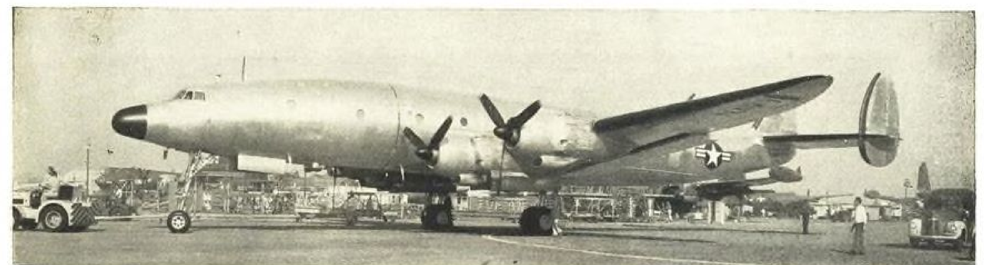
LOCKHEED R7V-1 SUPER CONSTELLATION is towed out for runup of Wright Turbo-Compound engines.
