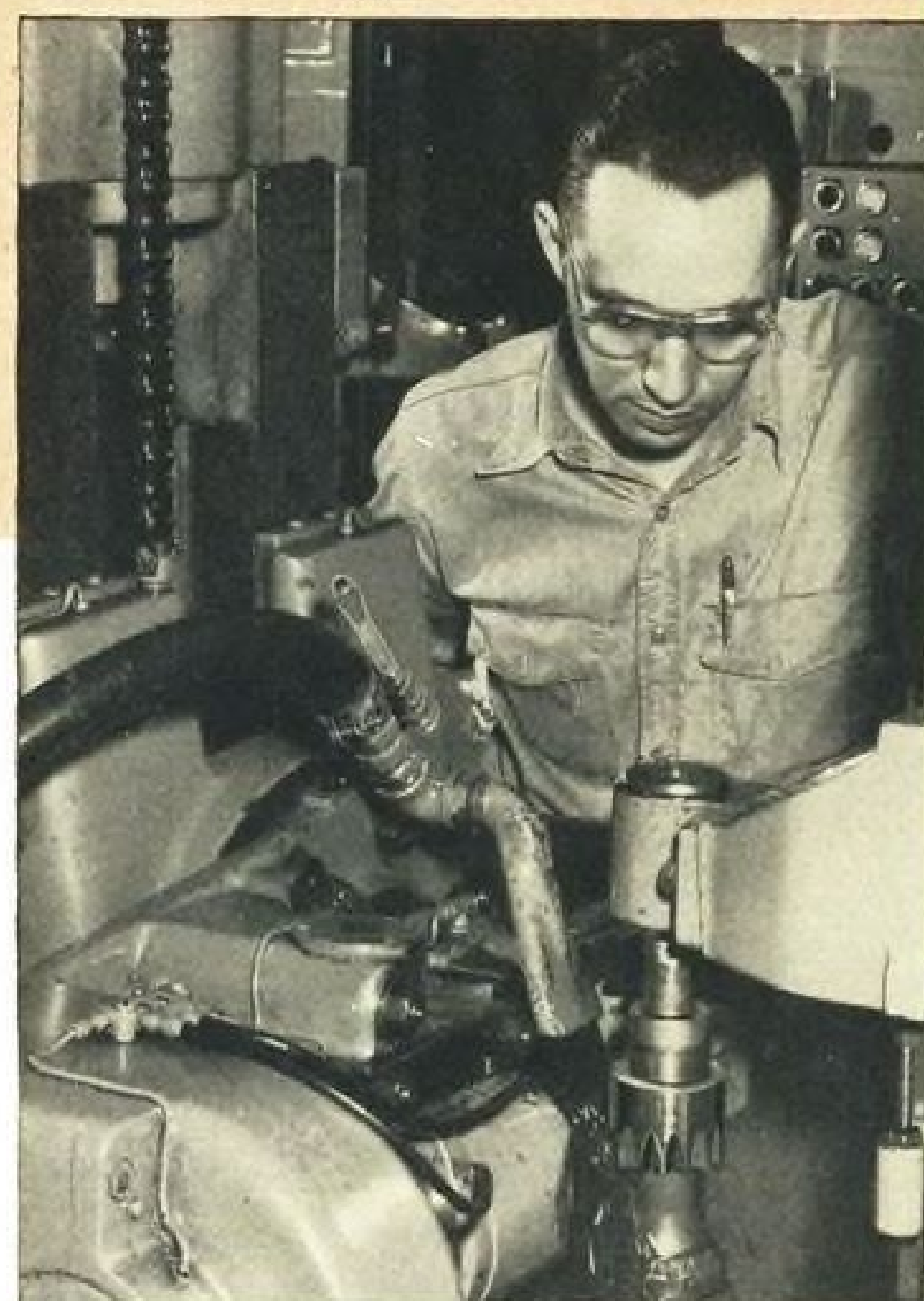
THE GEARS are machined directly from round bar stock. First step is hobbing, shown below.
