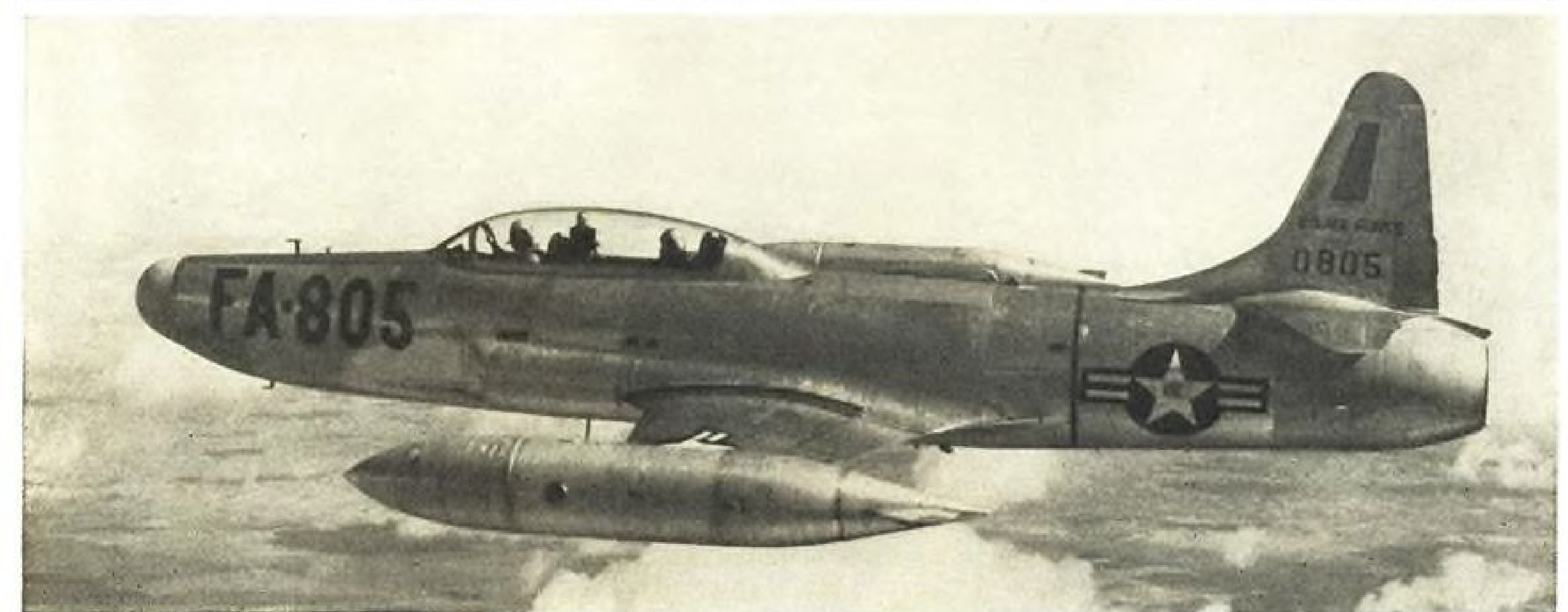
AFTERBURNER on this Lockheed F-94B fighter speedily gives extra jet power when needed for successful interception, typifying how . . .
