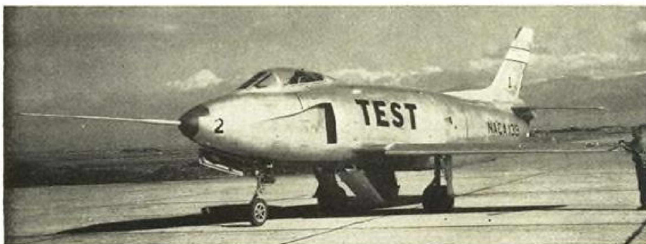
FLUSH INTAKES are fitted on No. 2 plane used by NACA for experiments.
