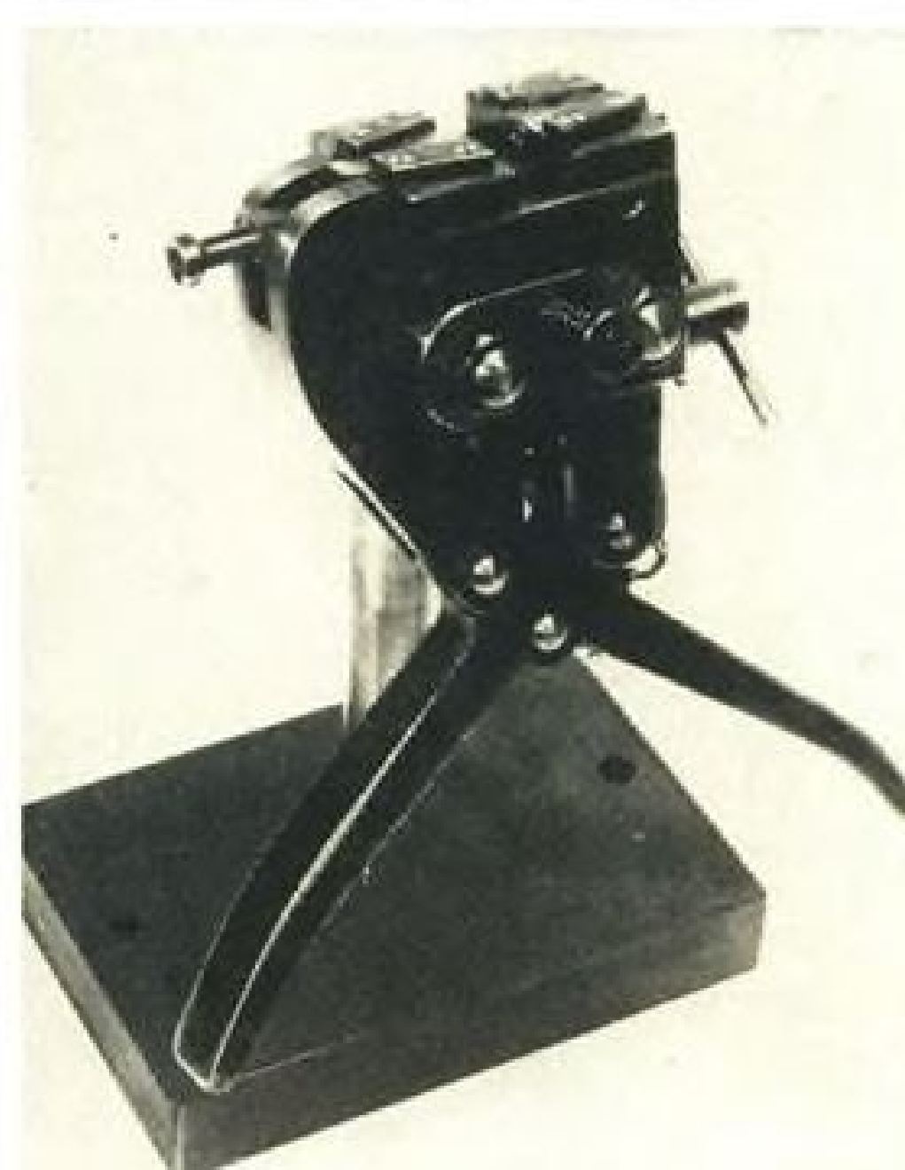
Koldweld hand tool developed by Utica.
