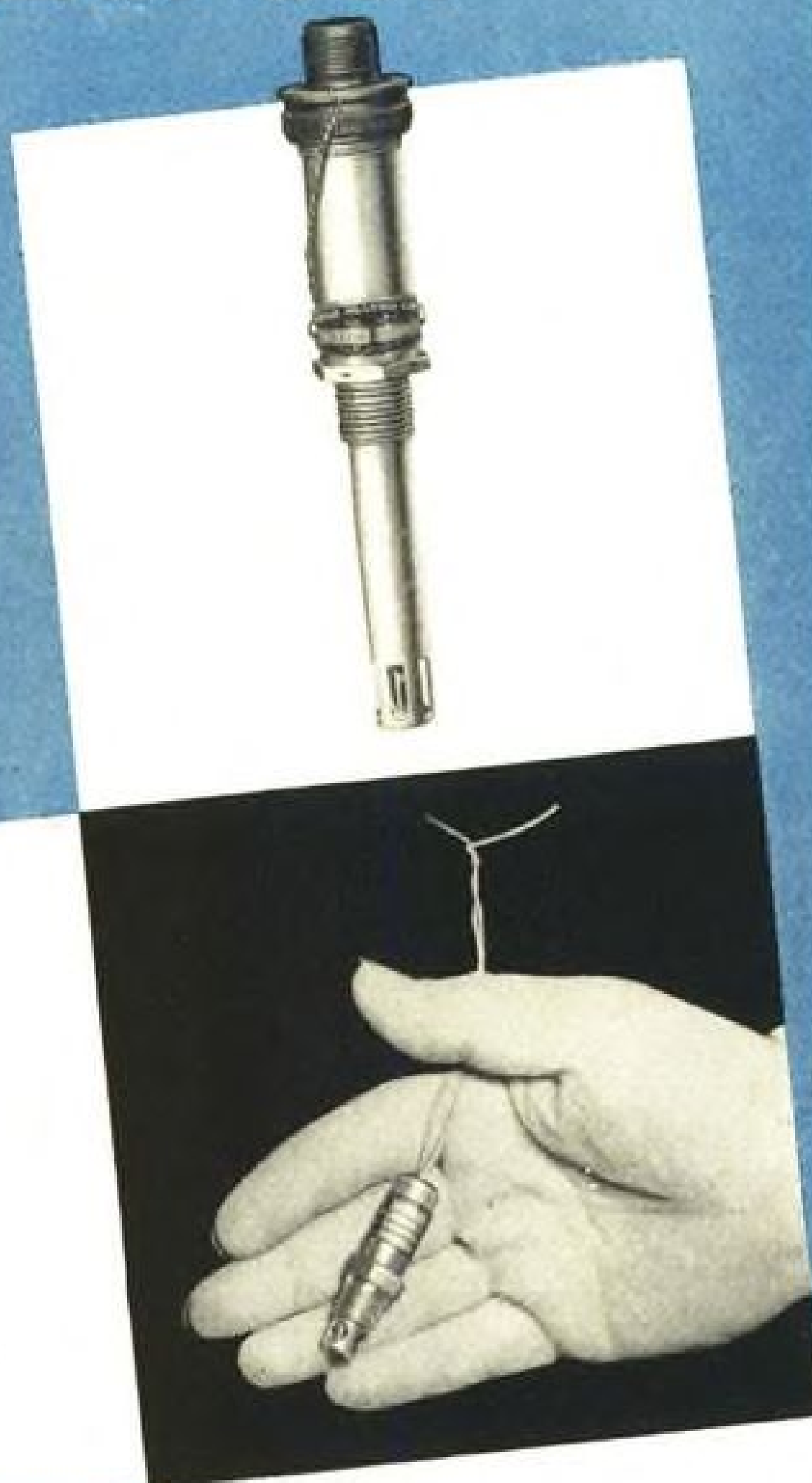
Fig. 8. Here's a full-scale working model of a four-flap variable nozzle.
