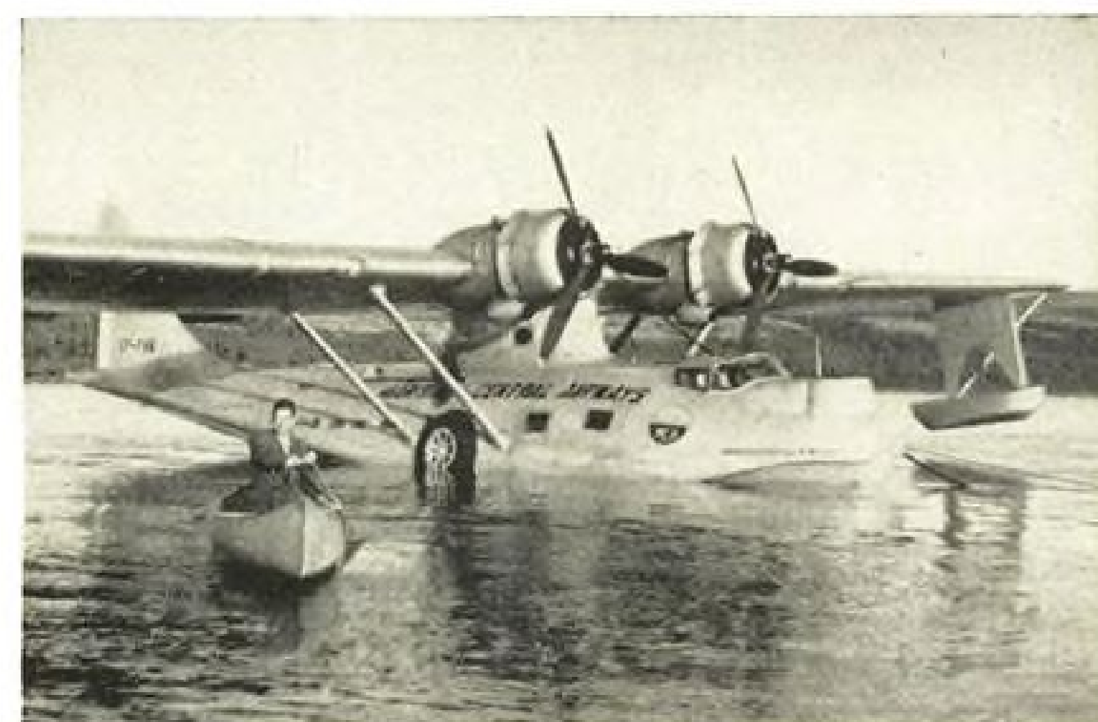
This PBV-5A amphibian Canso is used for long chartered hauls into areas that have no landing fields.
