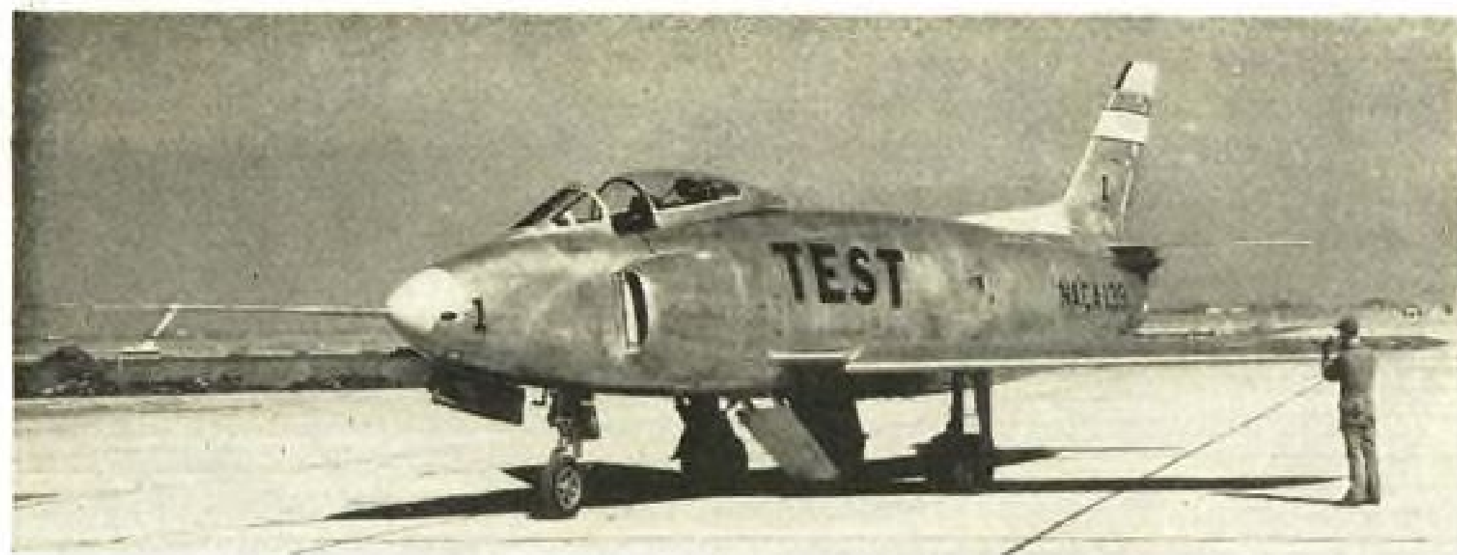
SCOOP INTAKES alongside cockpit mark No. 1 North American YF-93A while . . .
