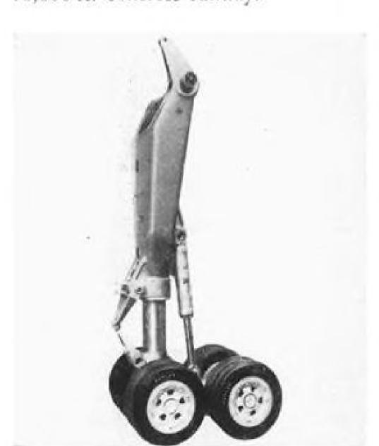
DOWTY landing gear for Avro 698 is light and rugged, features eight small wheels on bogie assembly.
