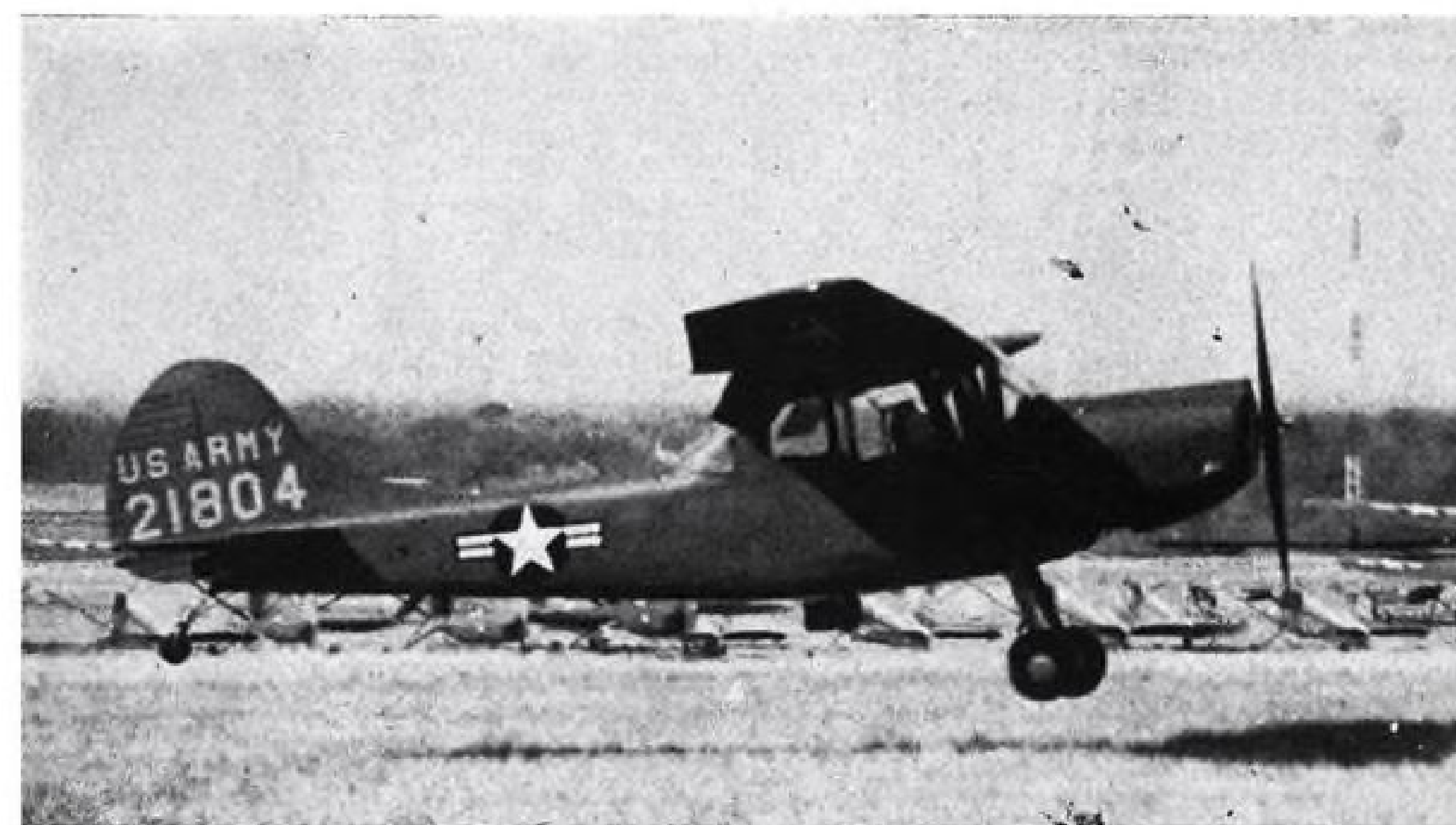
TURBOPROP CESSNA L-19 —Cessna XL-19B, first lightplane to be fitted with Boeing 502-8 turboprop engine, lands after a successful flight trial. The engine (closeup, right) delivers 210 hp. on takeoff and is some 125 lb. lighter than piston engines in other L-19s.
