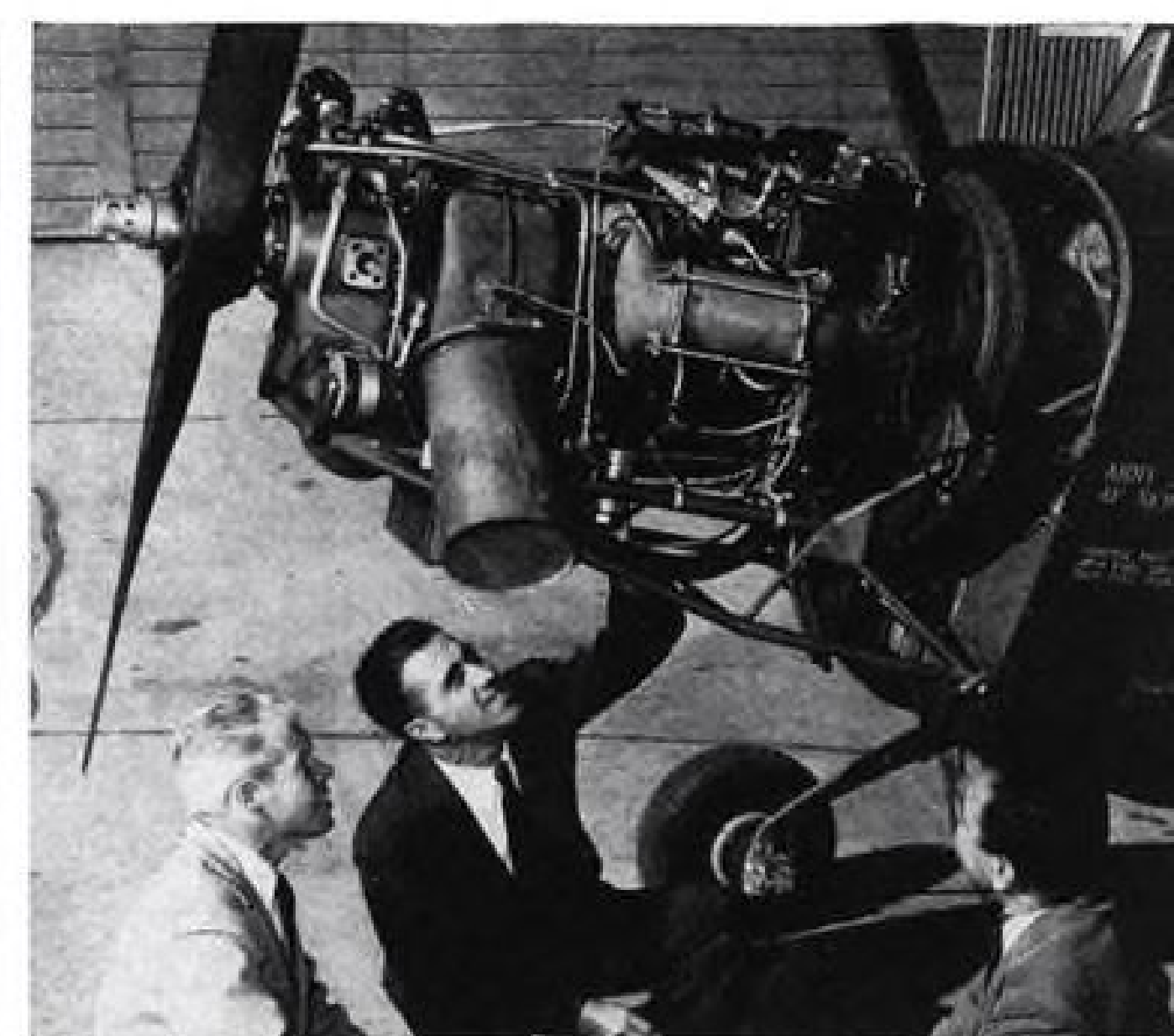
TURBOPROP CESSNA L-19 —Cessna XL-19B, first lightplane to be fitted with Boeing 502-8 turboprop engine, lands after a successful flight trial. The engine (closeup, right) delivers 210 hp. on takeoff and is some 125 lb. lighter than piston engines in other L-19s.
