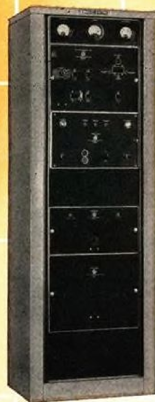
Type 396A Transmitter Station Single channel 250 watts 118-132 mc/s Maximum dependability for unattended service
