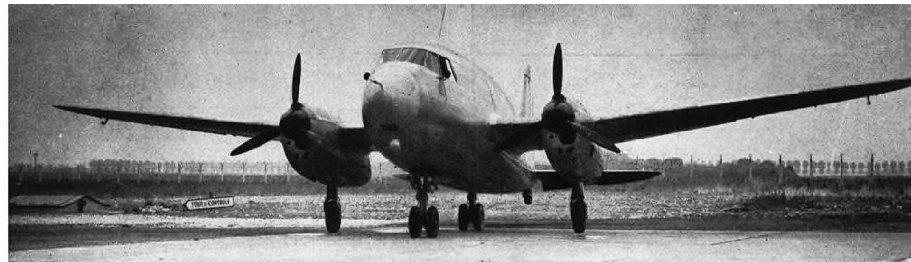
FRENCH TEST BICYCLE GEAR —SNCASO S.O. 30 is testing dual-wheel tandem landing gear developed by the company and made by Hispano-Suiza. A similar-type landing gear is fitted to the new S. O. 4050 Vautour twin-jet fighter (Aviation Week Nov. 3, p. 15).
