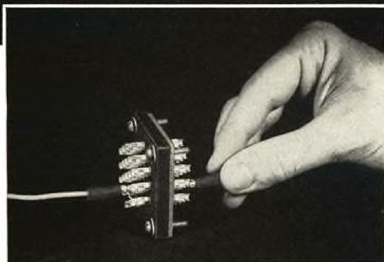
Disconnect one circuit at a time from either side; for wire sizes AN 20 through AN 10
