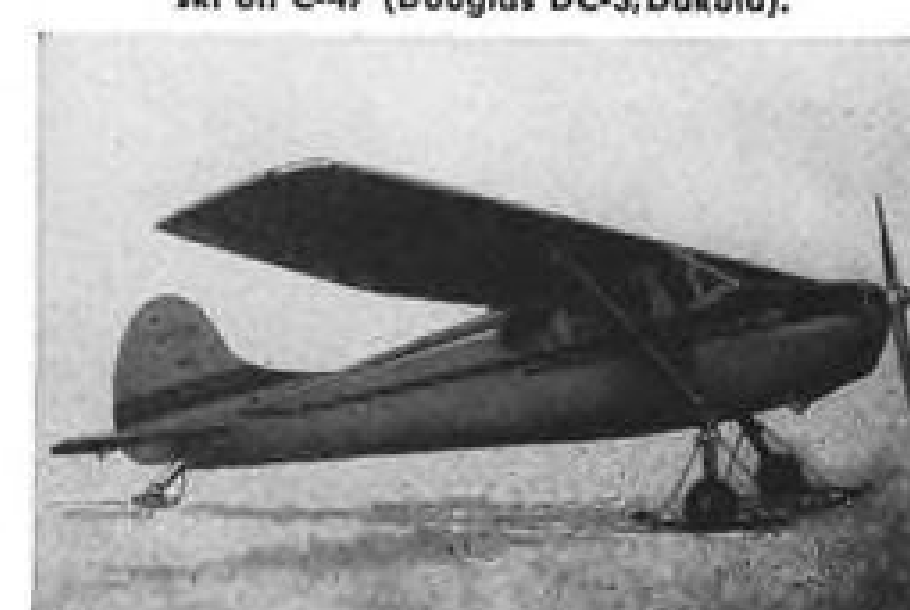
Federal hydraulically actuated, combination wheel ski installation on Cessna 170.
