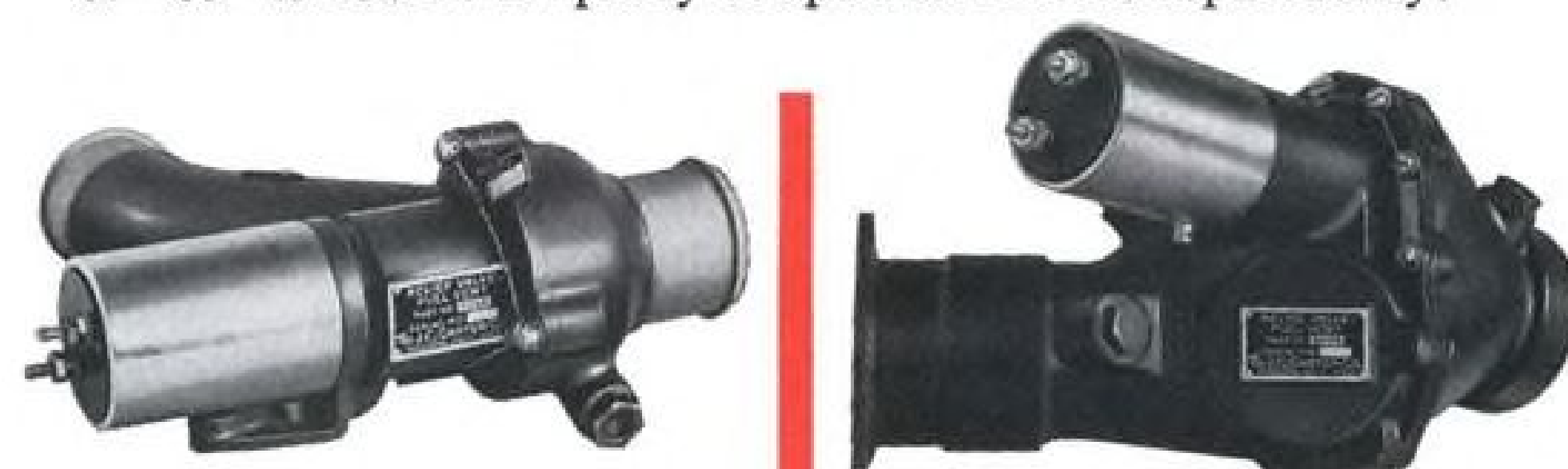
No. 5058 Fuel Vent Relief 2" Line Size 1 PSI \Delta P at 200 CFM Air Flow
