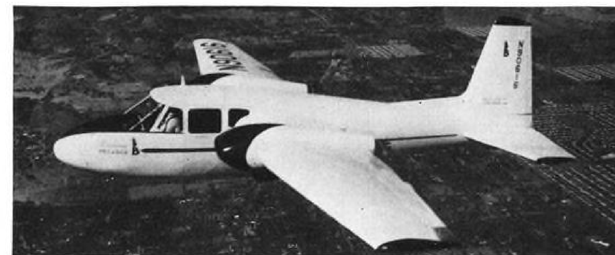
LOCKHEED P2V-6—Versatile new model Neptune (right) does a variety of jobs for Navy, is 12 in. longer than previous P2Vs, has pressure fueling and stainless steel engine nacelles. Powerplants are Wright Turbo-Compounds.
