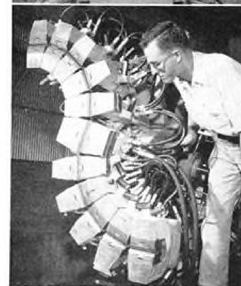
TOP—Start of the stretch-wrap forming operation showing jaws curved to match the vertical profile of a spherical die.
