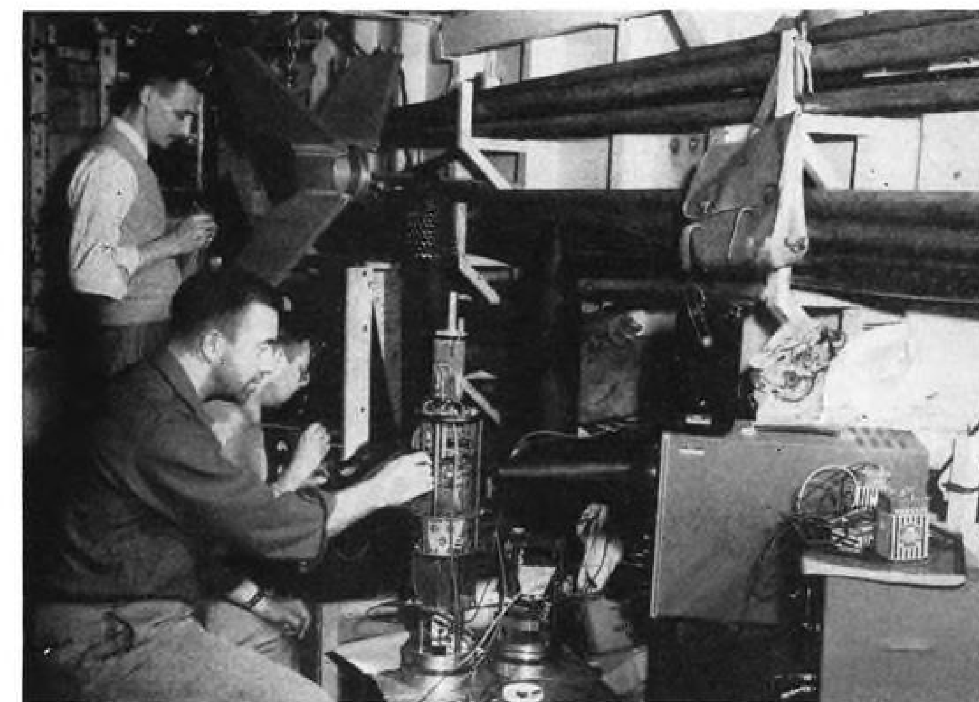
DEACON ROCKET ASSEMBLY is checked by State University of Iowa scientists, before high-altitude launching. Rockets are 10 ft. long, have diameter of 8 in.
