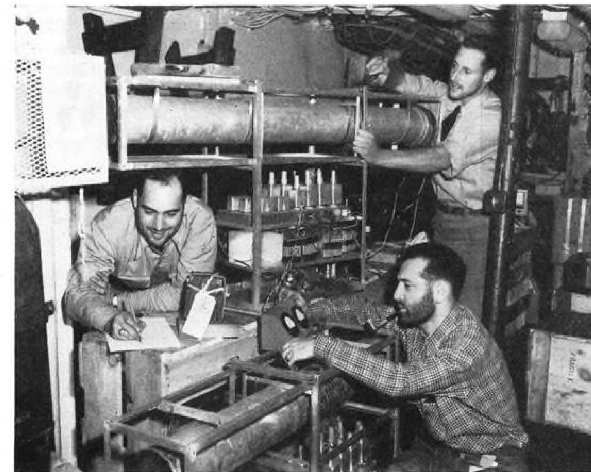
COSMIC RAY APPARATUS gets last-minute check below decks of Icebreaker Eastwind by New York University scientists. This equipment measures neutron intensity.
