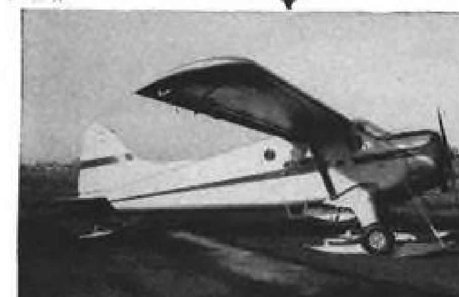
Federal Model AWB-4820 wheel ski on Beaver DHC-2. Ski in down position.
