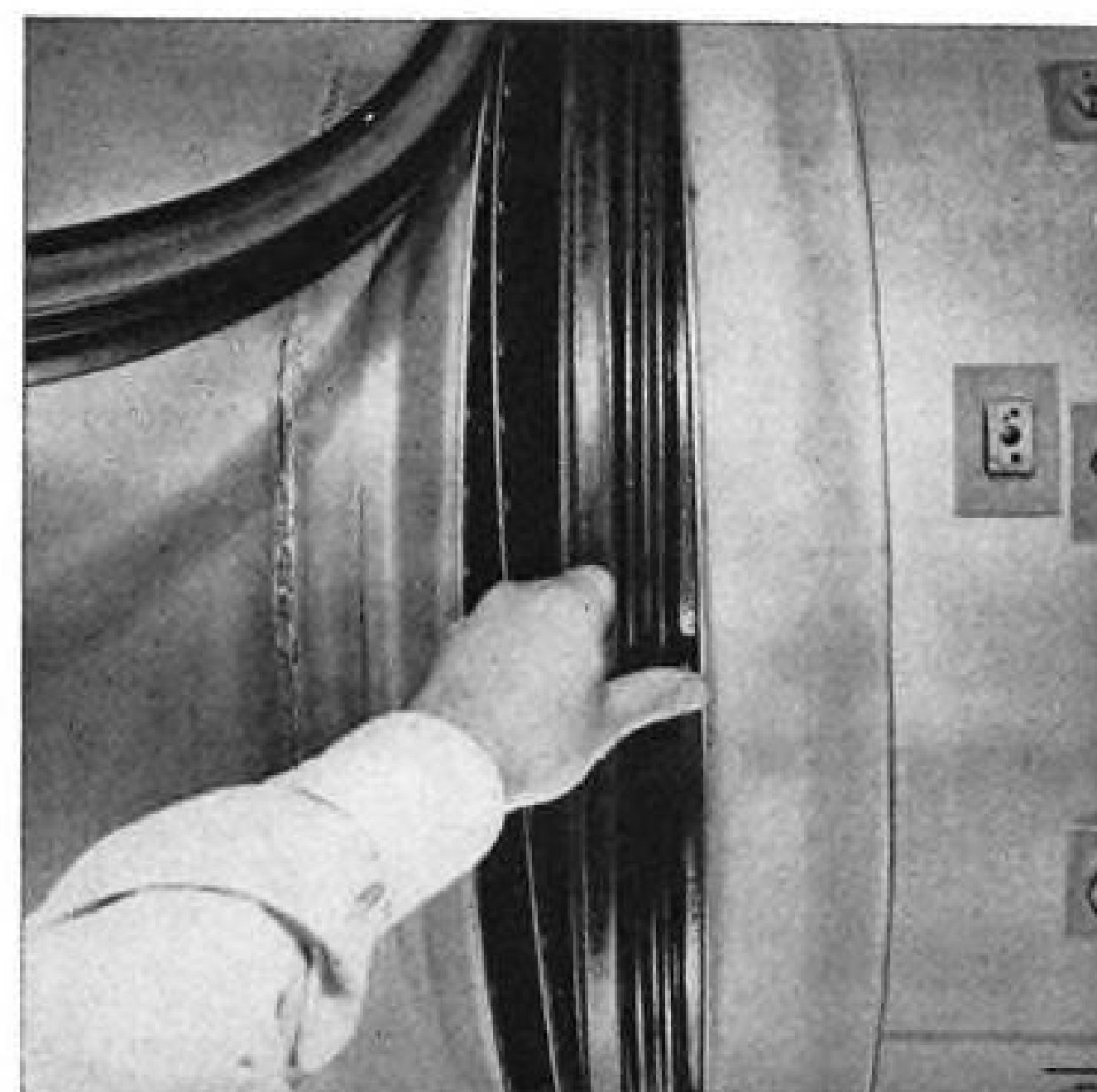
JET AFTERBURNERS boost power, but pose ticklish design problems. Bellows connection between main engine and afterburner must withstand high heat, flex through desired range, prevent hot gases from escaping. This bellows meets all specifications, enables afterburner to supply extra getaway zoom with top efficiency. Designed and manufactured by Solar Aircraft Company, San Diego, Calif., the bellows is made from .010 Inconel "X" sheet which is welded into a circular band—and then corrugated.
