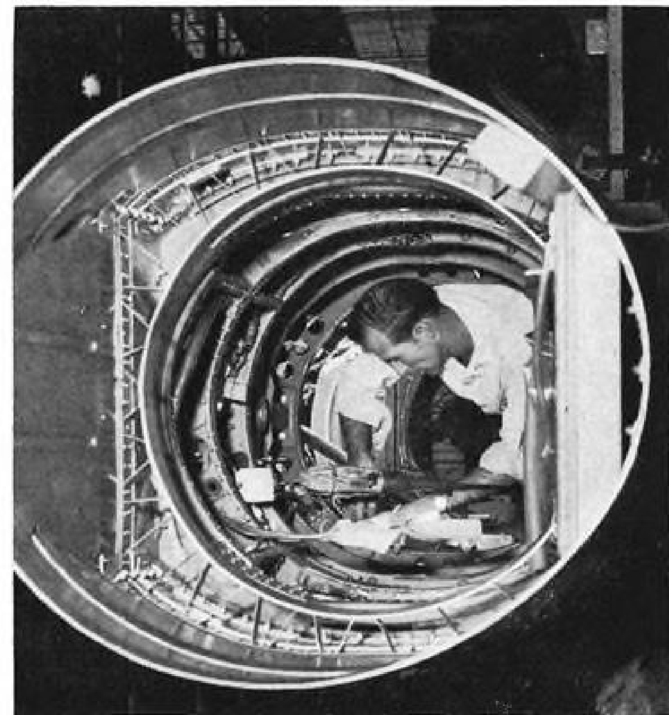
AFT FUSELAGE looking forward, tailpipe and shroud not yet installed.
