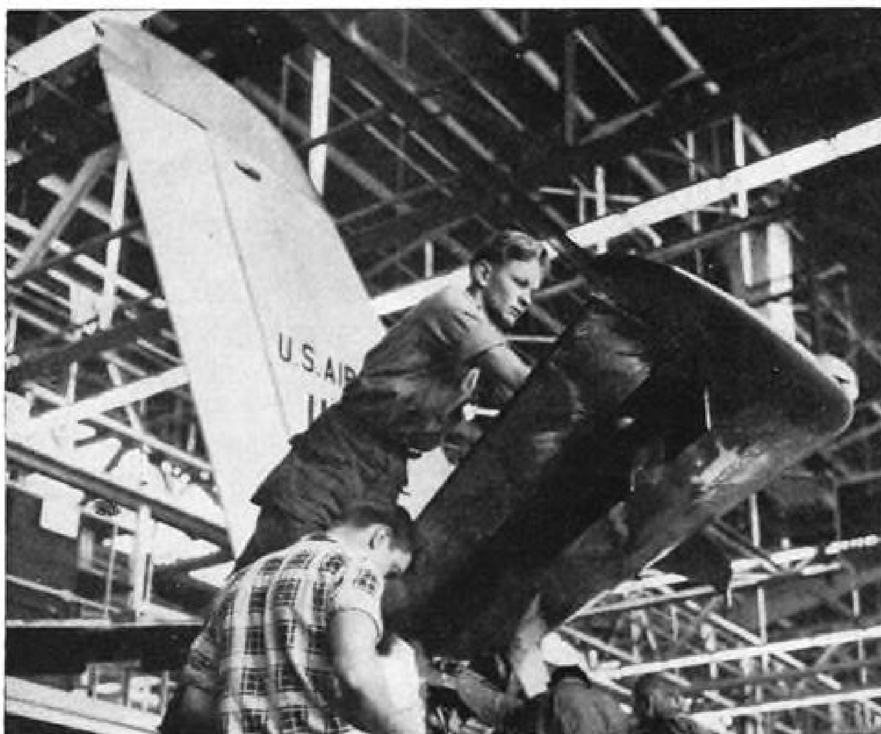
STABILIZER of current F-84F. Later Fs will have no elevator; adjustable stabilizer will give surface control, trim.
