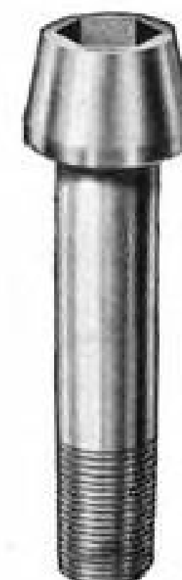
NAS INTERNAL WRENCHING AIRCRAFT BOLTS Latest NAS speci- fications. Threads are fully formed by rolling after heat treatment.
