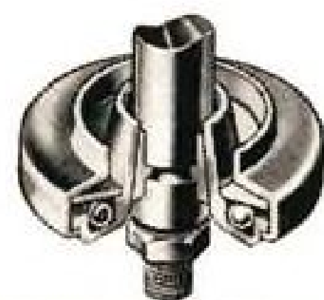
Thompson-developed "Rotocaps" and "Rotovalves" help increase valve life hundreds of hours.
