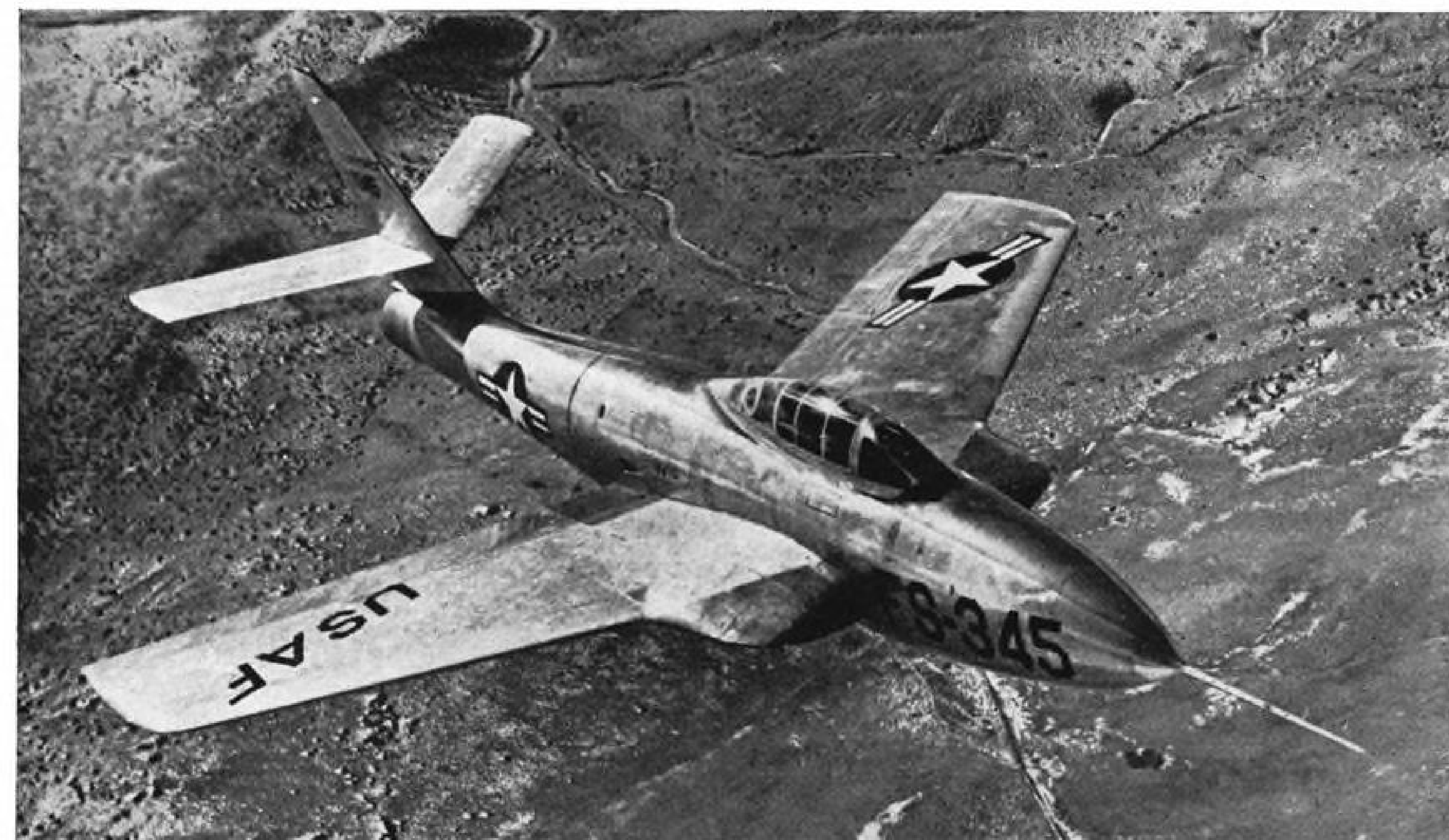
F-84F THUNDERSTREAK prototype incorporating solid nose and wing root intakes shows what final production version will look like.
