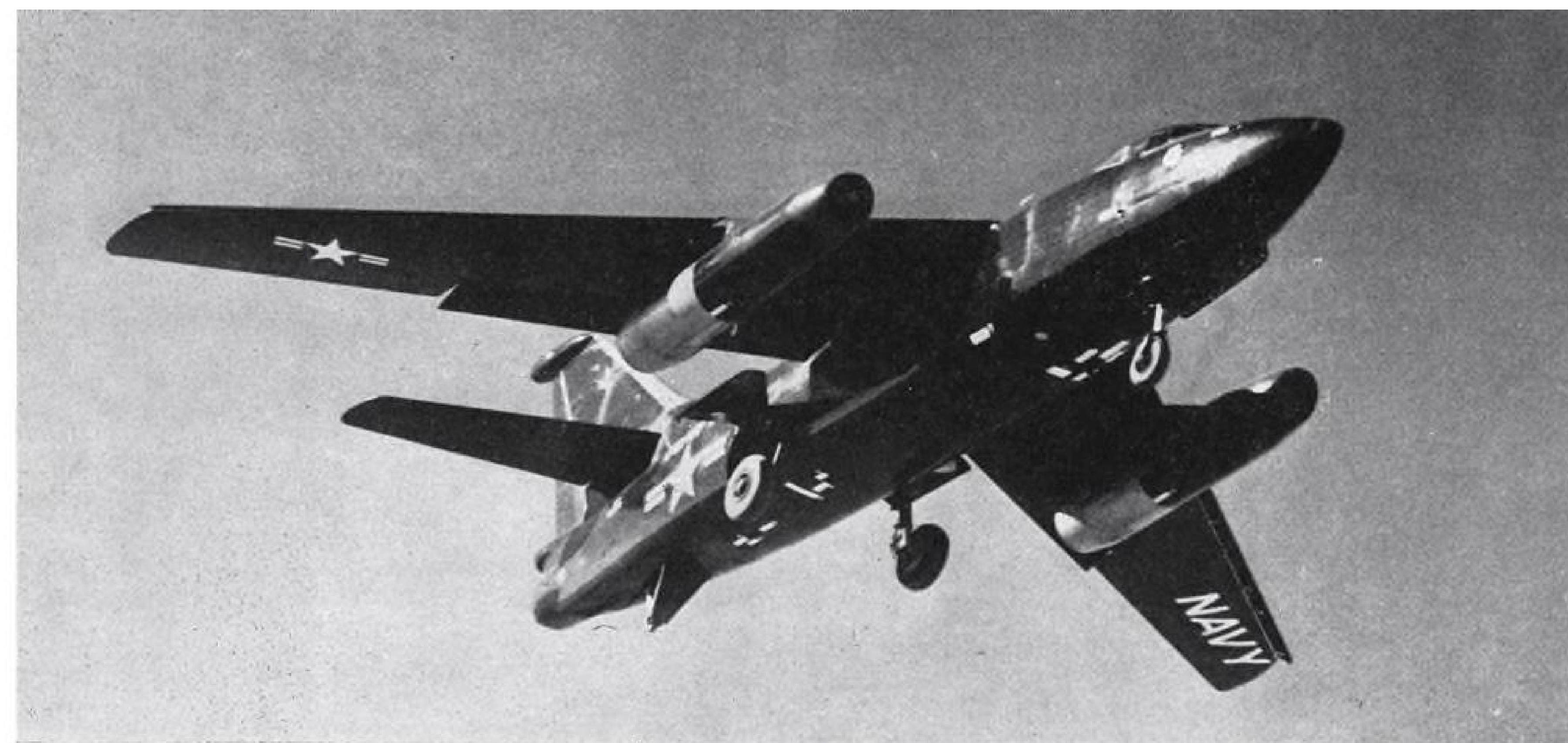
DOUGLAS XA3D-1 FIRST FLIGHT —Here is the first actual photo of Navy's new heavy attack plane taken during its first flight at Edwards AFB, Calif. Prototype is powered by two Westinghouse J40s slung under the wings in pods, but production models will have P&WA J57s. Gross weight is about 70,000 lb. and top speed is in the "600-700-mph. class." Bulge atop tail houses anti-spin chute.
