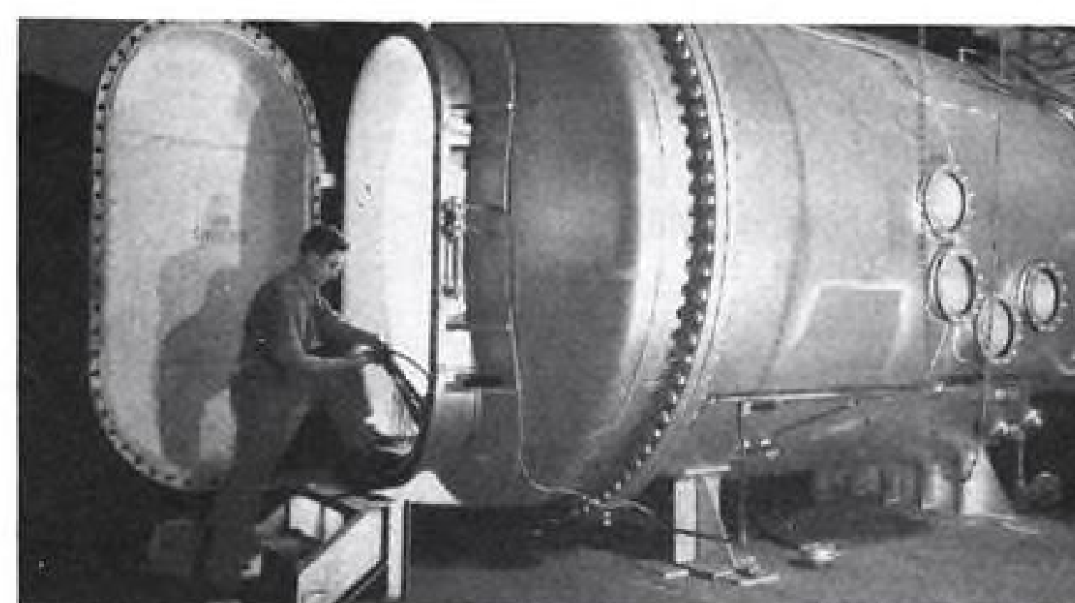
TESTING. . . Accessory turbines are tested under simulated operating conditions. Shown above is turbopump altitude chamber.
