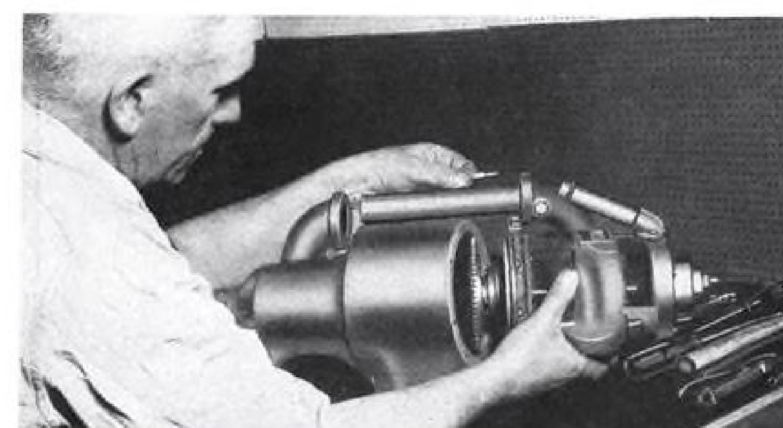
REHEAT FUEL PUMP bleeds air from jet engine to supply extra flow of fuel for afterburner operation.
