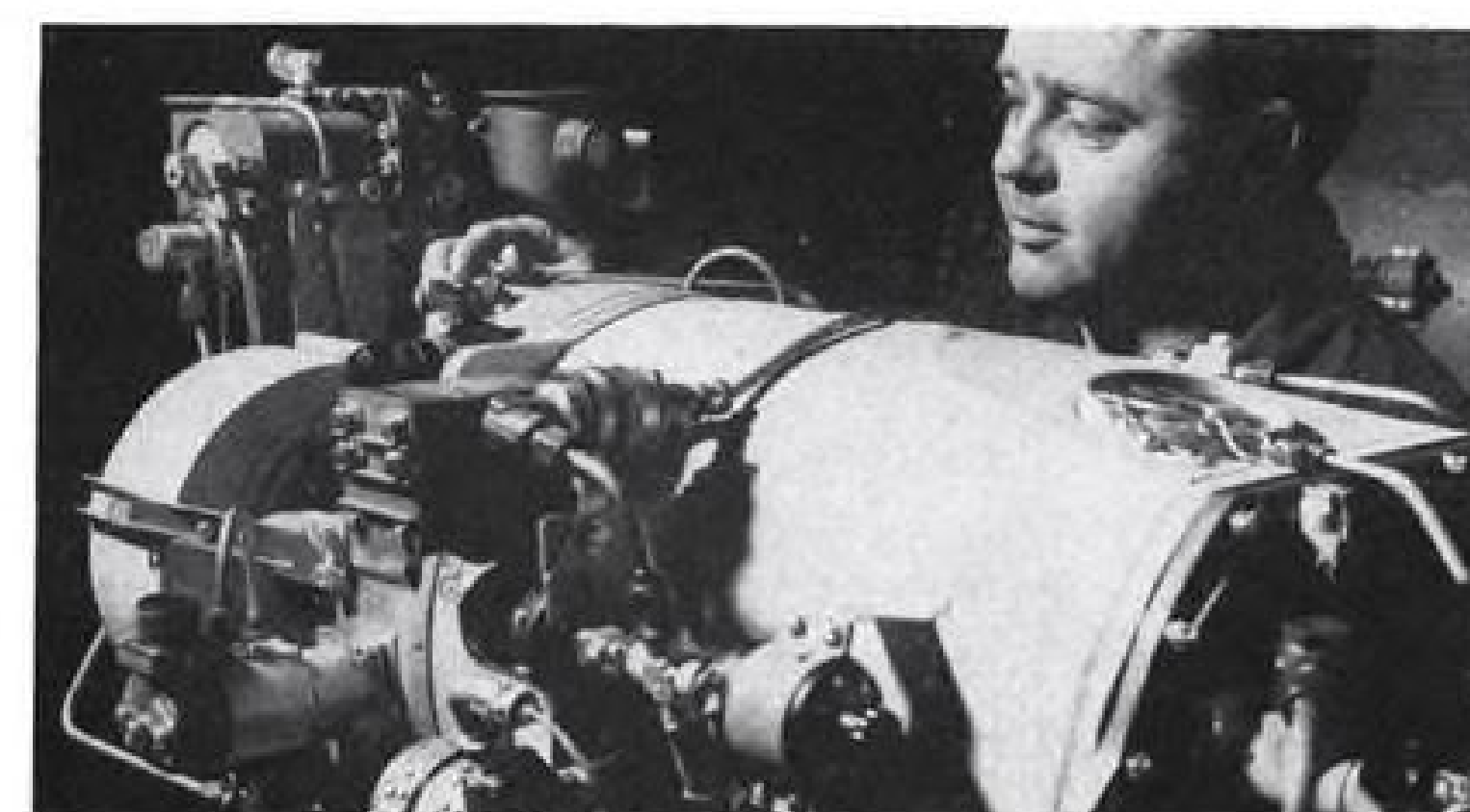
TURBO HYDRAULIC PUMPS bleed air from jet engine compressor to supply hydraulic power for entire airplane.
