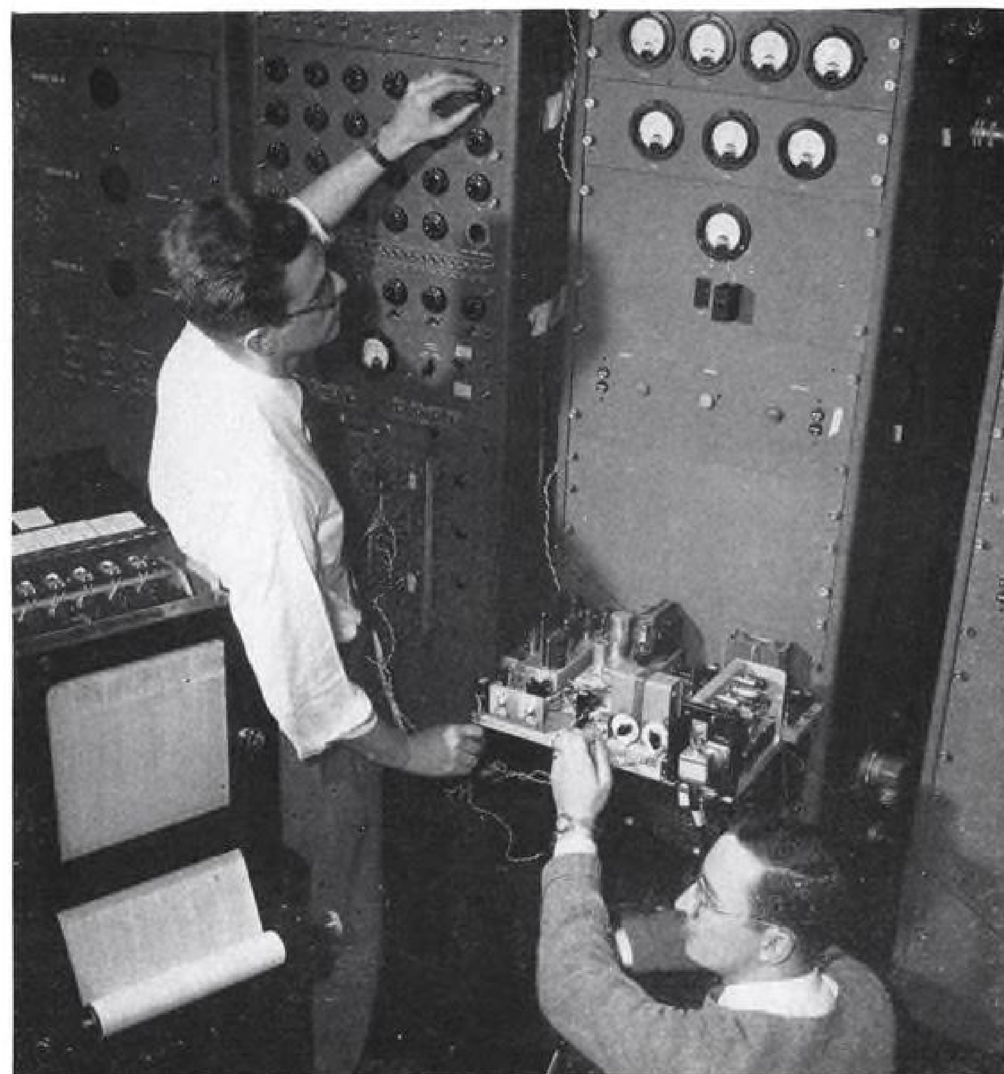
WORKOUT on analog computer simulates autopilot fault occurring in gusty air.
