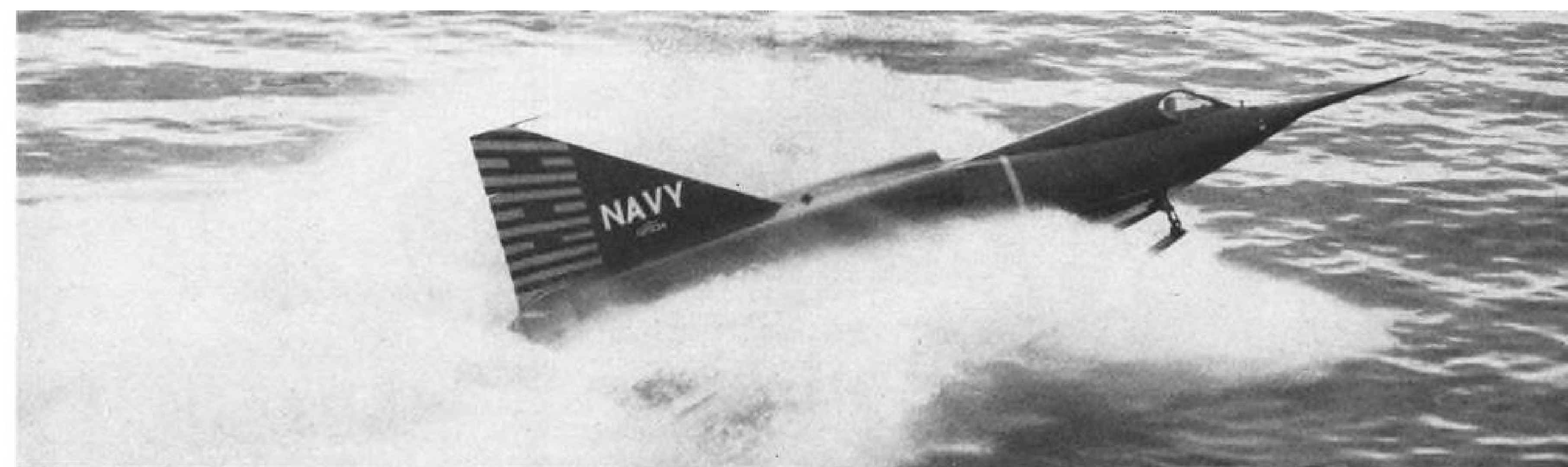
SEA TRIALS FOR CONVAIR SEA DART —Radical new Convair XF2Y-1 Sea Dart delta-wing flying boat fighter, world's first, is seen in photos above and below undergoing taxi trials in San Diego Bay. Barely visible under forward fuselage is craft's novel hydro-ski landing gear. Note how spray just misses engine intakes behind cockpit canopy, while XF2Y-1 planes on its hydro-skis at high speed.
