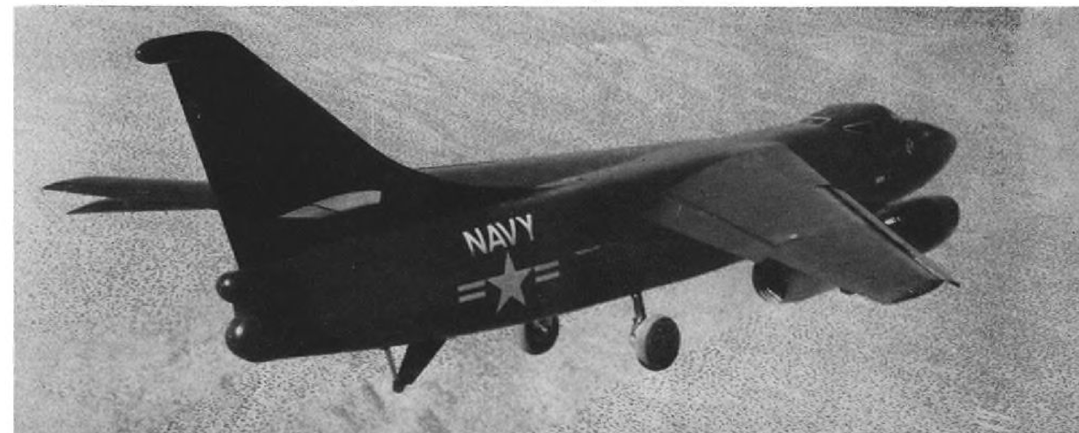
REAR VIEW—Douglas bomber has new-type cockpit canopy for resisting heat and stresses of high-speed flight, wing slats to improve flight characteristics at low speeds. Navy has ordered two XA3D-1 prototypes and 12 production versions to cost some $3,350,000 each.
