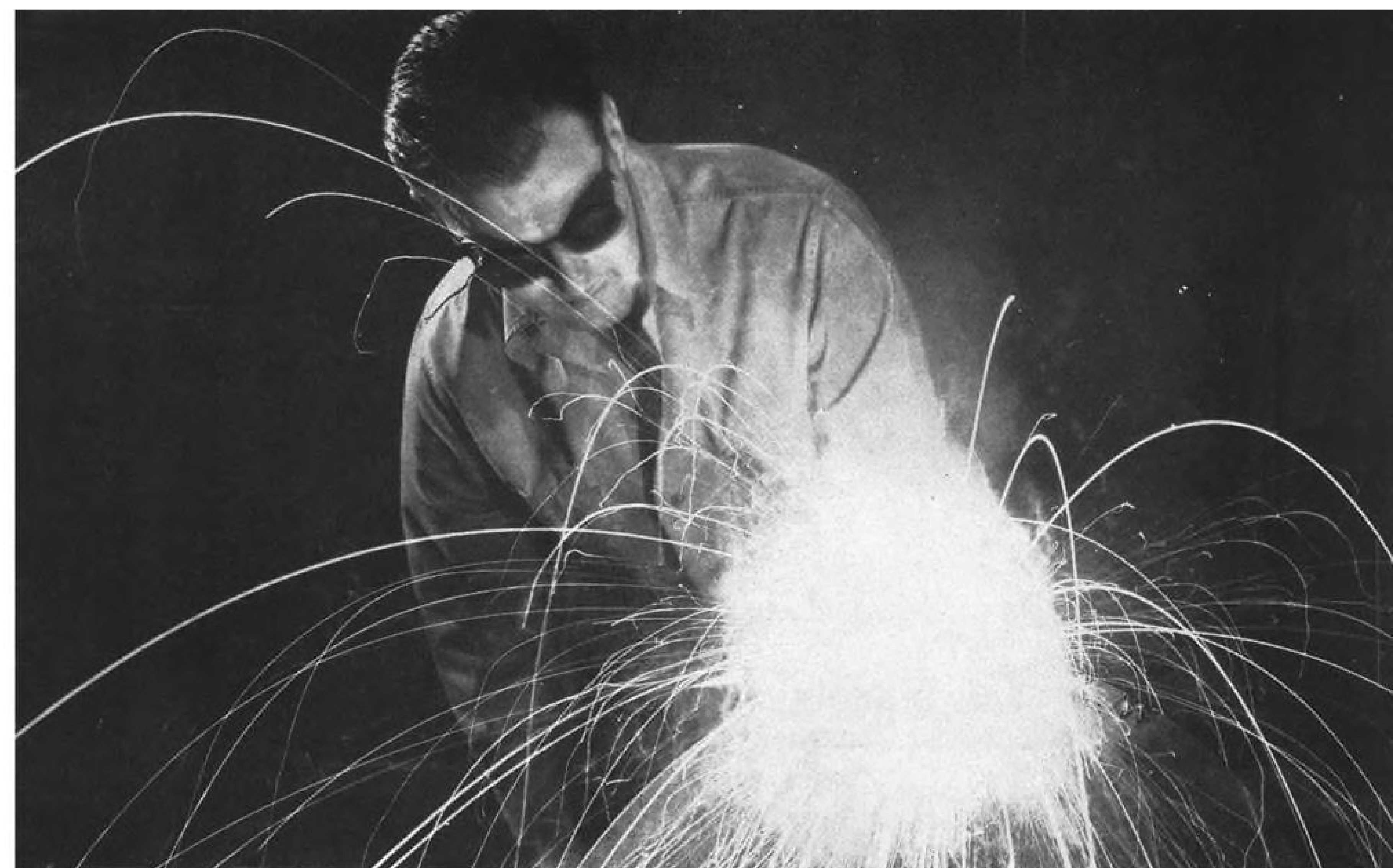
HERE'S DRAMATIC PROOF of the damage an arcing fault can cause in an aircraft. To get this picture, G-E engineers arranged a mockup of an aircraft electrical system, then touched the generator power cable against a test airframe. Note the white-hot glare at point-of-contact!
