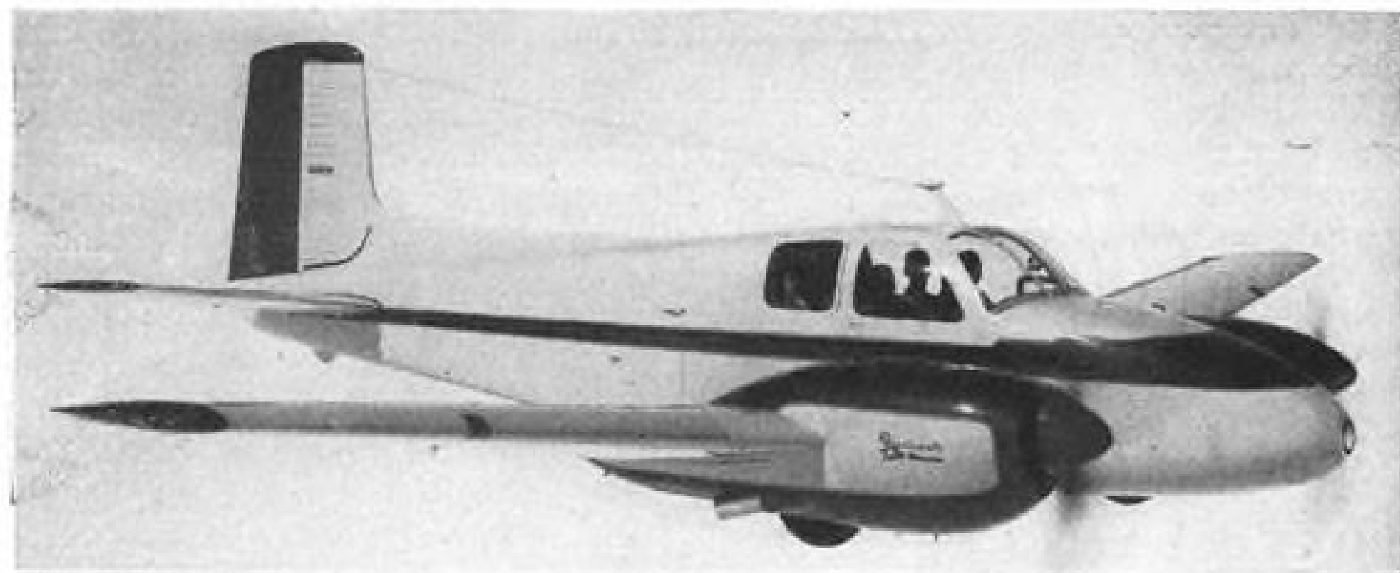
LONG NOSE of Twin-Bonanza is designed to provide safety cushion in event of crash.
