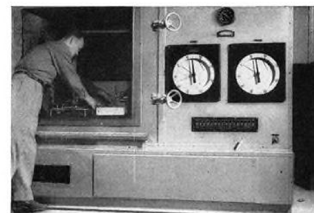
This Atmospheric Chamber simulates conditions from -65^{\circ} to +160^{\circ} centigrade, altitudes up to 80,000 feet. It also varies humidity 20 to 95 per cent and automatically controls these variable conditions to any pre-set values.
