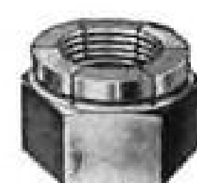
FLEXLOC SELF- LOCKING NUTS, REGULAR TYPE Both stop and lock nuts. One piece construction, re- siliant segments lock posi- tively with uniform torque. Aircraft approval, sizes # 4 to 1 1/4" inclusive. Reg- ular steel FLEXLOC approved for temperatures to 550°F.
