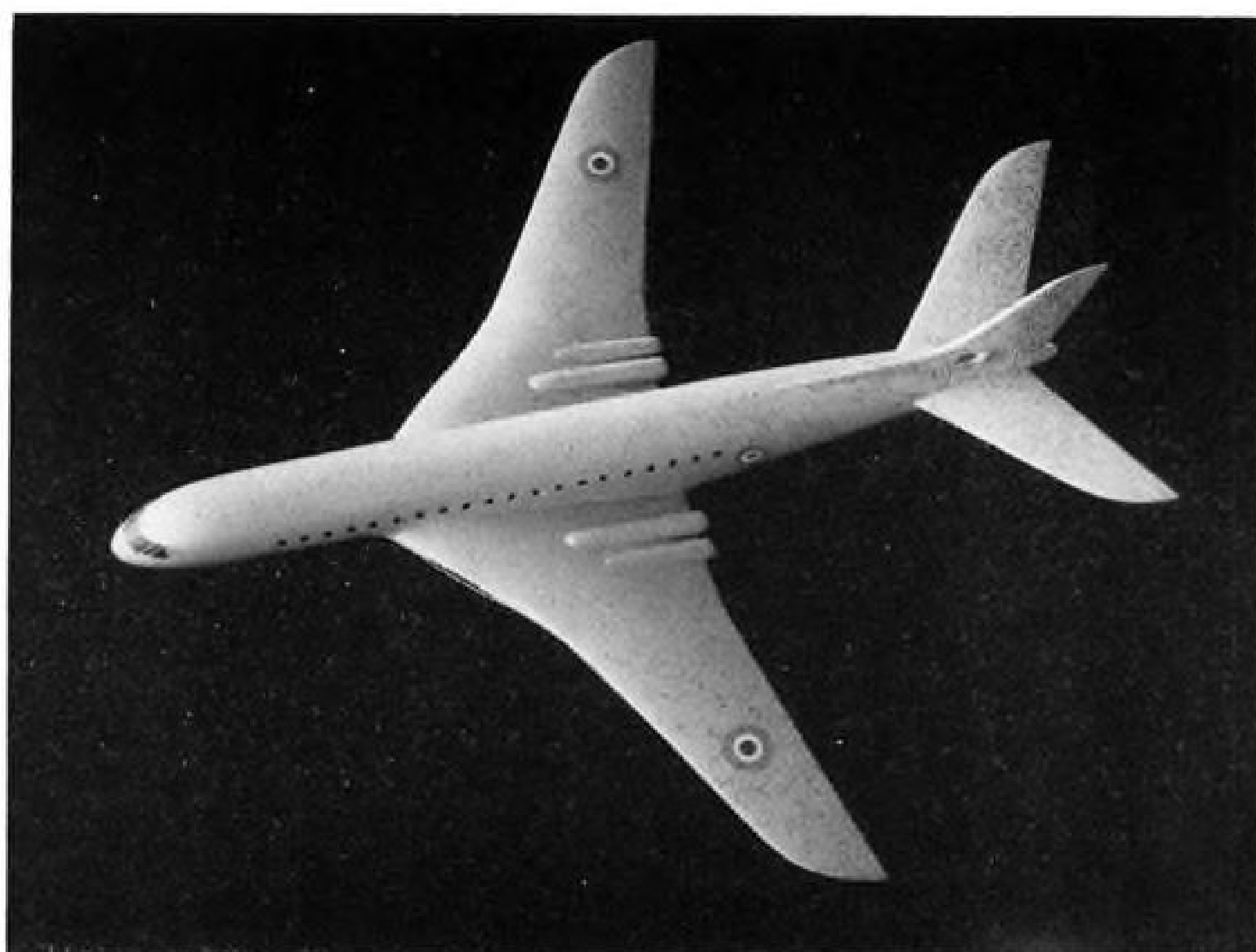
VICKERS JET TRANSPORT (in model), may carry 150 passengers, have 2,000-mi. range.
