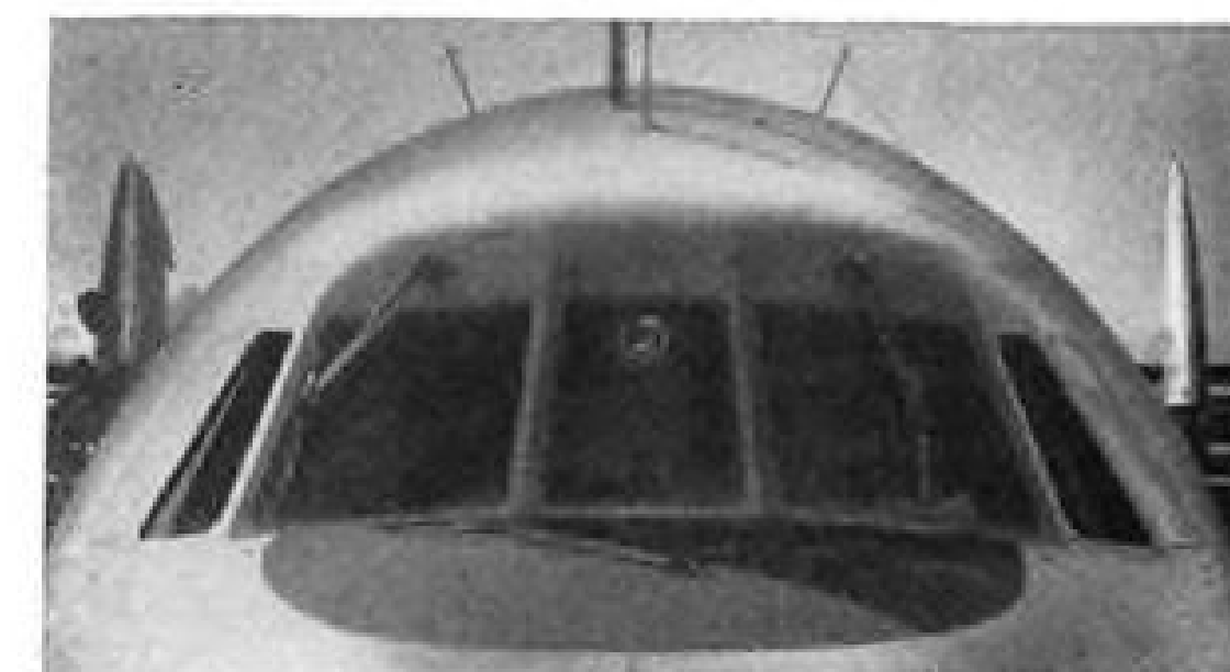
These three forward glass areas are electrically-heated NESA Glass to assure the best vision under every flying condition.
