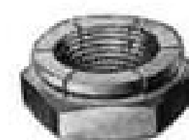
FLEXLOC SELF- LOCKING NUTS, THIN TYPE Less than regular height, yet conform to accepted standards. Every thread, including the locking threads, carries its share of load. Have all regular FLEXLOC features, but save weight and height. Aircraft approval, # 6 to 1 1/4".
