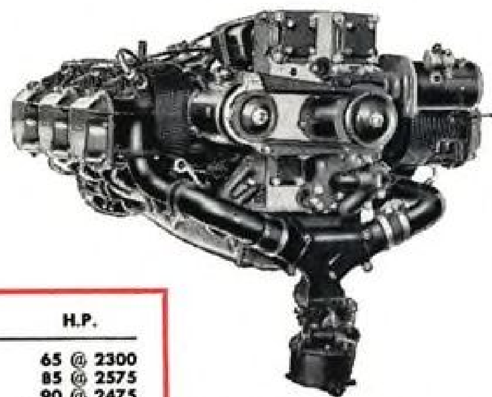
REAR VIEW, showing belt-driven generator; also starter mounted at angle of 90 degrees to engine's main axis. Engine is exceedingly compact.
