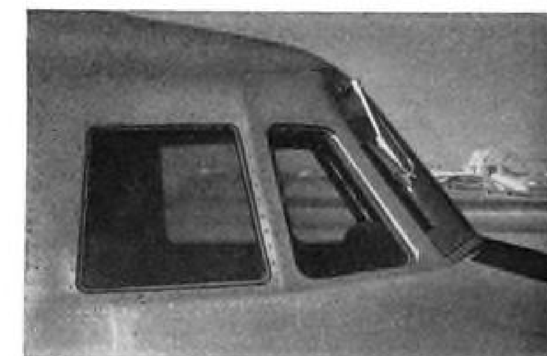
A close-up view of the side windows of the Super Constellation's cockpit. Note the unobstructed vision insured by an advanced joining method that permits the use of extremely narrow posts.
