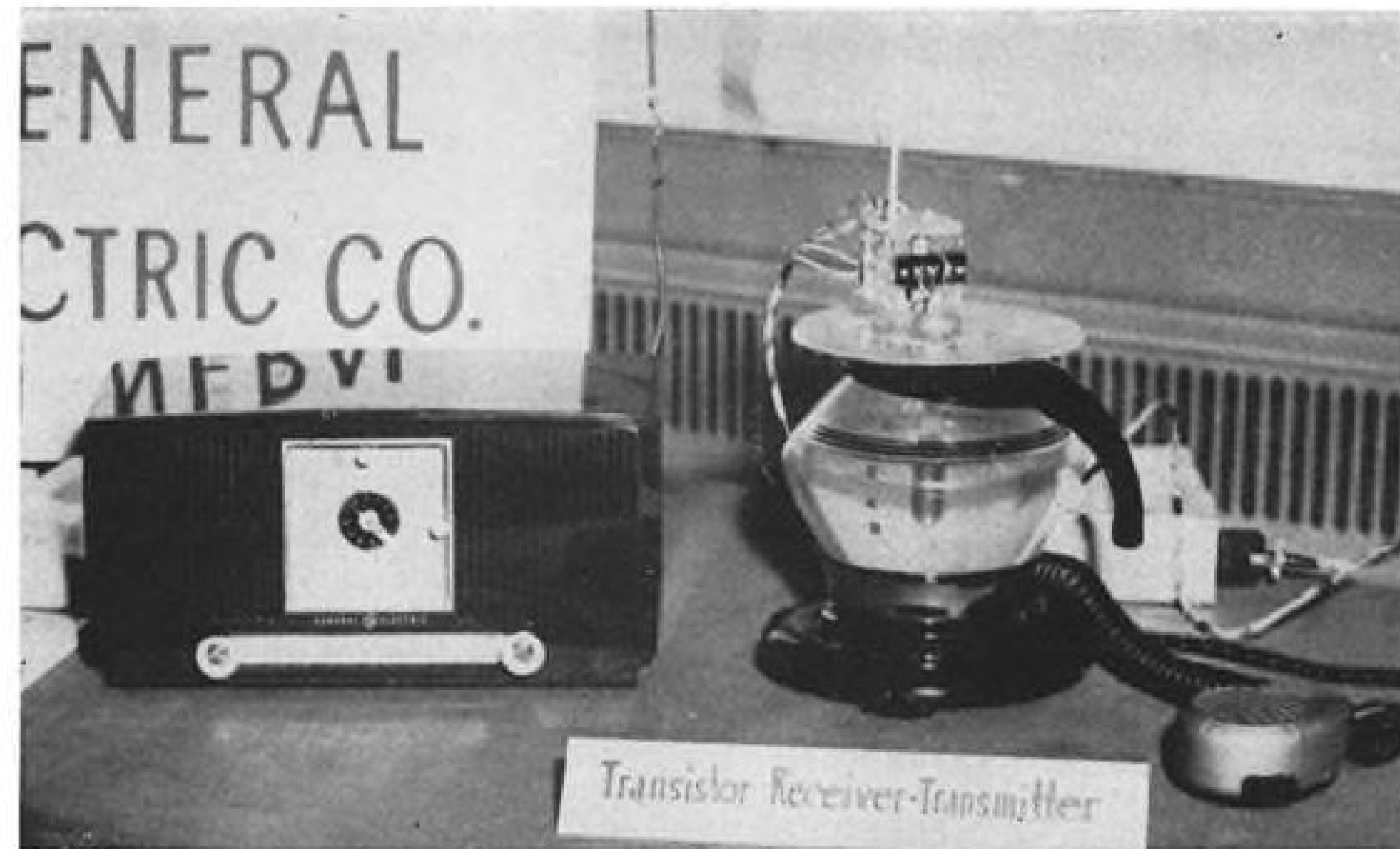
GE HIGH-TEMPERATURE junction transistor (in boiling water, right) is part of small transmitter "picked up" by transistorized receiver (left).
