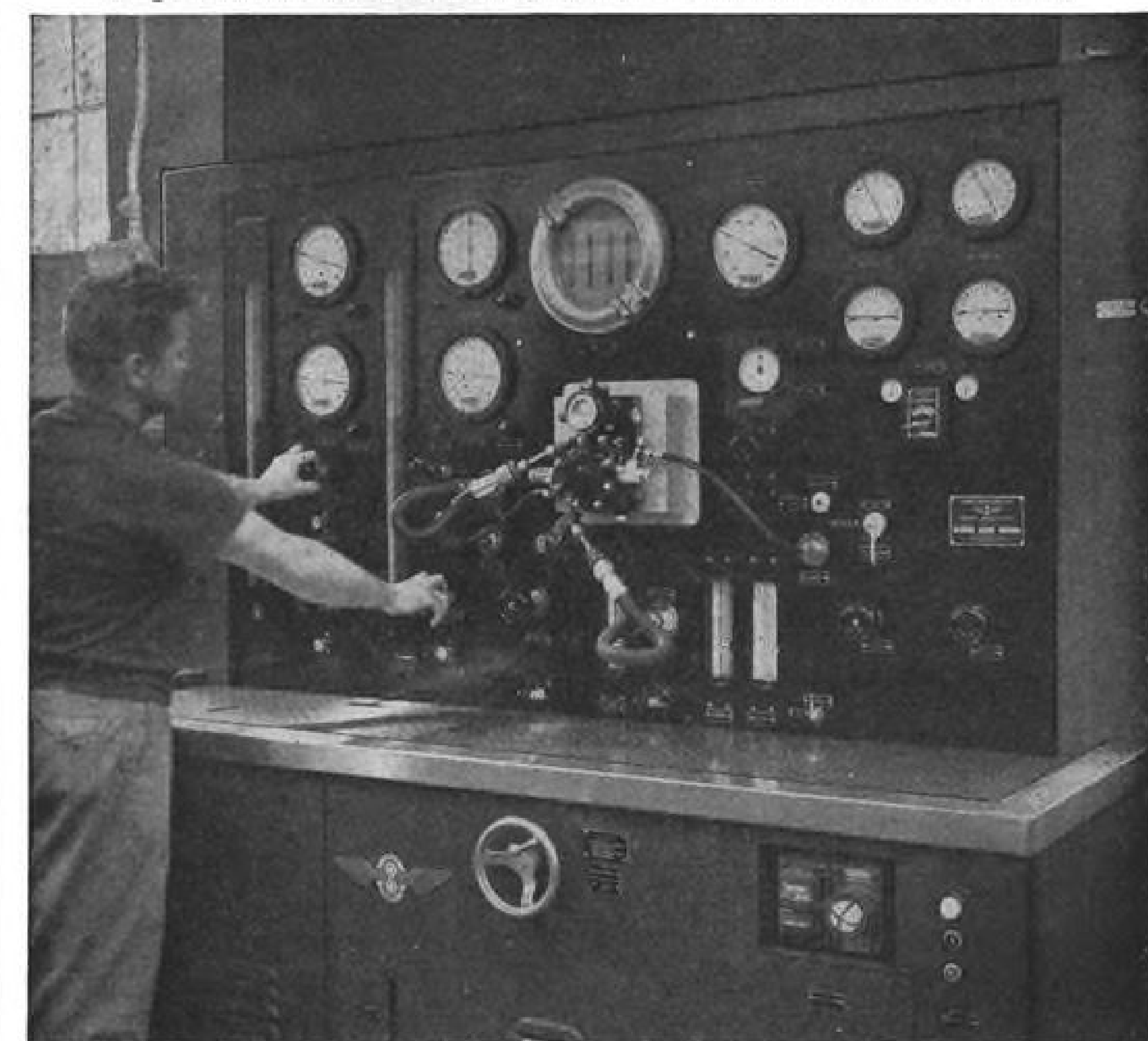
GREER LUBE PUMP TEST STAND supplies oil under rigid control conditions of temperature, flows to 10 gpm, pressures to 28 psi, and pump shaft speeds to 5000 rpm. It accurately checks the main oil pump assembly of the J-65 turbojet engine for the Wright Aeronautical Division, Curtiss-Wright Corp.
