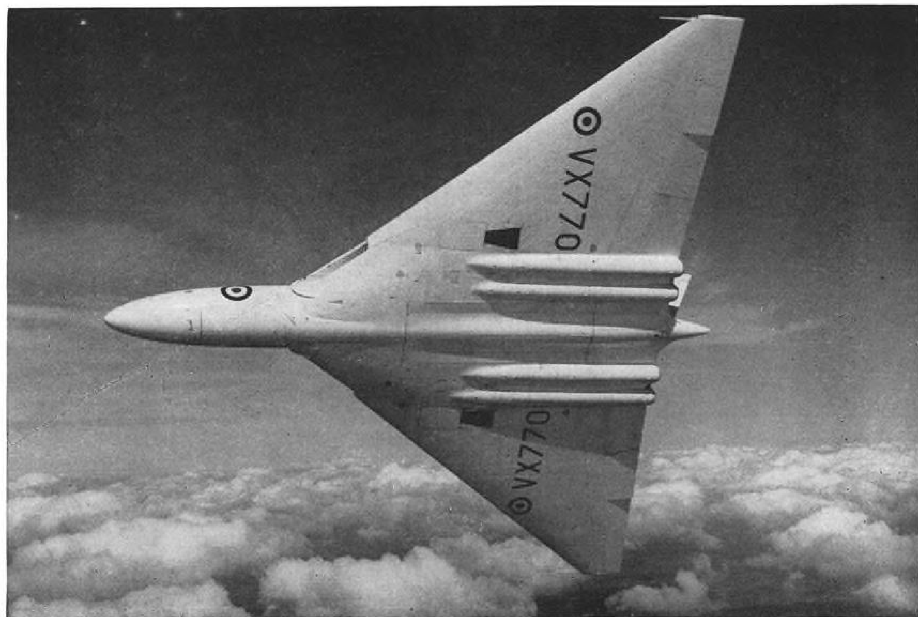
TIPPED TRIANGLE of the Vulcan's wing reveals important details of structural layout, shows layout of surface controls.
