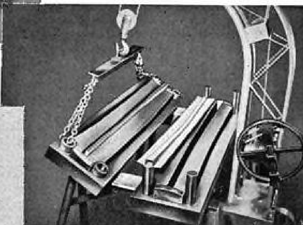
TWIX made Die to make a Hat-Sectioned Longerons in one operation. Longerons Dimensions: 72" long X 7" wide having Double Contour.
