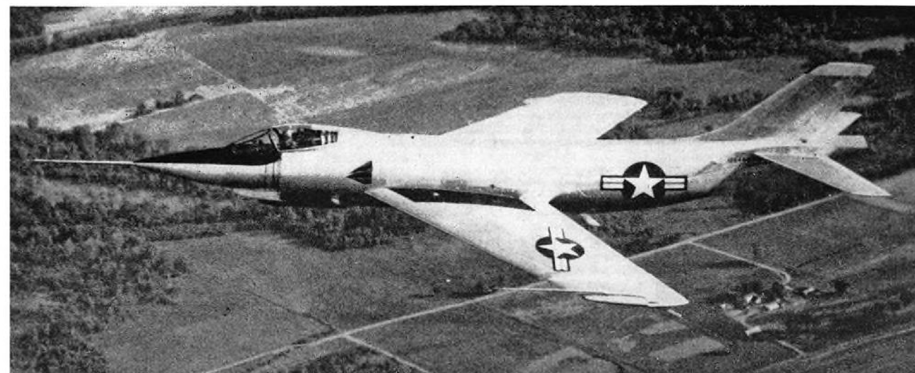
DEMON ALOFT —Flight view of XF3H-1 shows craft's sharply swept wings, also flat section behind the tail which maintains airflow continuity. Navy has ordered a quantity of Demons from McDonnell Aircraft Corp., St. Louis, Mo., and the plane will also be built by Temco, Dallas, Tex. The prototype is to undergo carrier suitability trials at the Navy Test Center at Patuxent, Md. and production deliveries are to begin before the end of this year.
