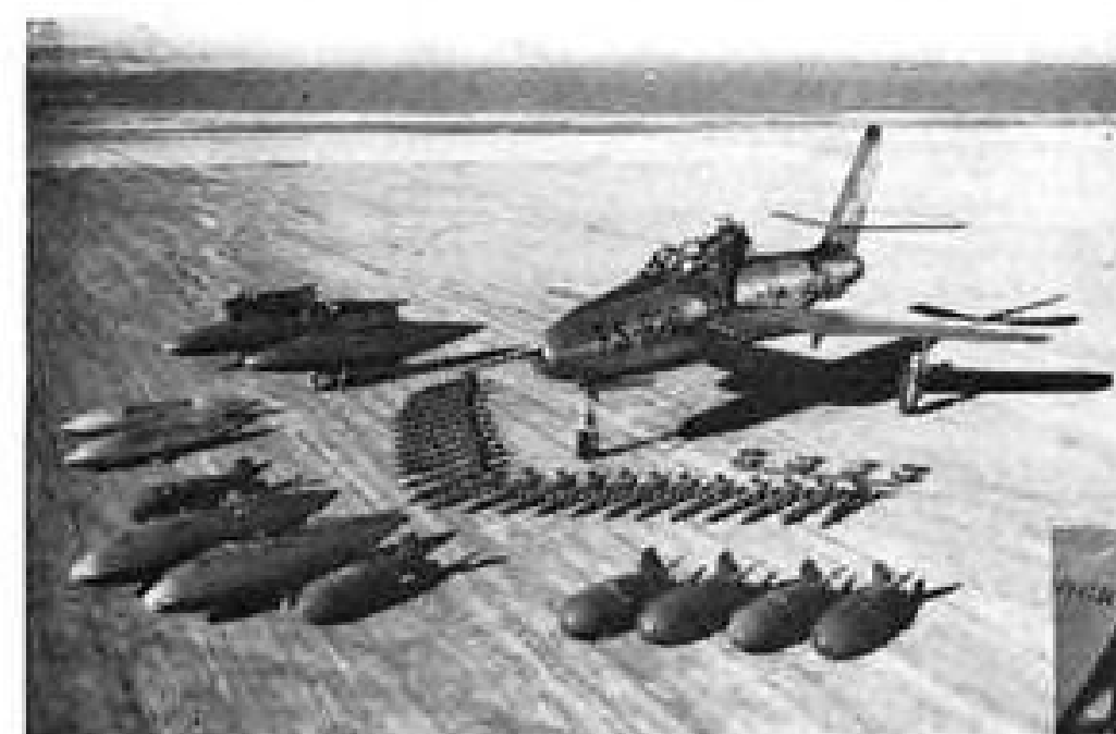
Photo (left) shows the wide variety of armament carried externally by the F-84F . . . 24 five-inch HVAR Rockets, or four 1000 lb. bombs, or two 1000 lb. bombs and two 230 gal. fuel tanks. Other armament such as Napalm tanks, smoke tanks, or anti-personnel bombs can also be carried.
