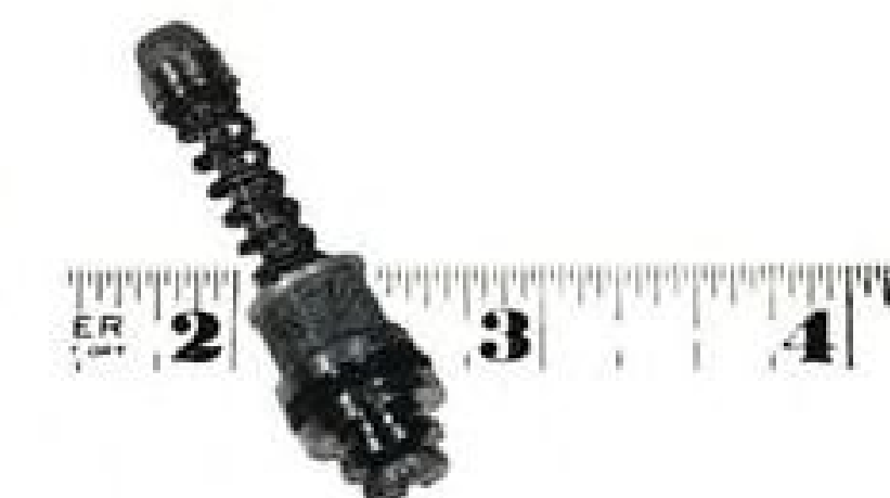
Advanced design fuel nozzle for ramjets and afterburners.
