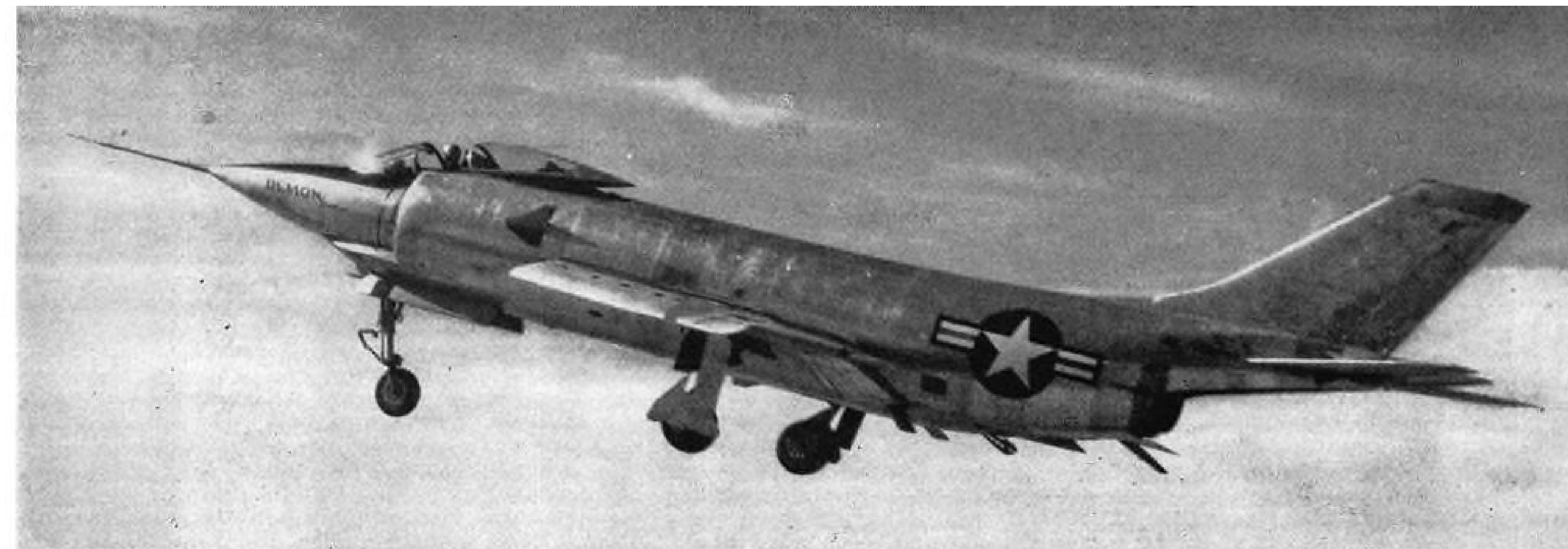
McDONNELL TRIES OUT DEMON —First unretouched photos of McDonnell XF3H-1 Demon carrier-based Navy jet fighter (above and below) show some detail blotted out by censors in earlier pictures. Note the large intake, previously concealed, for the Westinghouse J40 engine. In the above takeoff view, the plane's "droop snoot" leading edge is extended and the variable-angle tail has its leading edge well down.
