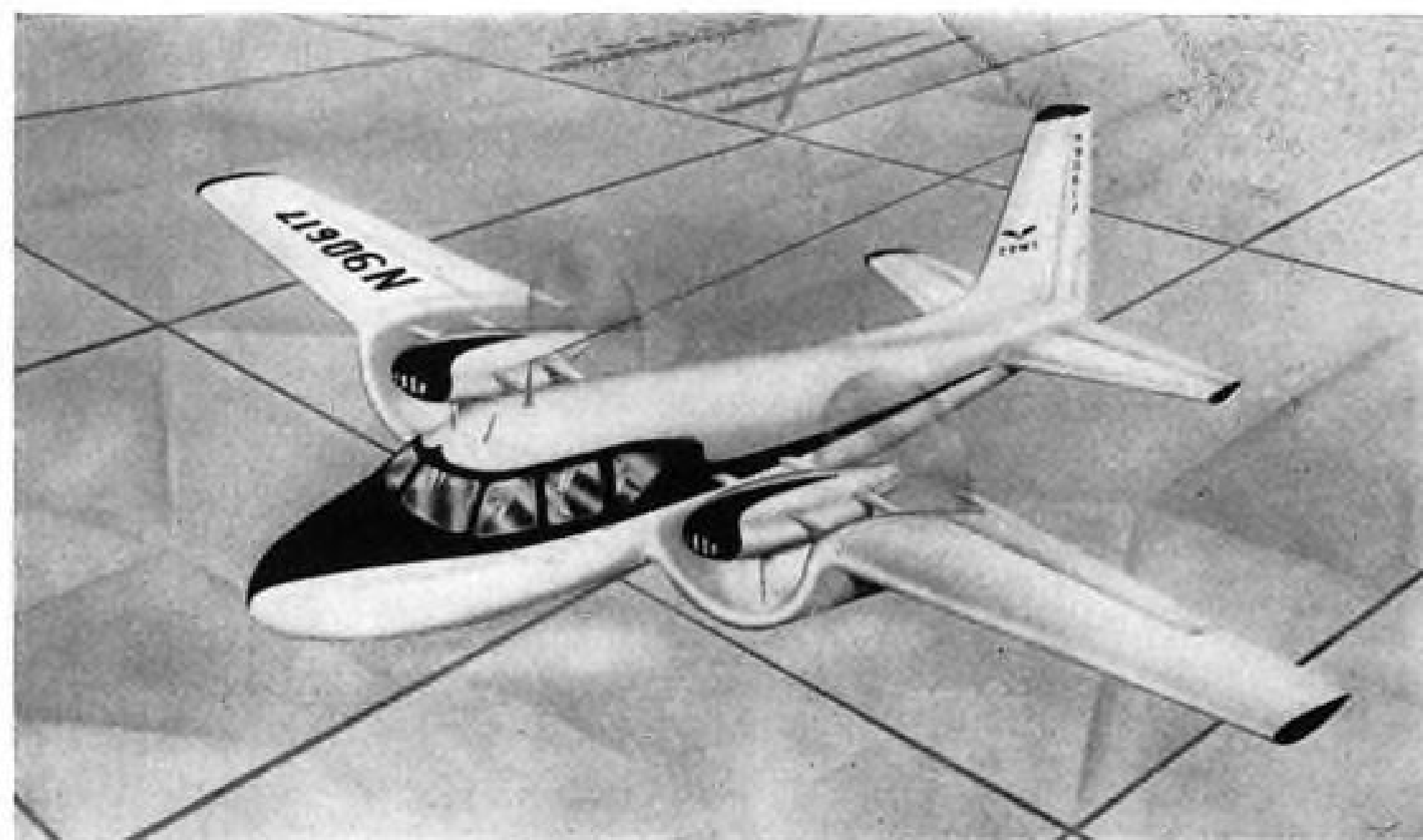
ONE PROPOSED APPLICATION of the Custer channel wing configuration is the CCW-5, which would combine a Baumann Brigadier airframe with the unusual wing.
