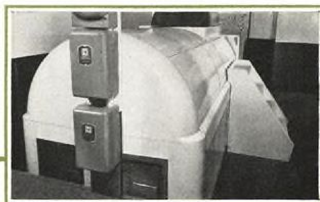
Front View of C-11B Jet Flight Trainer as it appears installed in its mobile training room. Steps lead to pilot's station under the canopy. Trailer training room is 14 x 20 with wall extended.
