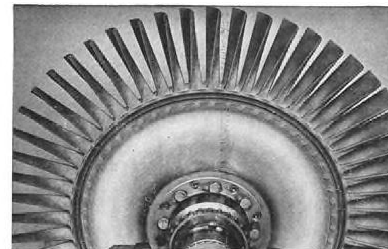
HERE IS HOW the Nimonic "80A" blading of a J-42 turbine looks after 500 hours of test running. The blades, according to Pratt & Whitney, are in almost as good condition as they were at the start of the test.
