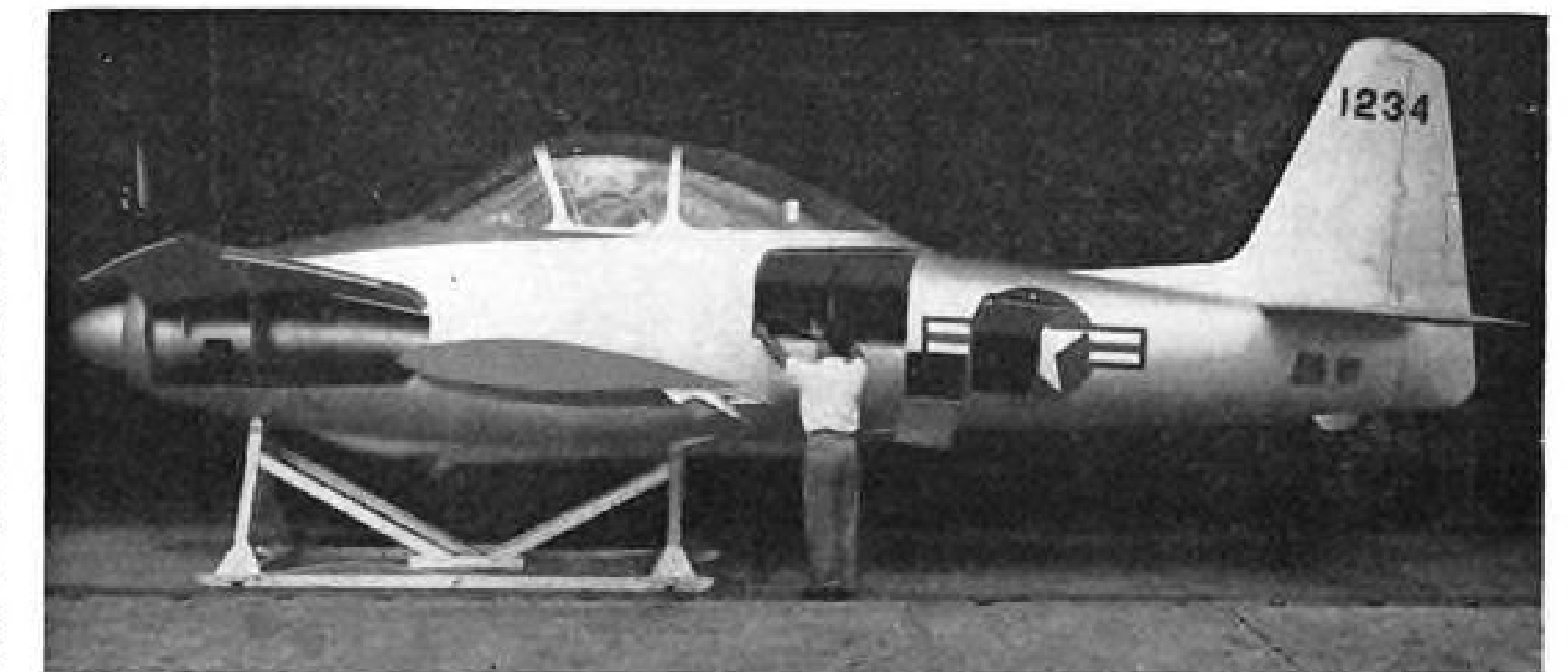
FUSELAGE MOCKUP of turboprop trainer designed by Temco Aircraft Corp., Dallas, for USAF competition won by Cessna (Aviation Week Jan. 1, p. 15). Photo of Temco Model 27 shows liberal use of access panels to ease maintenance. Slated to be powered by an Armstrong Siddeley
