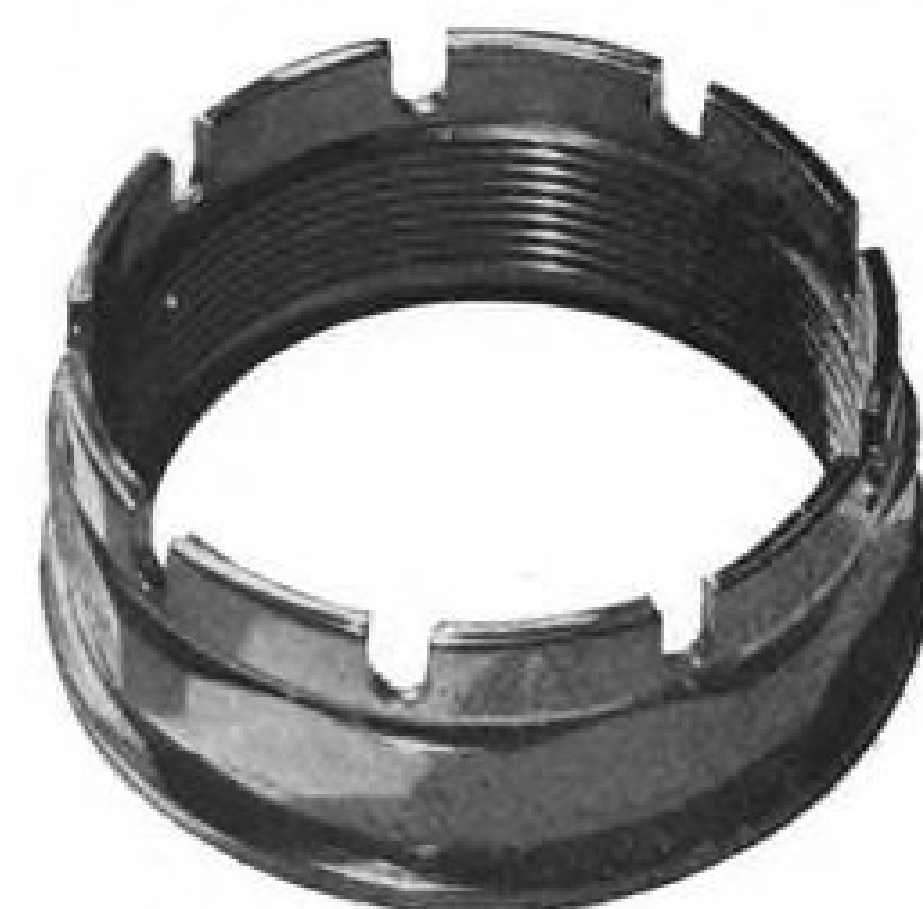
Propeller Nut Forged From 5% Nickel-Aluminum Bronze produced by MUELLER BRASS CO. for use in conventional aircraft.
