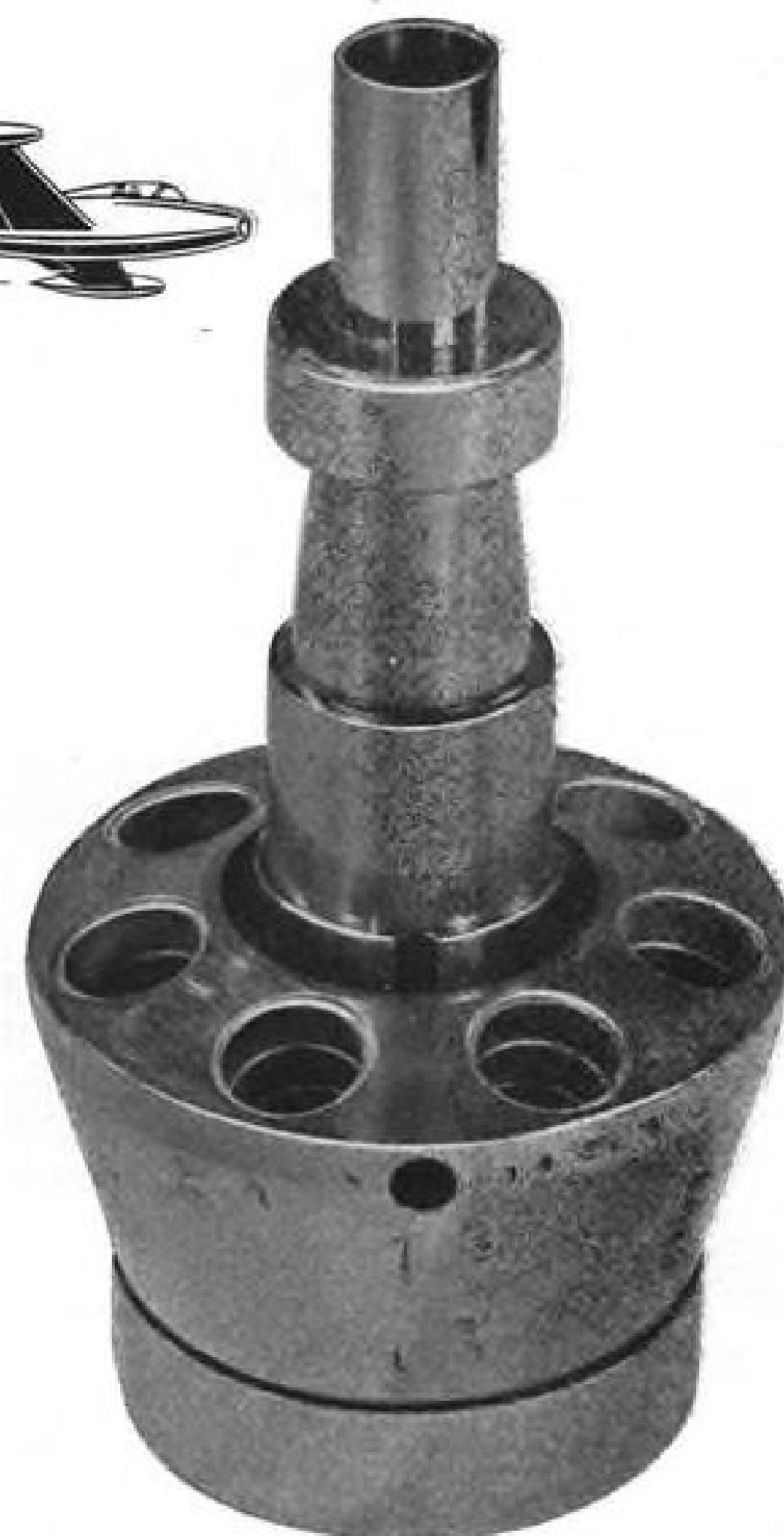
Fuel Pump Plunger Rotor of 5% Nickel-Aluminum Bronze. This is a heat-treated forging produced by MUELLER BRASS CO., Port Huron, Michigan, for use in jet aircraft engines.
