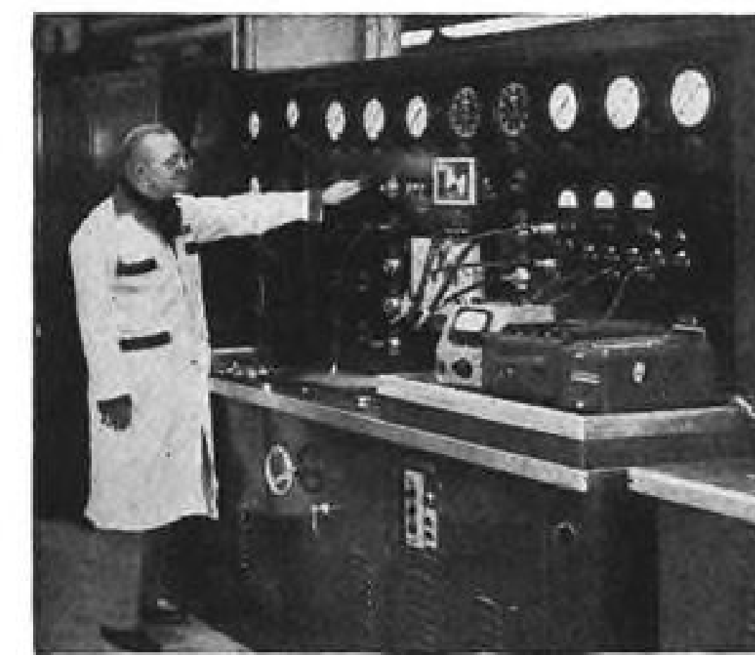
Greer Hydraulic Control Pump Test Stand meets the high quality control standards required at Westinghouse. Components are inspected under simulated flight conditions.
