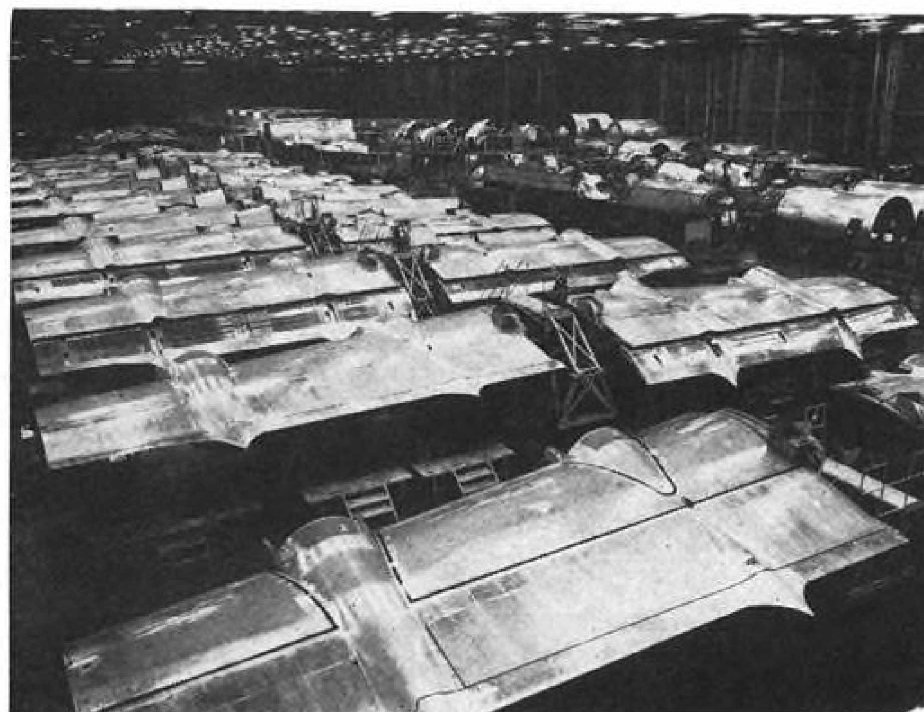
WINGS are given the finishing touches in this line before the panels are moved to the horseshoe swing for hookup to the fuselage.
