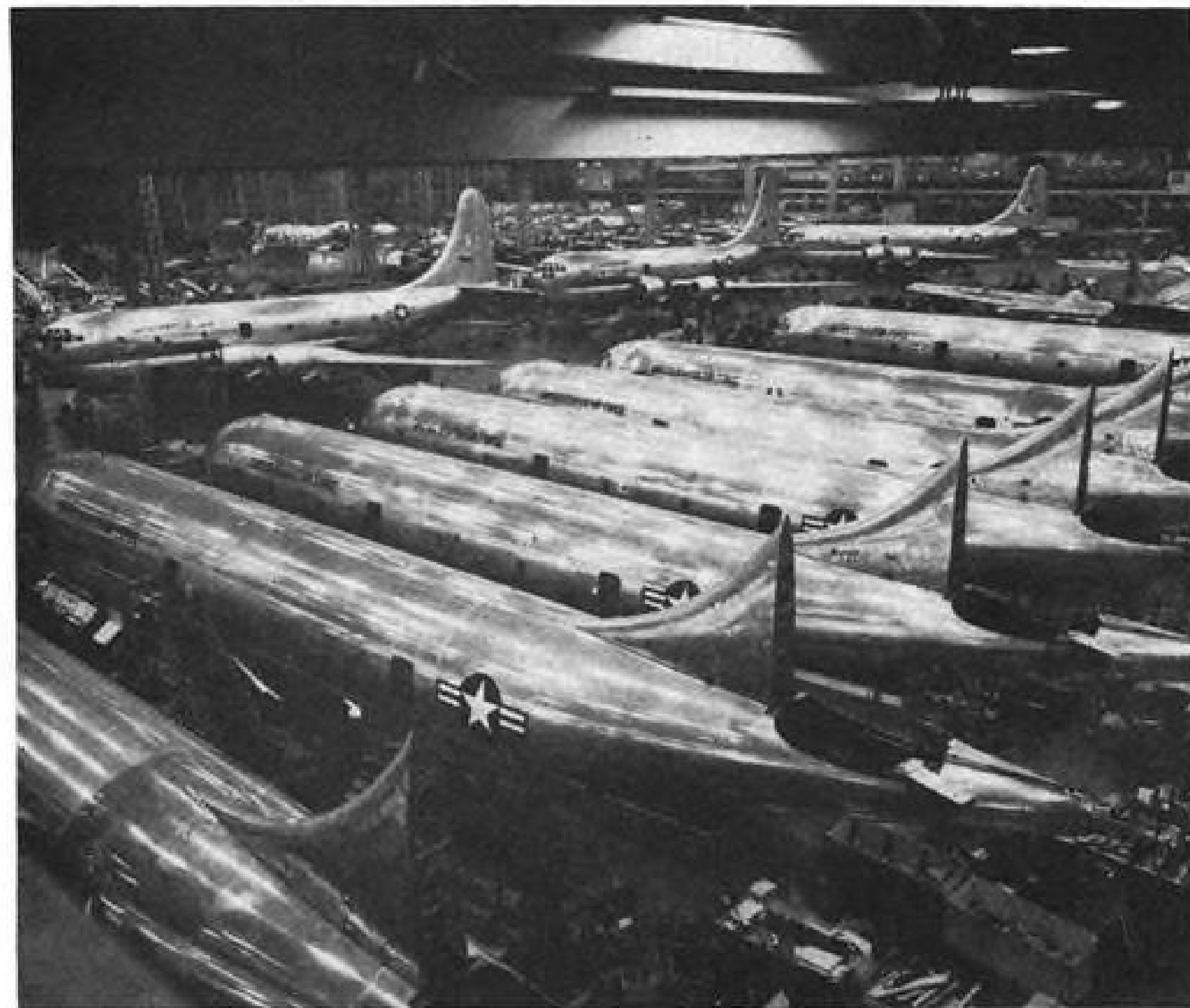
FUSELAGES are lined up, ready to be fed into horseshoe-shaped final line. Aft fuselage takes refueling pod or cargo doors.
