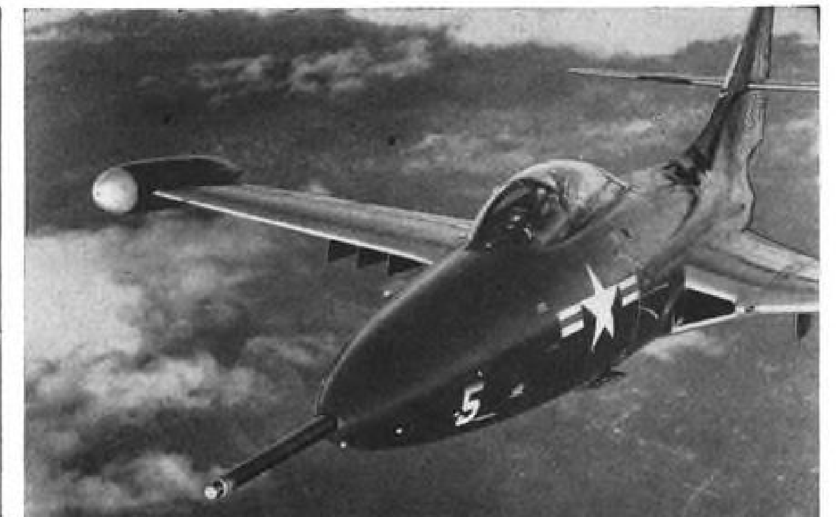
This fighter pilot flies nose probe into tanker's drogue where coupling is made automatically. Disconnect is made by reducing flight speed.
