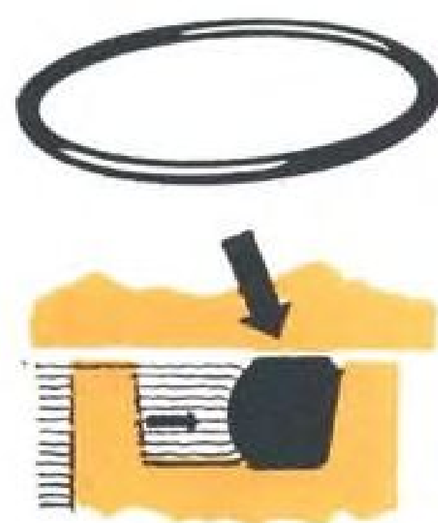
Cross section drawing of O-ring in groove, sealing under pressure.
