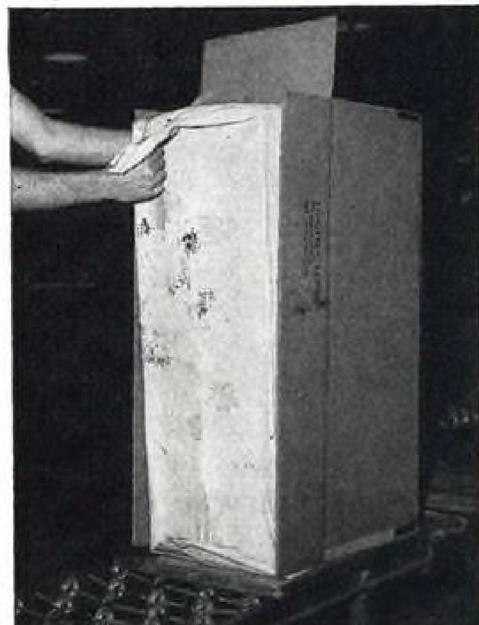
2. The carton is then bagged in an aluminum foil-lined sack from which the air is removed. This bag is placed in a slightly larger carton.
