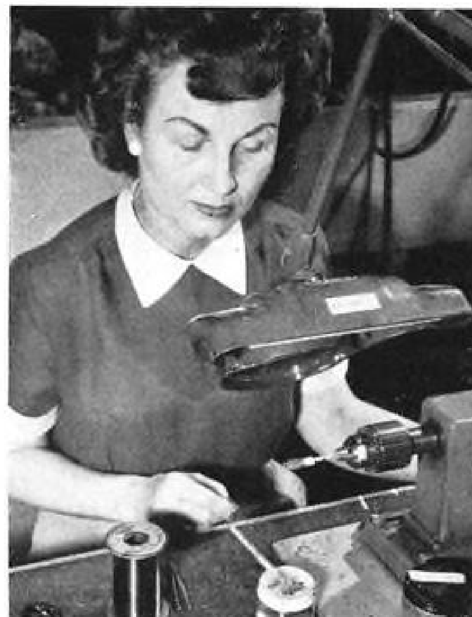
BIRTH of NAA transformer: winding . . .
