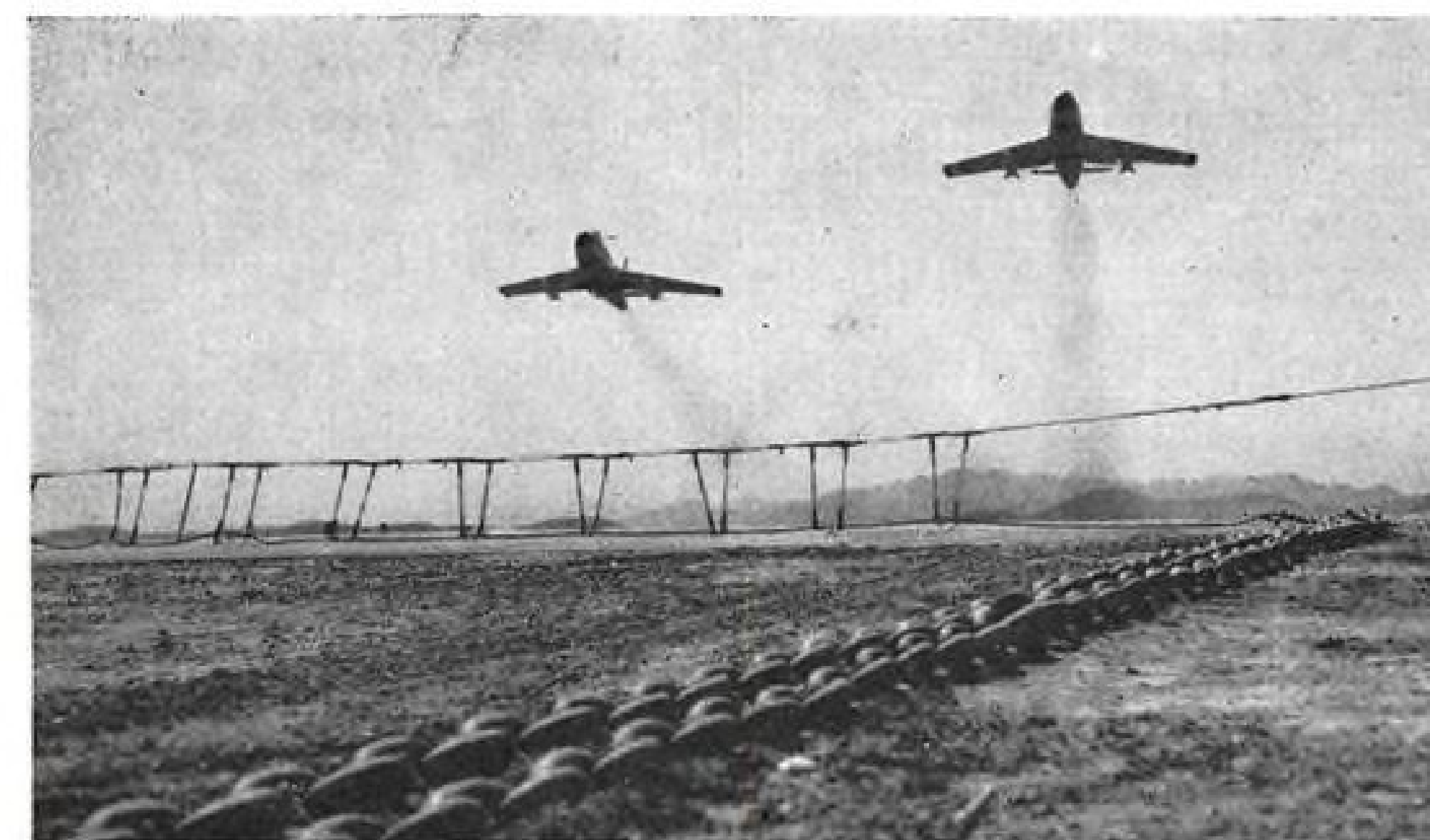
ARRESTING GEAR stretches across runway at Korean air base during F-86 takeoffs.
