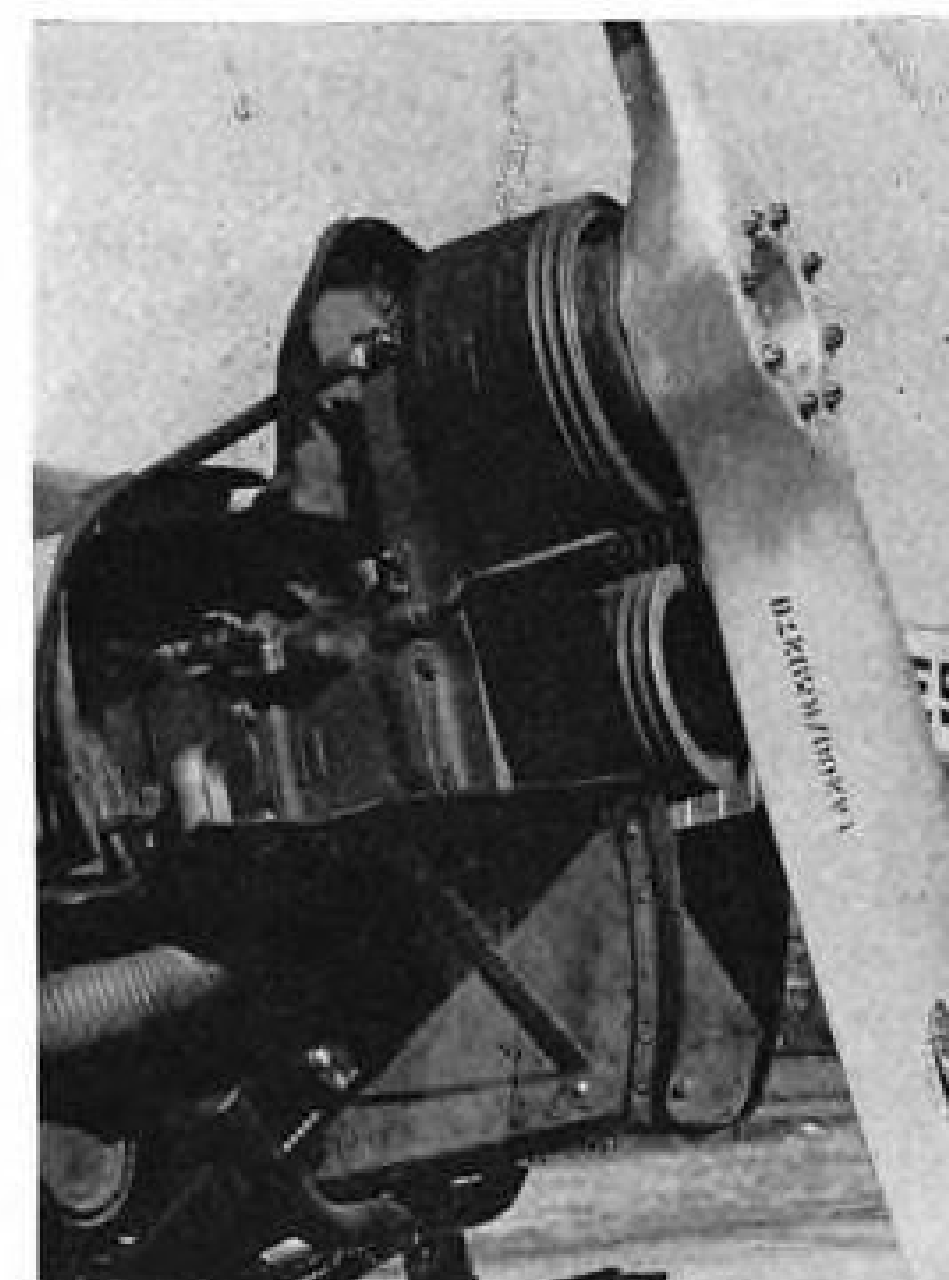
CESSNA 170'S V-BELTS are still usable after more than 800 hours running time.
