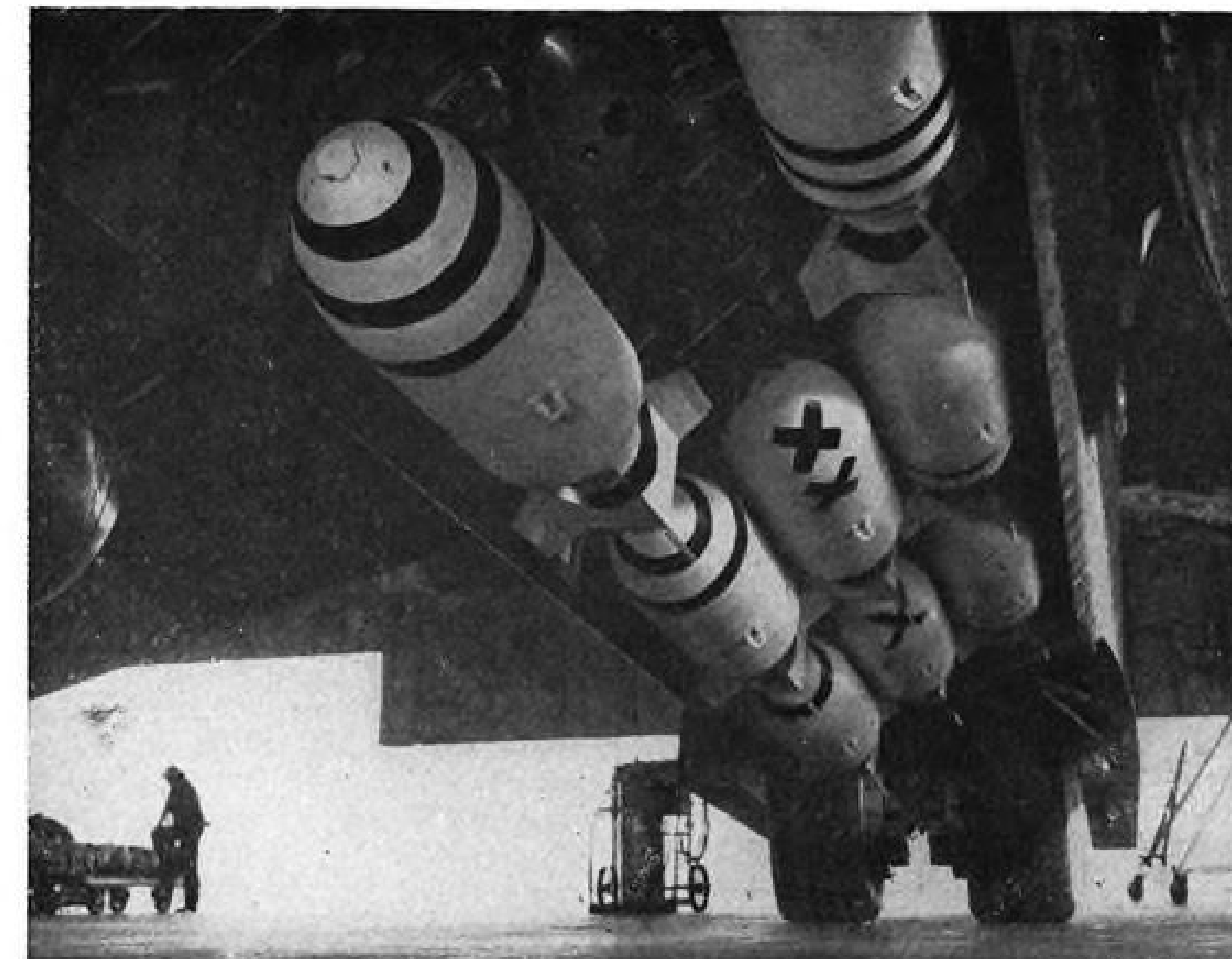
ROTARY BOMB DOOR is shown approximately three-fourths of the way through the 180-deg. turn the device makes to place it into position so the bombs can be released.
