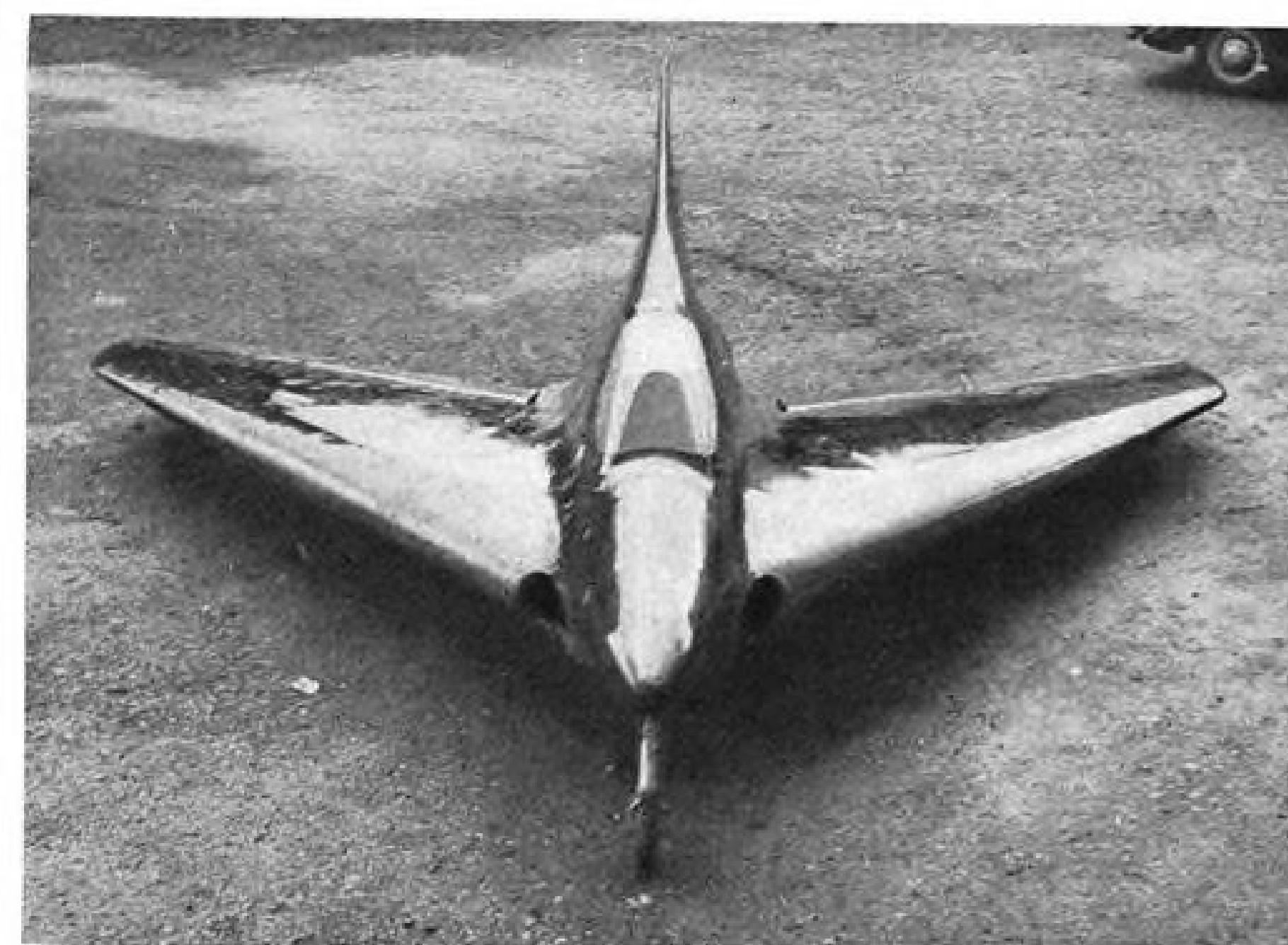
FRONT VIEW of Payen P.A.49 shows experimental plane's delta wing and jet-engine air inlets on either side of fuselage.
