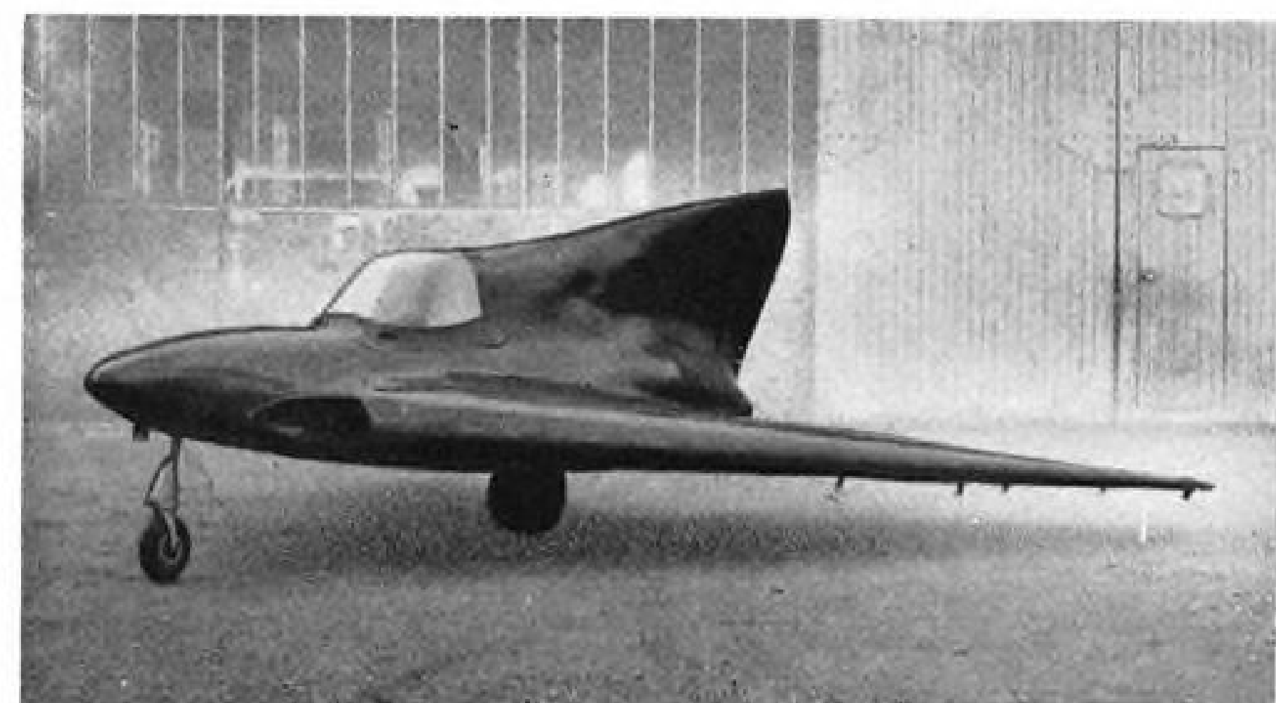
PROFILE shows how cockpit faired into vertical tail. Landing gear has main wheel under fuselage. No balancing outriggers are visible.
