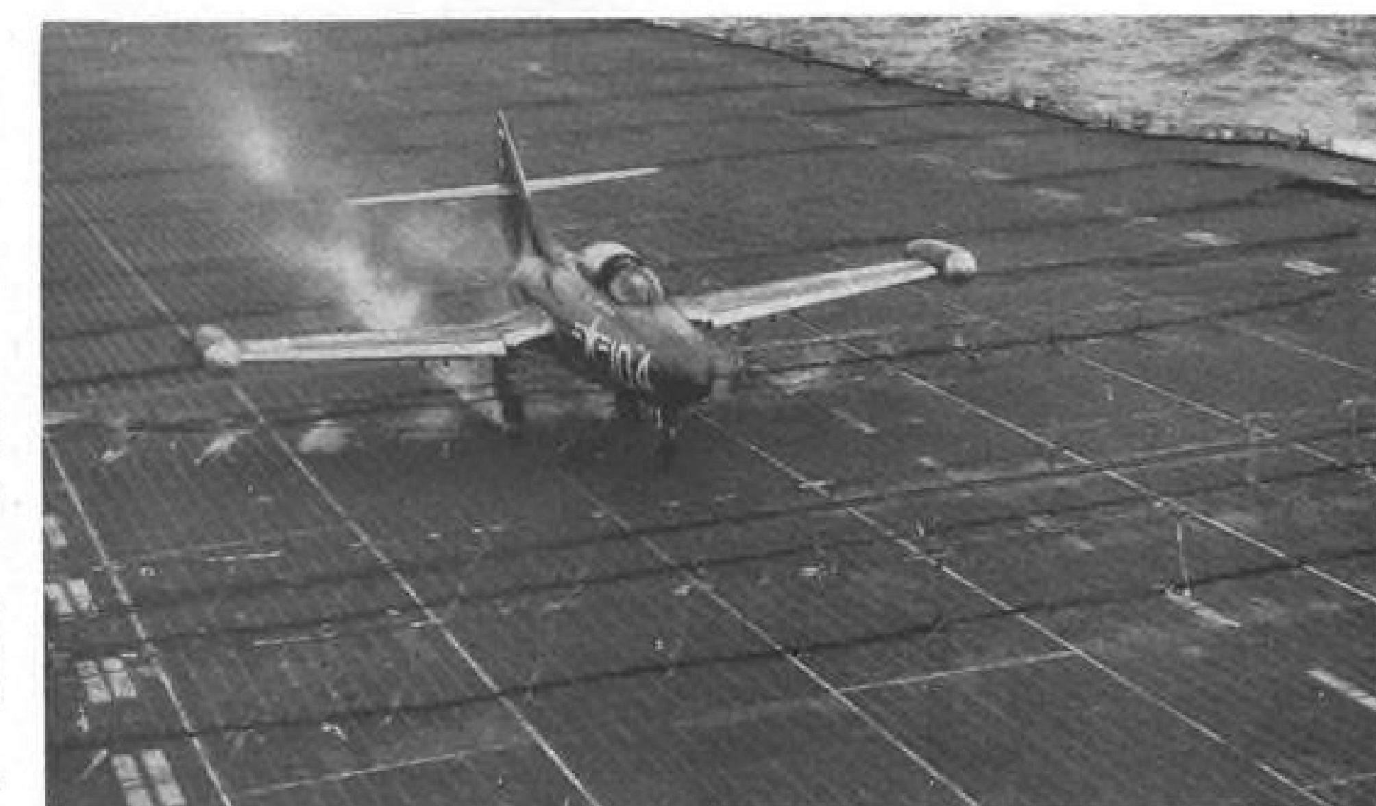
CONTACT with first of three nylon barriers is made by Panther's nose gear, but no slowing of jet's run is yet evident. Now look at last photo, below.
