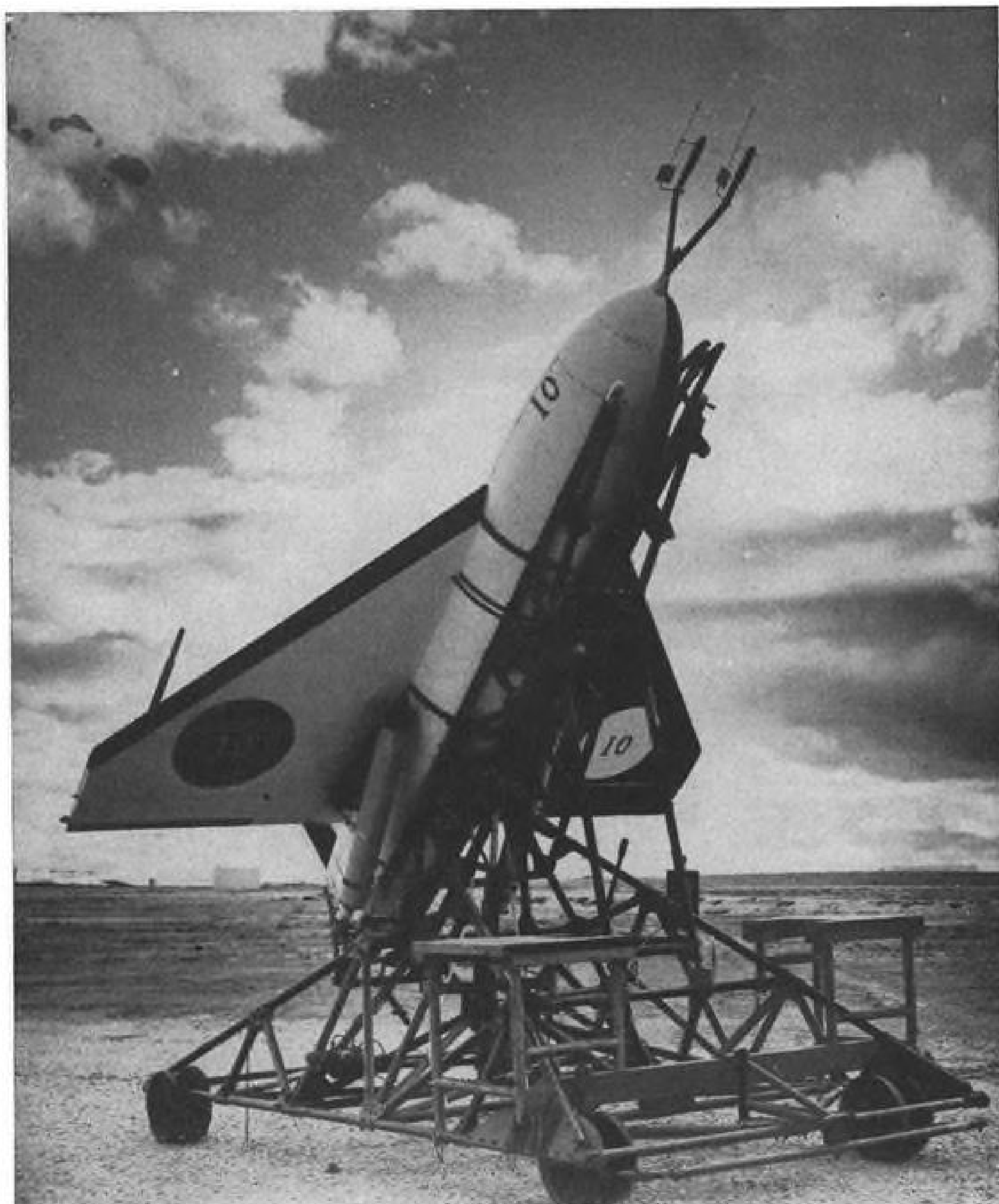
FAIREY vertical takeoff delta rocket model gets set for test at Woomera missile range.
