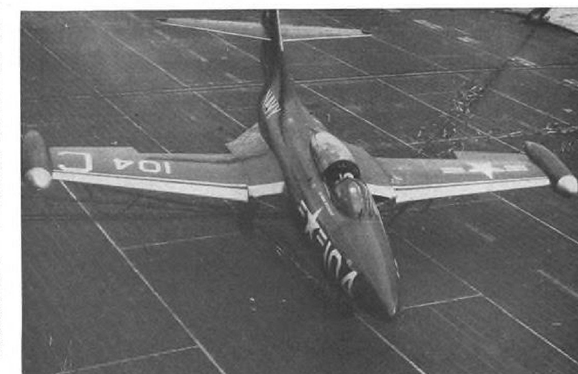
HALTED by all three barriers clutching at tricycle landing gear, F9F's tail lurches into air. Shoulder harness protects pilot from effects of sudden stop.
