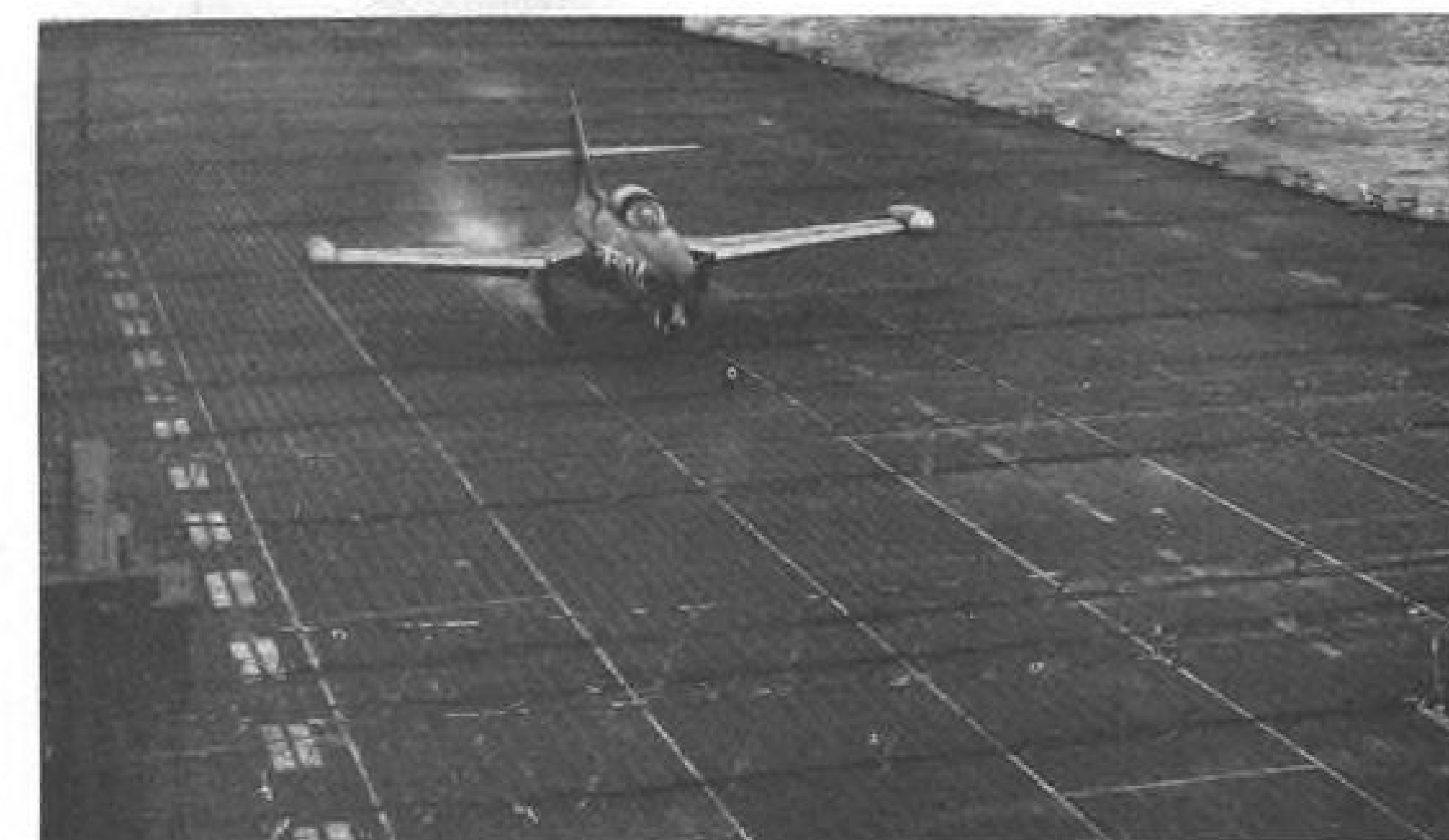
F9F-2 Grumman Panther jet fighter, tires smoking, passes over raised arresting cables on deck of USS Franklin D. Roosevelt and heads for raised crash barriers.
