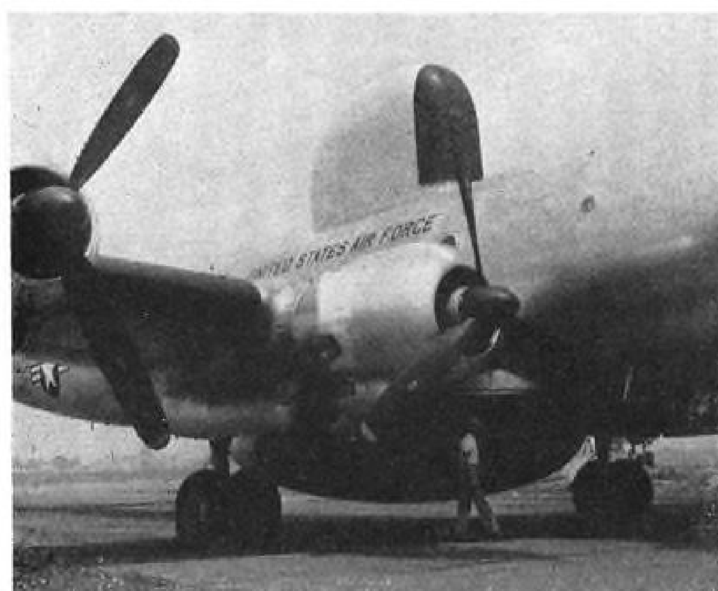
FRONT VIEW of RC-121C's top and bottom radomes.
