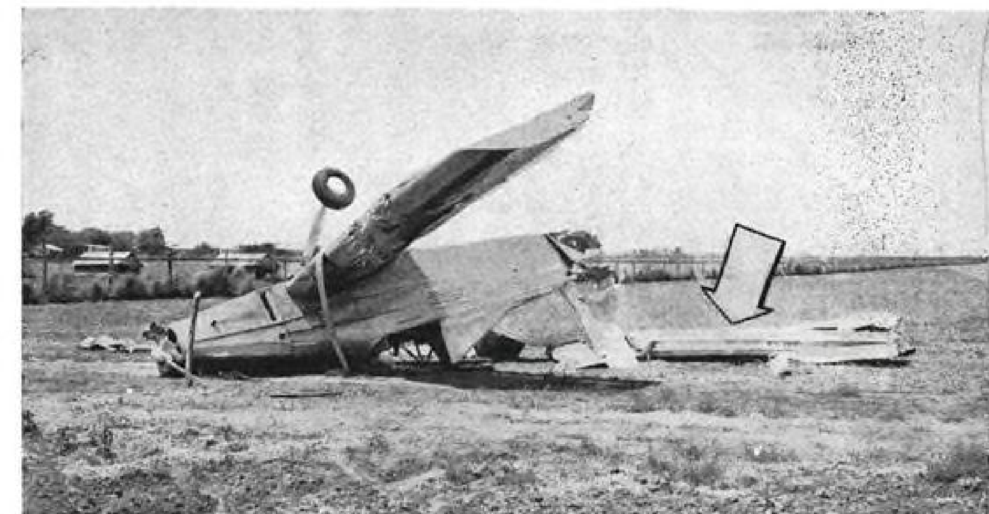
AG-1 CRASHED in this inverted position, but because of plane's crash-safety features, pilot walked away uninjured. Arrow points to AG-1's left wing.
