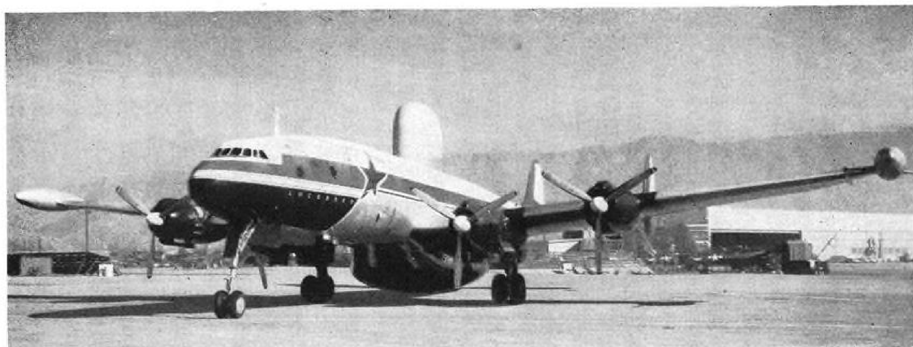
EXPERIMENTAL SUPER CONNIE, used by Lockheed to test radar picket installations, has wingtip fuel tanks.
