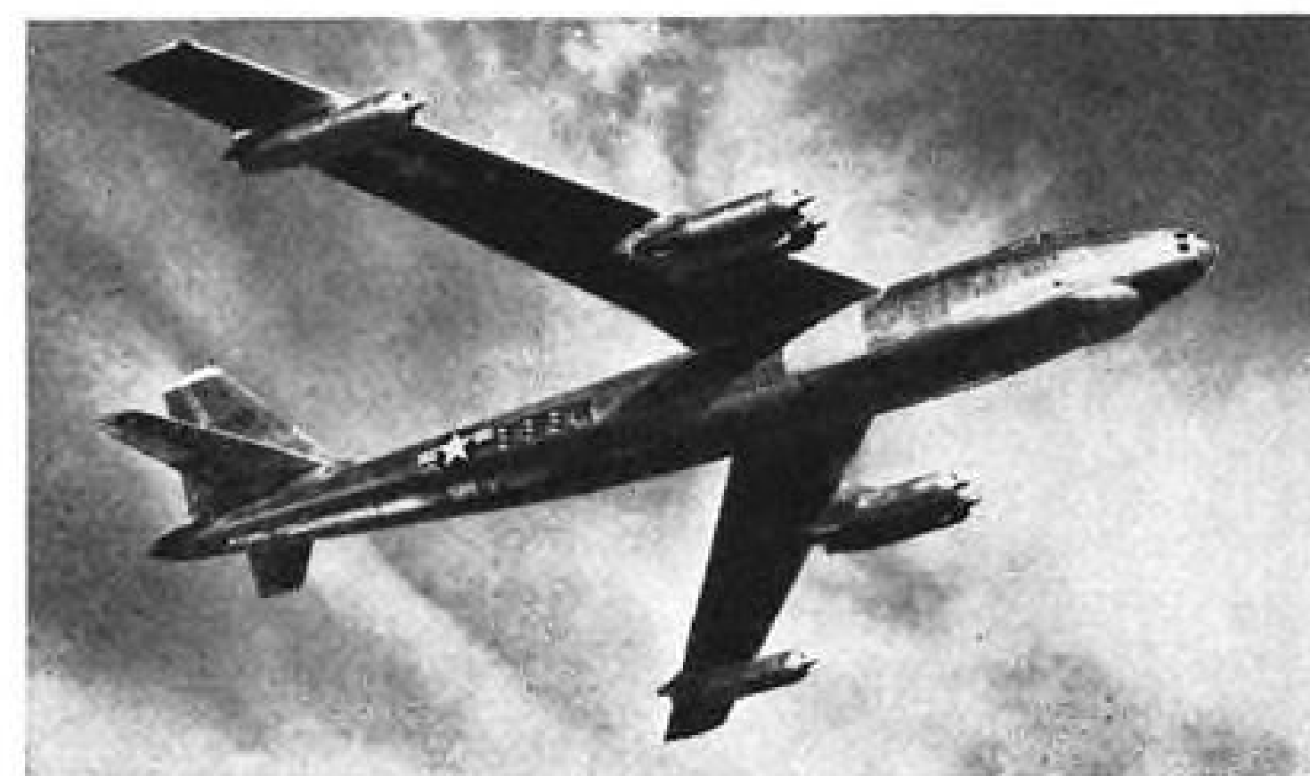
POWERED BY SIX G-E J47-25 engines, the Boeing B-47 Stratojet can now fly twice as many hours between engine overhauls . . . a direct result of G.E.'s engine improvement and development program and the USAF's quality control and field maintenance program.
