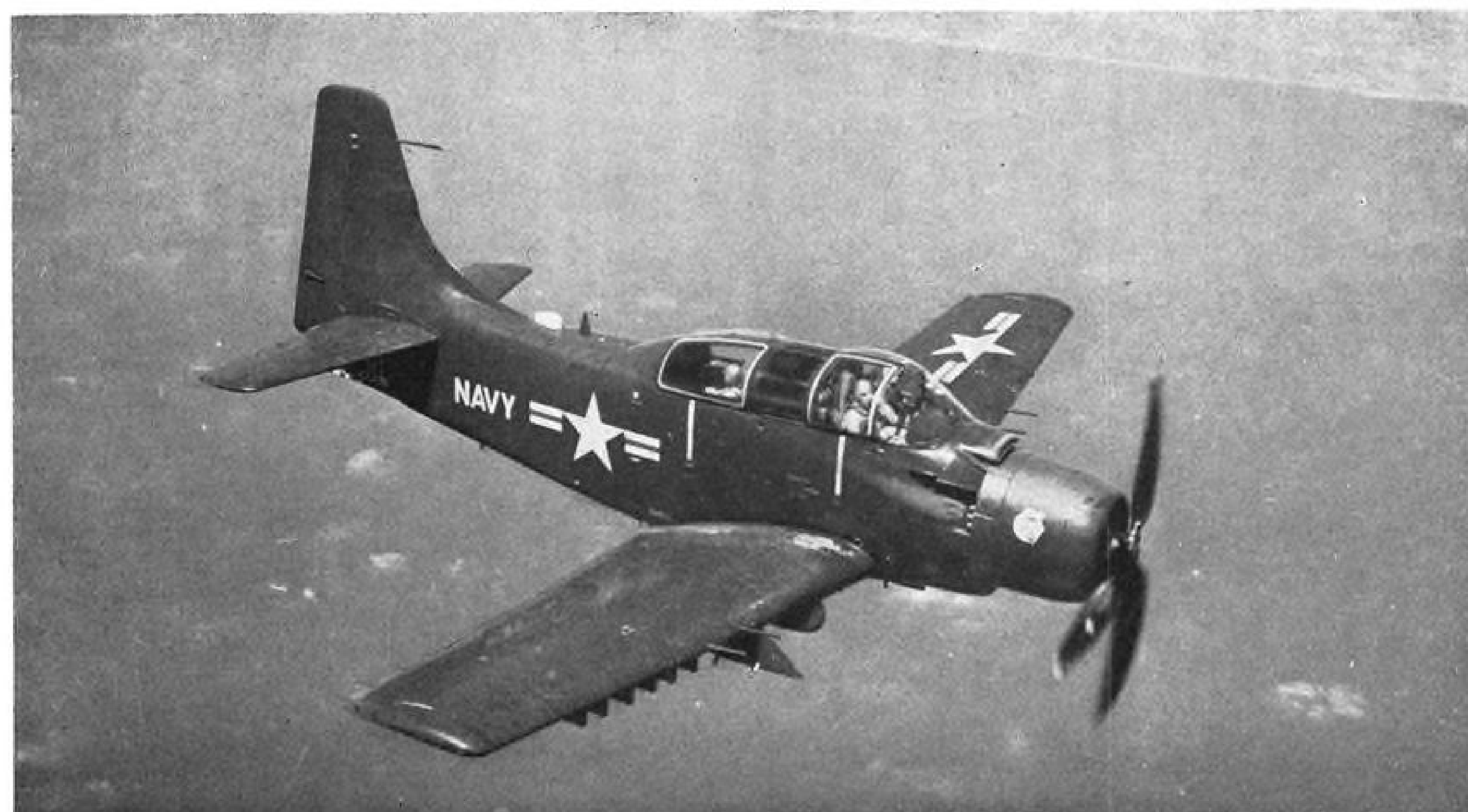
DOUGLAS AD-5 Skyraider differs externally from previous models mainly in new cockpit layout and slightly larger tail. Note four 20-mm. cannon protruding from wings and racks for rockets, bombs or napalm tanks.
