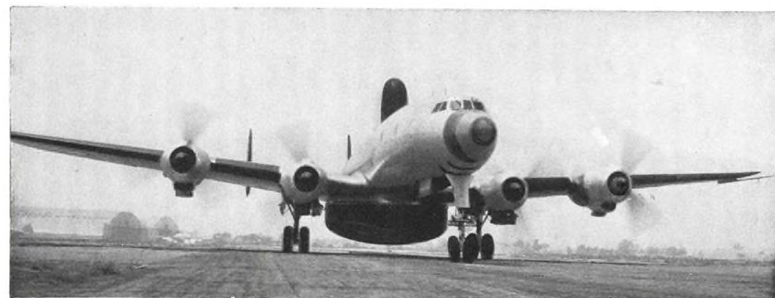
LOCKHEED RC-121C RADAR PICKET, with wide belly radome plus one atop fuselage, presents odd aspect from this angle.
