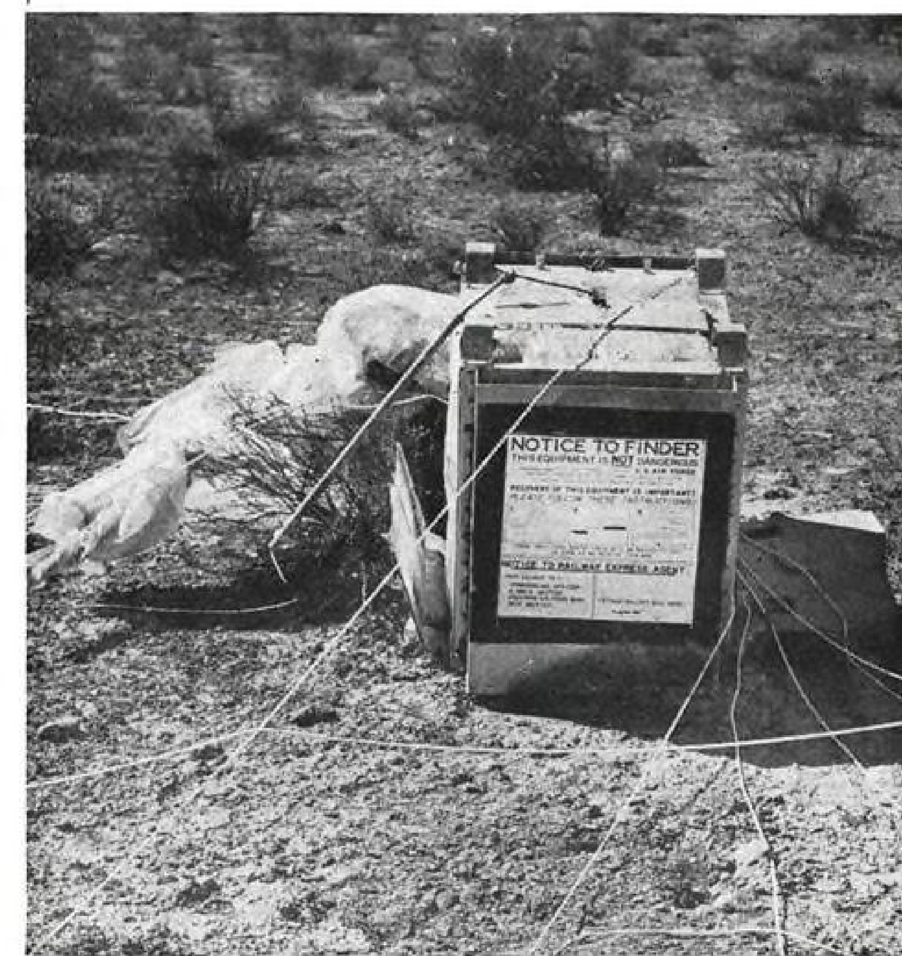
INSTRUMENTS are parachuted to ground, terminating flight to altitude.
