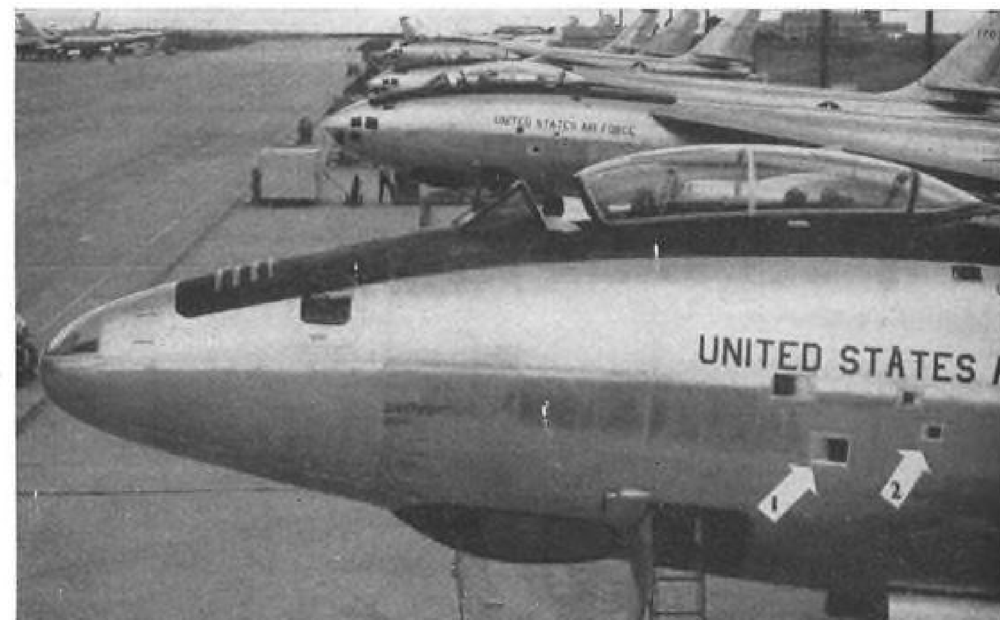
CLOSEUP OF RB-47E camera nose with B-47E bomber in immediate background points up differences in planes. Arrows indicate: (1) cooling unit inlet, (2) inverter ventilation inlet.
