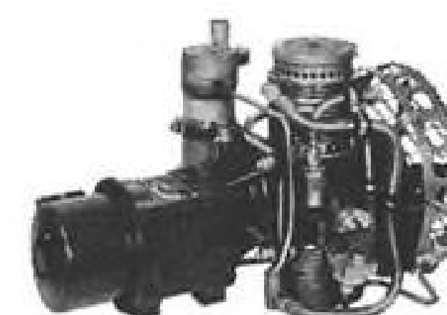
Airborne. 28v—2 hp motor. Vertical sump. At sea level, and at 15,000 ft. delivers 2 cfm of free air compressed to 3,000 psi.
