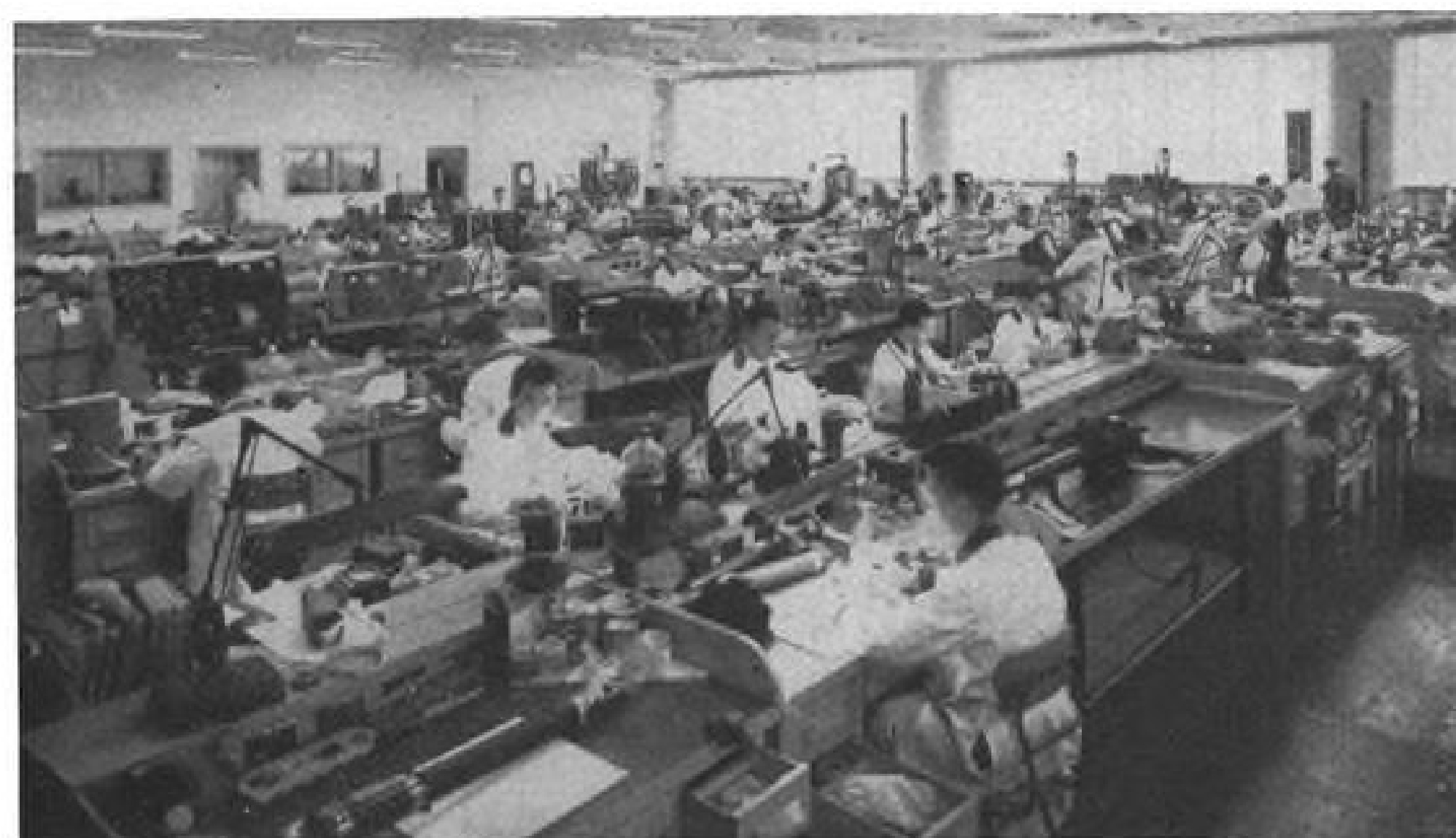
INSTRUMENT OVERHAUL is accomplished in air conditioned shop; at right, driftmeter is checked by technician.
