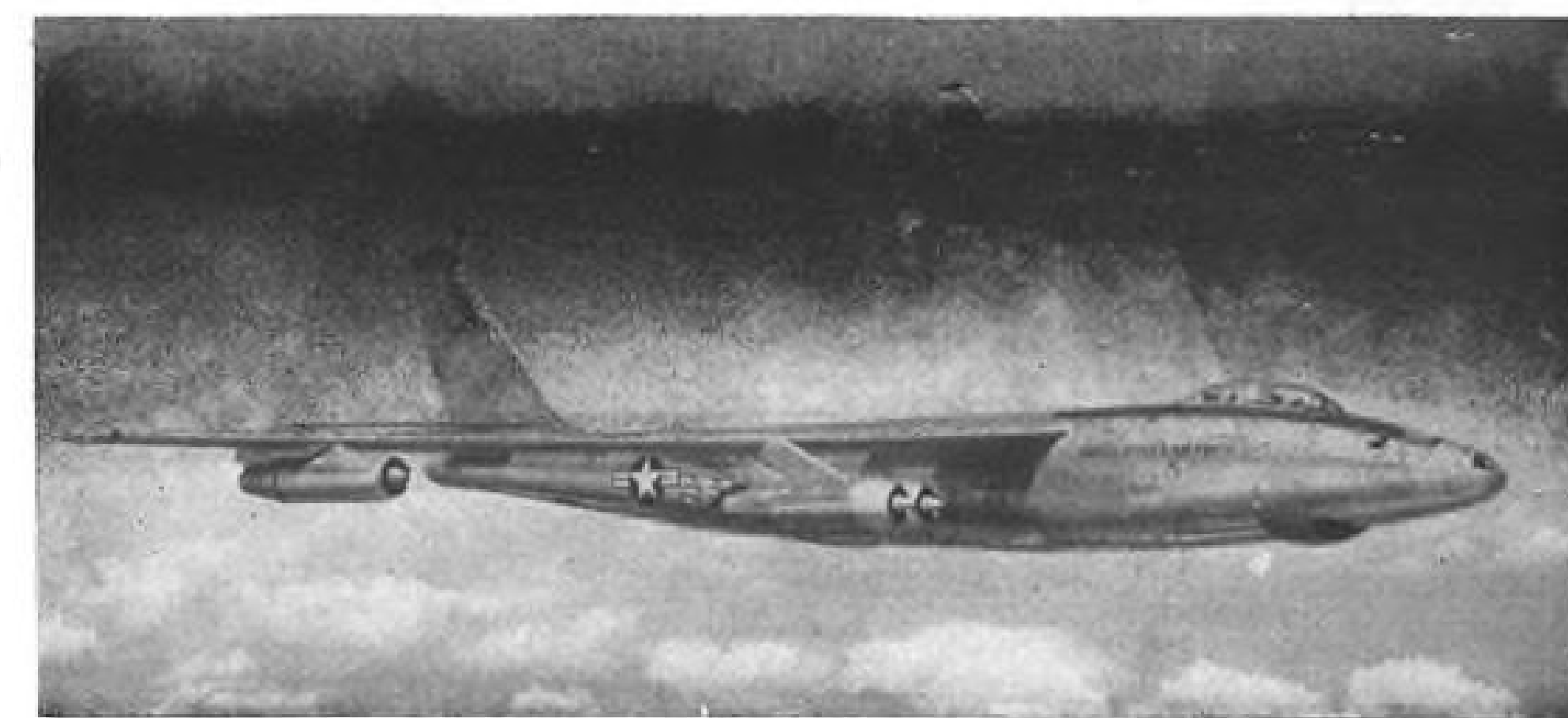
BOEING RB-47E camera plane (foreground) flying with B-47E bomber. Note longer nose on RB-47E compared with that on B-47E. Both planes have radar-directed tail gun turrets.
