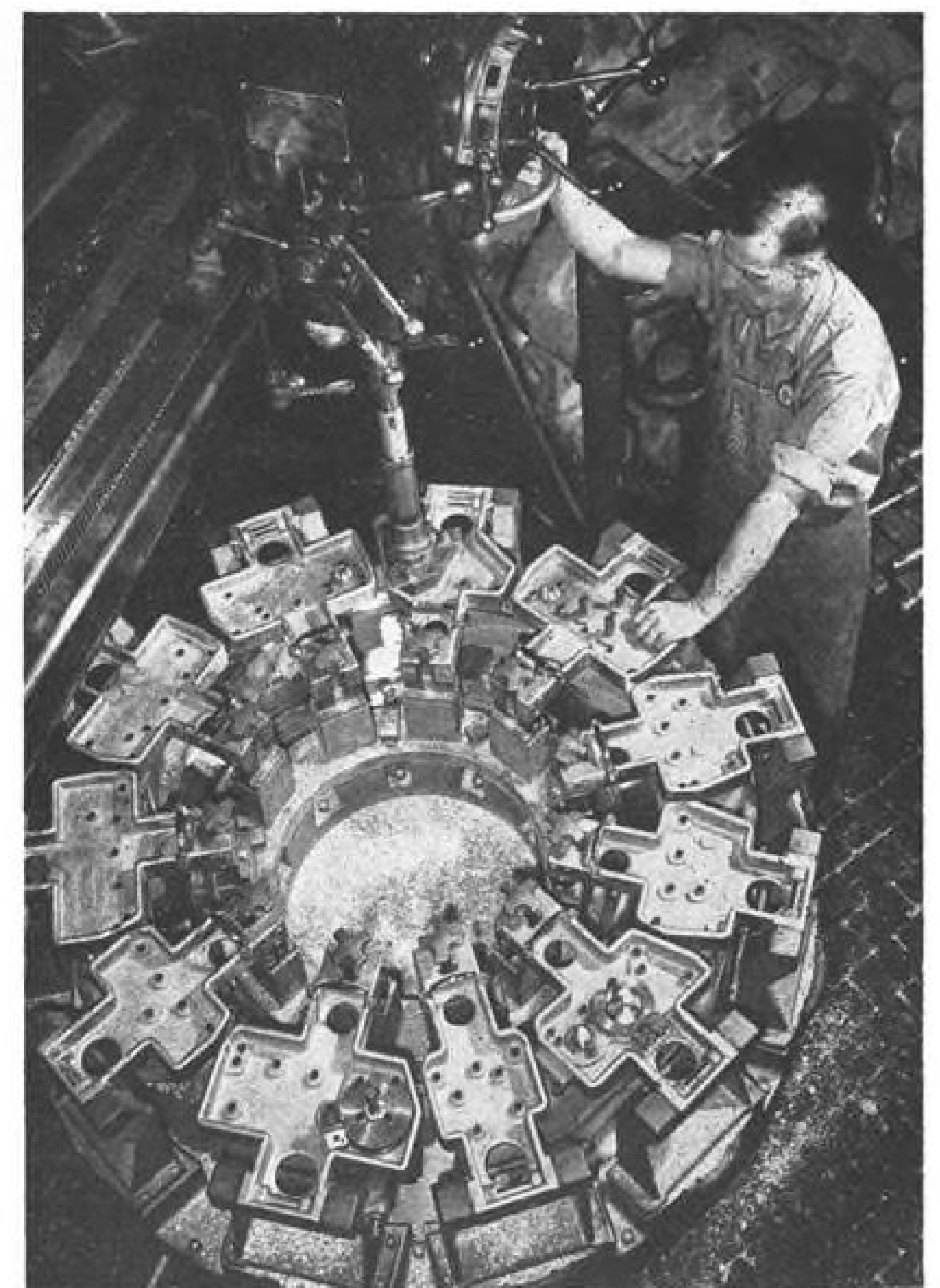
DRILL JIG took man-work-year to design and build.
