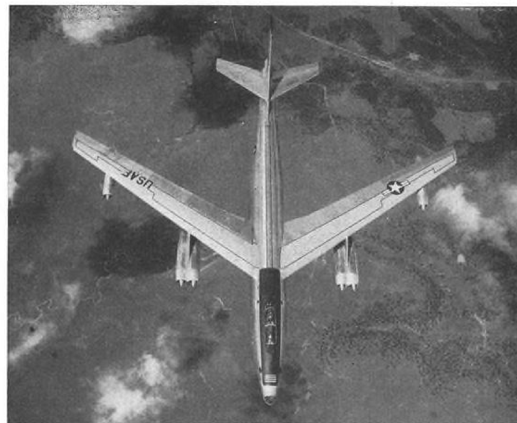
PLAN VIEW of RB-47E Stratojet provides a good look at the 600-mph.-plus plane's sweptwing configuration. This model of the aircraft carries cameras in its nose.
