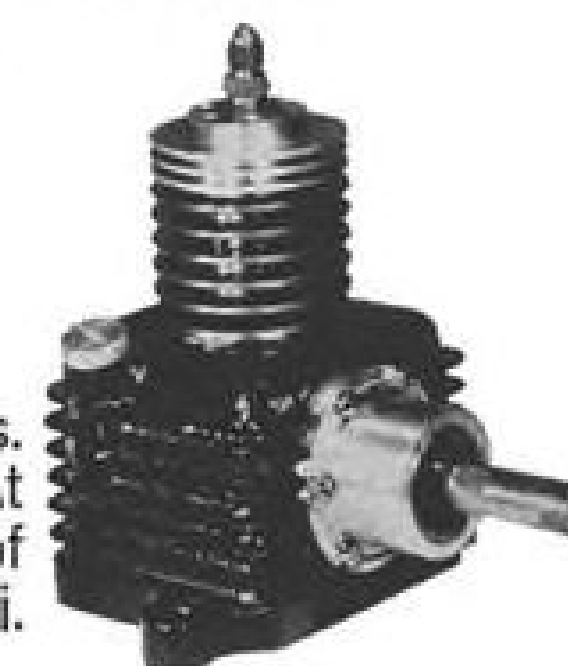
Ground application. Here the compressor can be driven by a 60 cycle 220 volt motor.
