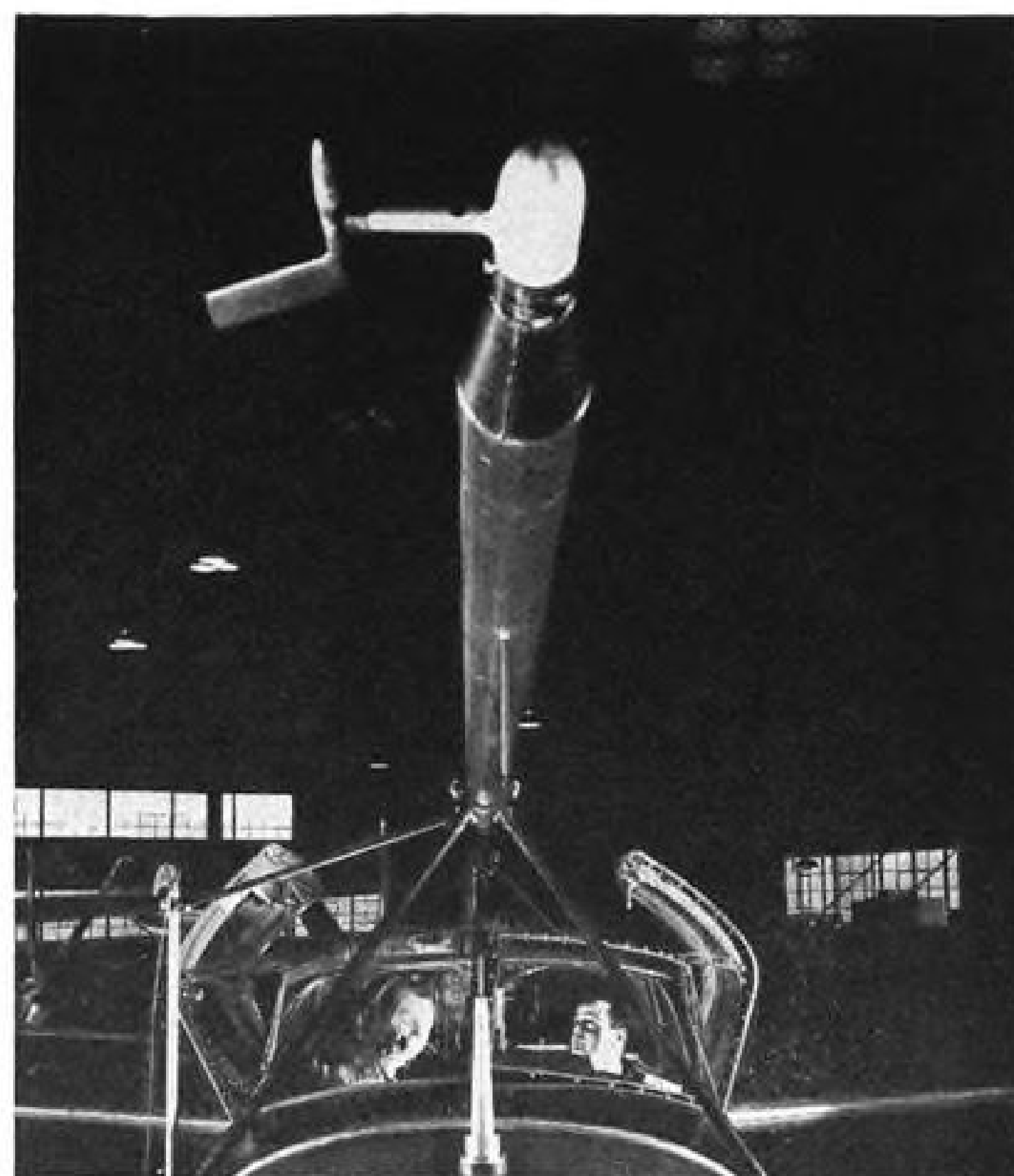
PERISCOPE? No—part of a G-E radar-autopilot-armament system. The boom (installed in B-26) measures pitch and yaw signals for determination of system performance. Such devices help G-E engineers get pin-point accuracy in flight-testing new aviation gear
