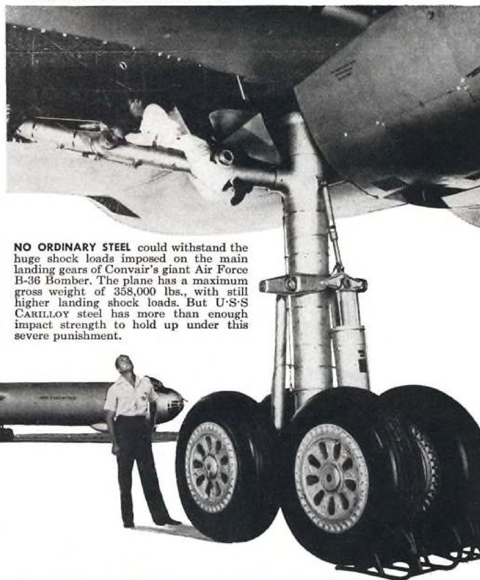
U-S-S CARILLOY electric-furnace aircraft quality steel meets every requirement for these vital parts. The precision machining and expert heat treatment they get at Cleveland Pneumatic Tool Company complete the job.
