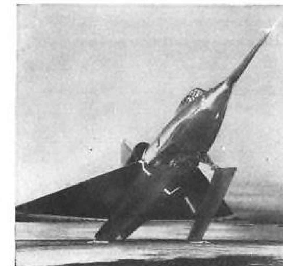
The Convair XF2Y-1 "Sea Dart", experimental U. S. Navy jet seaplane, is one of the latest in a long line of Westinghouse powered, high-performance fighters. It is the world's first delta wing seaplane and the first known combat craft to use hydro skis.
