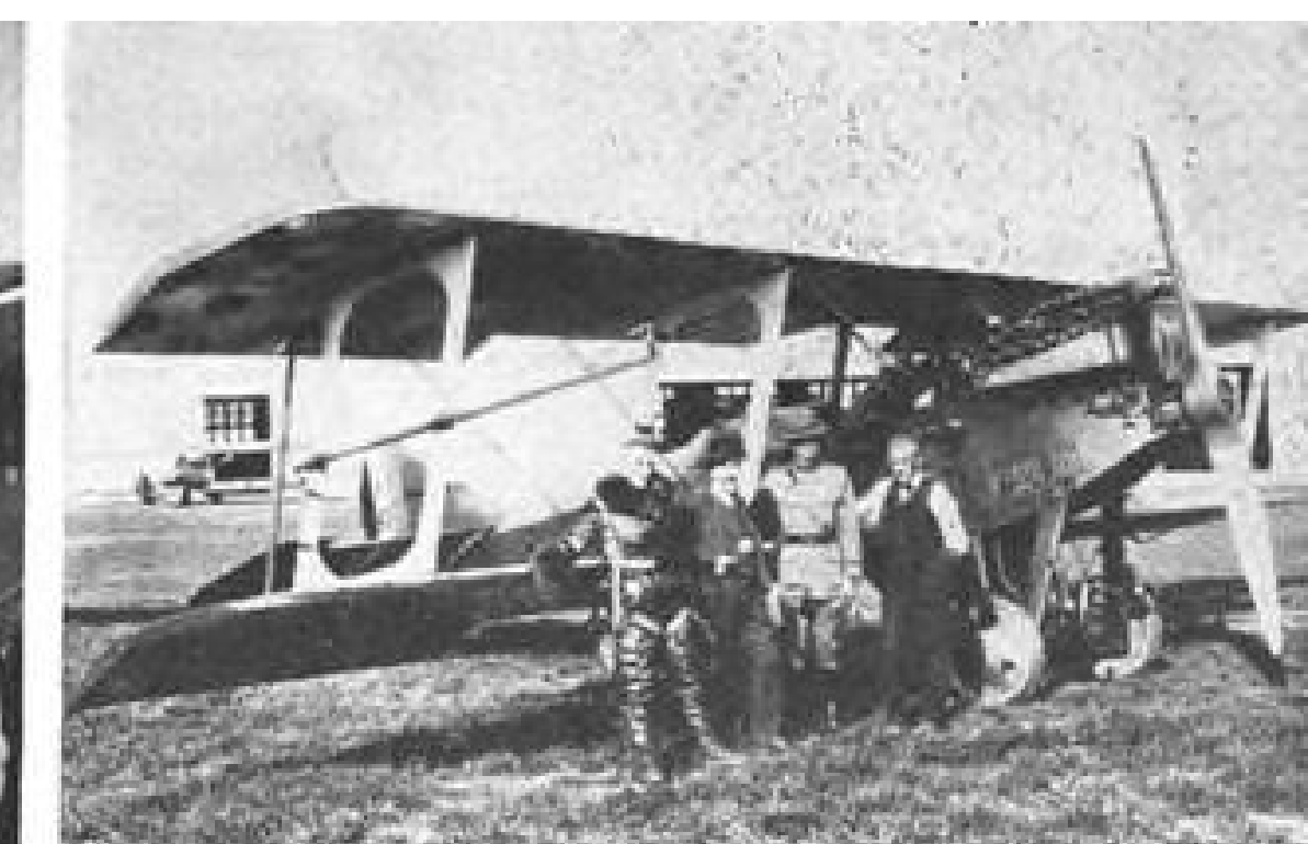
1921—Record altitude flight was made in "souped-up" turbo-equipped LePere biplane
