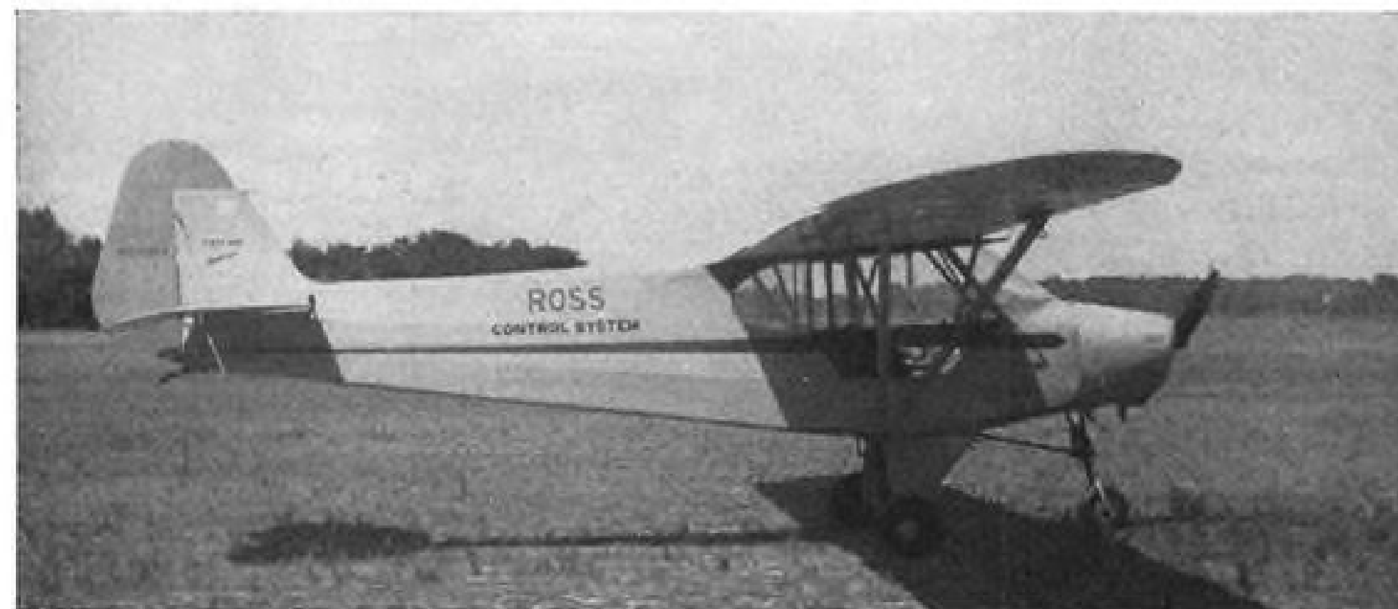
PIPER PA-11 was converted to tricycle landing gear for demonstration of Ross controls.
