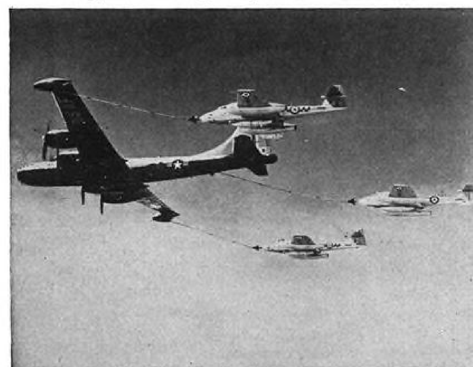
MULTIPLE. Several fighters can be refueled simultaneously with wing-tip hose units.
