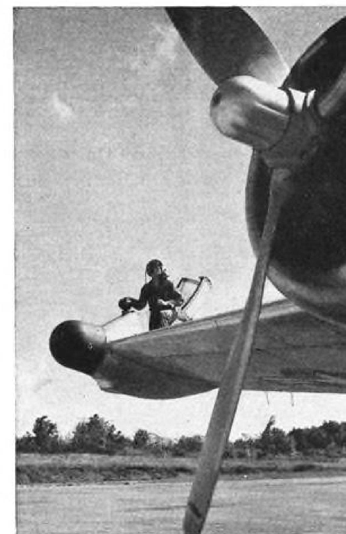
RADOME on tip of B-17 wing at Flight Test Center now carries special apparatus. But pods were originally designed for gunners and wing-tip observers.
