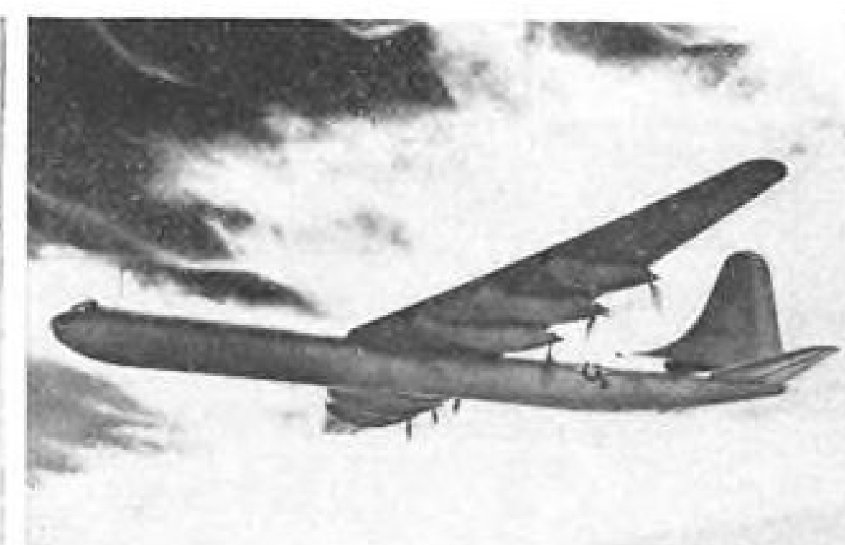
1946—twelve G-E turbosuperchargers help increase range and altitude of Convair B-36
