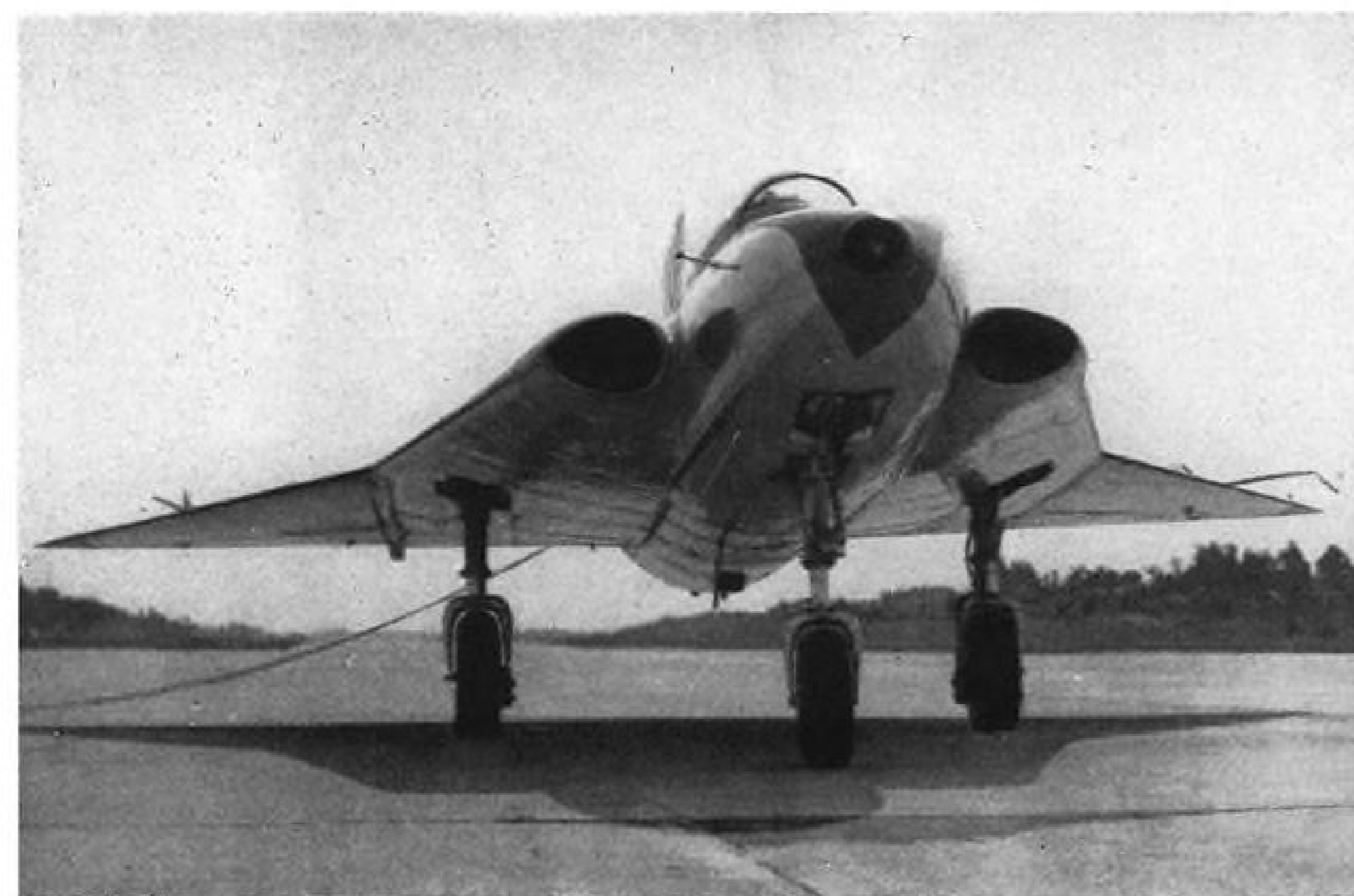
ALTITUDE PROBER —Model of new British experimental jet, Short Bros. & Harland's Sherpa (above), shows the altitude research craft's strange wing shape (Aviation Week Sept. 21, p. 14). Sherpa's aero-isoclinic wing is designed to deflect in bending, without twisting under aerodynamic load. Two Turbomeca engines power the plane.
