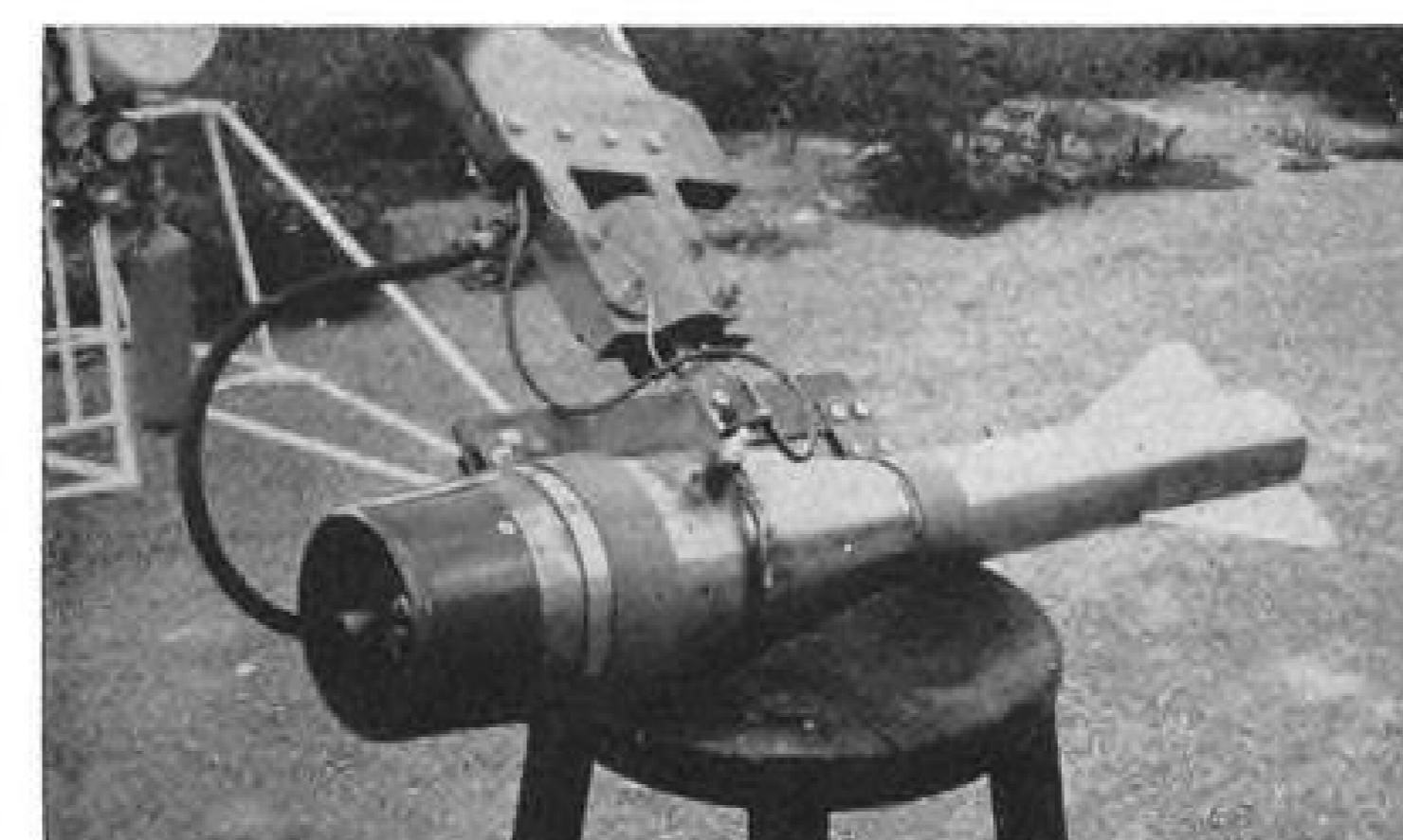
"ALMOST SILENT" PULSEJET ENGINE used by Schmidt delivers 105 lb. of thrust on special kerosene-base fuel.
