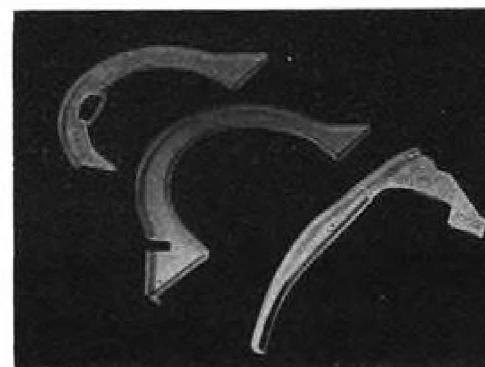
HOT-FORMED parts include 3-ft. cockpit floor tunnel (left) made on press brake and bulkhead sections of .064-in. Dow FS-1h24 magnesium made on hydraulic press.
