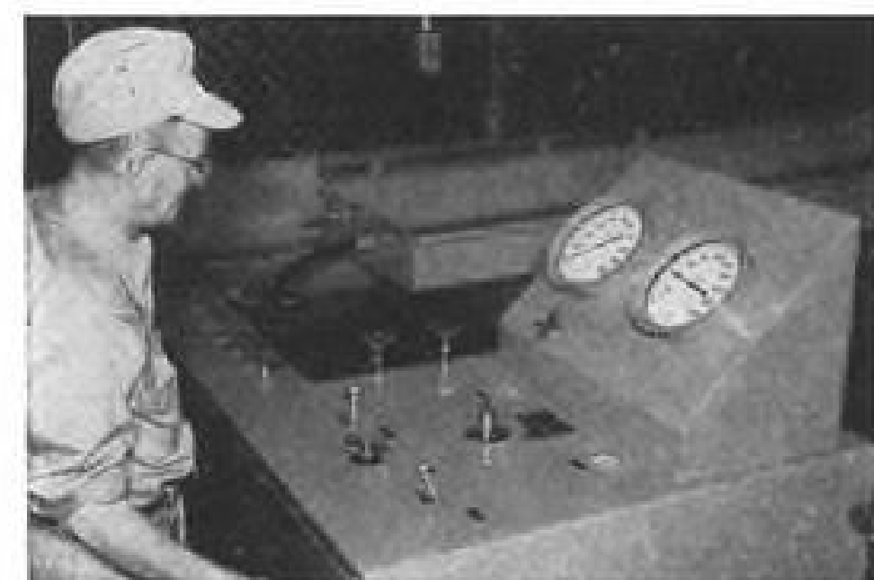
Greer Hose Tester tests from one to six hose lines or similar production components to pressure of 25,000 psi. Covered burst chamber is provided for safety.
