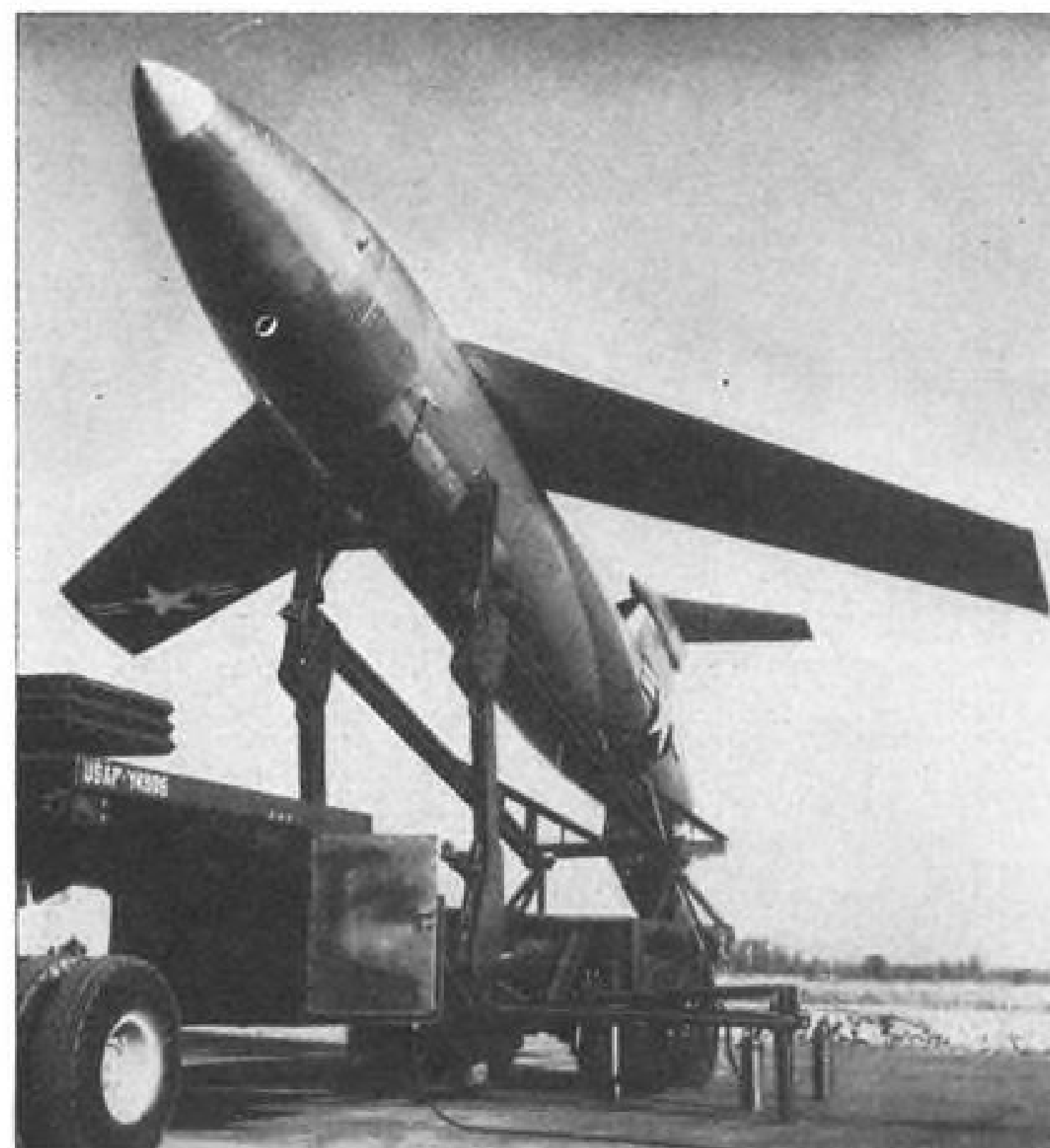
PRODUCTION VERSION of Martin Matador incorporates castings and metal bonding to make manufacturing easier and quicker.
