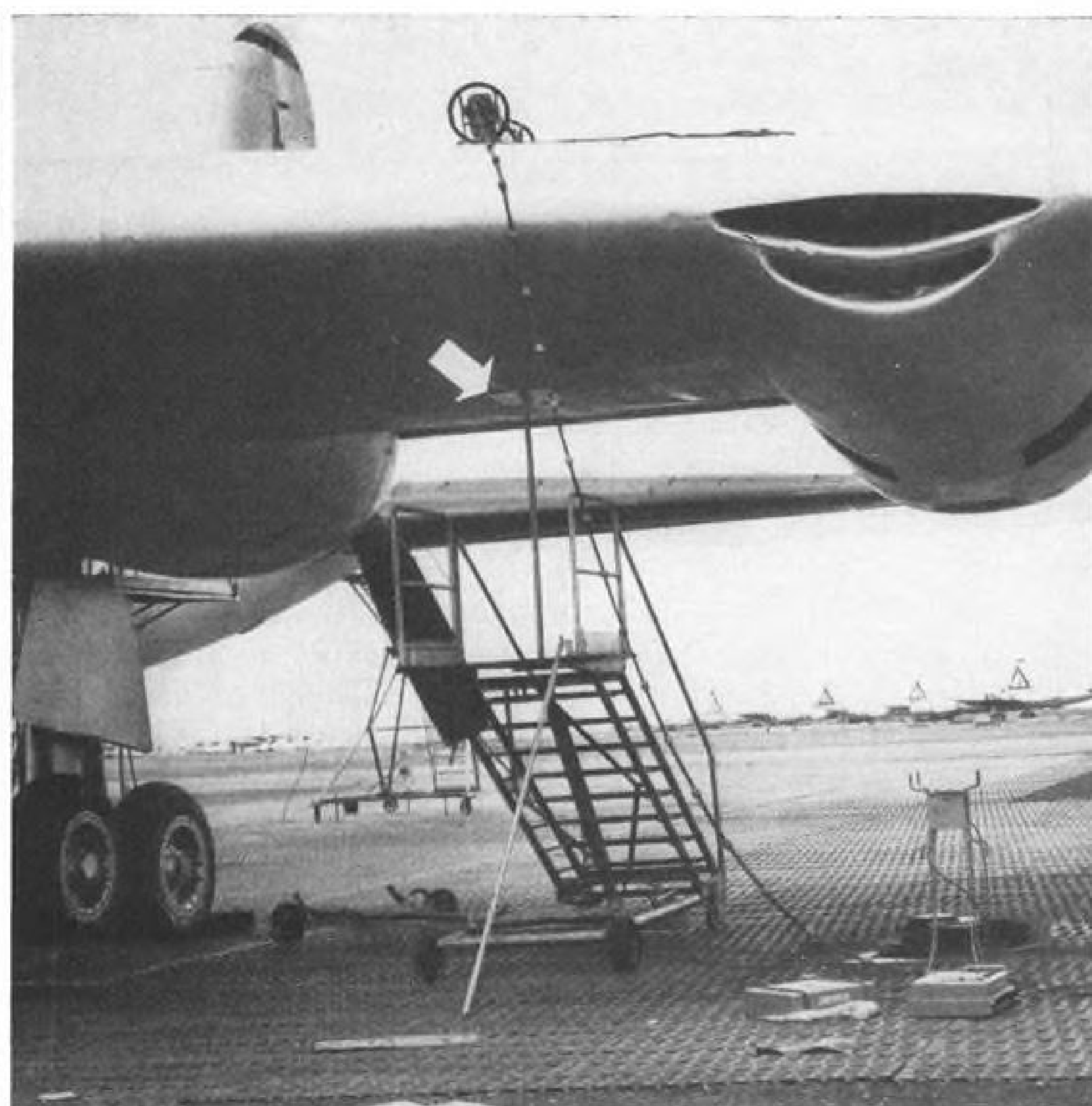
AIRC kit X-rays B-36 wing for defects. Arrow points to film under wing.
