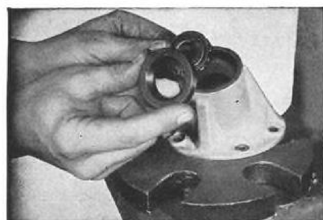
Clipper Seal being installed in the intermediate gear box of the Sikorsky HO5S helicopter to seal oil in, keep abrasives out.
