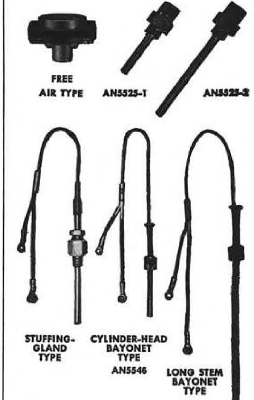
Free-air bulb is designed for flush mounting with the wing surface.
