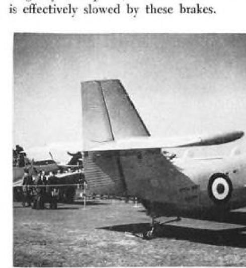
SEA MEW tail structure shows simplified design approach characterizing this "stripped-down" anti-submarine craft by Short Bros. Tailplane has constant chord; corrugations of rudder eliminate internal structure.
