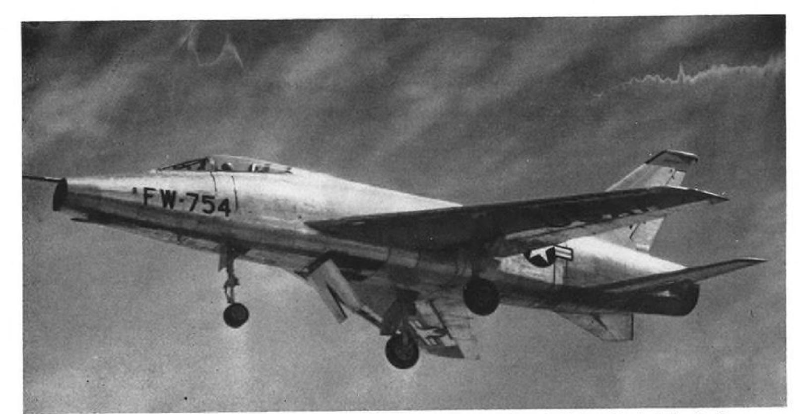
YF-100 IN FLIGHT with tricycle landing gear extended and large airbrake lowered beneath the jet fighter's belly aft of nose gear.
