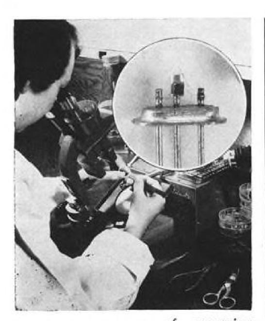
germanium 6. ASSEMBLY of germanium particle and wire "cat's whiskers" is done with tweezers under a microscope. Wire spacing (approximately 0.001 in.) has critical effect on performance.
