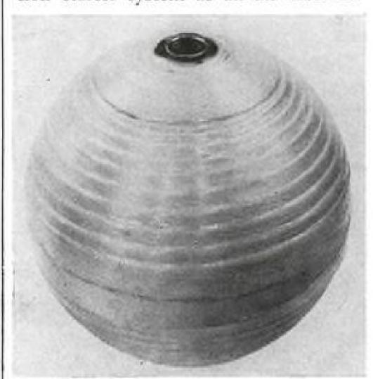
TANK is made by winding resin-impregnated glass thread around low-melting alloy.
