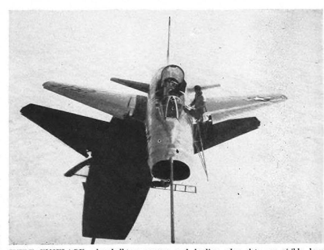
WIDE FUSELAGE, clamshell-type canopy and leading edge slats are visible here.
