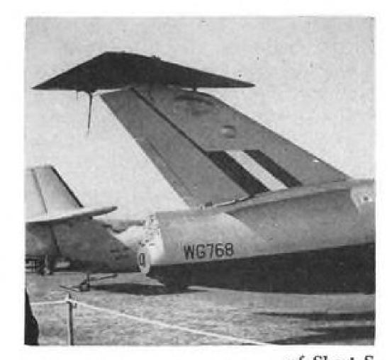
TRIANGLE TAIL of Short S. B.5 perches atop vertical surface for Farnborough flights, will be lowered below fuselage for future tests. Tail is adjustable-incidence type. Antispin and brake chutes are used.
