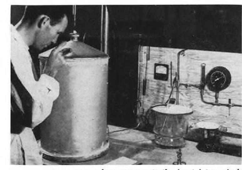
3. GROWING furnace converts the ingot into a single crystalline structure. A helium atmosphere is also maintained in this furnace to insure exclusion of undesirable impurities.
