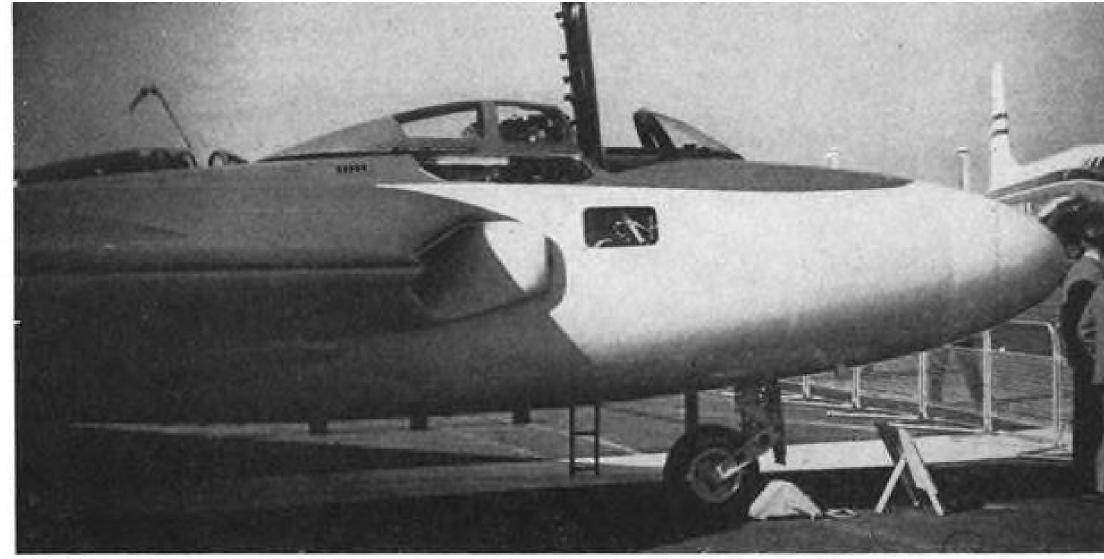
of de Havilland 110 shows difference between COCKPIT CLOSEUP pilot's position on left side of elliptical fuselage and that of radarman on right side under hatch. Nose radome and structure conceal half-ton of radar and armament. Production version will have single tail and engine.
