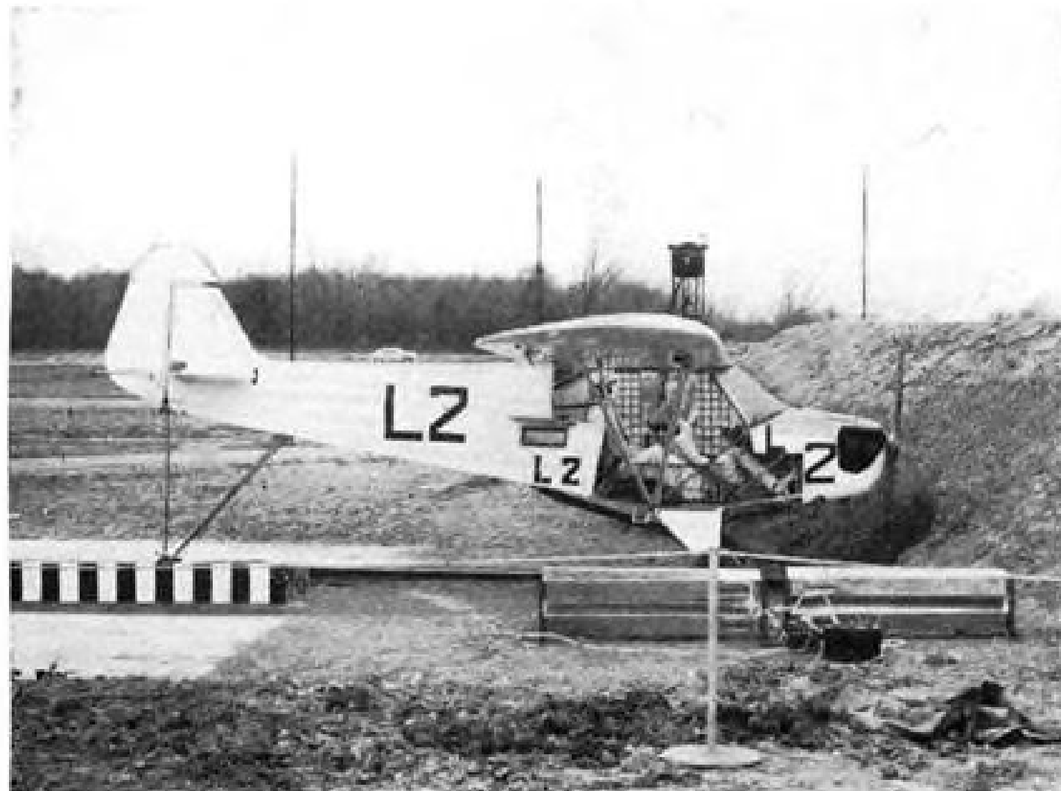
42 MPH. Impact during NACA test indicates that rear occupant would be safe if he wore shoulder harness, front occupant would suffer fatal injury unless he had harness. Carefully staged "crashes" were recorded from all angles.
