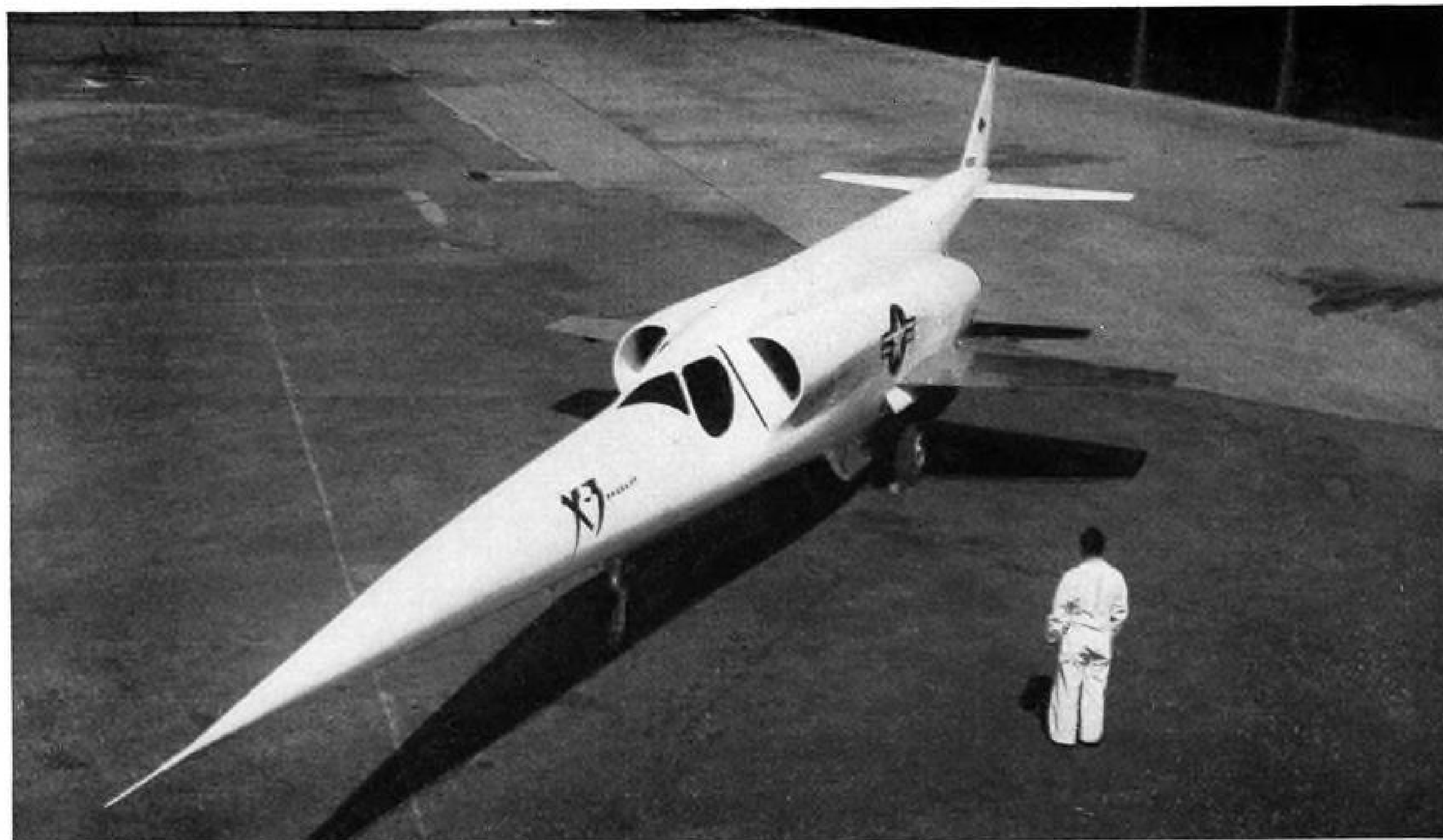
JET INTAKES for X-3's two Westinghouse J34s flank fuselage closely behind the research aircraft's triangular-shaped canopy.
