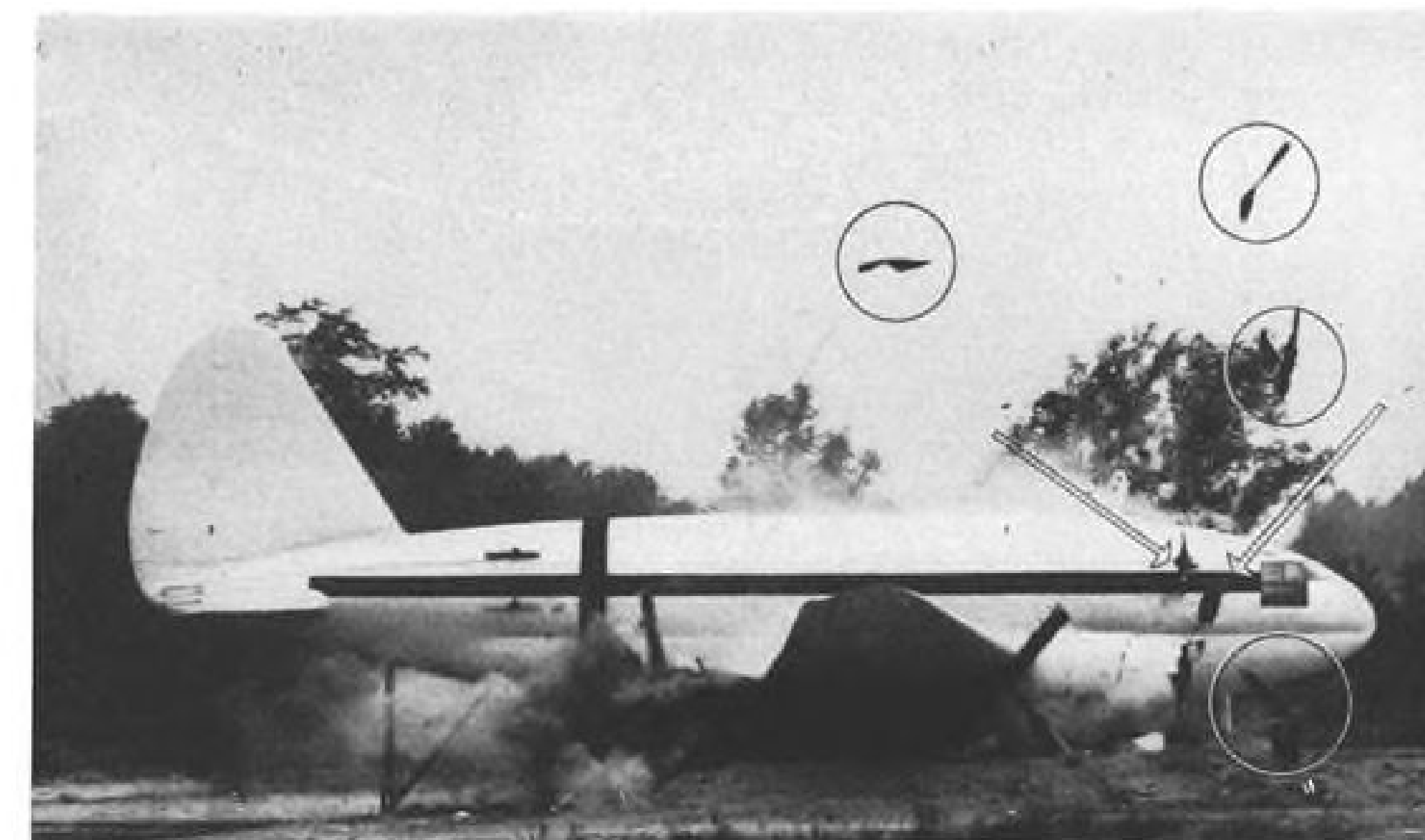
PROP BLADES of deliberately crashed Curtiss C-46 hurtle through the air (circles). Note their impact points (arrows).
