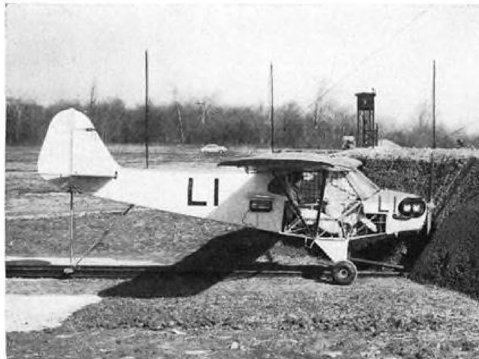
60 MPH. Impact into earth embankment, simulating severe stall-spin crash, collapses nose of Piper Cub test plane into front occupant. However, rear occupant would stand a good chance of survival if he wore sufficiently strong shoulder harness.
