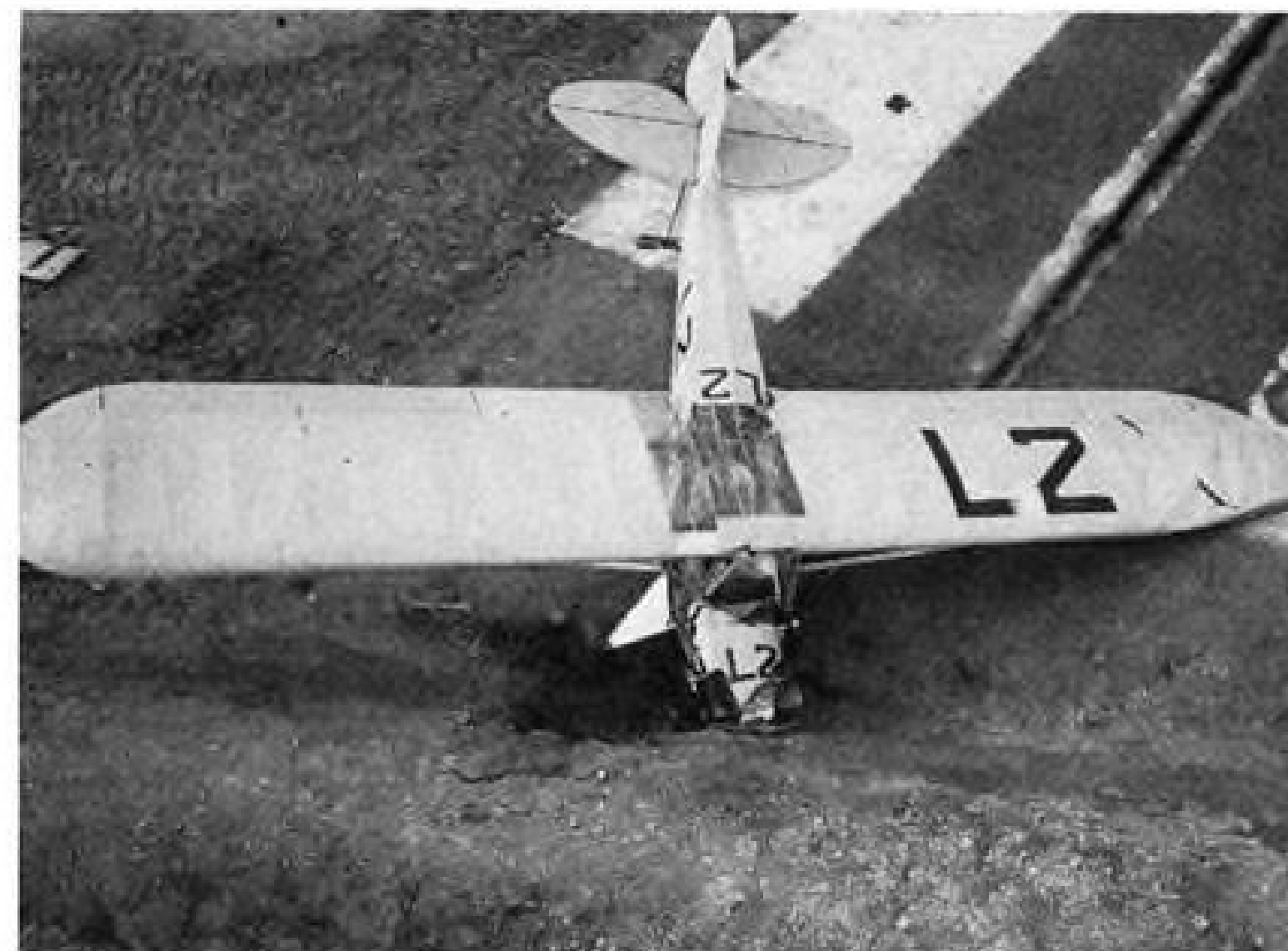
42 MPH. Impact during NACA test indicates that rear occupant would be safe if he wore shoulder harness, front occupant would suffer fatal injury unless he had harness. Carefully staged "crashes" were recorded from all angles.
