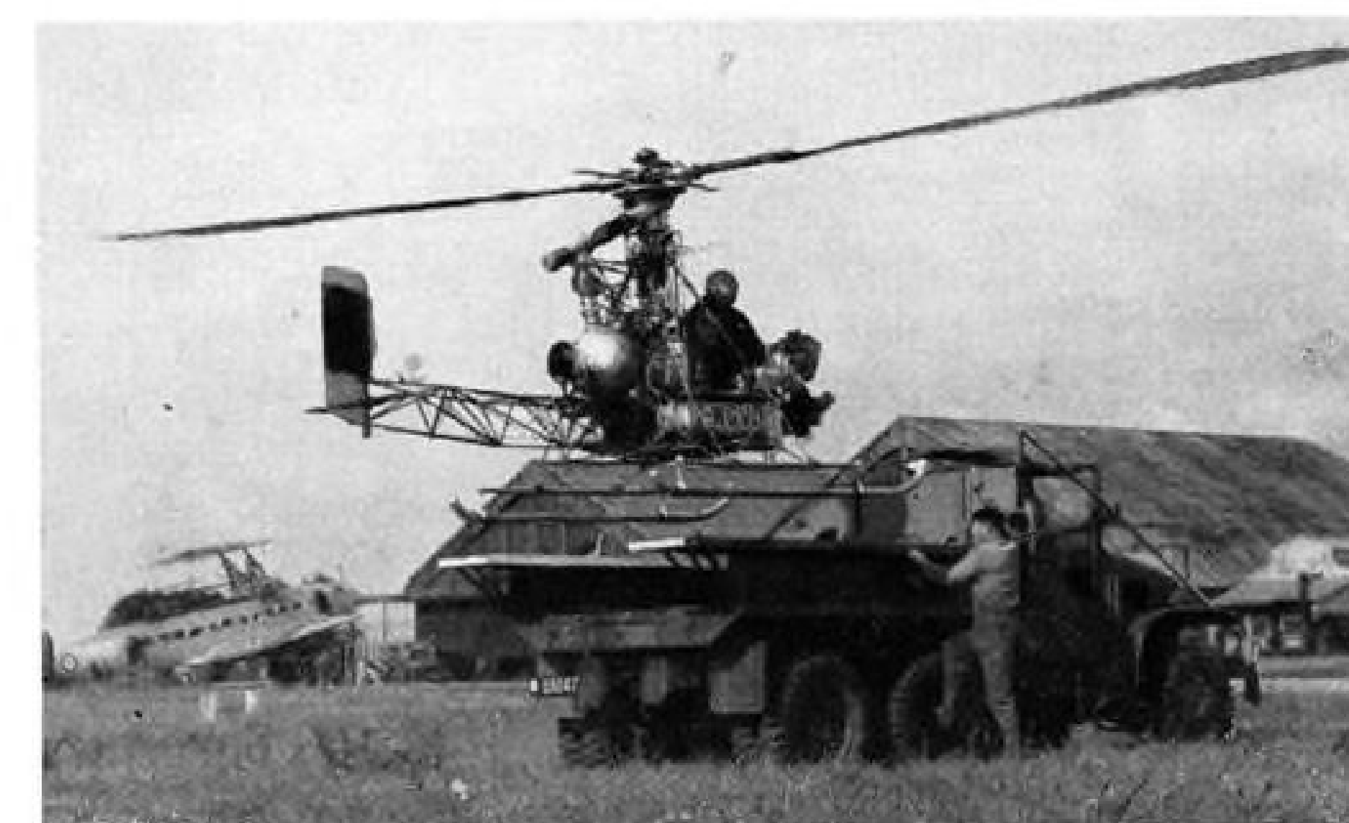
LANDING is nearly completed. Note Turbomeca jet unit behind pilot and angled tubing that feeds compressor gases to rotor head.
