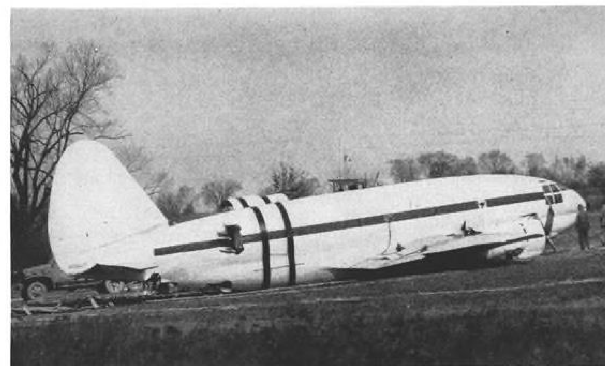
CABIN FLOOR of C-46 suffered "insignificant damage" because fuselage structure and engine nacelles afforded protection.
