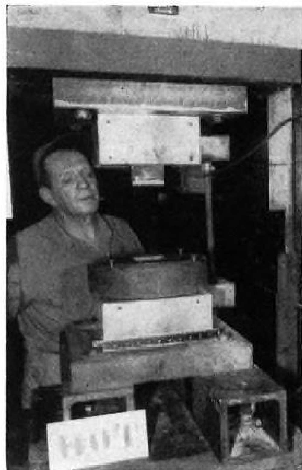
RESEARCH laboratory's 300-ton hydraulic press with forging dies installed.
