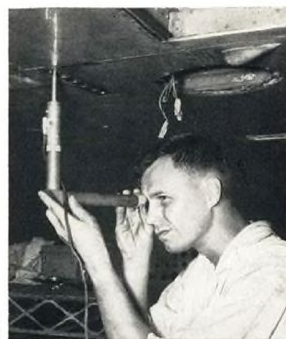
BOROSCOPE is used to examine wing spar splice bolt hole for corrosion.
