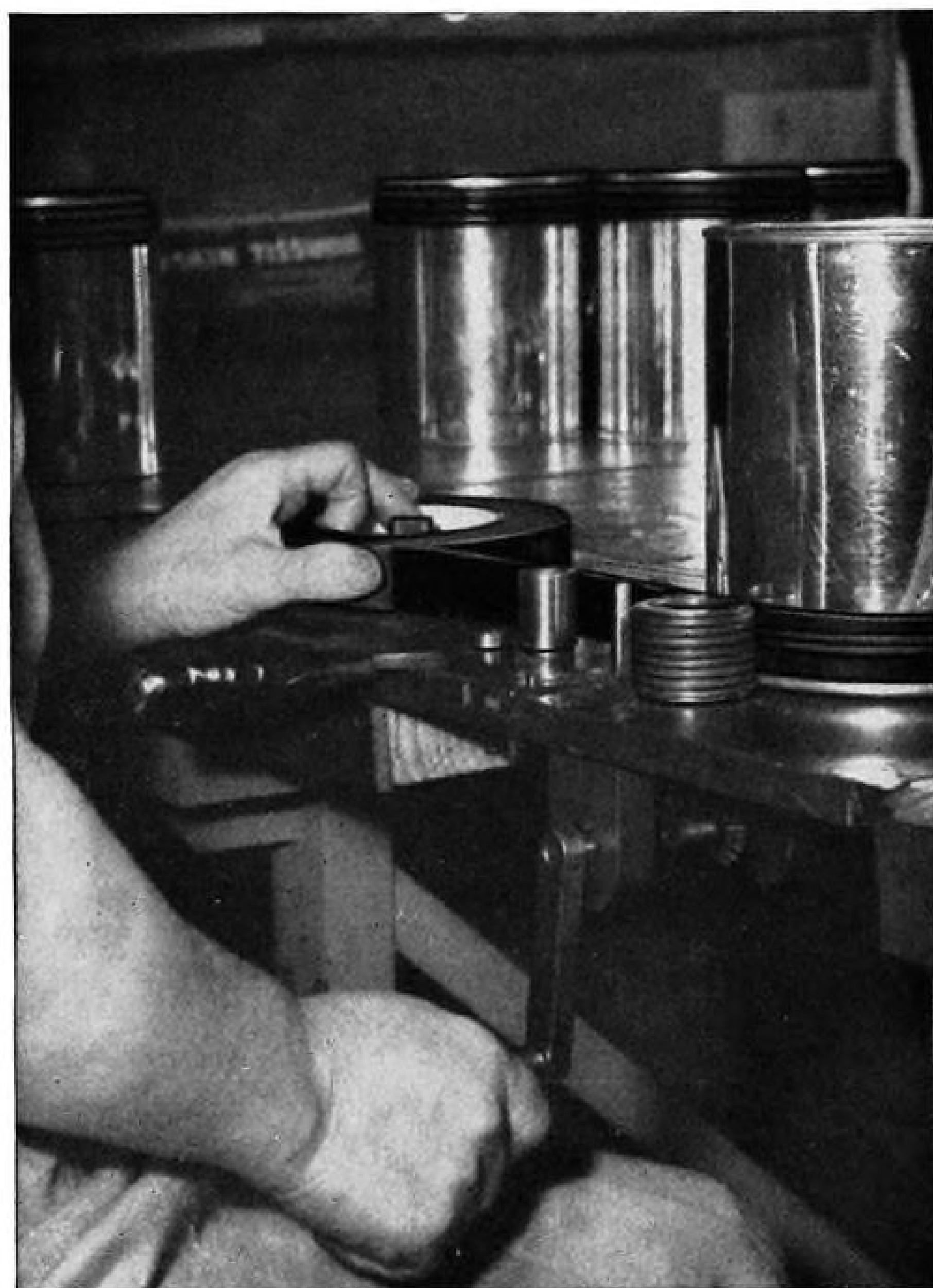
Polyken Tape No. 214 seals the lids on "canned" aircraft parts at these taping tables. Even the largest cans are sealed in approximately eight seconds.
