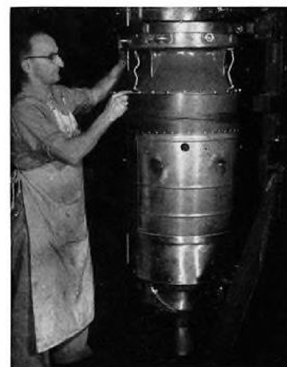
6 Compressor housing covers impeller and attaches to studs on diffuser flange.
