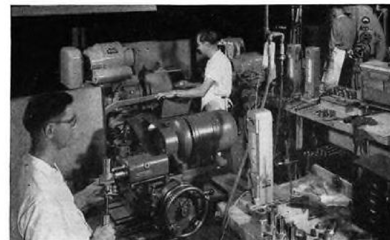
Precision grinding (shown above) on these stainless steel parts is checked to within 0.0001-inch accuracy. Grinders are able to hold 0.0002-inch concentricity between diameters.
