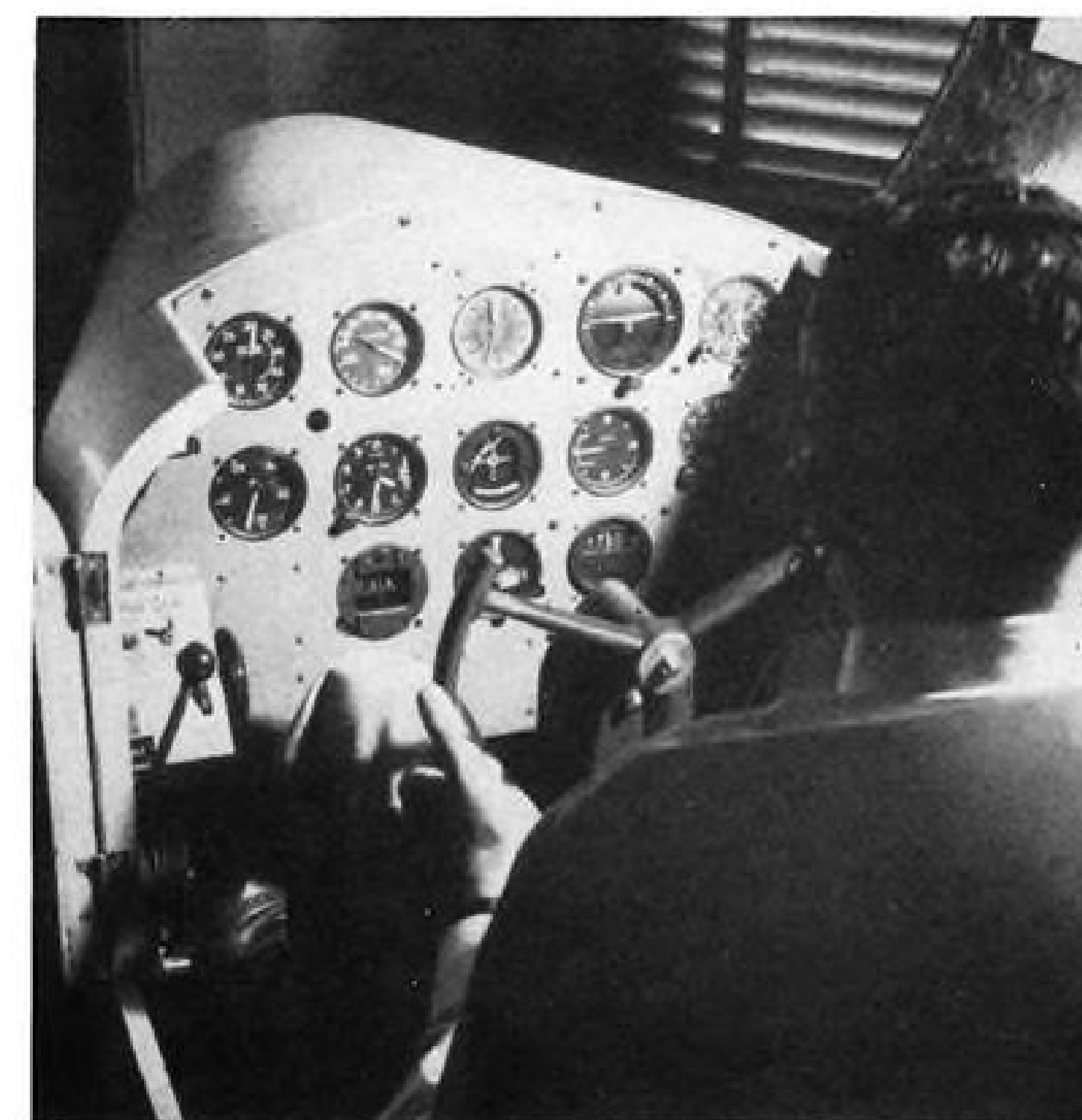
LINK cockpit, where trainee is called upon to fly ranges and practice approaches and holding procedures. Dehmel records actions.
