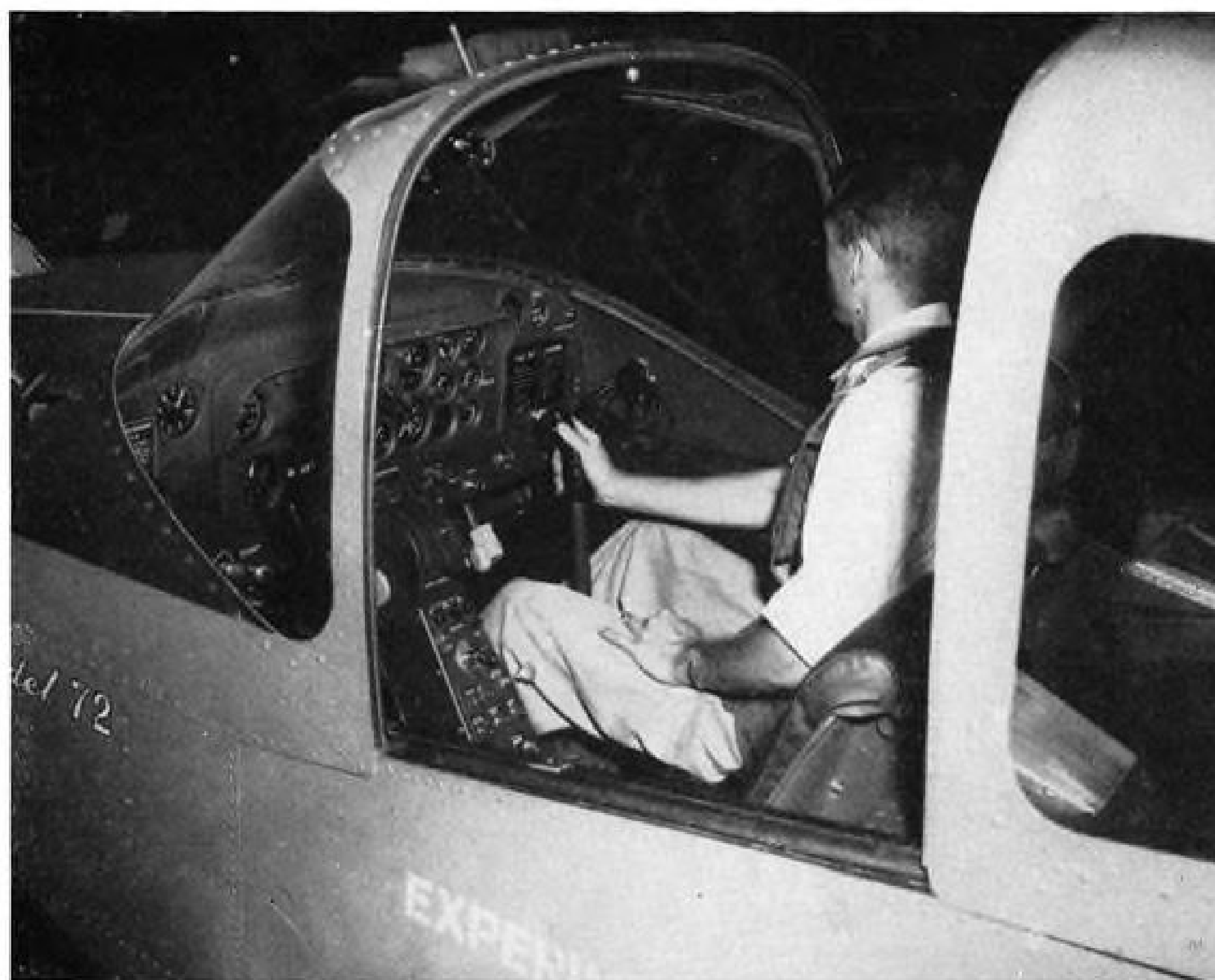
SIDE-BY-SIDE SEATING of instructor and pupil in the Model 72, Ryan Aeronautical Co.'s entry in Navy primary trainer competition, could start U.S. trend.
