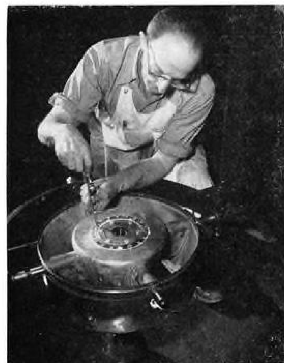
1 Exhaust section is first major component in the jig. Bearing retainer is secured.
