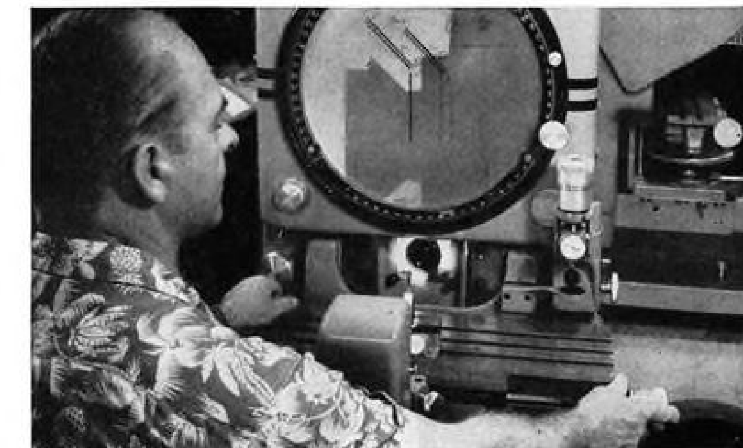
Inspections prove quality. Every accessory is 100% tested and inspected. Here's an optical comparator in use. We maintain close customer liaison to correlate test methods and results.
