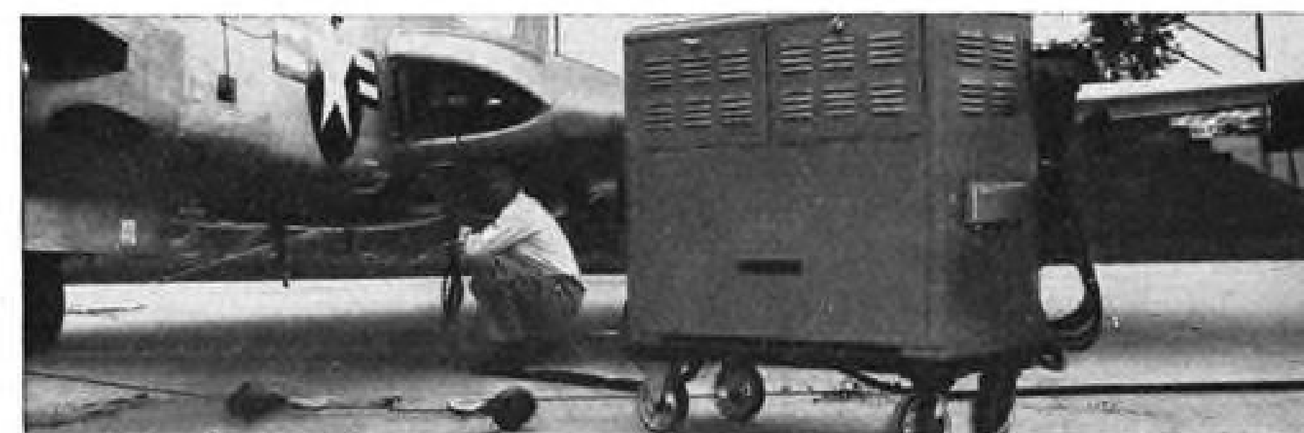
Navy type NC-5 Energizer manufactured by O. E. Szekely and Assoc., Inc. Phila., Pa., and equipped with G-E AC and DC generators and control (below)
