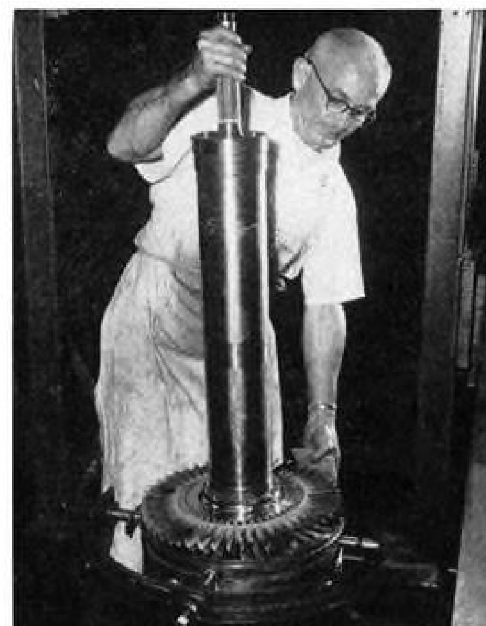
2 Turbine wheel with large diameter shaft fits into rear bearing with stub shaft.
