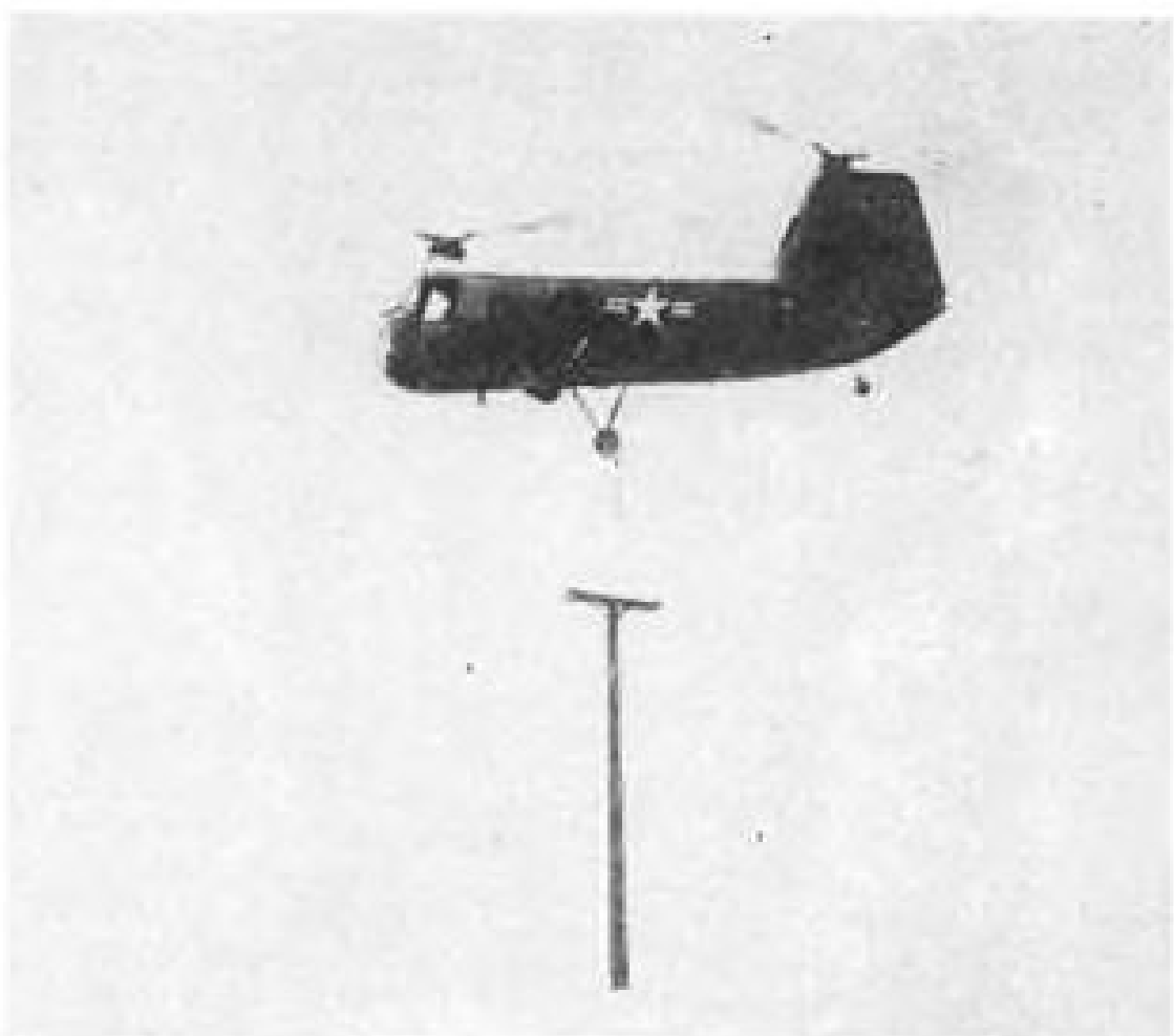
1 Phone pole slung vertically beneath Piasecki H-25A can be dropped easily into prepared holes dug previously by airlifted linesmen.
