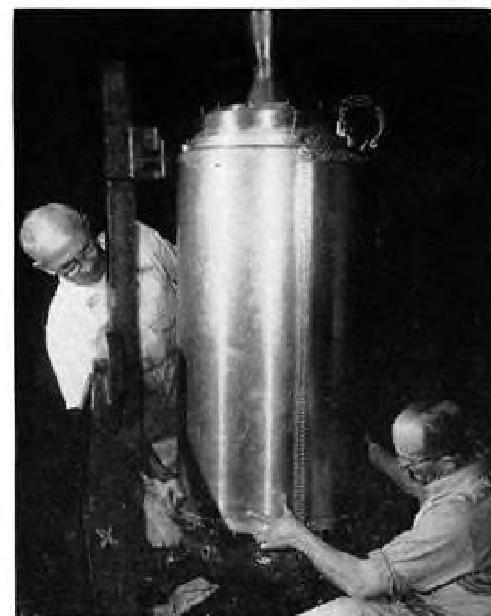
7 Monocoque shell slips over engine body after assembly has been inverted.
