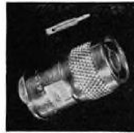
AI-11072, Army-Navy type UG-21D/U, improved type N plug for use with RG-8, 9, 9A, 10/U cables. Weatherproof. Teflon insert. Neoprene mating seal gasket, silicon rubber cable clamp gasket.
