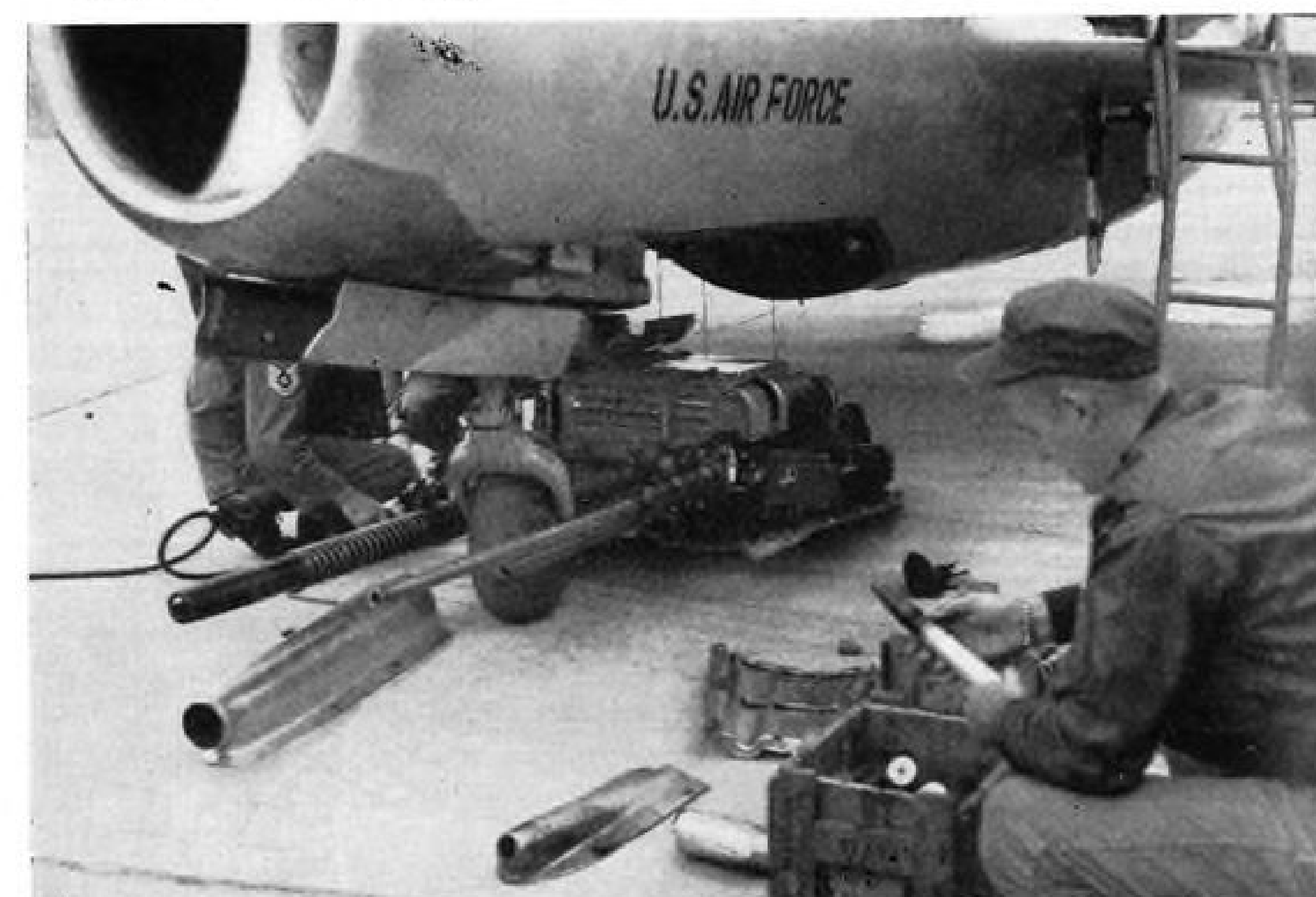
MIG ARMAMENT pack lowers from fuselage on four cables for access. Fairings on ground cover exposed barrels. Larger cannon (37-mm.) mounts recoil spring and blast tube externally. Panel under nose probably is steel, protects against gunblast.
