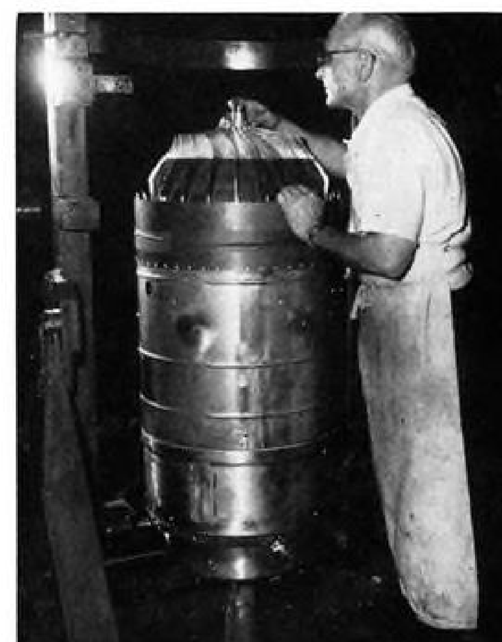
5 Impeller fits over extension shaft also used to drive gearing for accessories.
