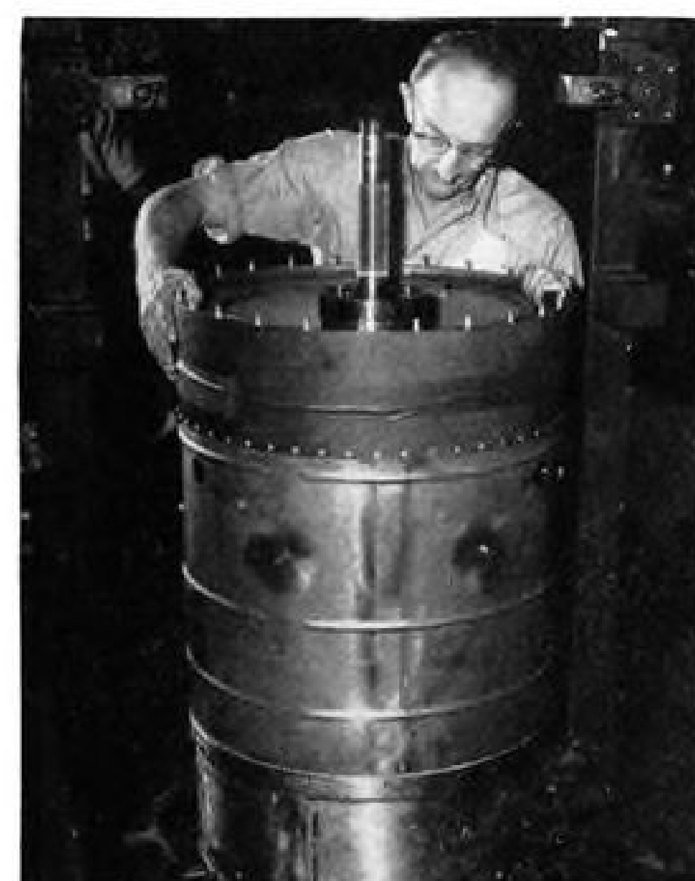
4 Diffuser with combustion chamber outer housing riveted to it is installed.
