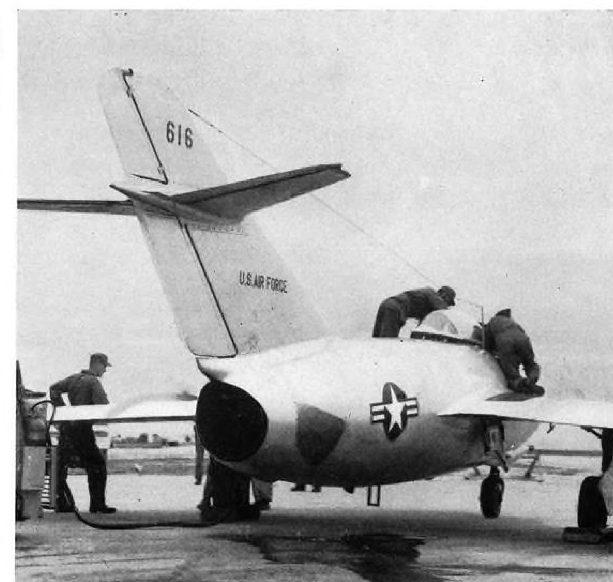
MIG TAIL has large blister at juncture of horizontal and vertical surfaces to prevent flow breakaway. Elevator has external skin doubler near outboard hinge. Top rudder hinges are external; lower are hidden. Dark patch is speed brake.
