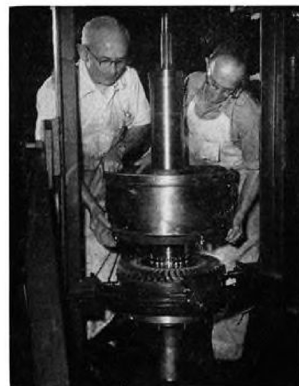
3 Turbine housing containing cast nozzle assembly is slipped over turbine shaft.
