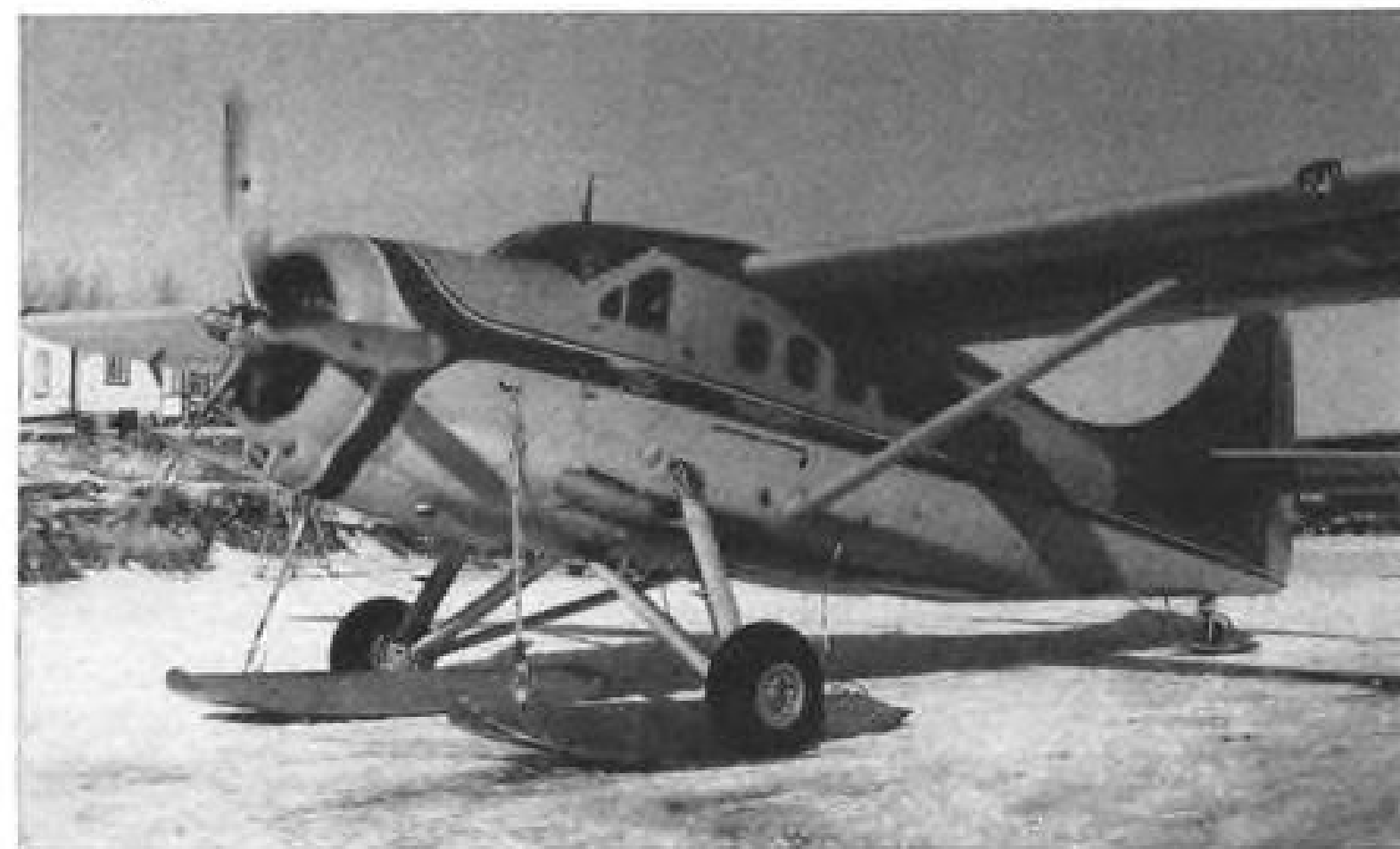
Typical Federal Wheel-Ski Installation on De Havilland Otter
