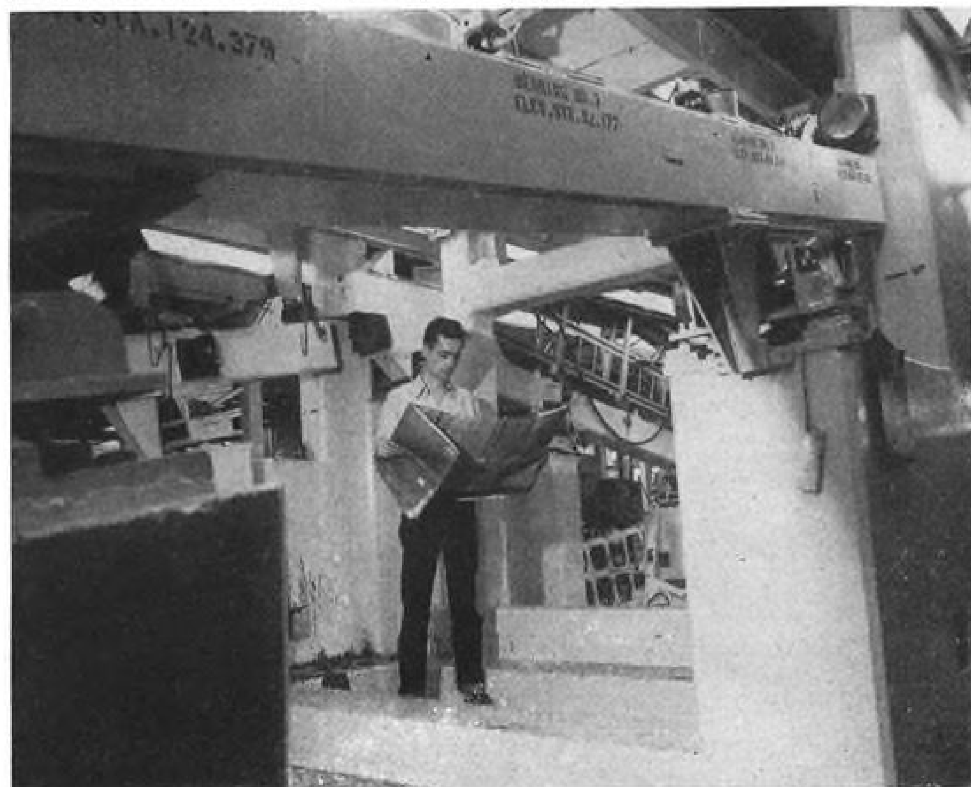
SLANTED BEAM (top) holds B-52 stabilizer during final assembly at Boeing-Seattle.
