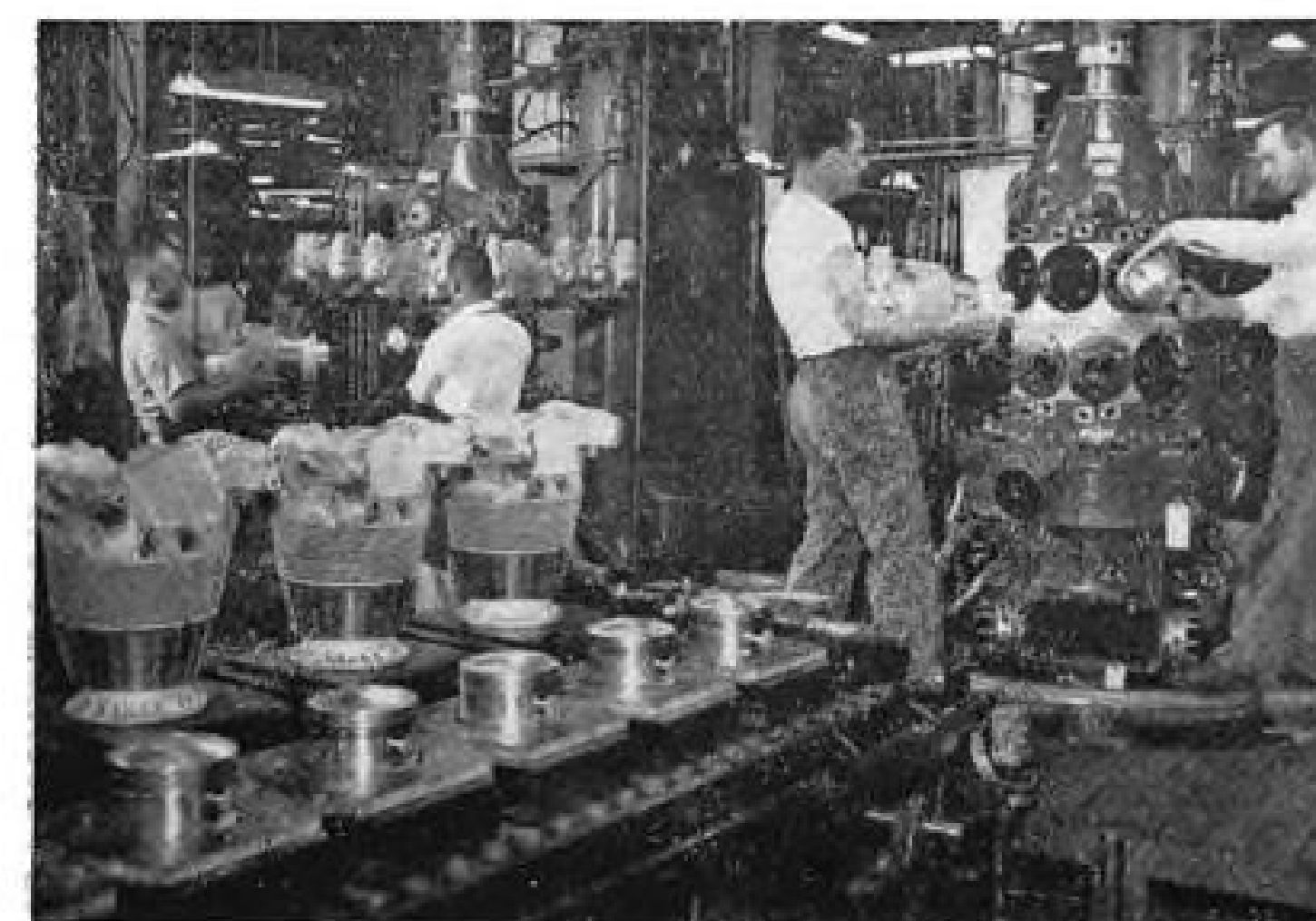
PISTONS and cylinders are installed as connecting rod is extended and cylinder mounting surface is turned to worker.
