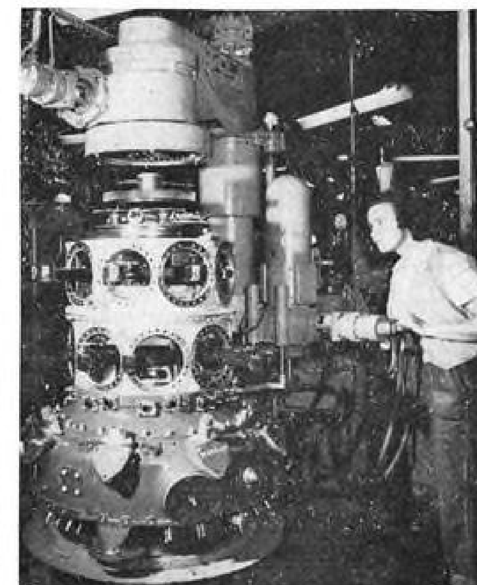
BOLT TIGHTENING, TORQUING is automatic for such operations as these on engine's front cam section (left), securing annular plate around propeller shaft extending from front section (center), locking reduction gear drive on power section (right).
