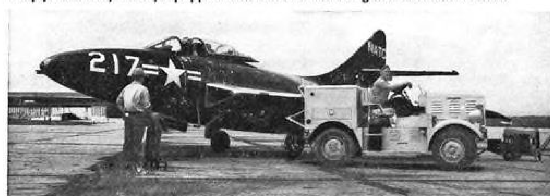
Navy Type NC-5 Energizer manufactured by the Consolidated Diesel Electric Corp., Stamford, Conn., equipped with G-E AC and DC generators and control.
