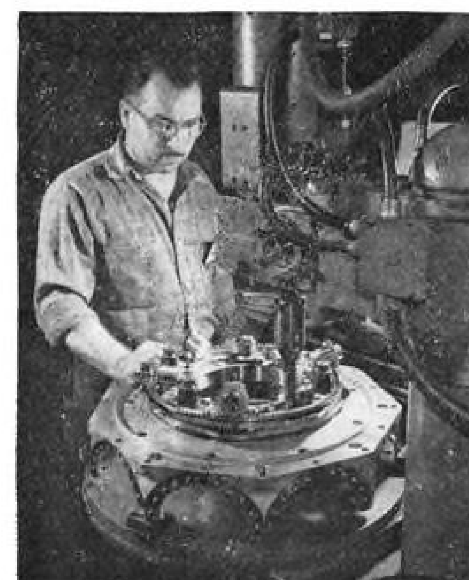
BOLT TIGHTENING, TORQUING is automatic for such operations as these on engine's front cam section (left), securing annular plate around propeller shaft extending from front section (center), locking reduction gear drive on power section (right).
