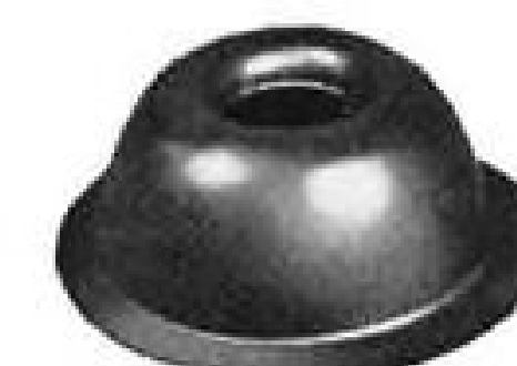
Hydroforming saved one operation
