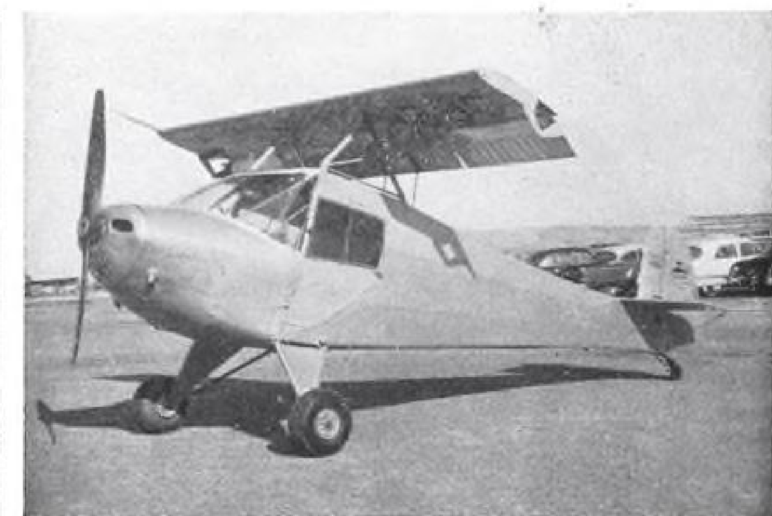
NEW WING TESTED—Rebuilt Taylorcraft embodies a 12-ft.-span wing with approximately 3-ft. chord fitted with spoilers and full-span flaps. Builder Merle Larson, Oakland, Calif., believes this will provide higher speeds in addition to other efficiencies over conventional designs. The plane is undergoing flight trials.
