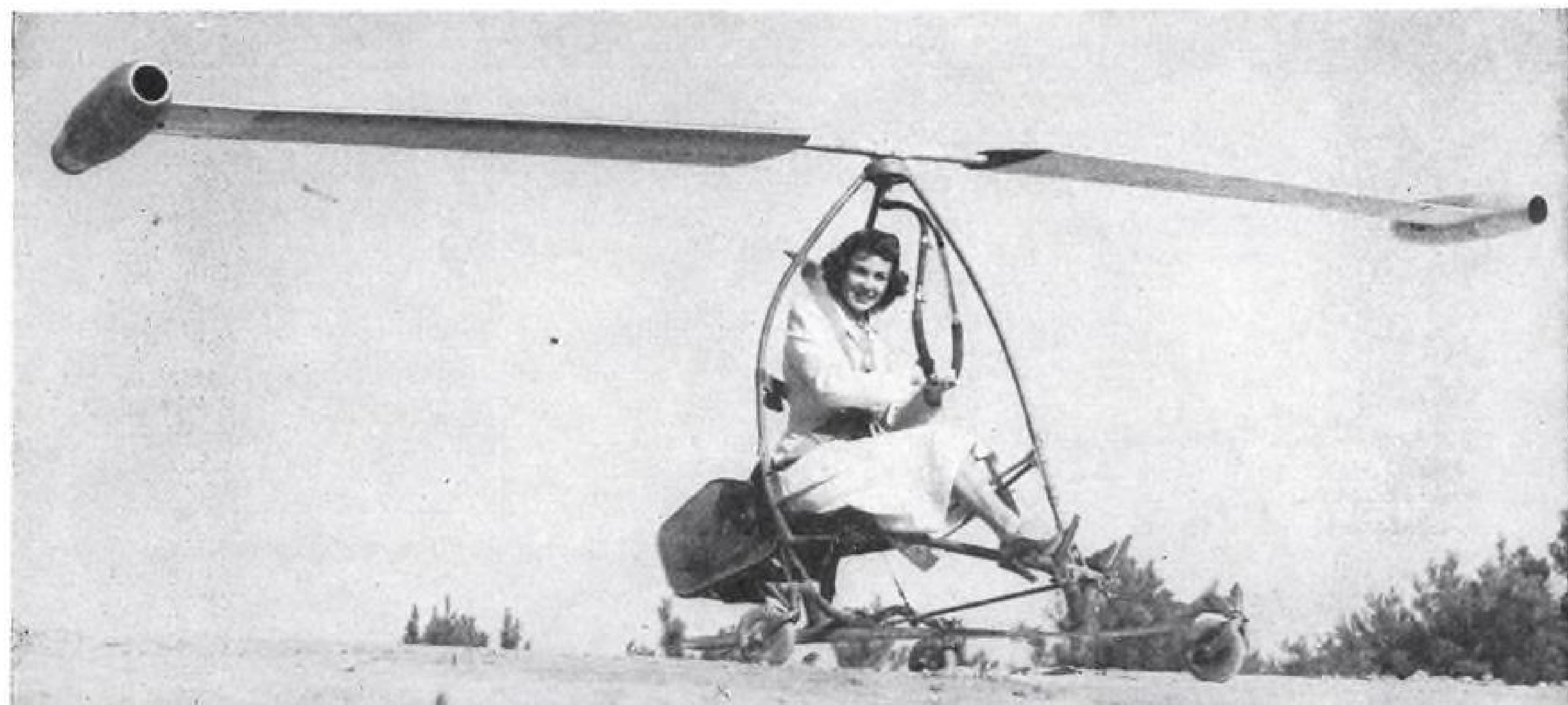
JET COPTER NEARS TESTS—First photo of 100-lb. ramjet-powered copter designed and built by Bensen Aircraft Corp., Raleigh, N. C. The Mid-Jet is designed to lift four times its own weight and attain 80 mph. Famed aerobatic pilot Betty Skelton is seen checking the Bensen Mid-Jet, which is expected to be entered in the Navy's forthcoming design competition for small helicopters.
