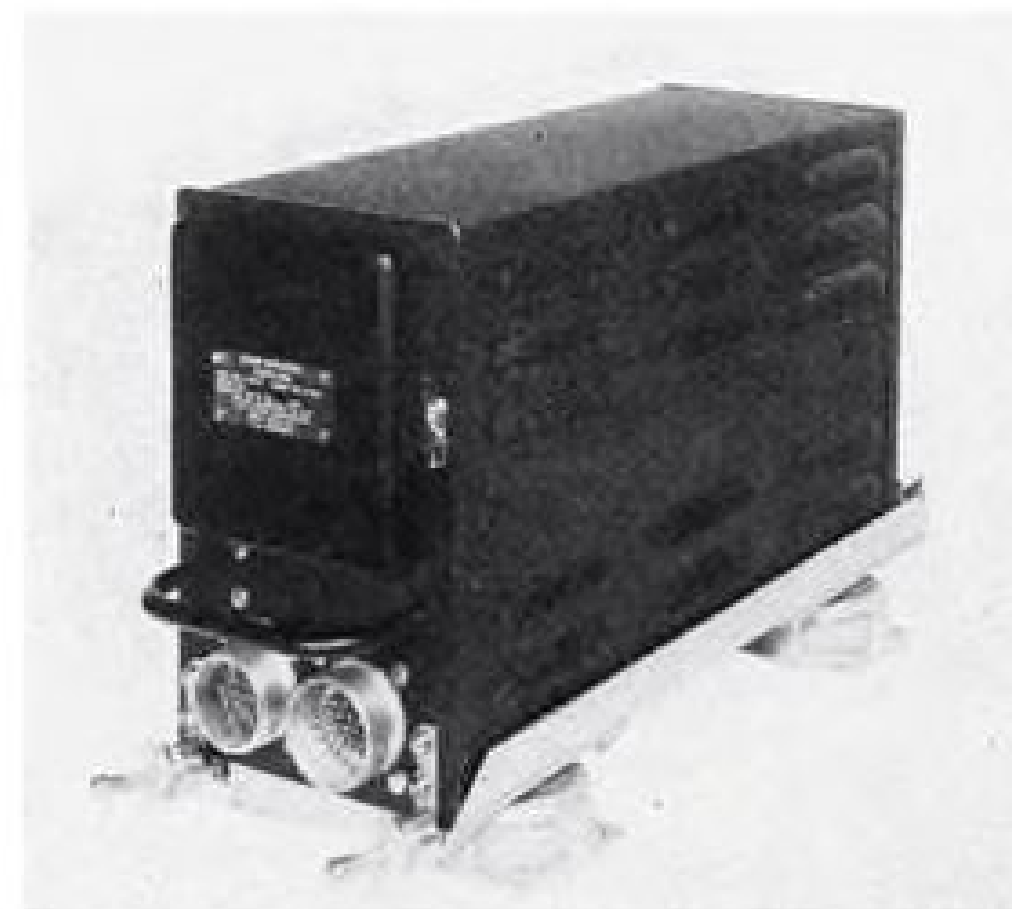
SPERRY RBC is designed to fly VOR airways as well as make improved ILS approaches, all with more automaticity than its predecessor.
