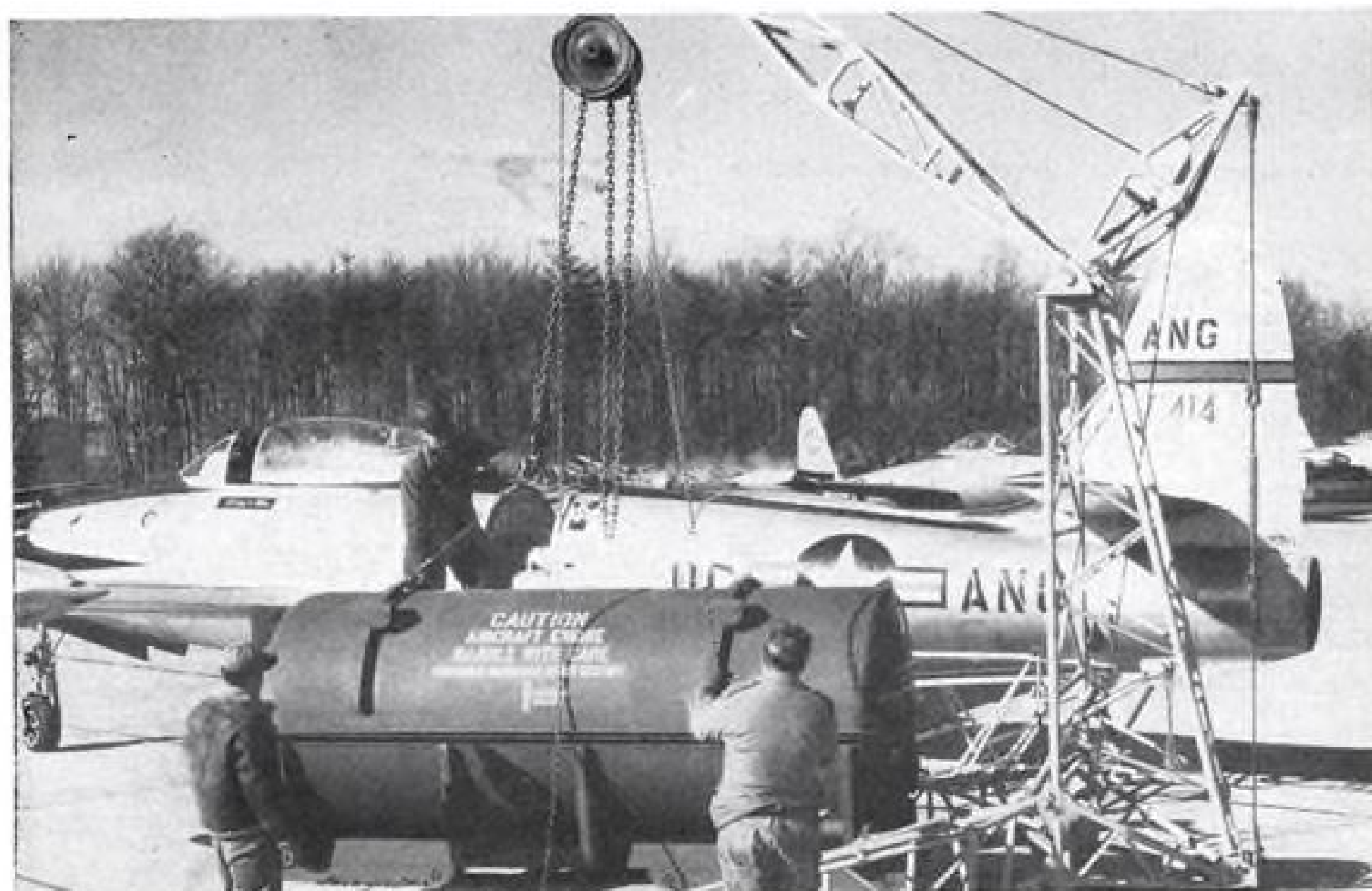
DIRECT TRANSFER of engine to aircraft in field is made from metal can. Hermetic sealing has prevented corrosion and eliminated need for special preparation or check.
