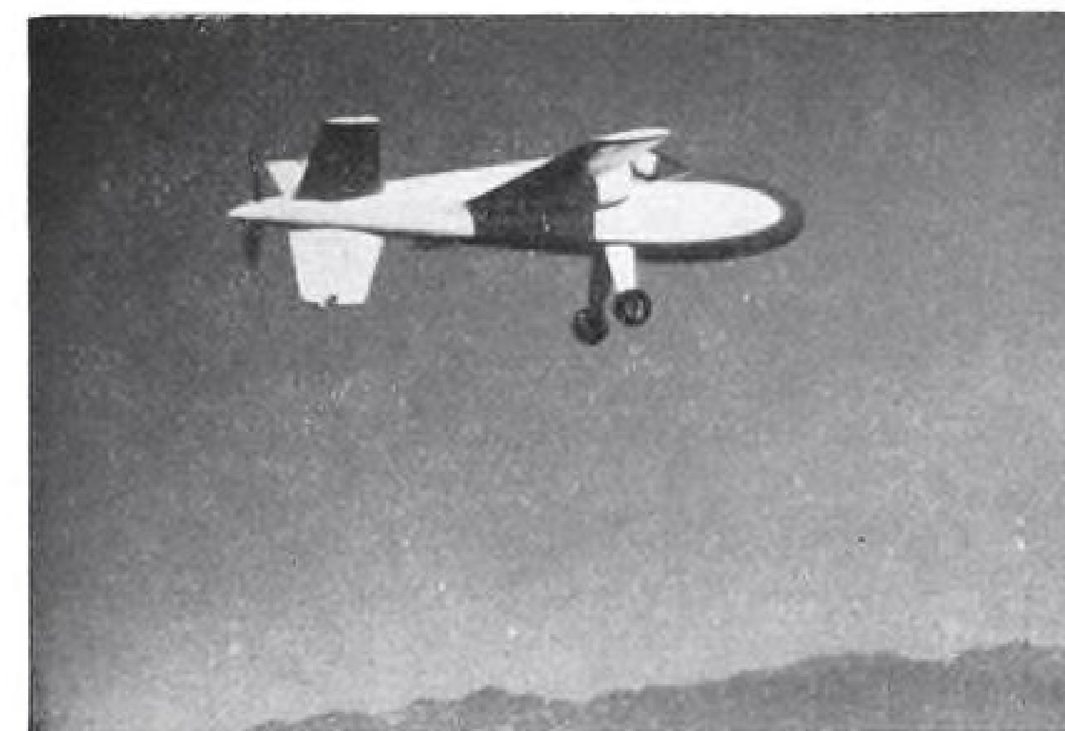
JR. MIXMASTER—Acme Aircraft Co., Torrance Municipal Airport, Calif., plans to use this single-place pusher racer built by Sierra Aviation Co., Los Angeles, as a testbed for a two-place, cross-country plane or four-place, twin-engine, high-performance pusher. Craft has 85-hp. Continental. (Also see Aviation Week Oct. 26, p. 21).
