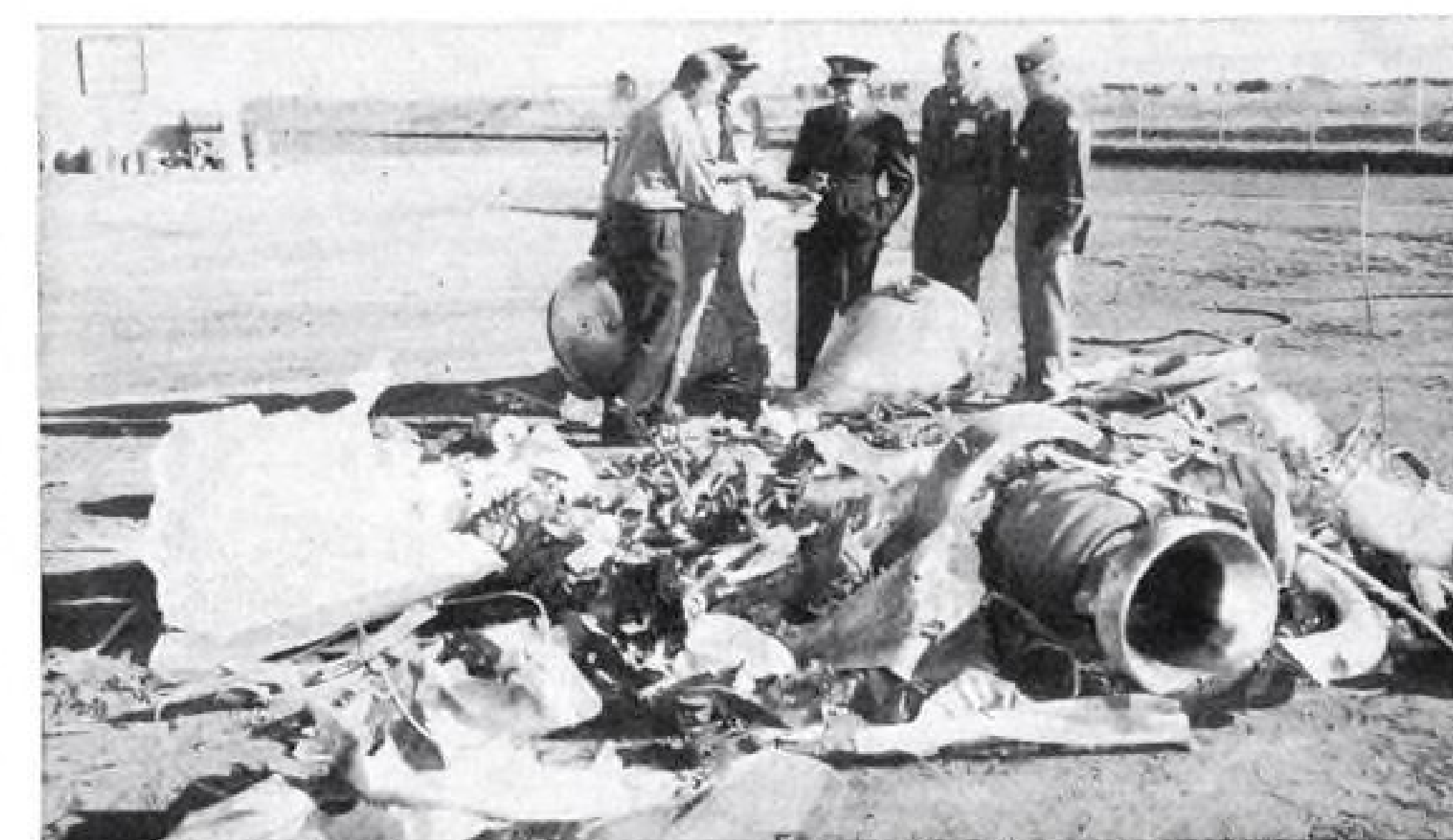
VIKING REMAINS are collected after typical test. Gimbal-mounted motor and mount are visible in right foreground. Rocket is separated on downward leg into nose section and body to increase drag by causing pieces to tumble.
