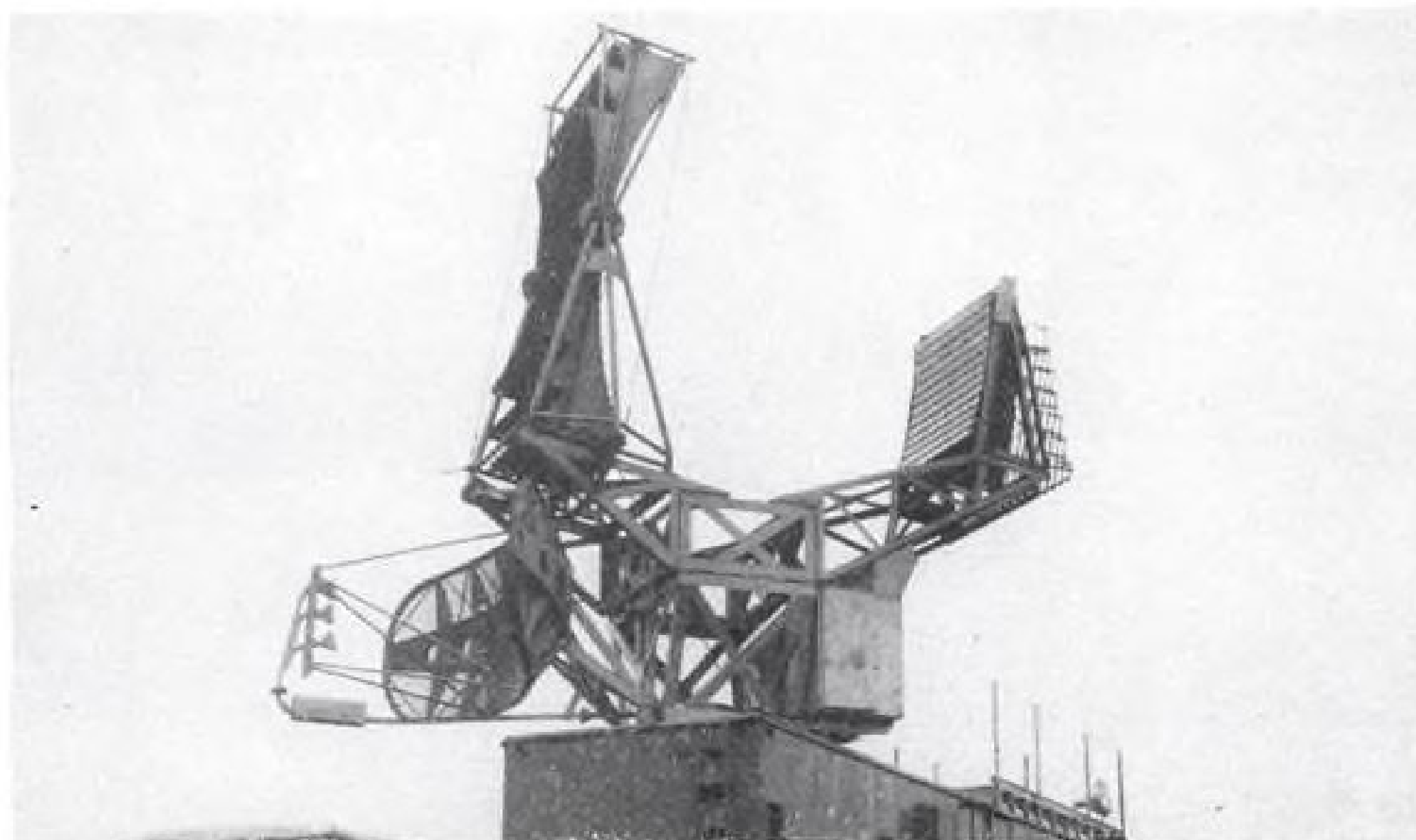
SURVEILLANCE RADAR like this experimental unit, or more-conventional existing military or civil radars, provide plane location information to Volscan computers.
