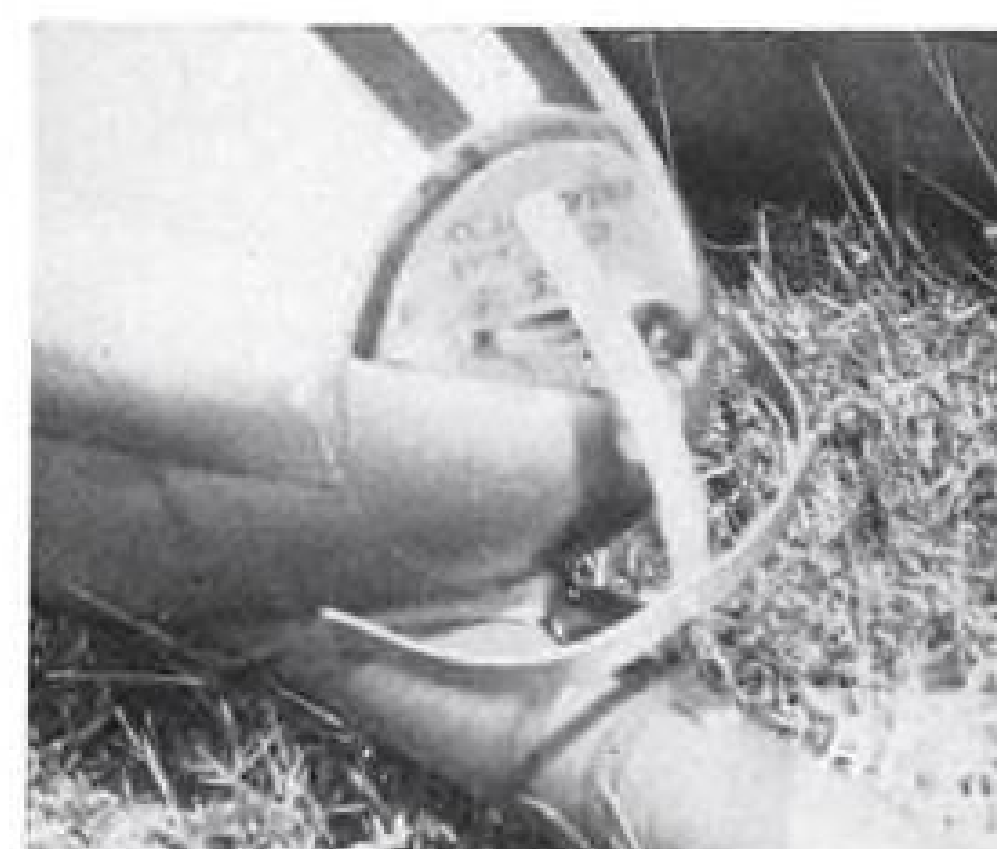
NOSE of modified tank is fitted with protective guard of crossed metal strips. Tank is standard 230-gal. receptacle.
