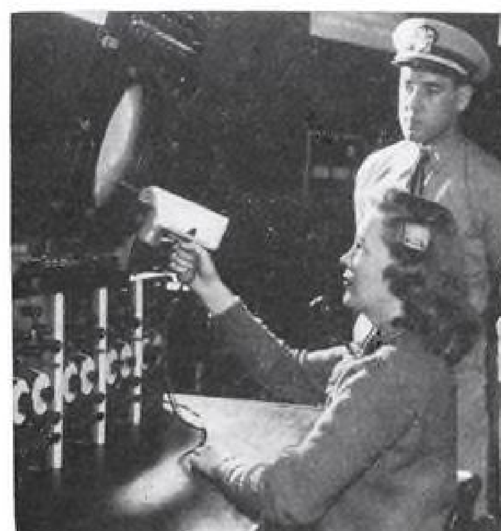
TRAFFIC CONTROLLER puts newly arrived aircraft under automatic Volscan control by placing pistol-shaped device over aircraft's blip on surveillance radar scope.
