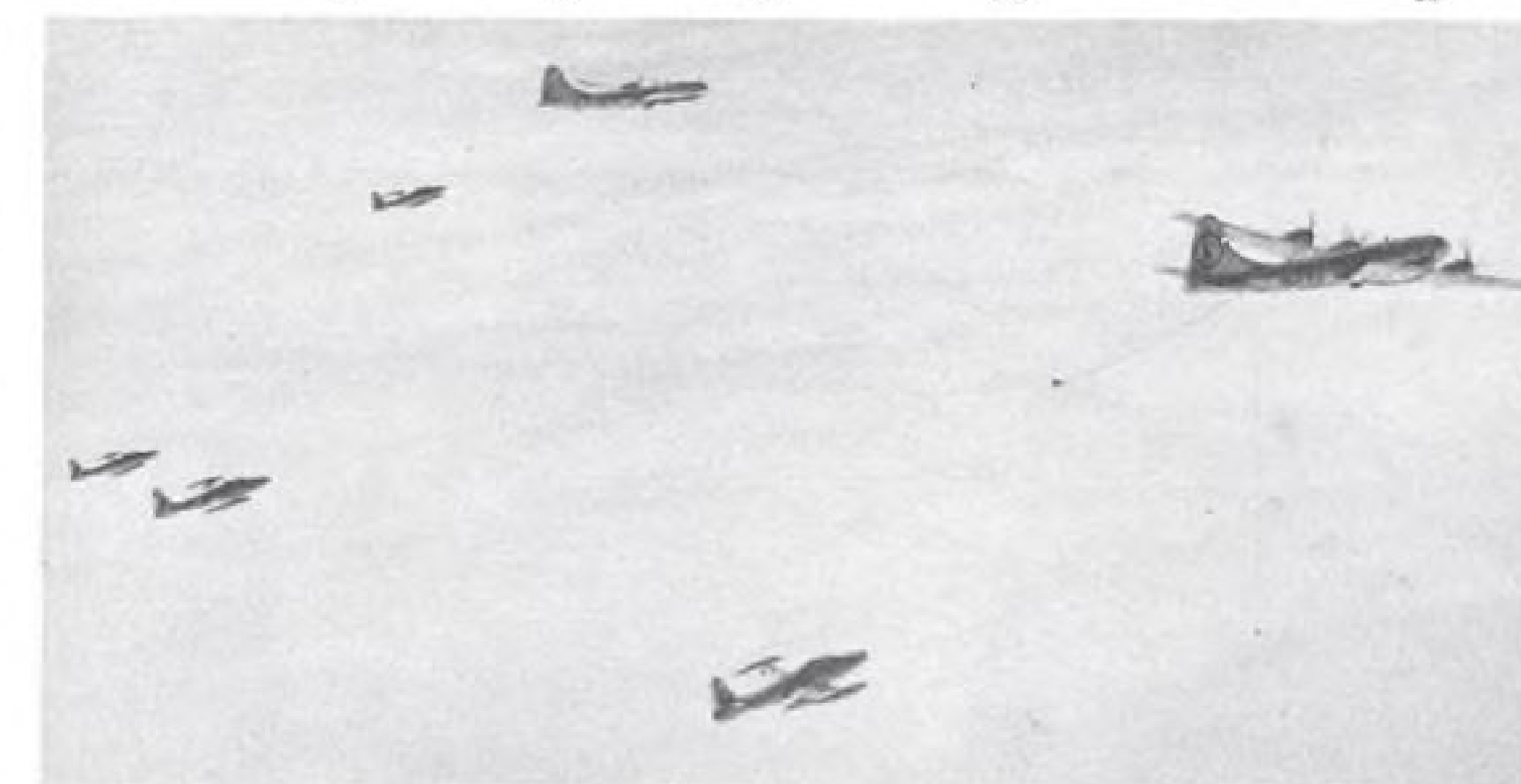
FOUR F-84GS MOVE IN to take on fuel from a pair of Boeing KB-29M Superfort tankers high over the South China Sea during course of 2,500-mi. nonstop training flight from Tokyo to Thailand. Jets are using Flight Refueling probe-and-drogue system.
