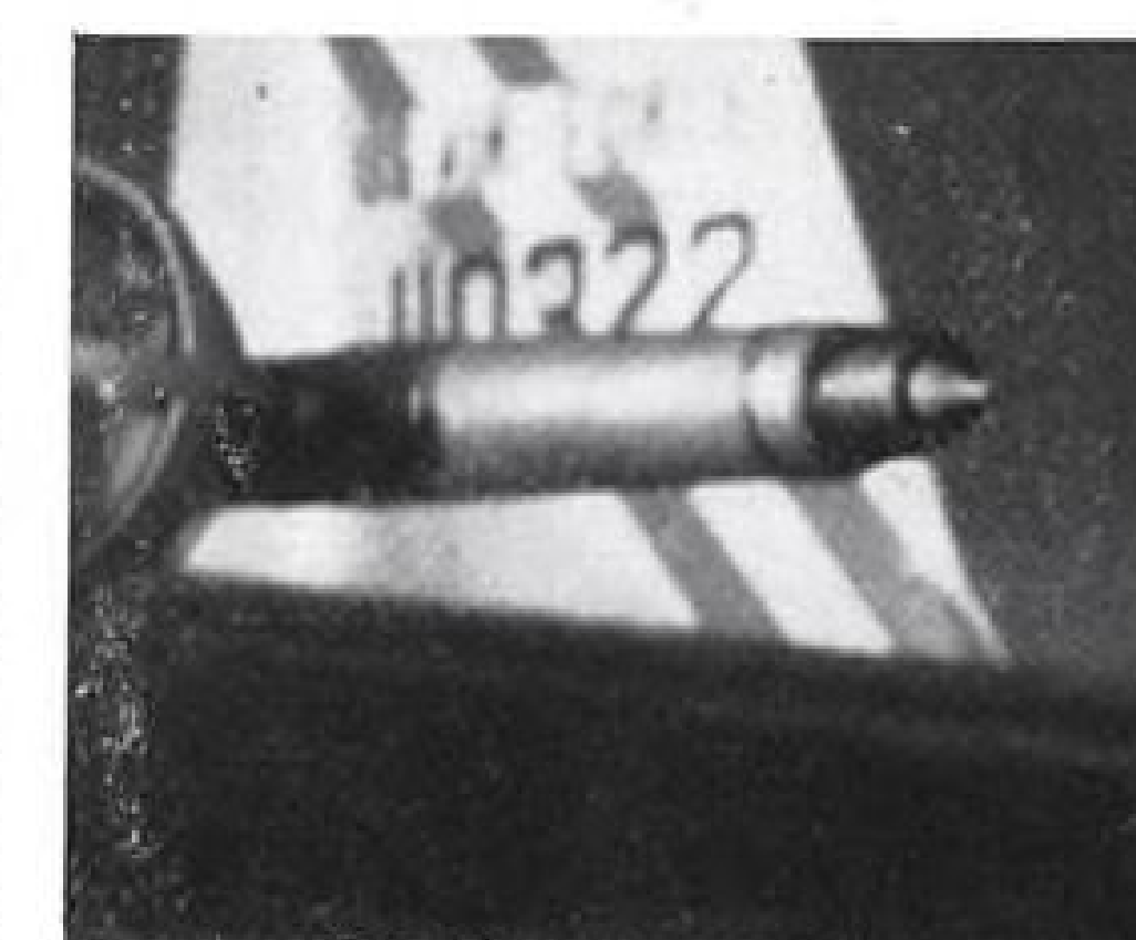
PROBE, which contacts tanker's hose, juts from inboard side of F-84G's tiptank. These are first photos of installation.
