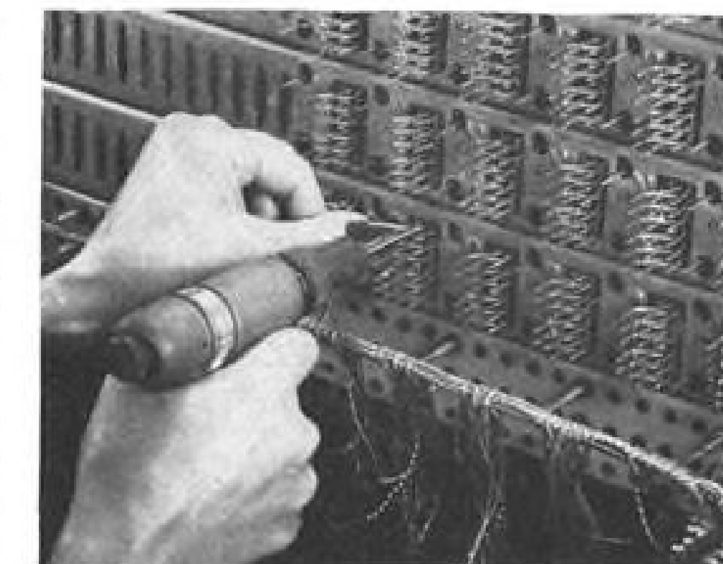
HAND TOOL is now used to make wire-wrap connections. It would be replaced by machine with multiple wrapping tools.
