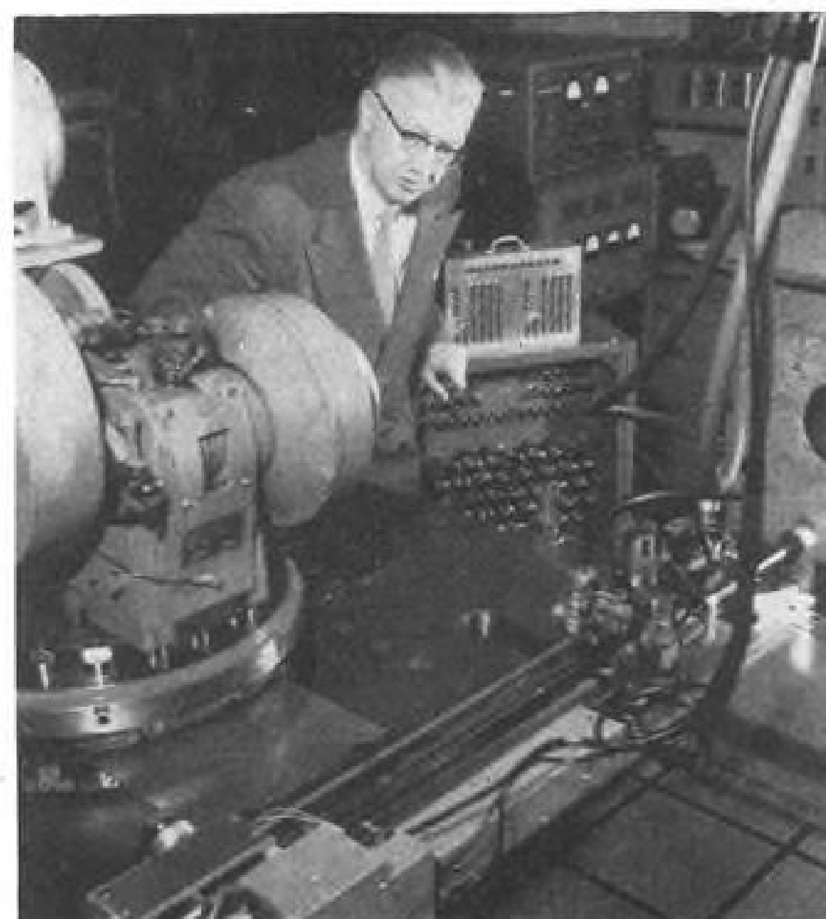
MECHANIZED PRODUCTION of electronic equipment by automatic machines is typified by punch press (left) operated from plastic punch card and digital control (right). This setup is the first step in a General Electric program for Army Signal Corps.
