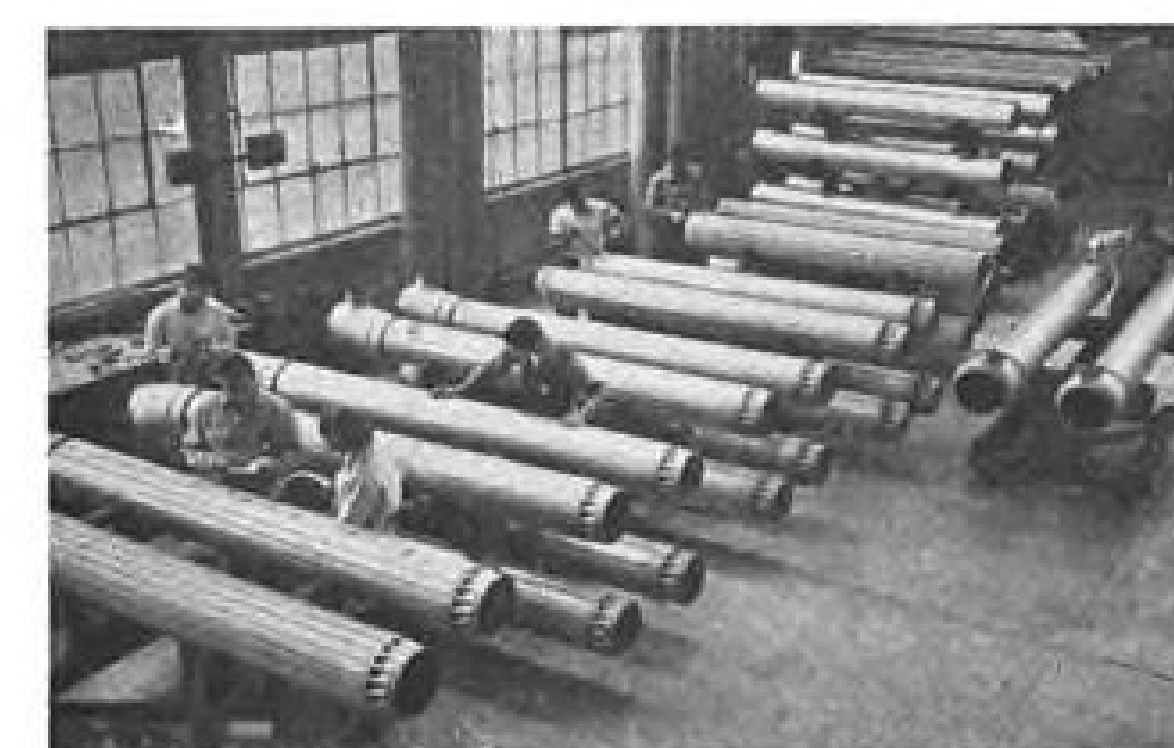
Stainless Steel augmentor tubes, also produced by Rohr Aircraft, are resistant to heat and corrosion, and carry exhaust gases from engine to rear of nacelle for additional or augmented thrust.
