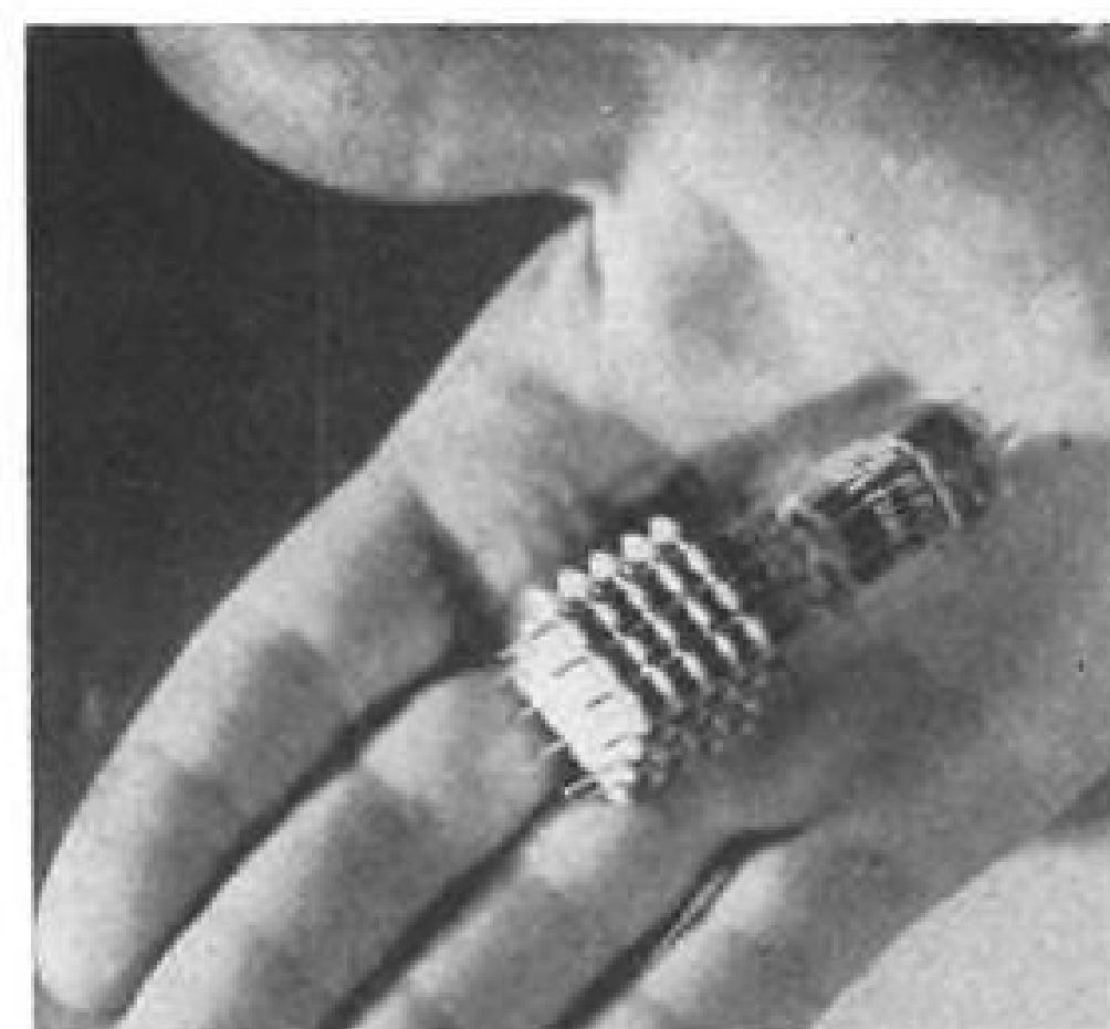
"TINKERTOY" MODULE, product of the country's first automatic factory, serves as a benchmark for comparing other automation techniques now under development.
