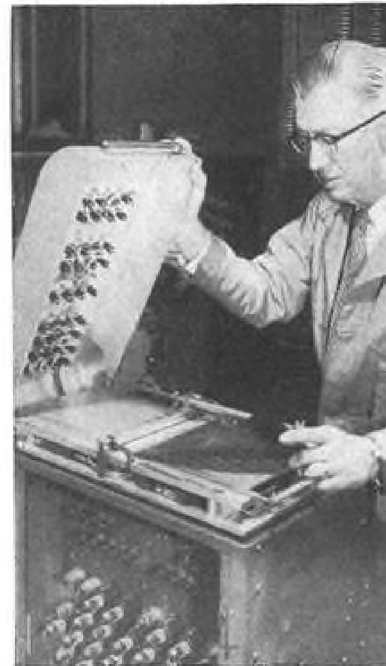
MECHANIZED PRODUCTION of electronic equipment by automatic machines is typified by punch press (left) operated from plastic punch card and digital control (right). This setup is the first step in a General Electric program for Army Signal Corps.
