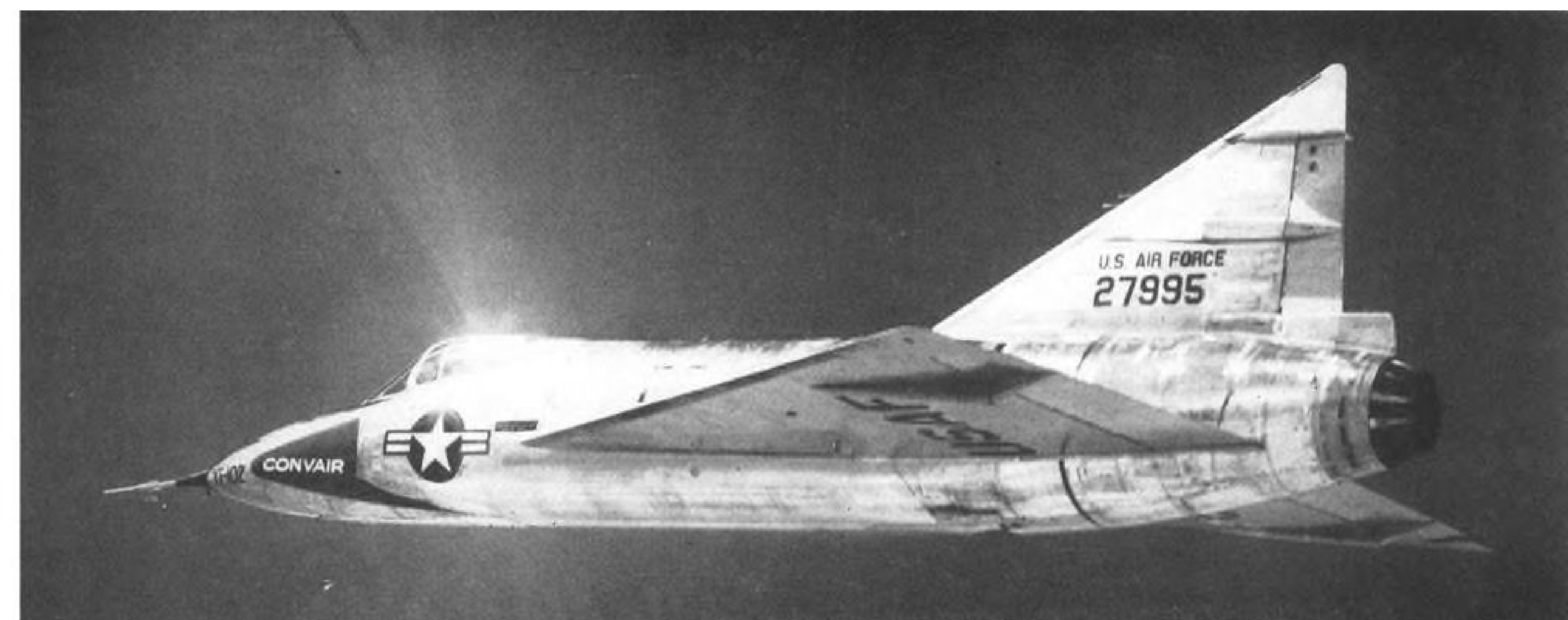
CONVAIR YF-102, supersonic all-weather USAF interceptor, reveals delta-wing configuration resembling its research predecessor, the XF-92A that the company built for the Air Force in 1948. The YF-102 is powered by a P&WA J57 engine with an afterburner.
