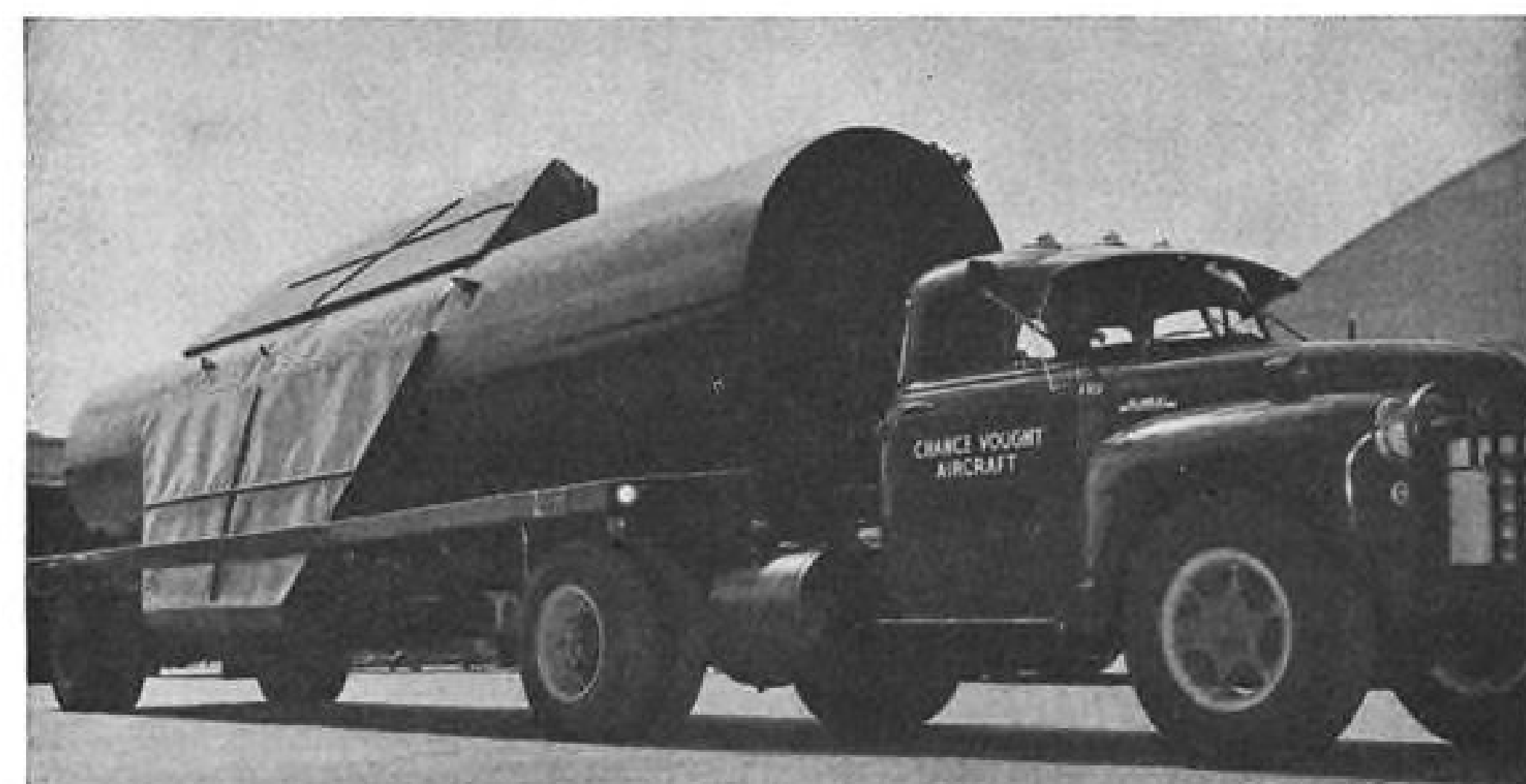
READY TO TRAVEL with container rotated to minimize width of "package." This feature speeds transportation because truck need not take special route to avoid obstacles.
