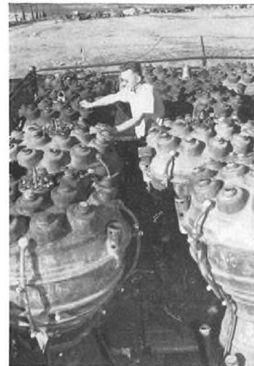
LIQUID OXYGEN and alcohol gave V-2 rocket engines 50,000-lb. thrust.
