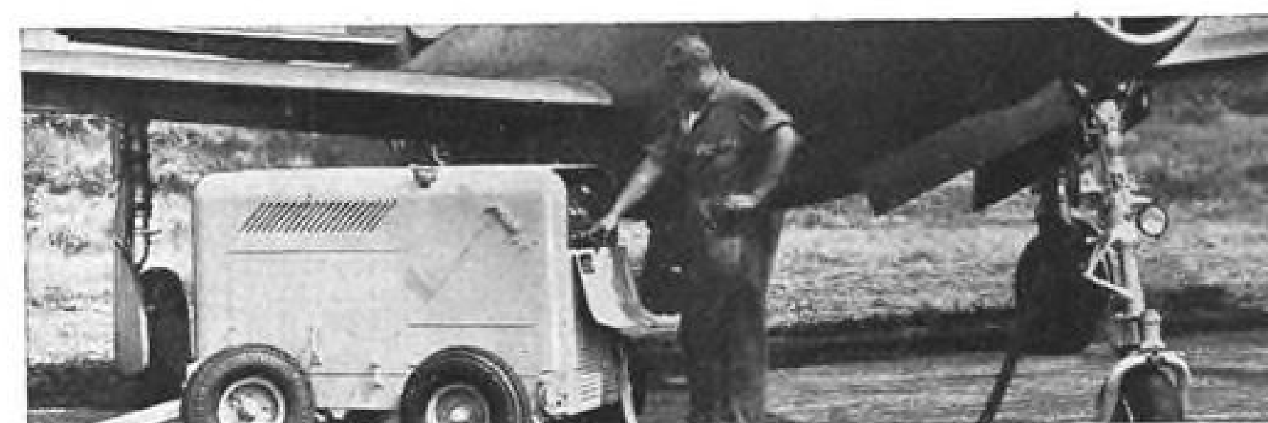
Engine Driven G-E Energizer, 28-volt, 500/1000-amp (above) G-E Frequency Changer Energizer, 400-cycle (below)
