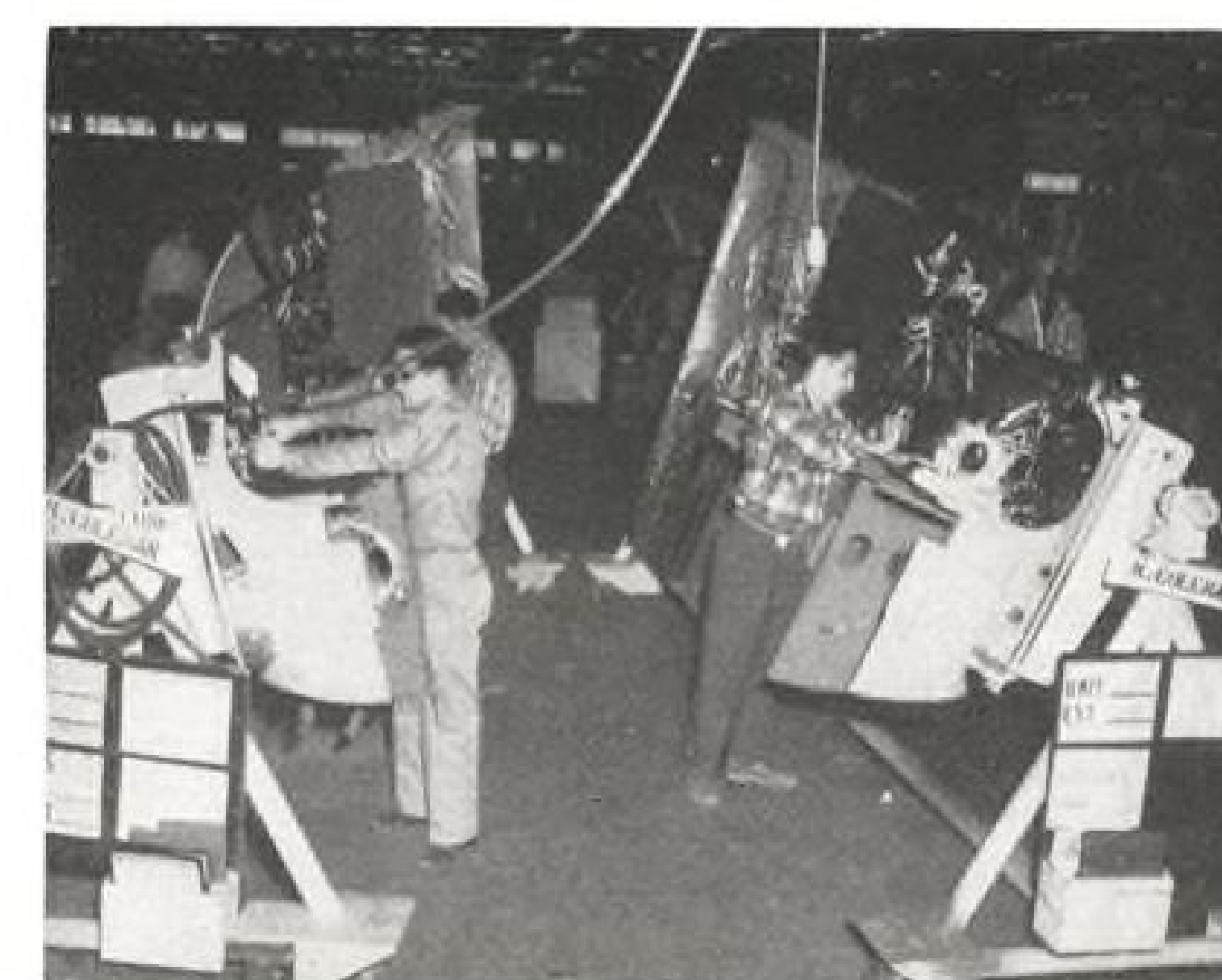
SIDE PANELS will be joined to form the forward fuselage.
