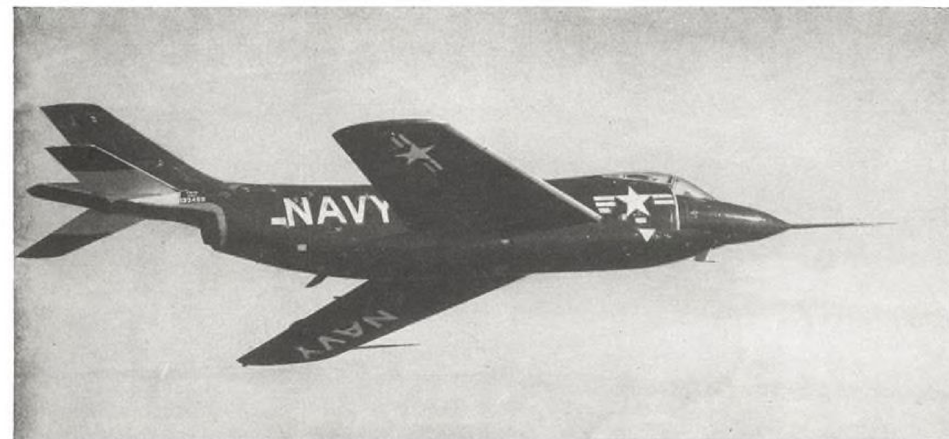
F3H-1N DEMON displays empennage on platypus tail. Stabilizer pivots for trim, maneuvering. Wings fold for carrier stowage.
