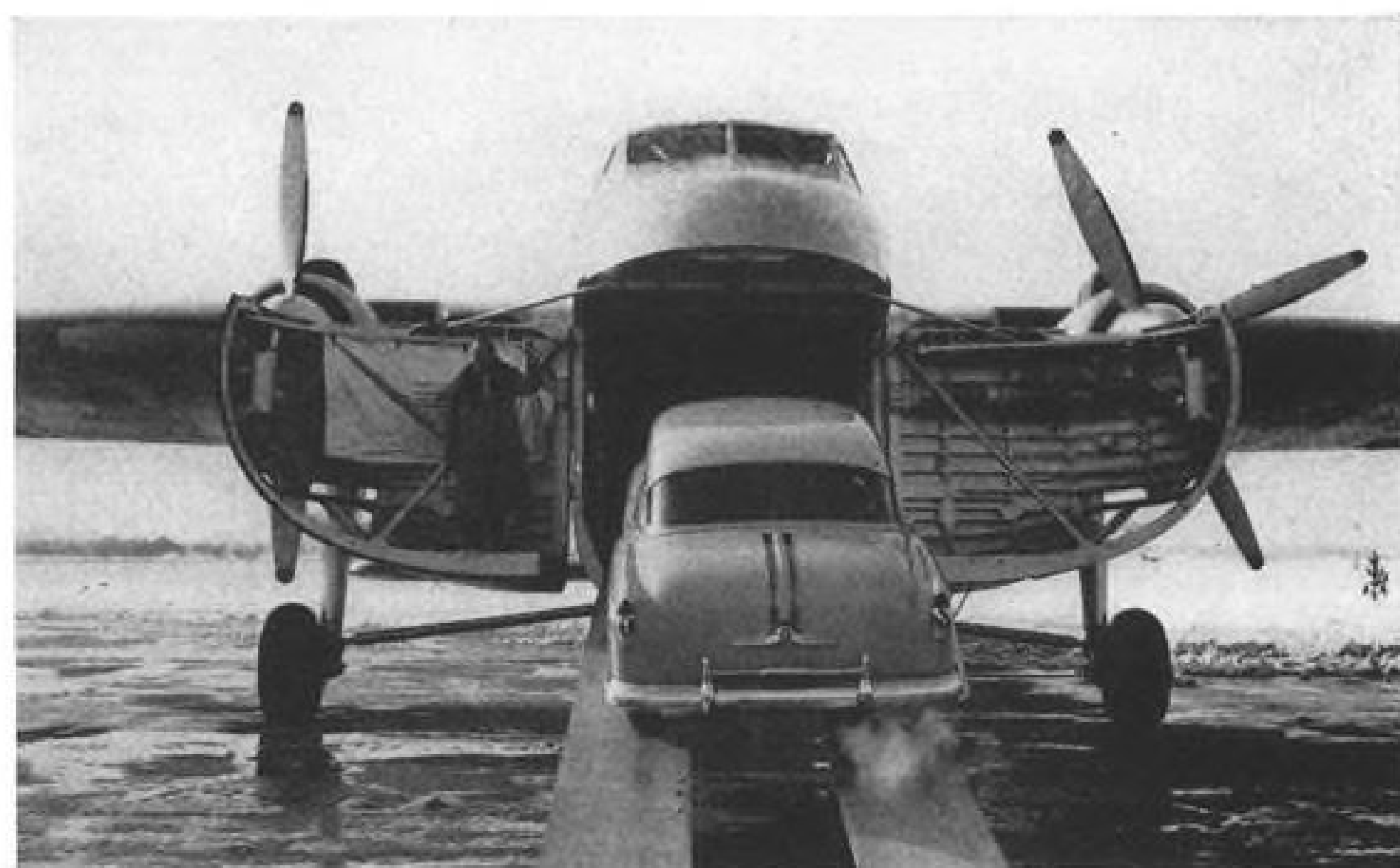
STANDARD-SIZE CAR rides up ramp. Bristol-installed heaters are on each door.
