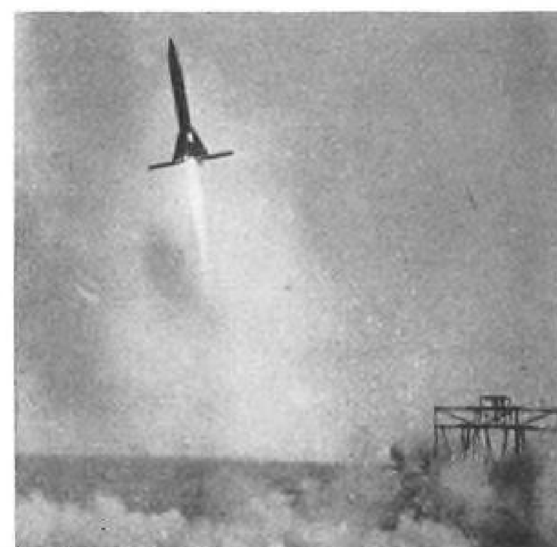
CORRECT ANGLE is insured by drum set up which shortens two inner cables. Cable cross is jettisoned at end of guidance period.
