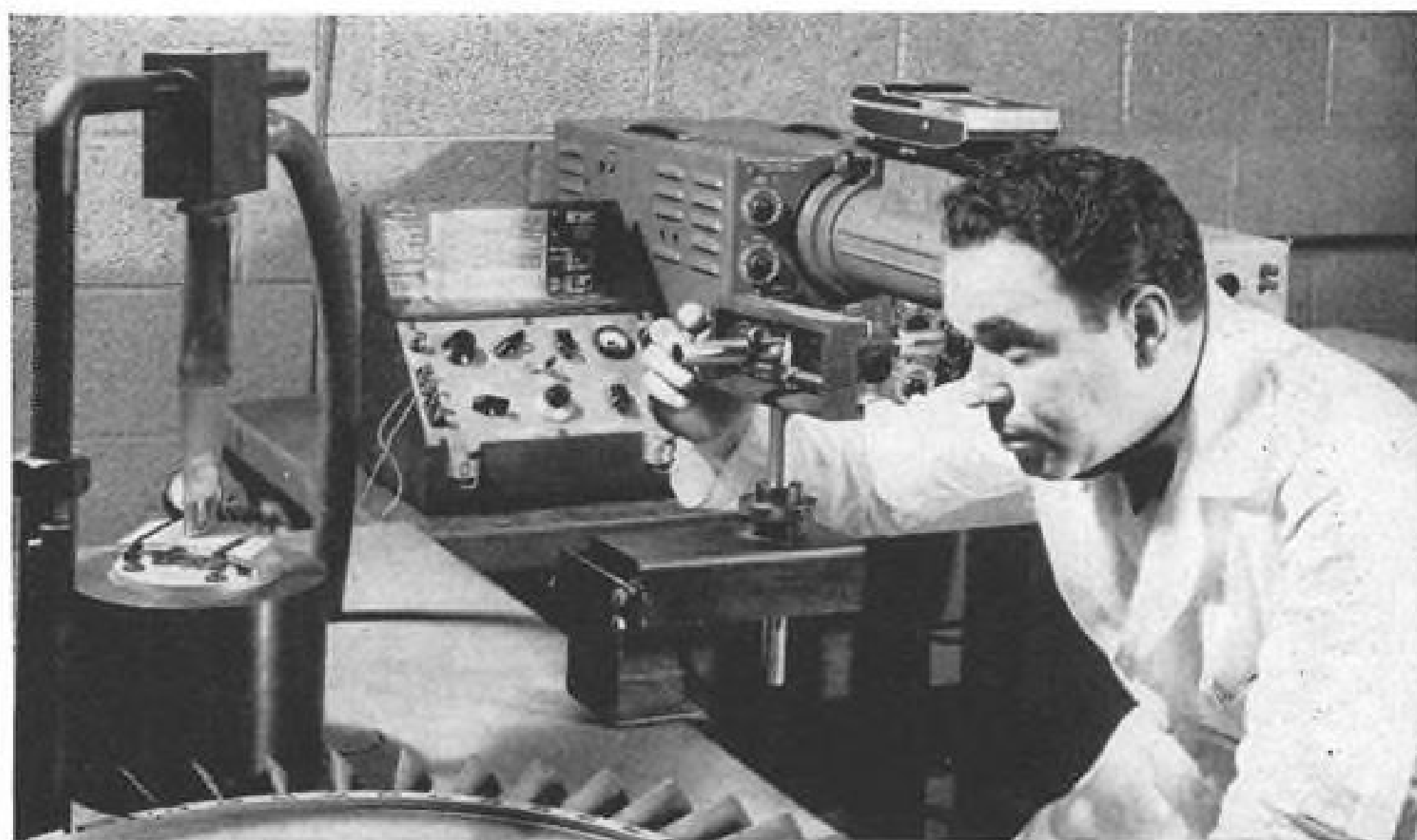
FATIGUE PROPERTY CHECK is given glass-plastic compressor blade after completion of 100-hr. test run in turbojet. Portion of third-stage rotor is at bottom.
