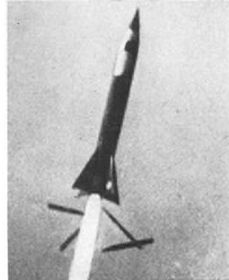
CORRECT ANGLE is insured by drum set up which shortens two inner cables. Cable cross is jettisoned at end of guidance period.
