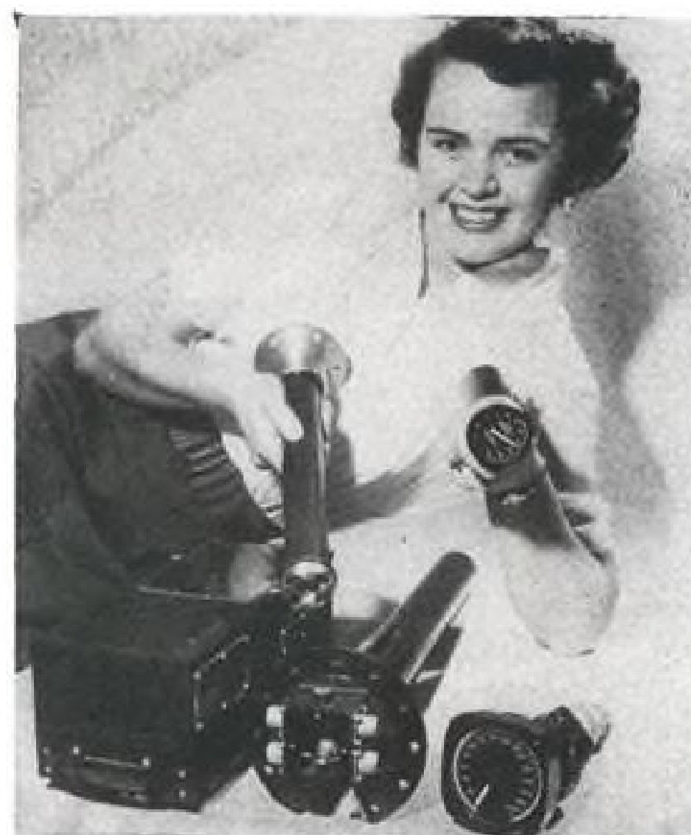
THIS IS FIRST transistorized fuel-gage system in nation, says M-H.
