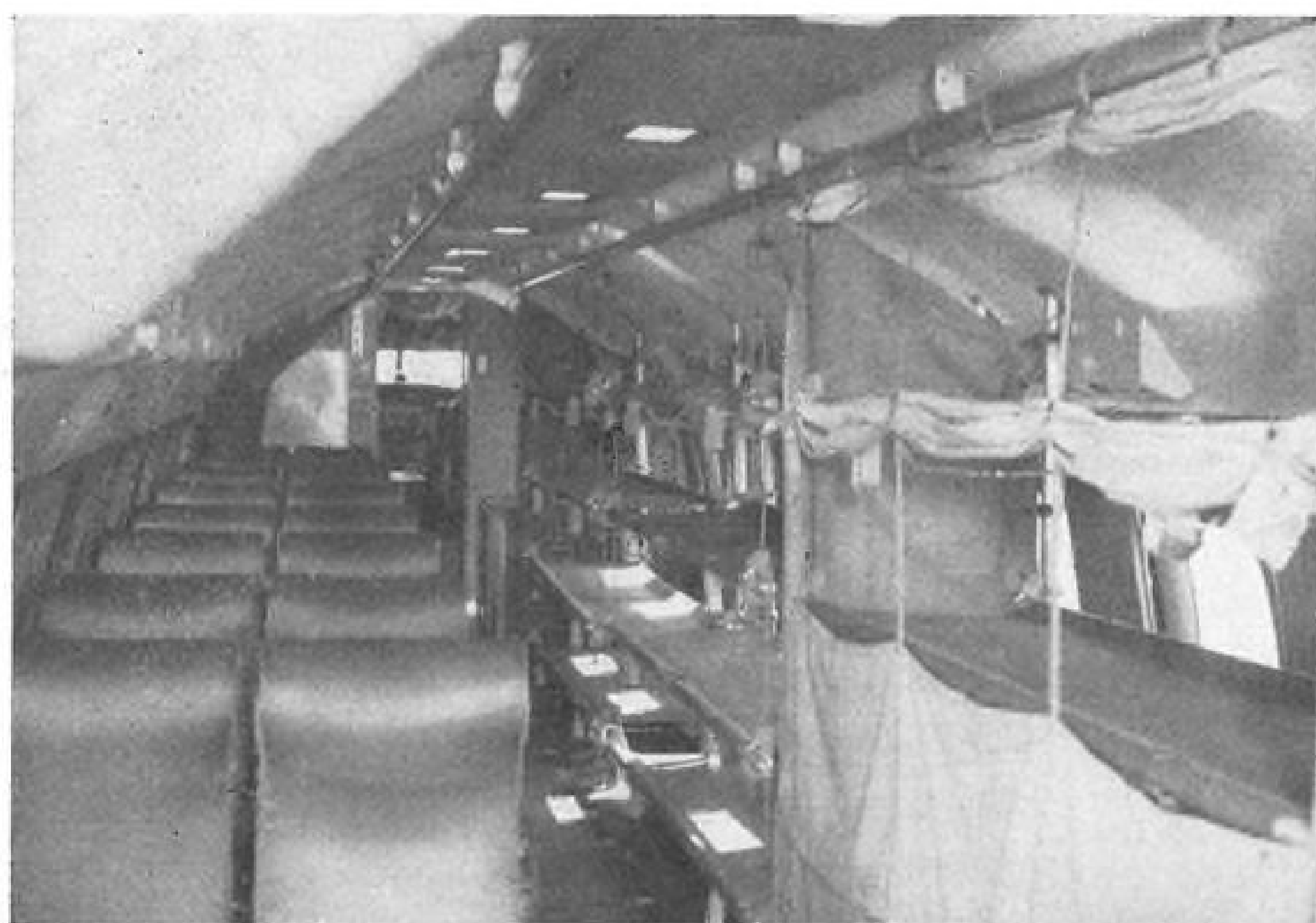
SEAT-LITTER COMBINATION inside C-131A. Quickly detachable seats face rearward.
