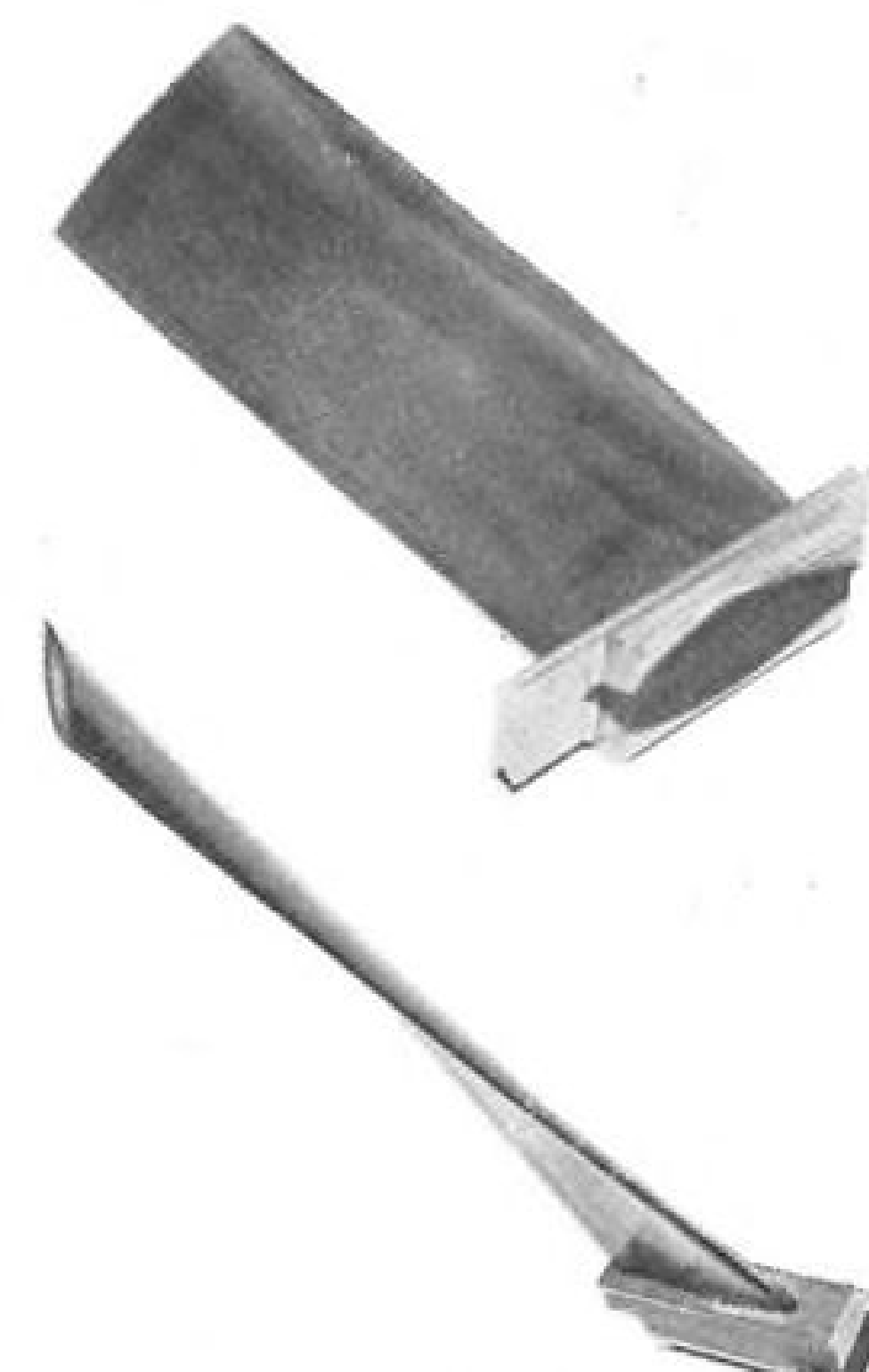
GLASS-PLASTIC BLADE has fine surface finish, metal dovetail root.
