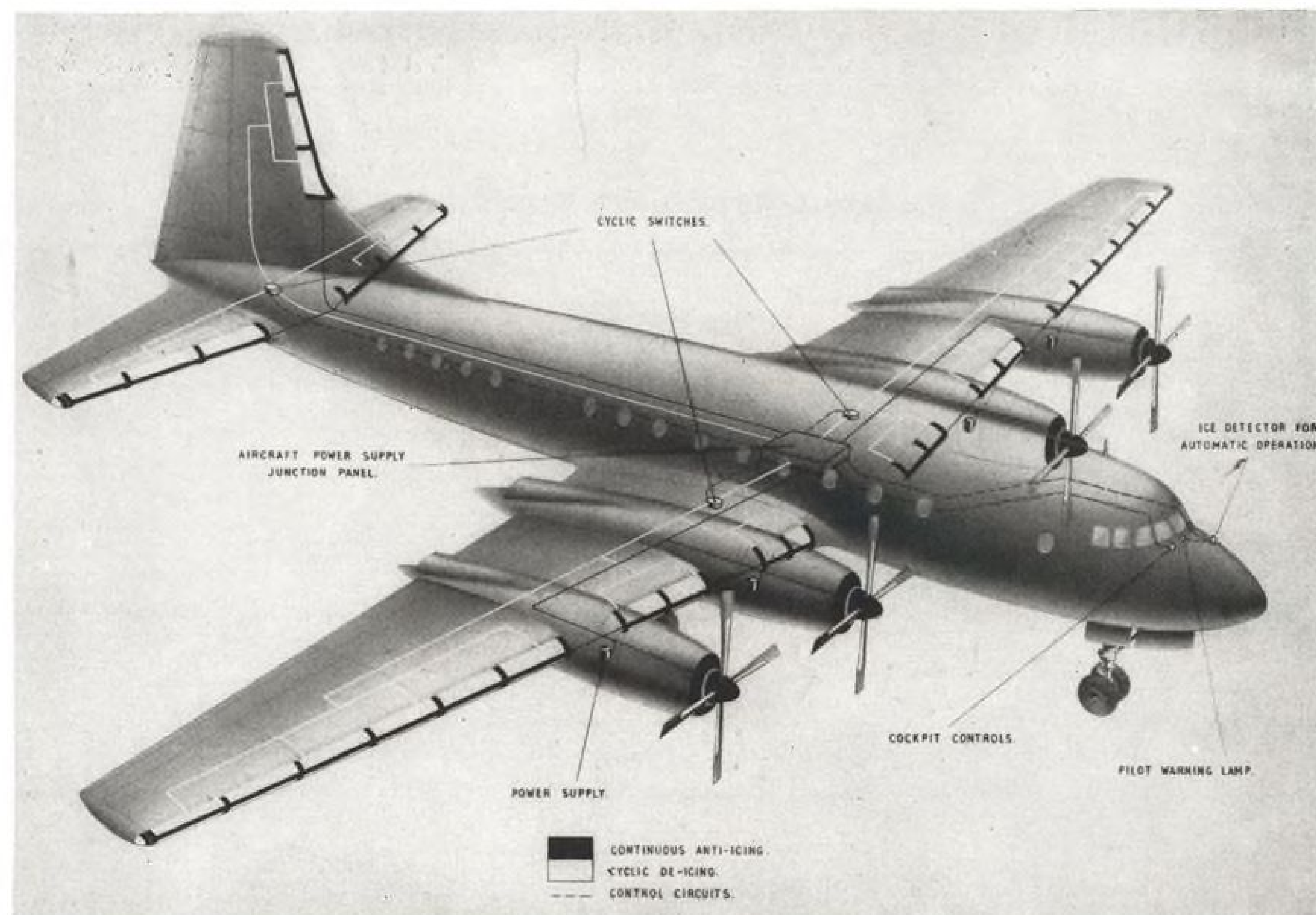
HYPOTHETICAL TURBOPROP TRANSPORT of estimated 120,000-lb. gross weight with sprayed-on de-icing system totaling 1,064 lb.
