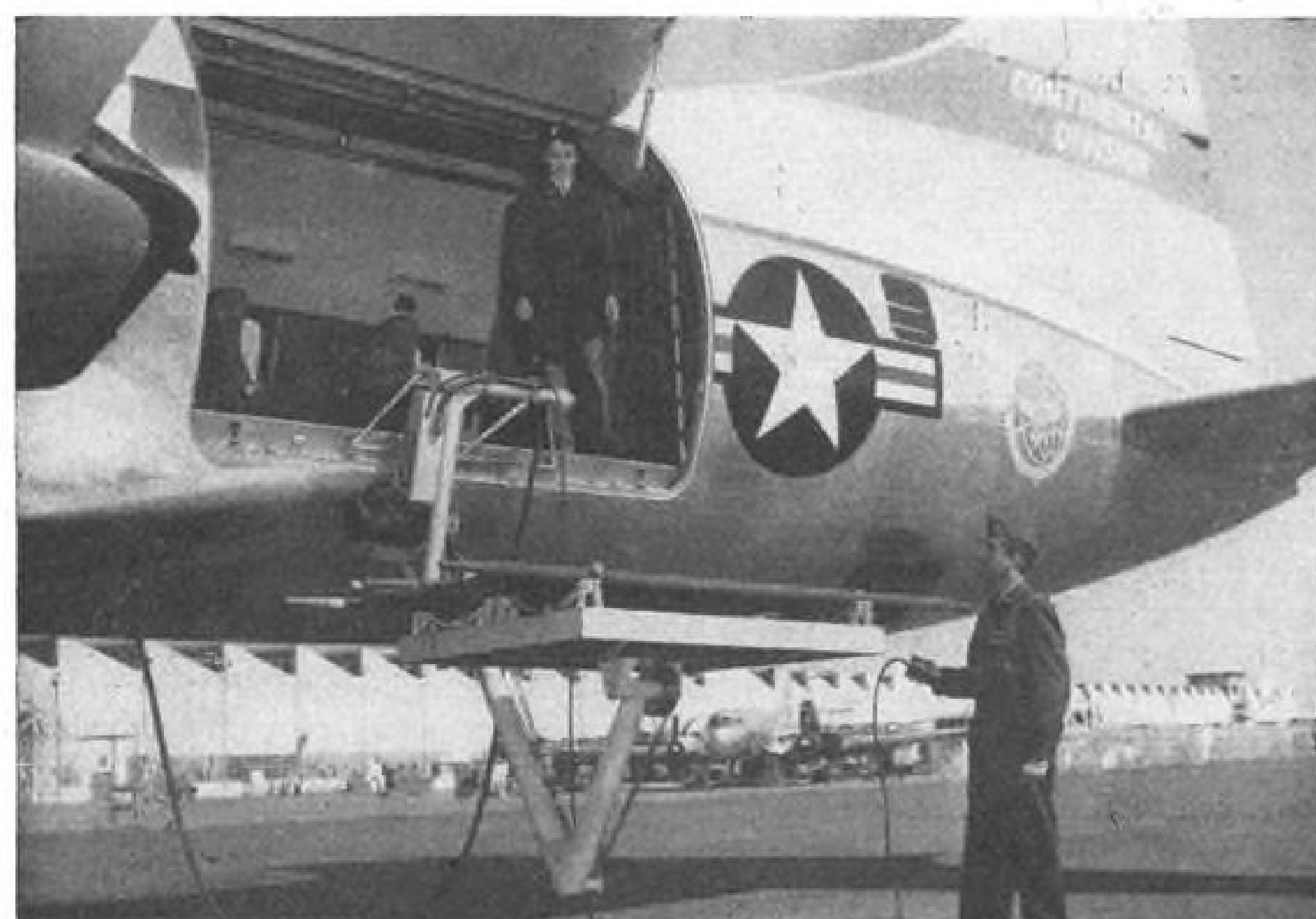
ELECTRIC LIFT can hoist two litters or 500 lb. of cargo smoothly through wide door.
