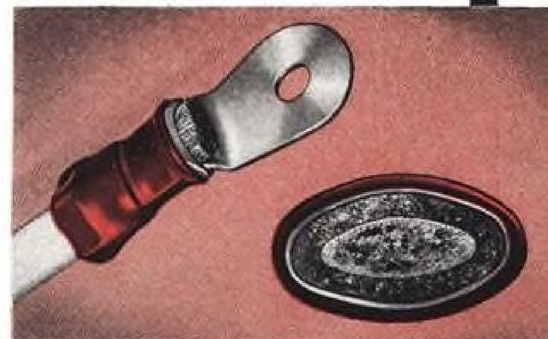
BONDING FEATURE MOST IMPORTANT Bonded insulation is the most important factor in producing a successful insulated terminal. The positive and complete bond of the insulation to the terminal sleeve insures uniform insulation thickness under crimping pressures, and therefore transmits this pressure evenly to the center of the crimp area. With this precision-engineered A-MP crimp and BONDED insulation you can be sure of maintaining proper dielectric and tensile values in the finished connection. More intimate contact achieved by confining, over a greater area, terminal and wire under intense crimping pressure.
