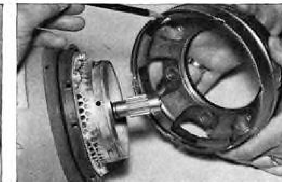
QUICK-ATTACH-DETACH mounting flange sharply reduces time required for generator removal or installation.
