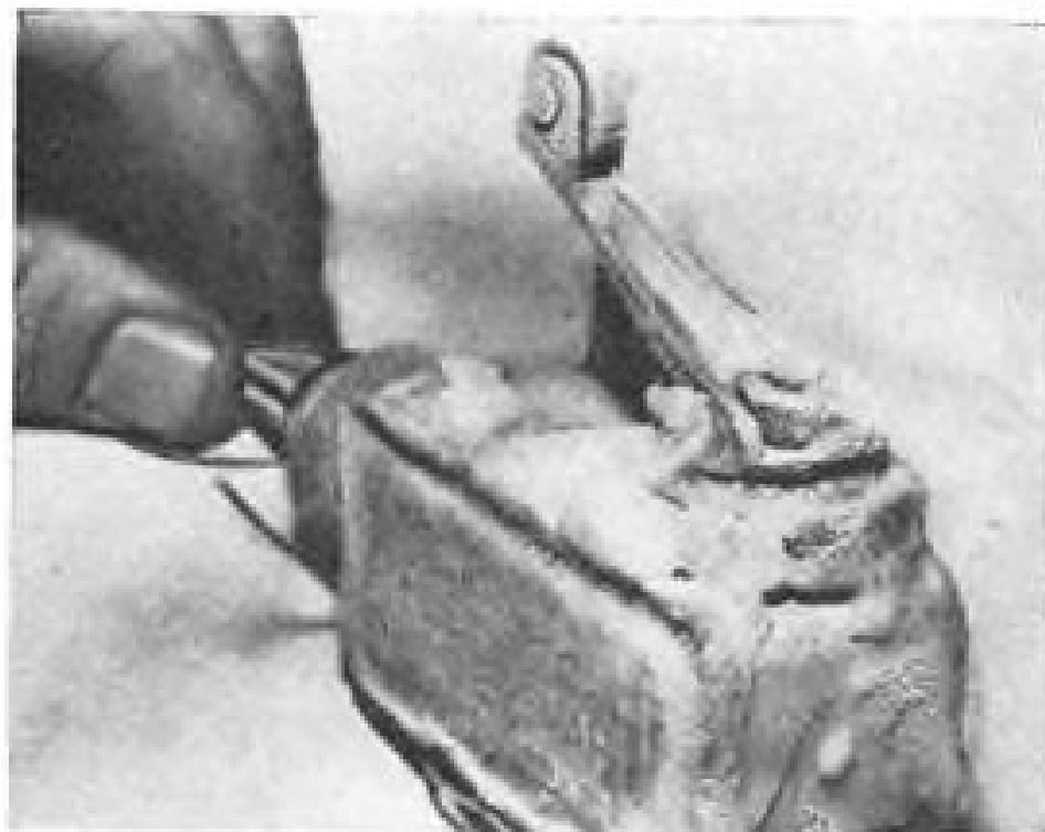
ICE FORMATION on B36H hermetic-sealed switch (shown in depressed position in top photo) does not prevent switch release (bottom).
