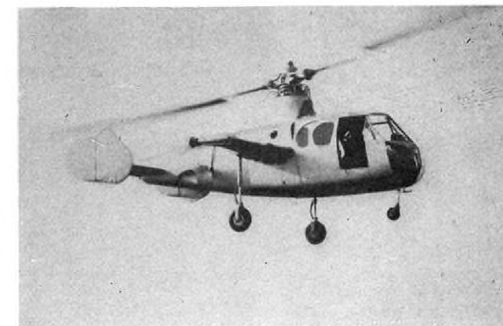
JET COPTER ALOFT—British Fairey Gyrodyne starts flight tests. Piston engine drives compressors supplying air to pressure jets at rotor tips. Wing stubs have pusher props.
