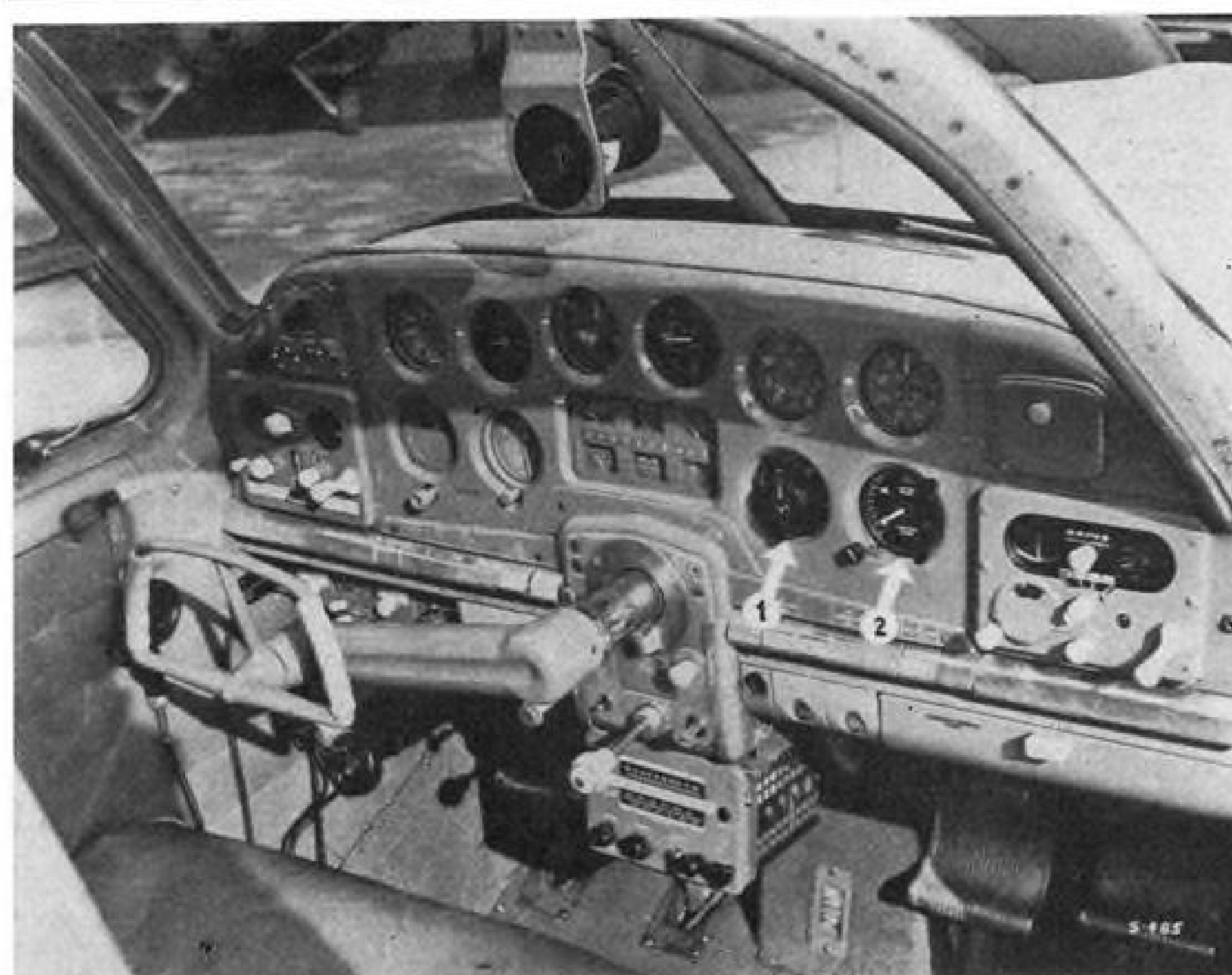
NARCO DME installed in Beech Bonanza. Frequency selector switch (1) operates crystal-tuned receiver. Range scale (2) is changed from "en route" (0-200 mi.) to "approach" (0-20 mi.) by turning knob. Designated UDI-1, set costs $5,000.
