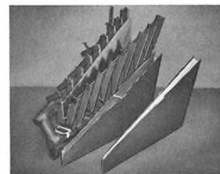
From left to right: (1) Open jig for wing assembly. (2) Skin of same wing assembly before core is poured. Note that no interior strengthening members or re-inforcements are necessary. (3) Finished assembly. Stronger, lighter, and more economically produced.
