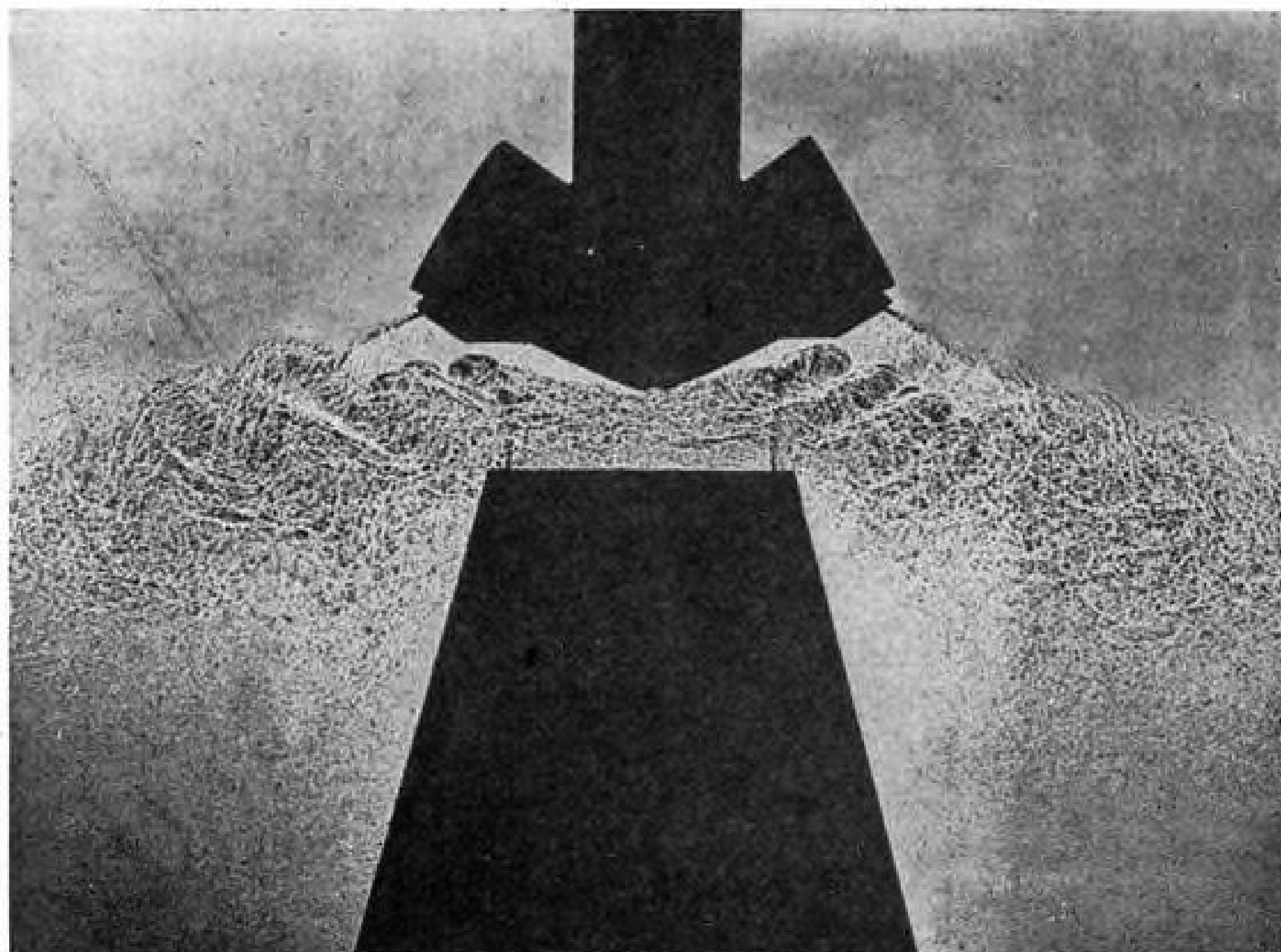
BLAST SHADOWGRAPH reveals how tailpipe exhaust is deflected by jet reverser.
