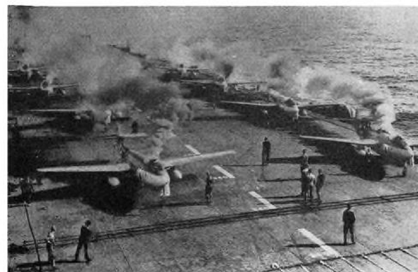
SMOKY START—Dense smoke from cartridge starters of Hawker Sea Hawk jet fighters rolls over the deck of 36,800-ton HMS Eagle during recent maneuvers in the Mediterranean Sea.
