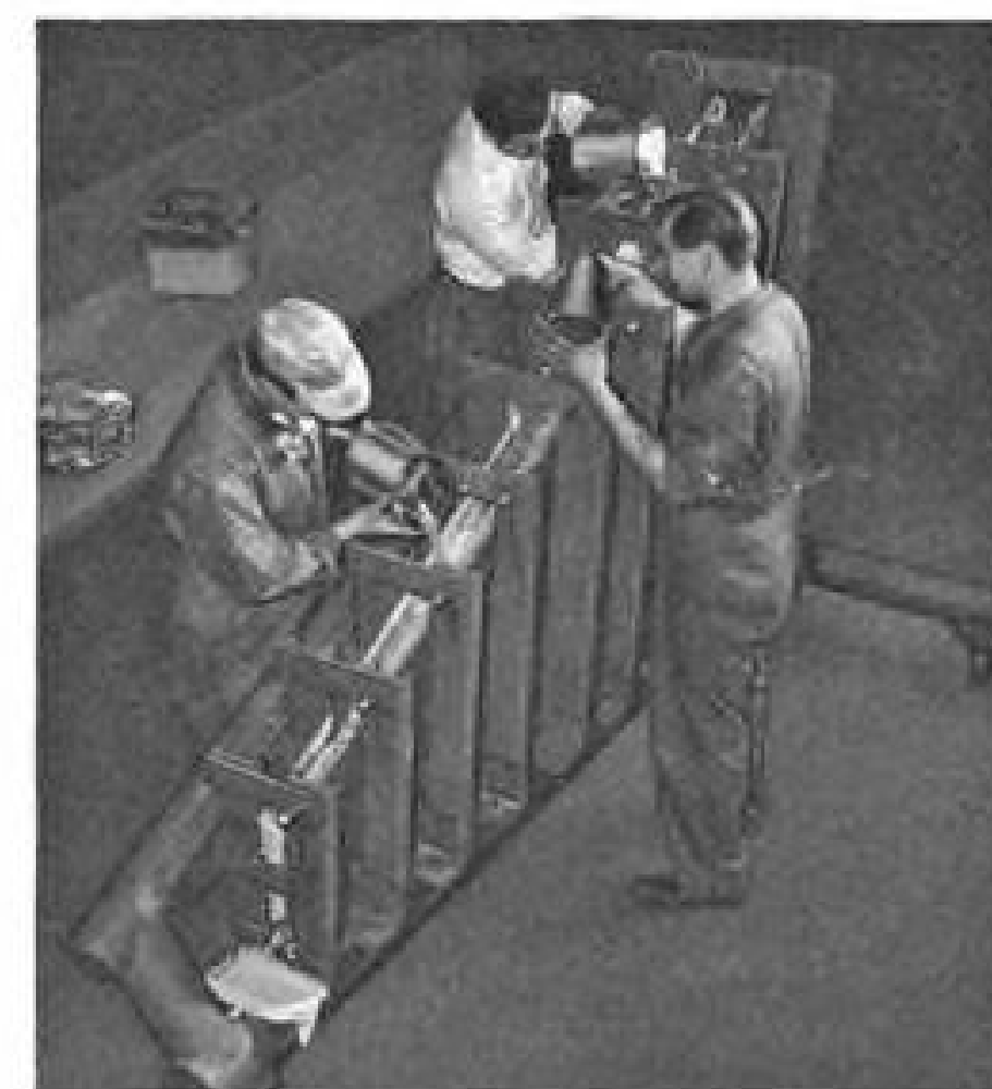
Here workmen are pouring the entire core of a complete wing assembly.
