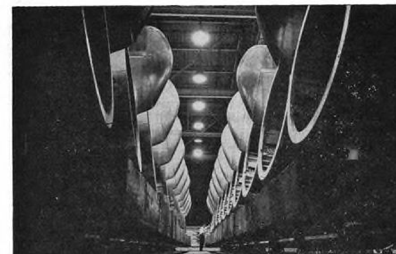
TAIL ASSEMBLIES and control surfaces are stacked on wheeled storage racks awaiting their turn to be fed into Martin B-57A production lines at the company's Baltimore, Md., factory.
