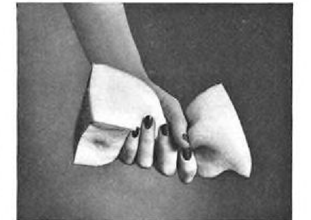
Ease of compressibility of Flexible STAFOAM is shown here. Other STAFOAMS can be made tough and leathery.
