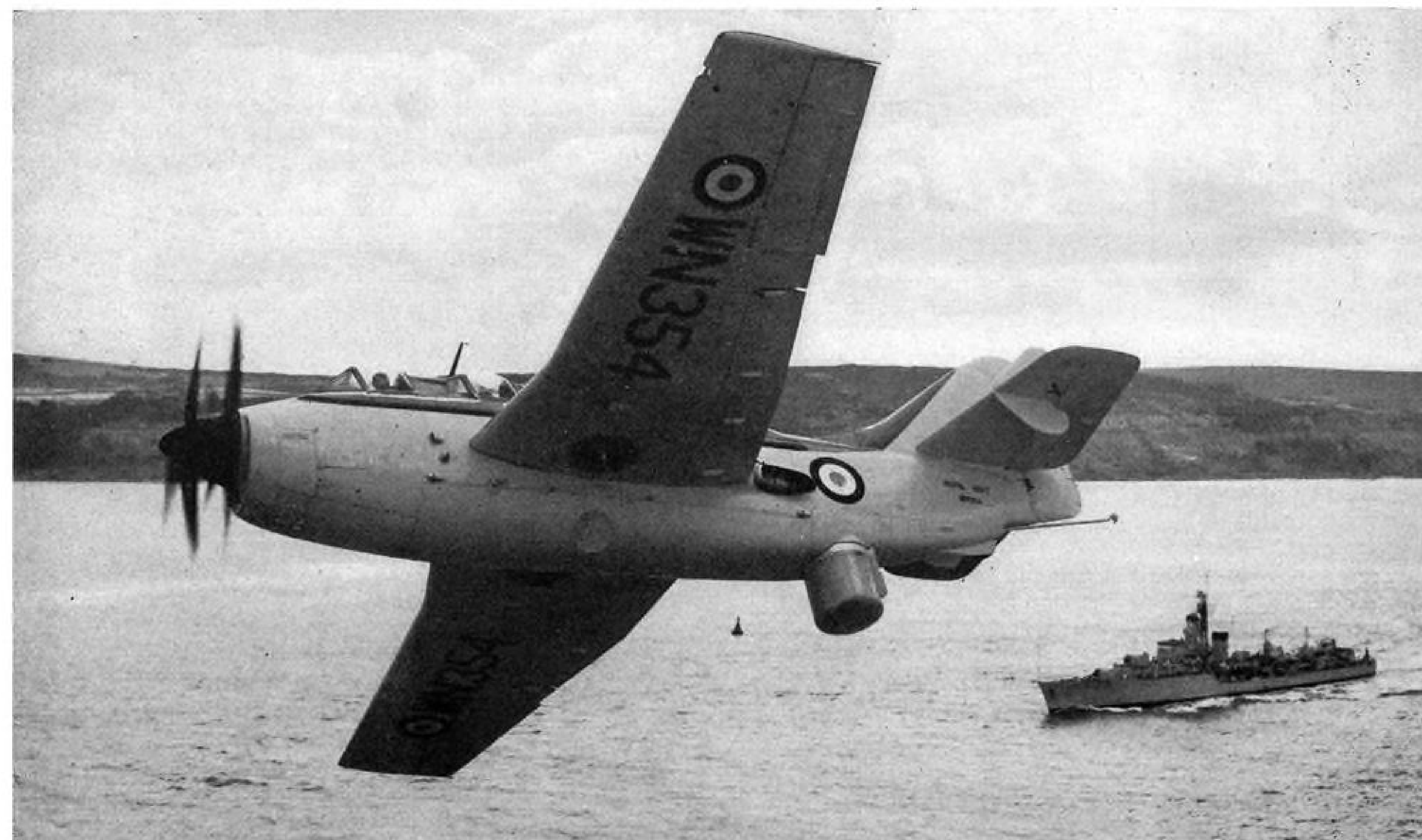
BRITISH SUB HUNTER—Turboprop-powered Fairey Gannet (below) banks low over the water with its radar "bin" extended.
