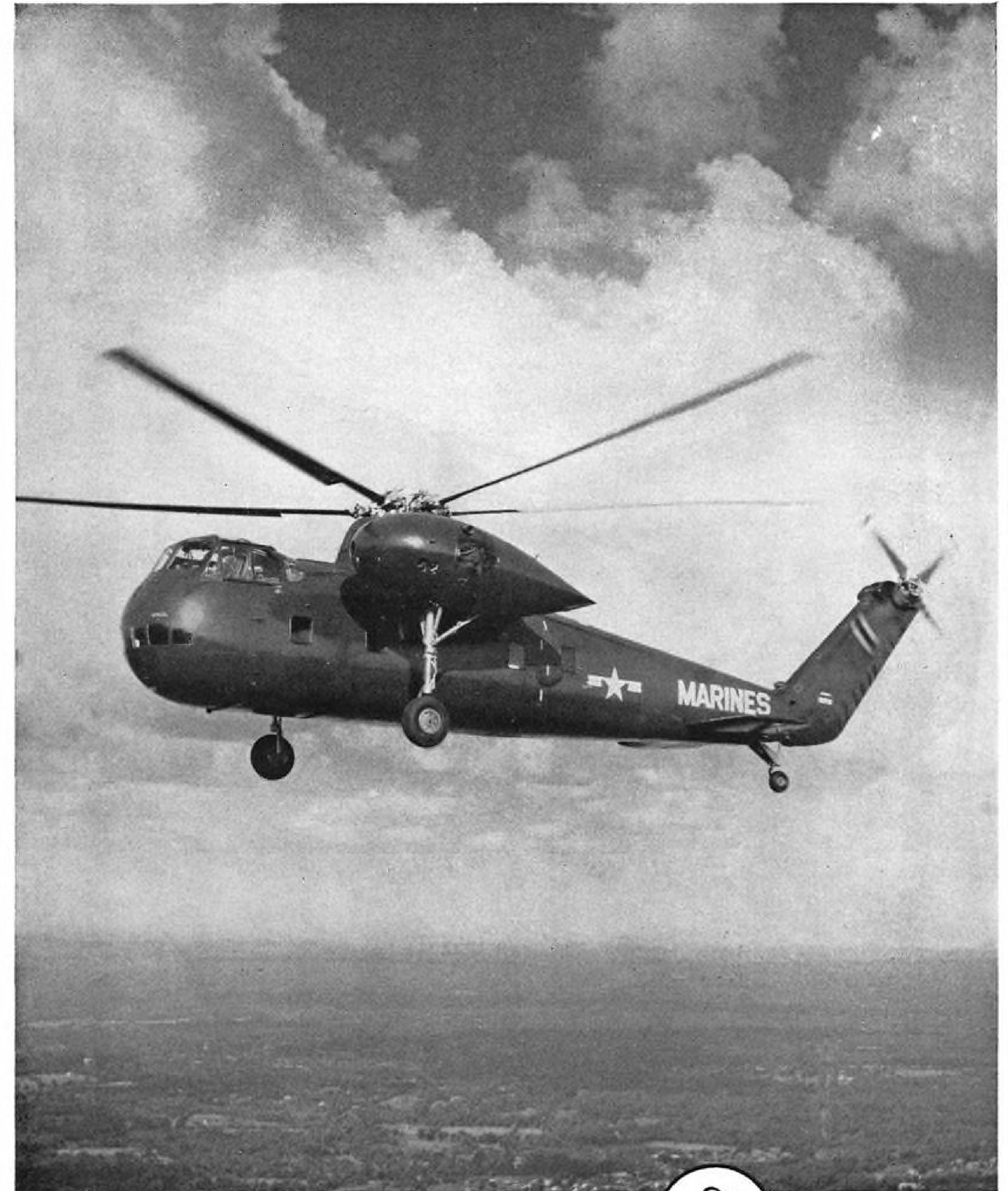
BUILT FOR BATTLE —Sikorsky Aircraft's rugged XHR2S, the most powerful helicopter now flying, was designed to carry out modern vertical assault tactics. It has flown with over 6,500 pounds of payload, and at speeds well over 150 m.p.h. with landing gear retracted into engine pods. Five-bladed main rotor and the tail both fold mechanically for easy stowage and handling aboard ship.
