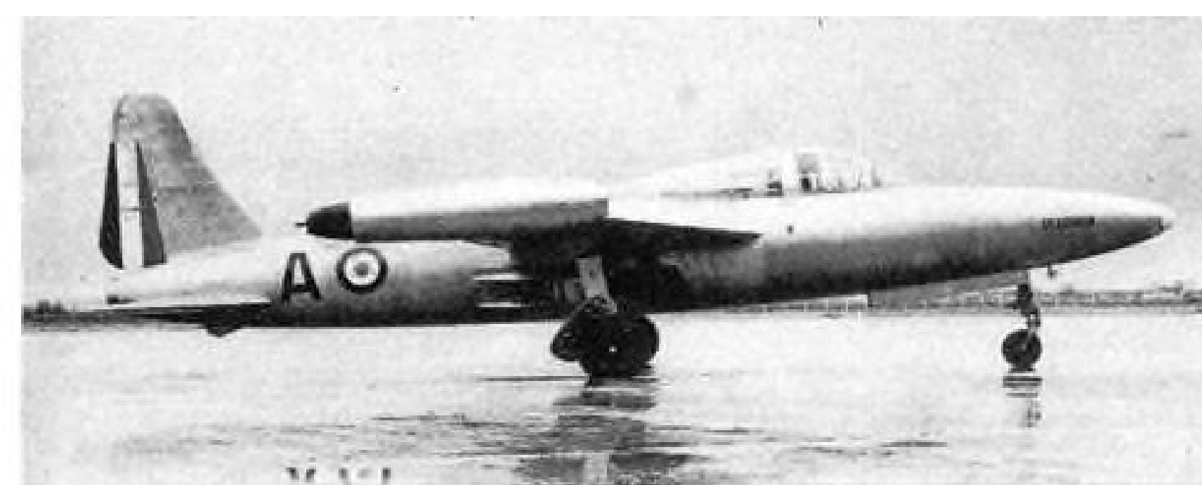
WINGTIP JET TESTS—French are testing a Sncaso S.O. 6020 Espadon jet fighter (above) with small wingtip-mounted Turbomeca turbojets fitted with afterburners.
