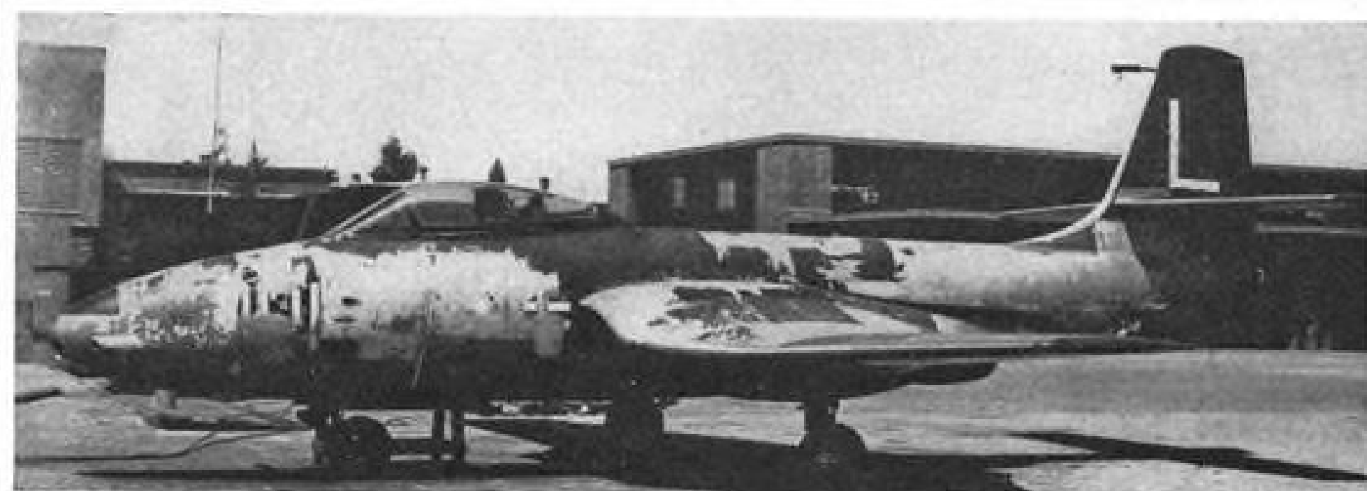
CONVENTIONAL PAINT peels off large areas of Banshee after only 37 flying hours.
