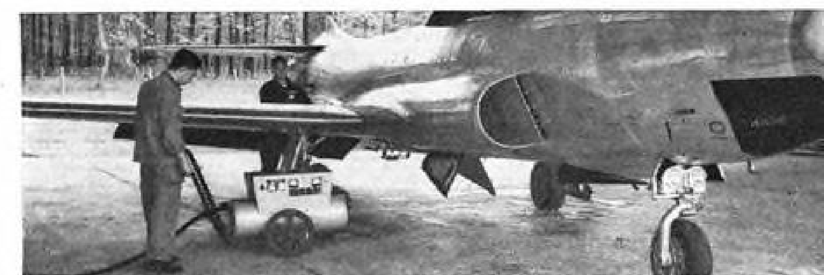
G-E Motor Driven Energizer, 500/1000-amp, 28-volt (above) See Bulletin GEA-5989
