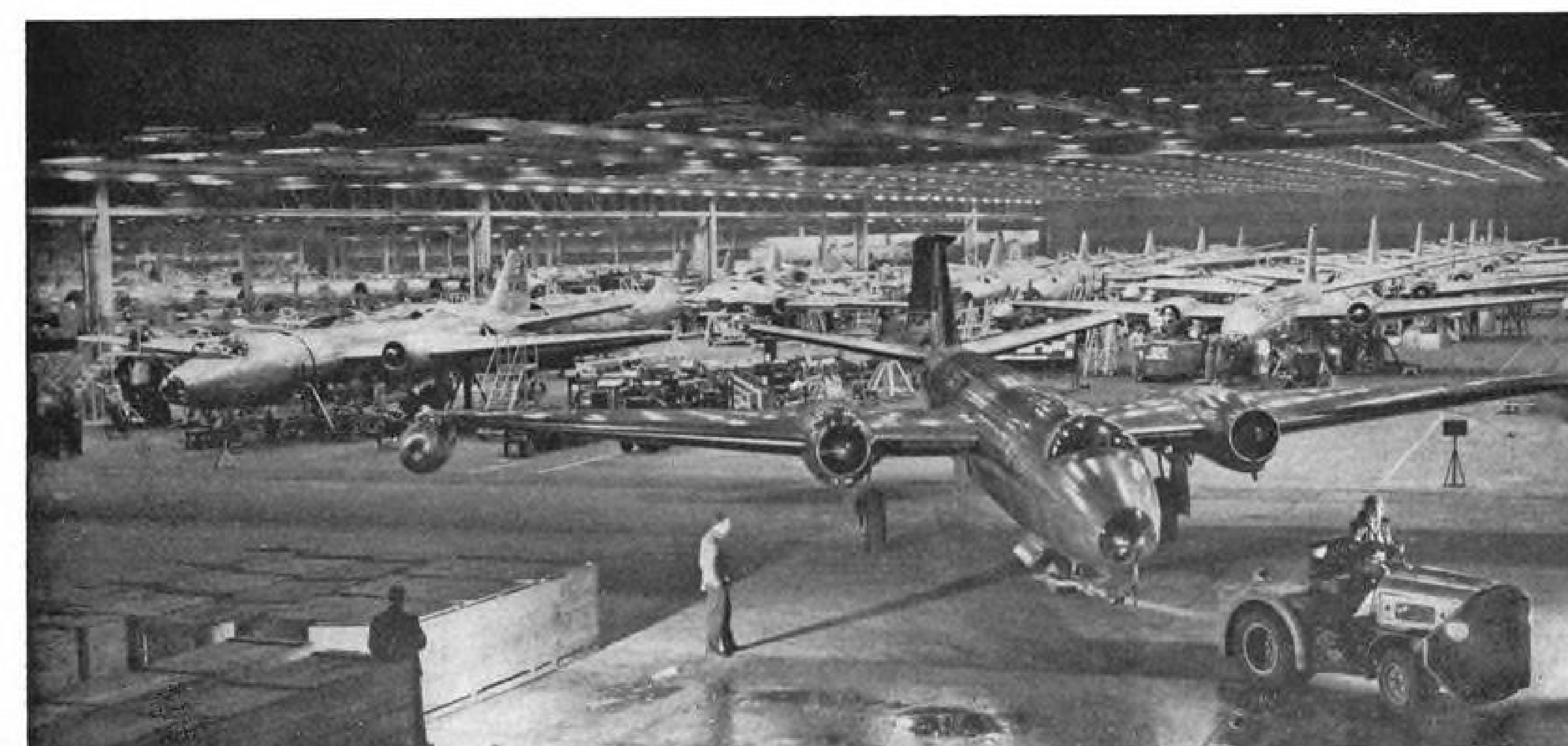
MARTIN B-57A light bomber leaves U-shaped final assembly lines at night. Bomber deliveries began last August.
