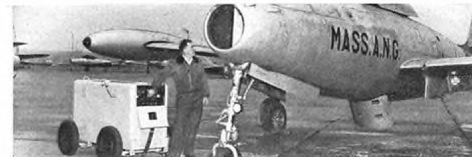
Engine Driven G-E Energizer, 28-volt, 500/1000-amp, (above) See Bulletin GEA-5988
