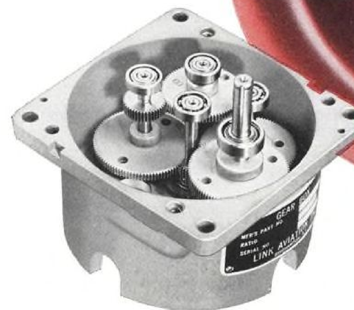
Link Hi-Precision Gear Box, one of many in the Flight Simulator, shows the New Departure ball bearings that maintain accurate gear pitch-line contact . . . almost entirely eliminate backlash and friction.
