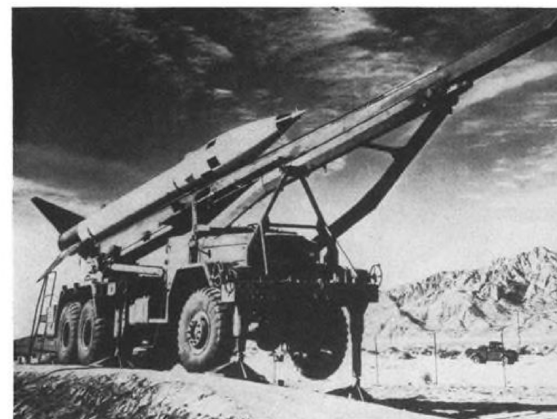
HONEST JOHN is heavy field artillery rocket with mobility exceeding some current conventional artillery. Fired from special truck which combines transport and launcher, Honest John is unguided, can carry atomic or conventional warheads with equal ease. Diameter is 30 in.
