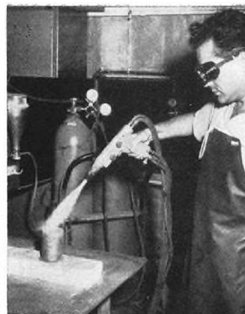
CERMETS are sprayed like paint on stainless steel parts with 5,500F gun.
