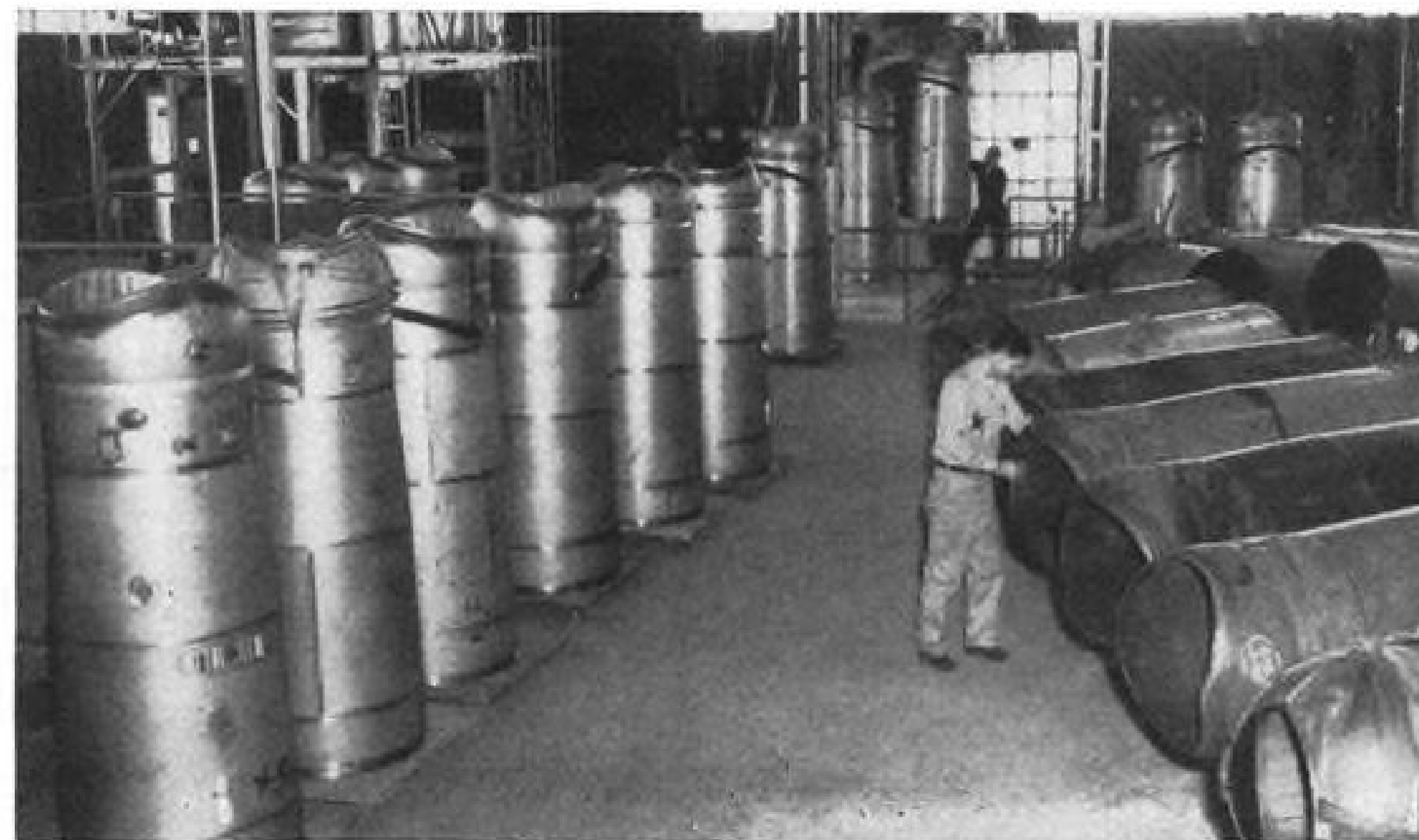
RYAN AFTERBURNERS, like these for the J47, generate temperatures to 3,500F.
