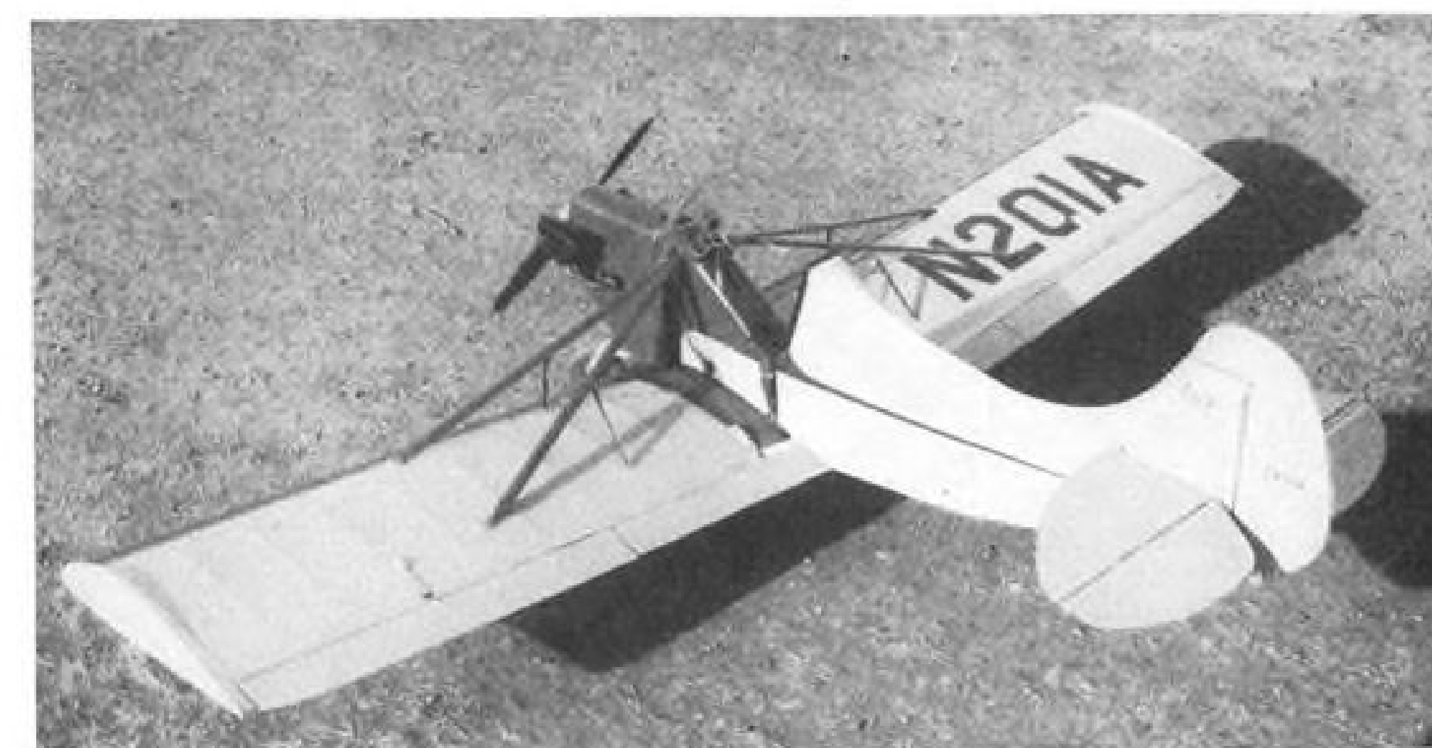
NARROW FUSELAGE is only 12 in. wide. Small spray tanks may be fitted in wings.
