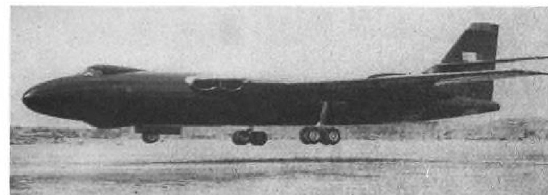
BOGIE LANDING GEAR has four wheels on each main leg. Fuselage, longer than prototype's, has been extended, apparently by adding section ahead of wing.
