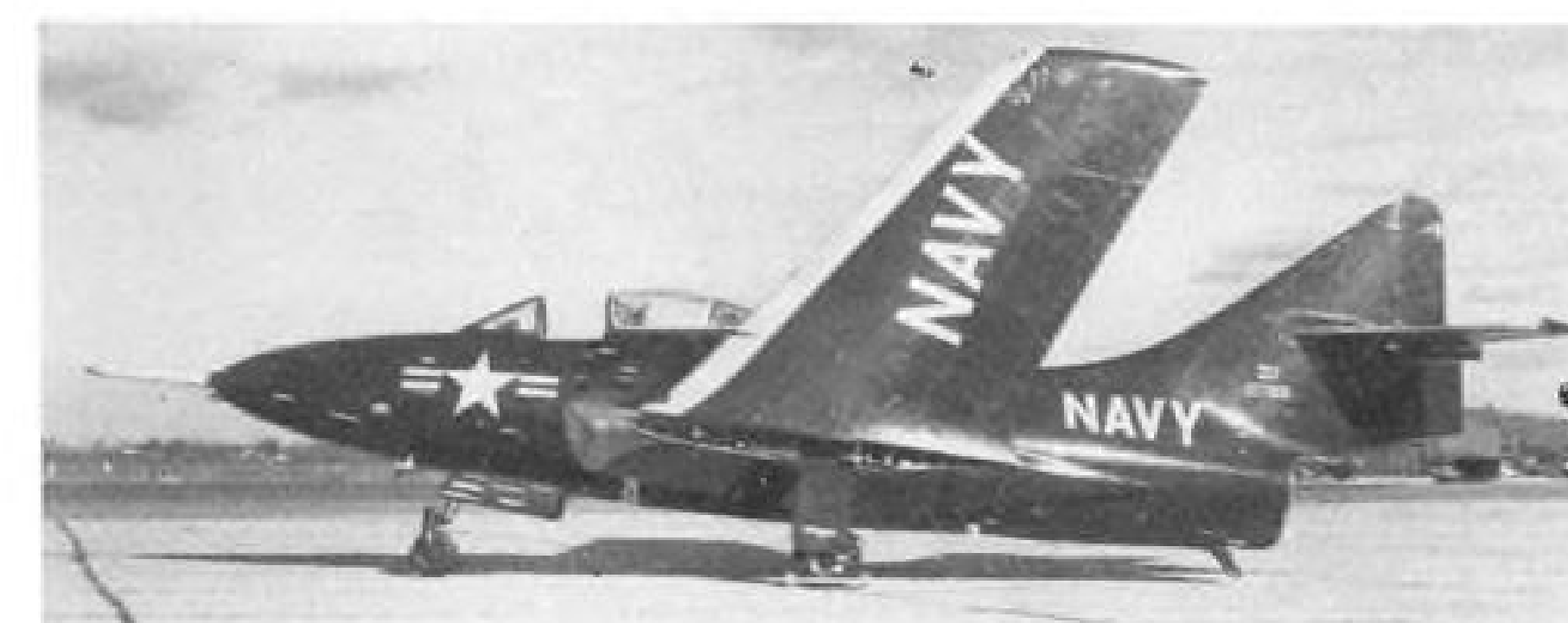
F9F-6 COUGAR with wings folded shows straight-line leading edge, shorter wing fillet stopping well short of P&WA J48 exhaust. Note air-refueling nose probe.
