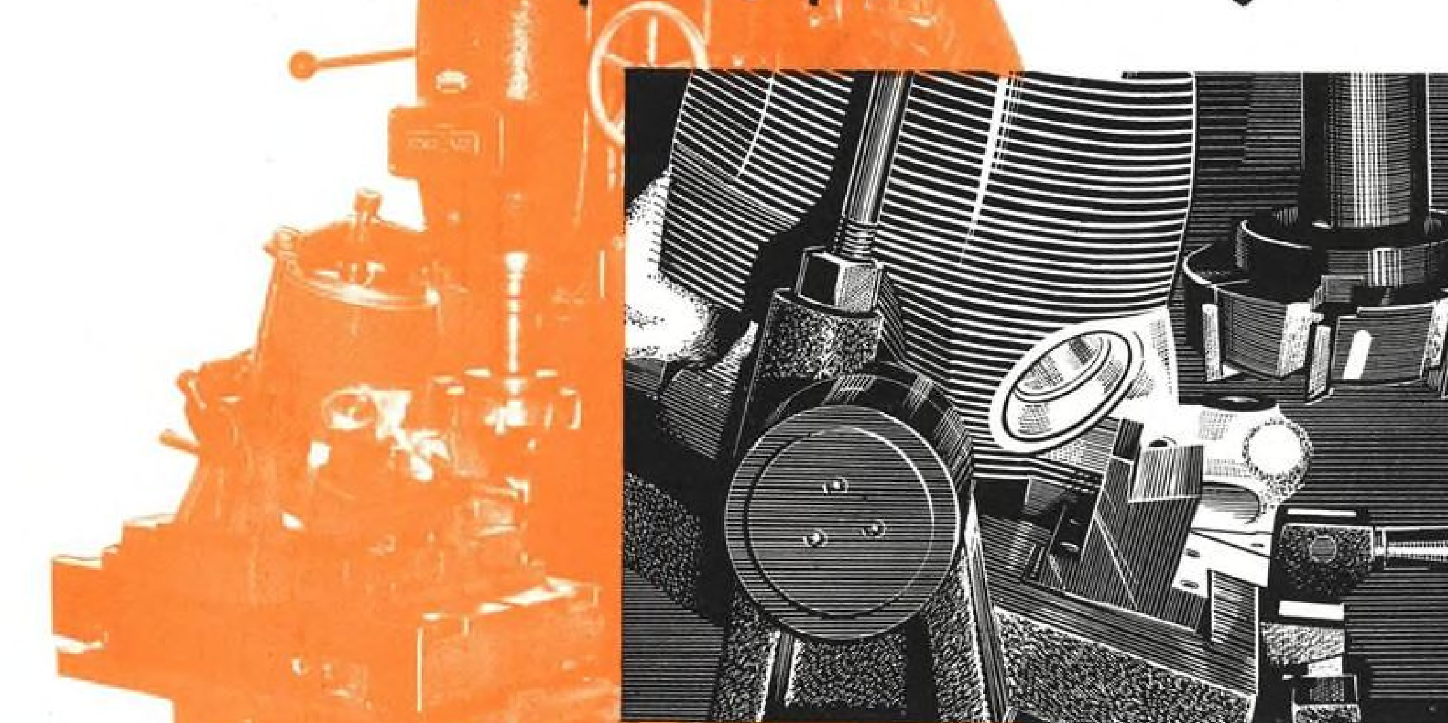
OK CARBIDE CUTTER, ON CINCINNATI VERTICAL FINISH-MILLS RIGHT ANGLES OF INTAKE AND EXHAUST PUSH ROD FACES, OF PRATT & WHITNEY AIRCRAFT WASP MAJOR ENGINE CLIMB-MILLING ONE AND CONVENTIONAL-MILLING THE OTHER
