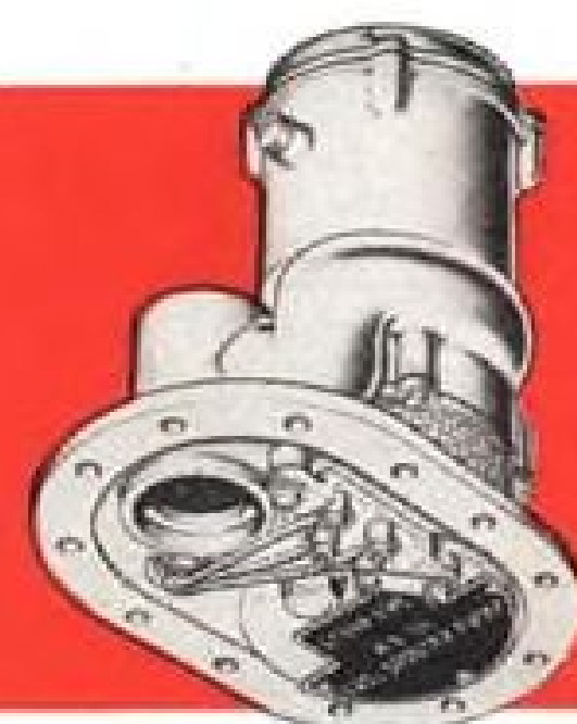
Submerged A.C. Electric Motor Driven Fuel Booster Pump. Supplies 20,000 lb. per hour of Aviation Fuel at 6 psig discharge pressure.
