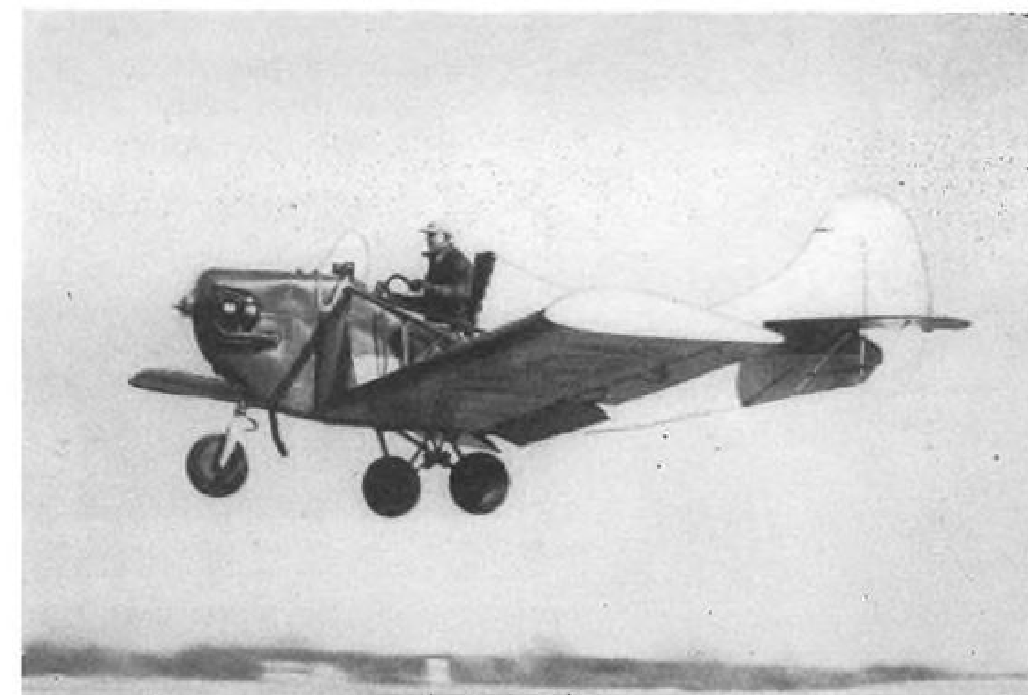
PILOT SITS ASTRIDE Fly-Cycle fuselage and uses motorcycle-type handlebar controls.
