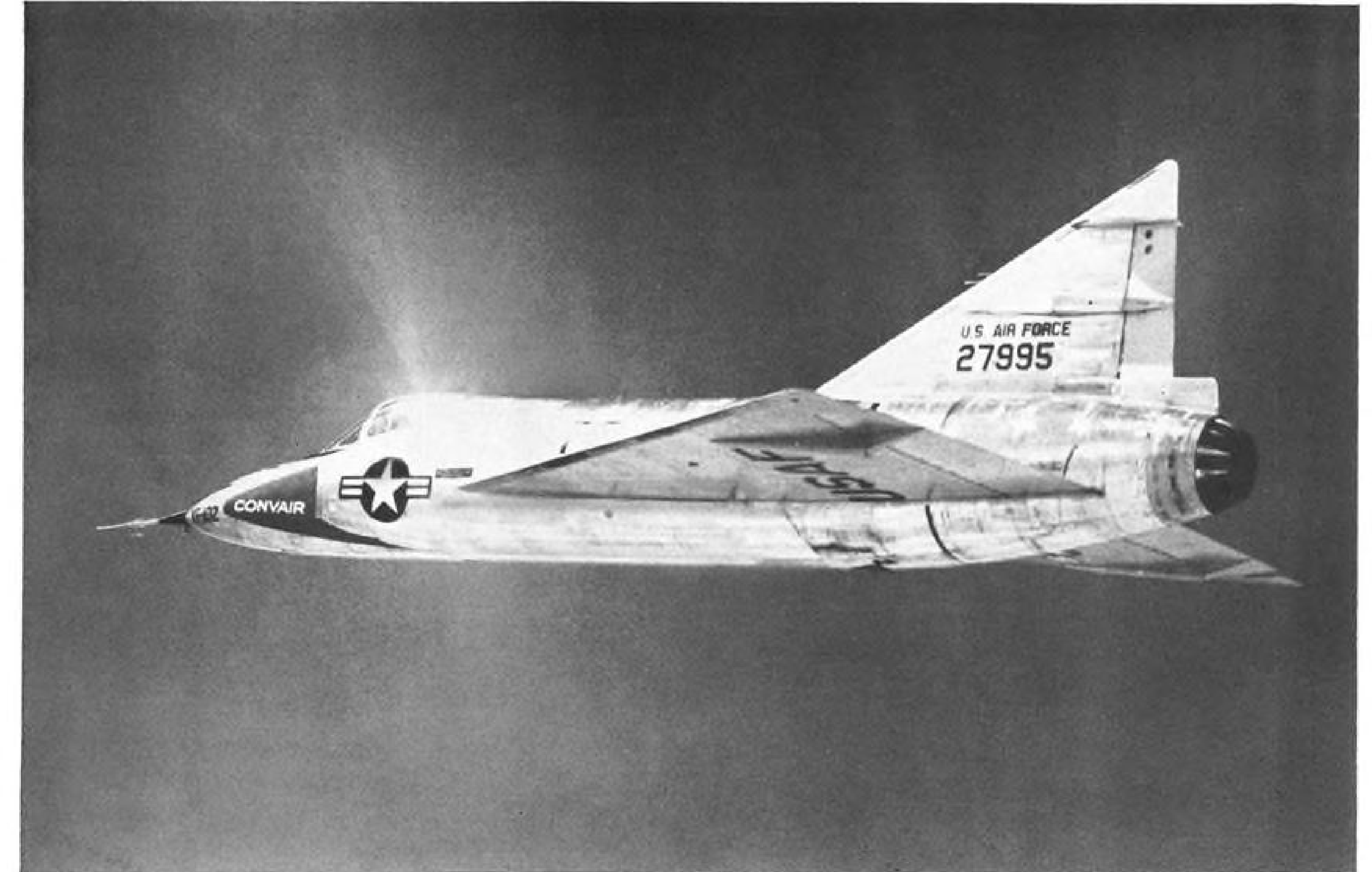
Sun glints from the canopy of this F-102, prototype of the first delta-wing, all-weather interceptor. It was designed and built for the U.S. Air Force by Consolidated Vultee Aircraft, and is powered by the Pratt & Whitney Aircraft J-57 with afterburner.
