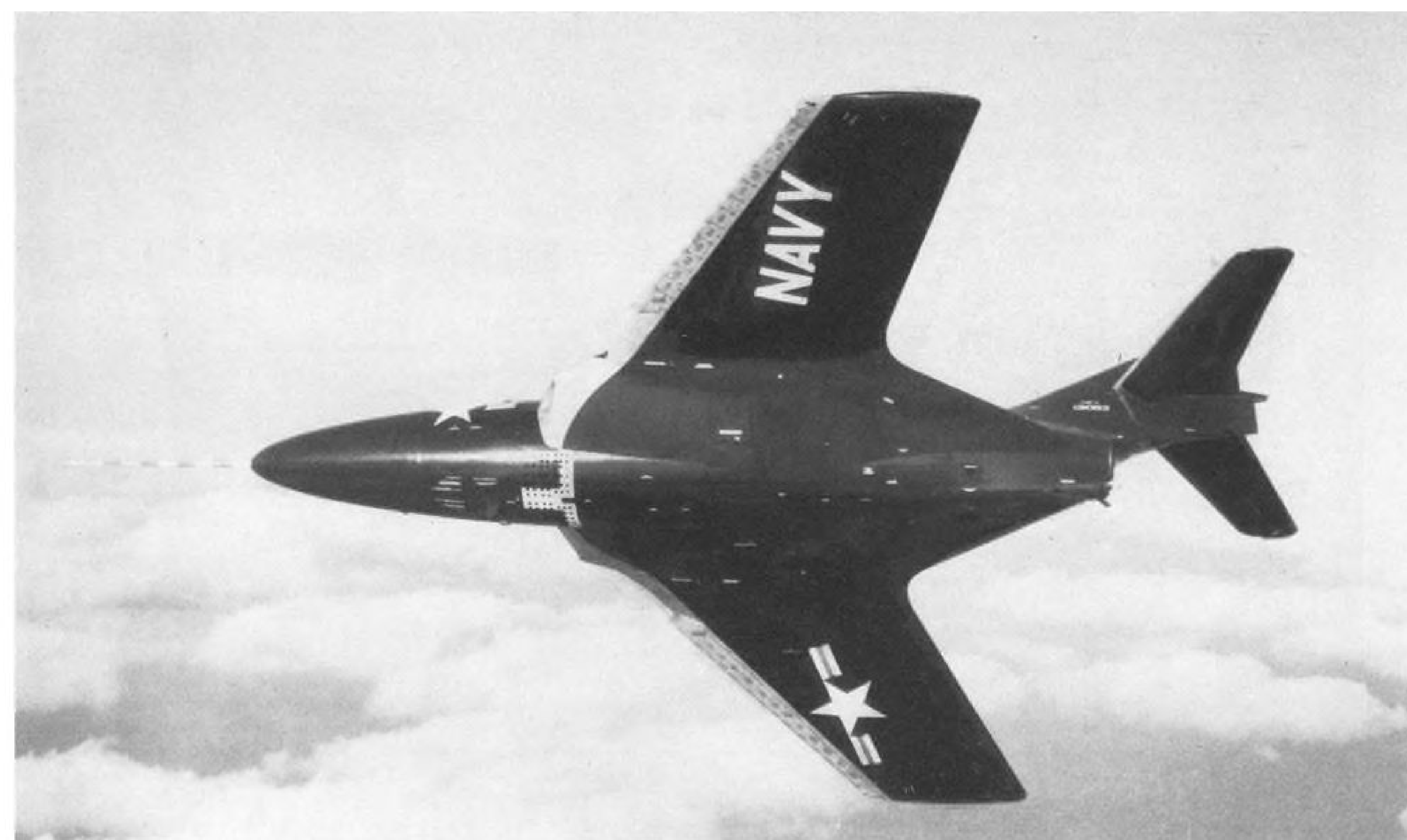
F9F-8 COUGAR differs from earlier Grumman F9F-6 (below, right) in its cambered leading edge wing extensions and extended trailing edges, increasing wing chord 15% and providing relatively thinner wing for higher speeds. Deletion of leading edge slats provides space for 30 gal. of extra fuel in each wing. F9F-8 is being phased into F9F-6 and F9F-7 lines at Bethpage, N. Y.
