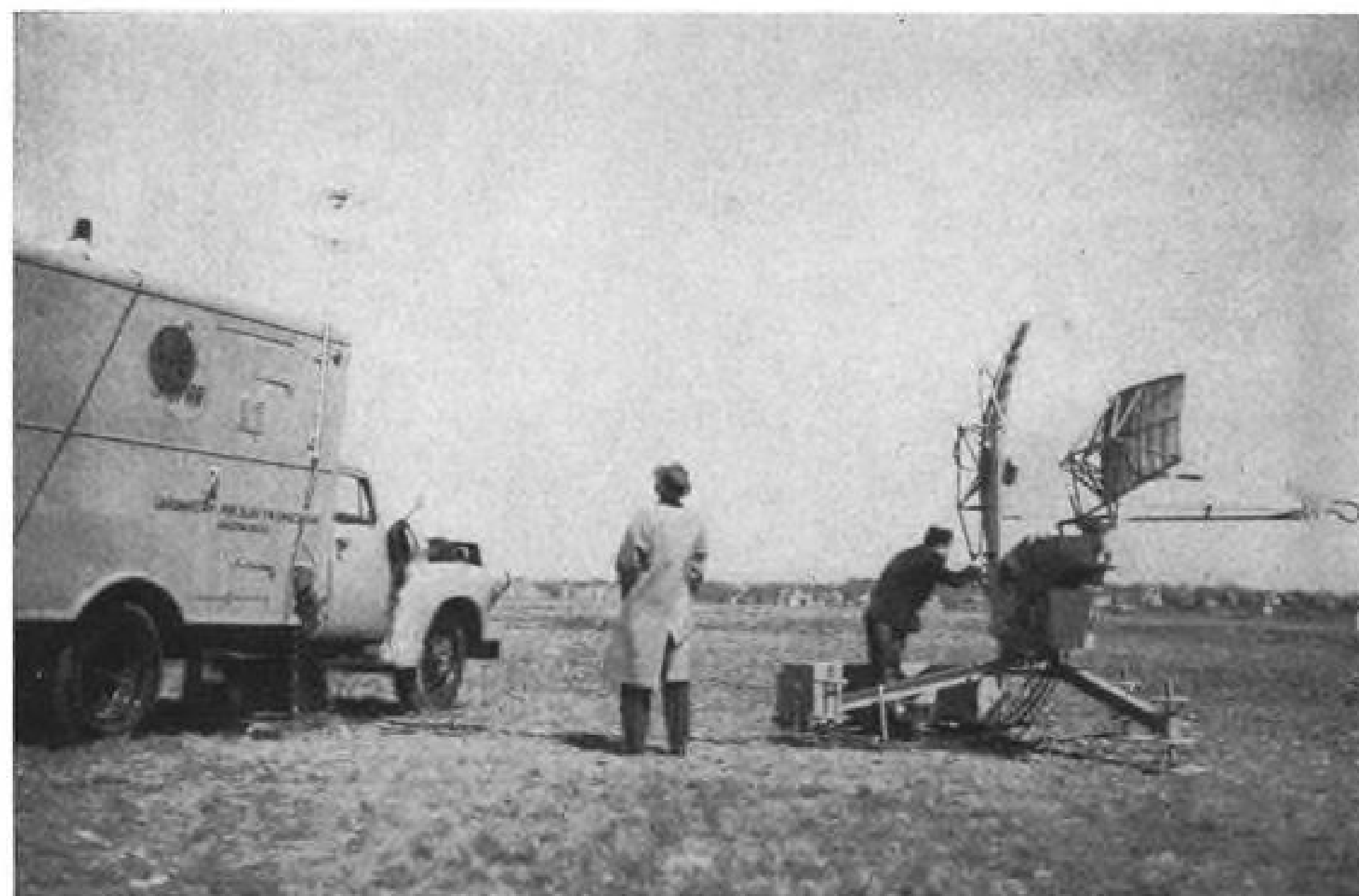
QUICK INSTALLATION is one feature of new approach system. SPAR's radar transmitter-receiver and power supply are housed in weatherproof metal boxes which can be laid on ground. Operator's console can be placed in truck, in tent or control tower.
