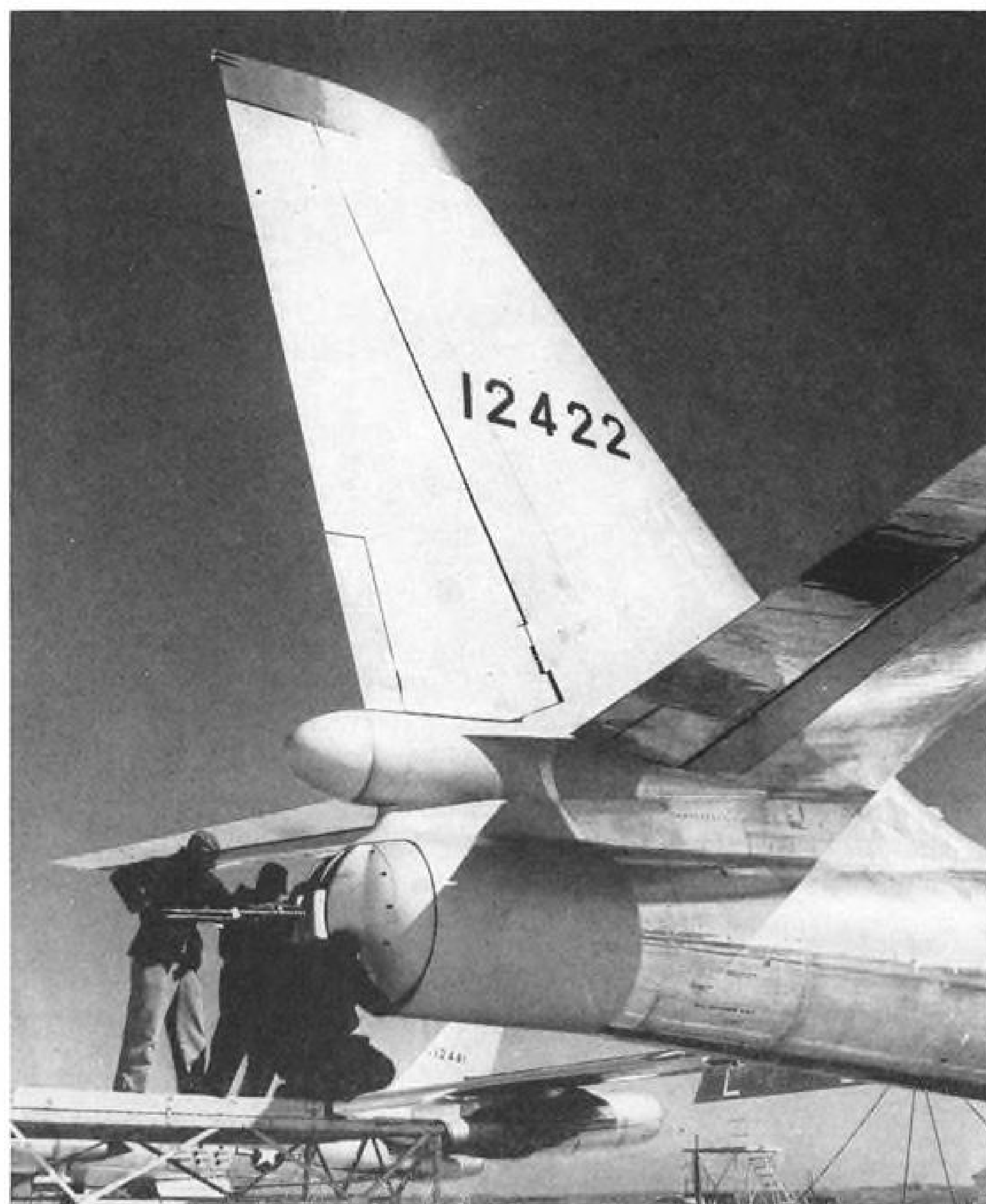
CANNON-PACKING 20-mm. tail turret installation and maintenance is simplified and speeded by detachable pod arrangement which permits system to be replaced in field.
