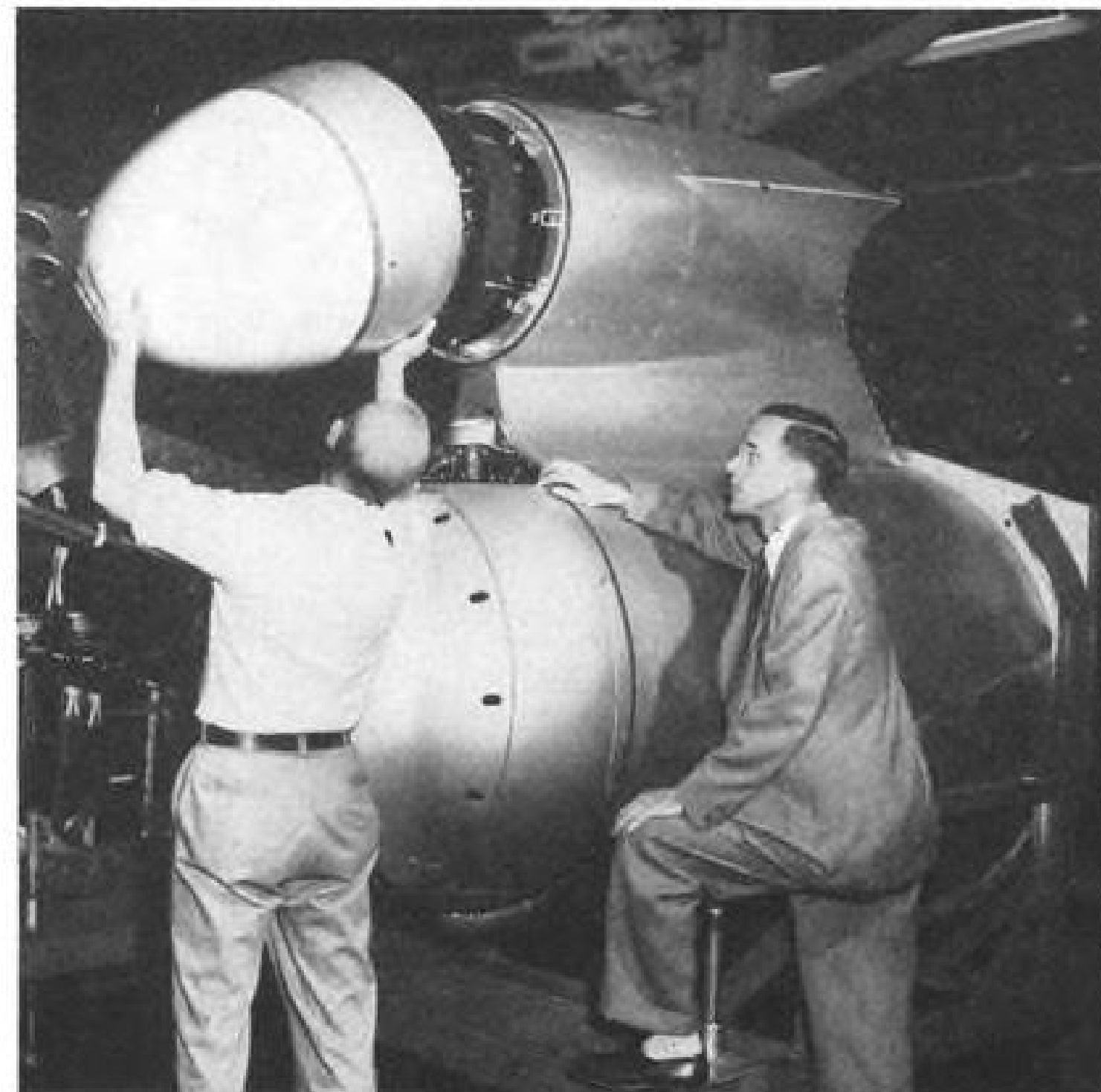
B-47E TAIL STINGER , G-E developed automatic radar-directed fire control system, is first to be made in a detachable pod.
