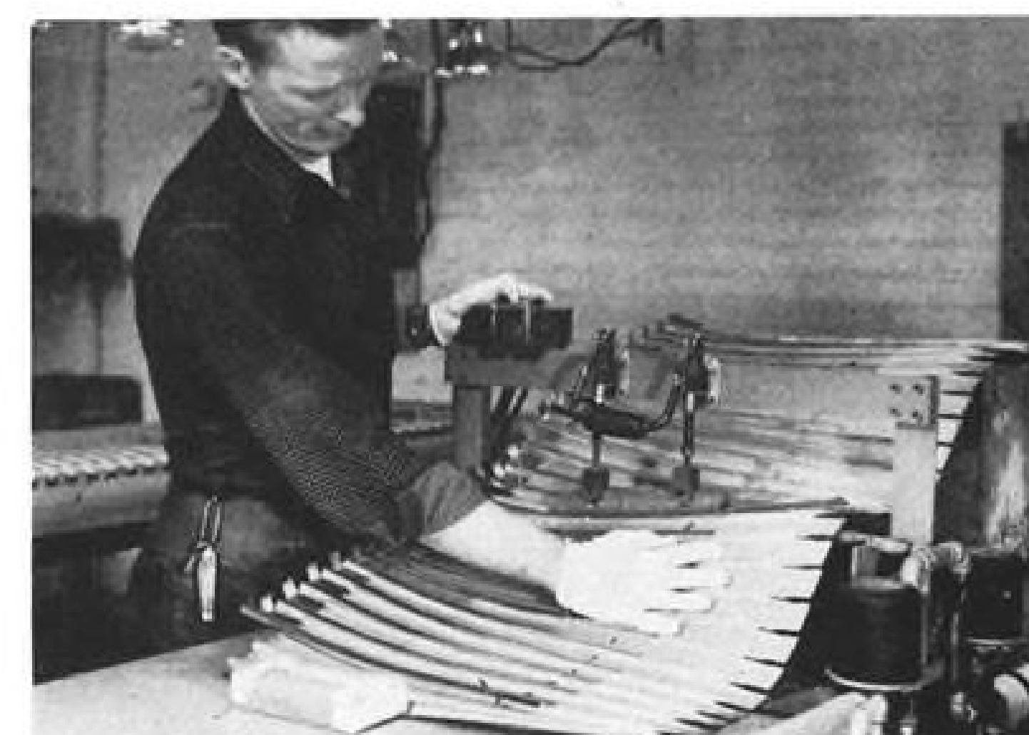
LOADING the mold, skin laminations and spar web are positioned before final heat curing of the complete XH-16A blade assembly.
