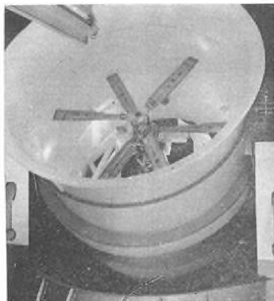
TEST DEVICE rotates 90 deg. on two large bearings to vertical or horizontal positions.
