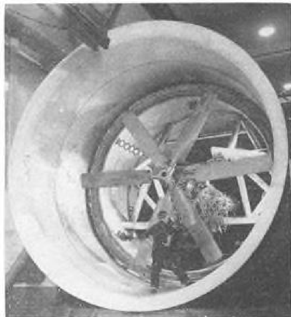
WINDTUNNEL, developed by Allison for VTO turboprop testing, dwarfs employee.
