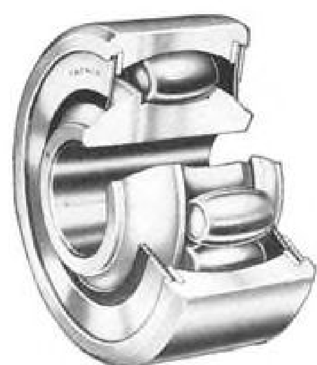
Fafnir DSRP Roller Series High Capacity, Self-Aligning Airframe Control Bearing
