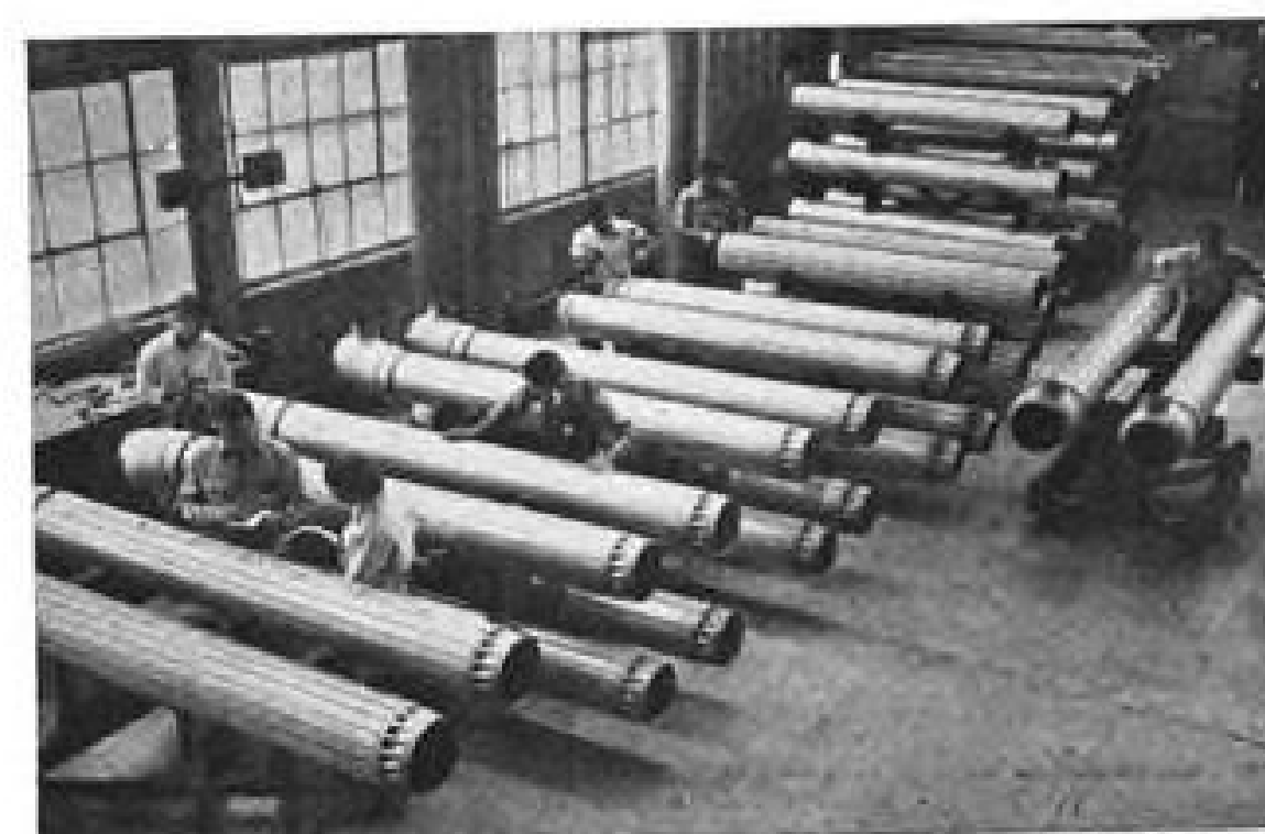
Stainless Steel augmentor tubes, also produced by Rohr Aircraft, are resistant to heat and corrosion, and carry exhaust gases from engine to rear of nacelle for additional or augmented thrust.
