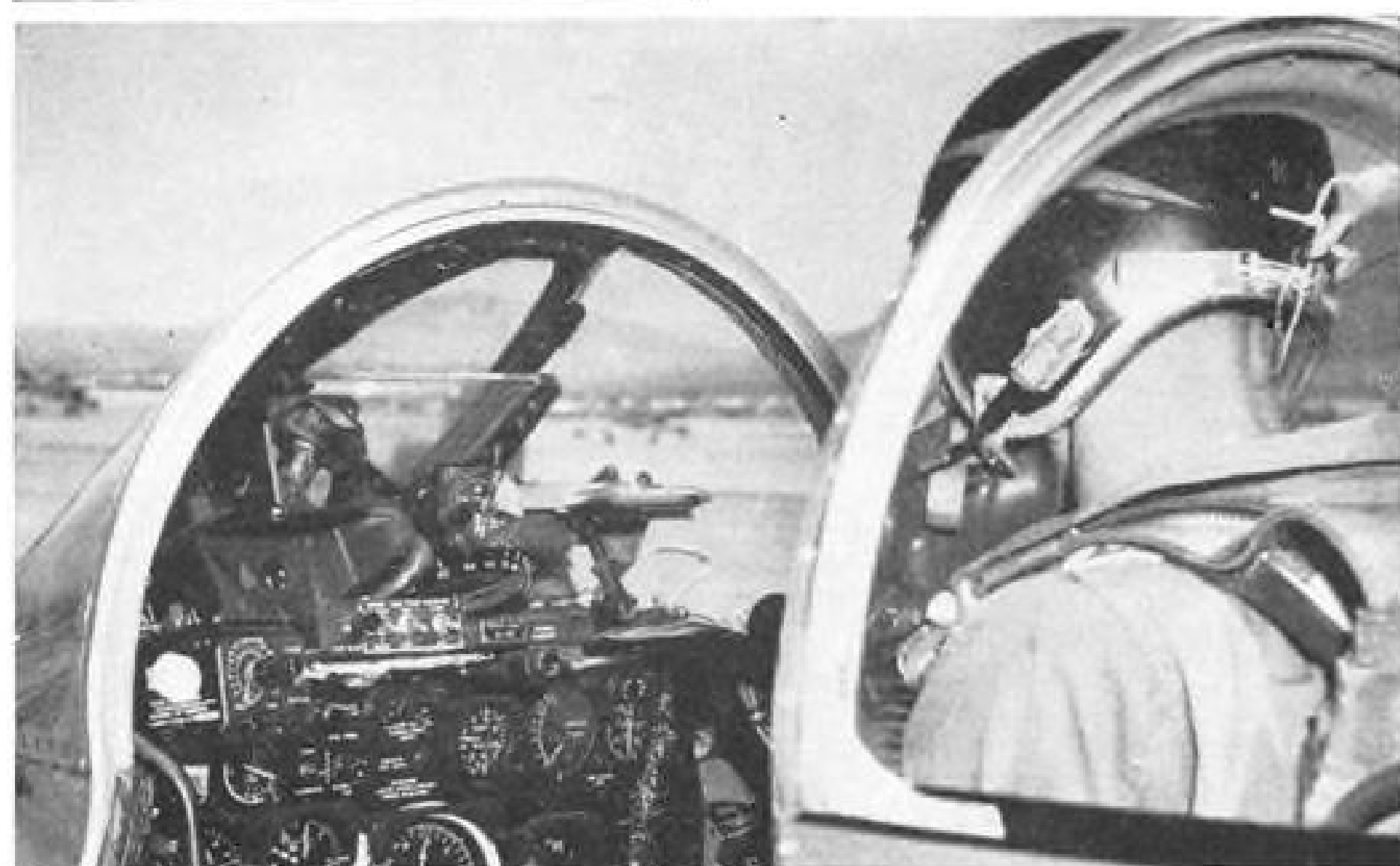
USAF's A-4 fighter gunsight, shown in F-86, automatically computes aiming point.
