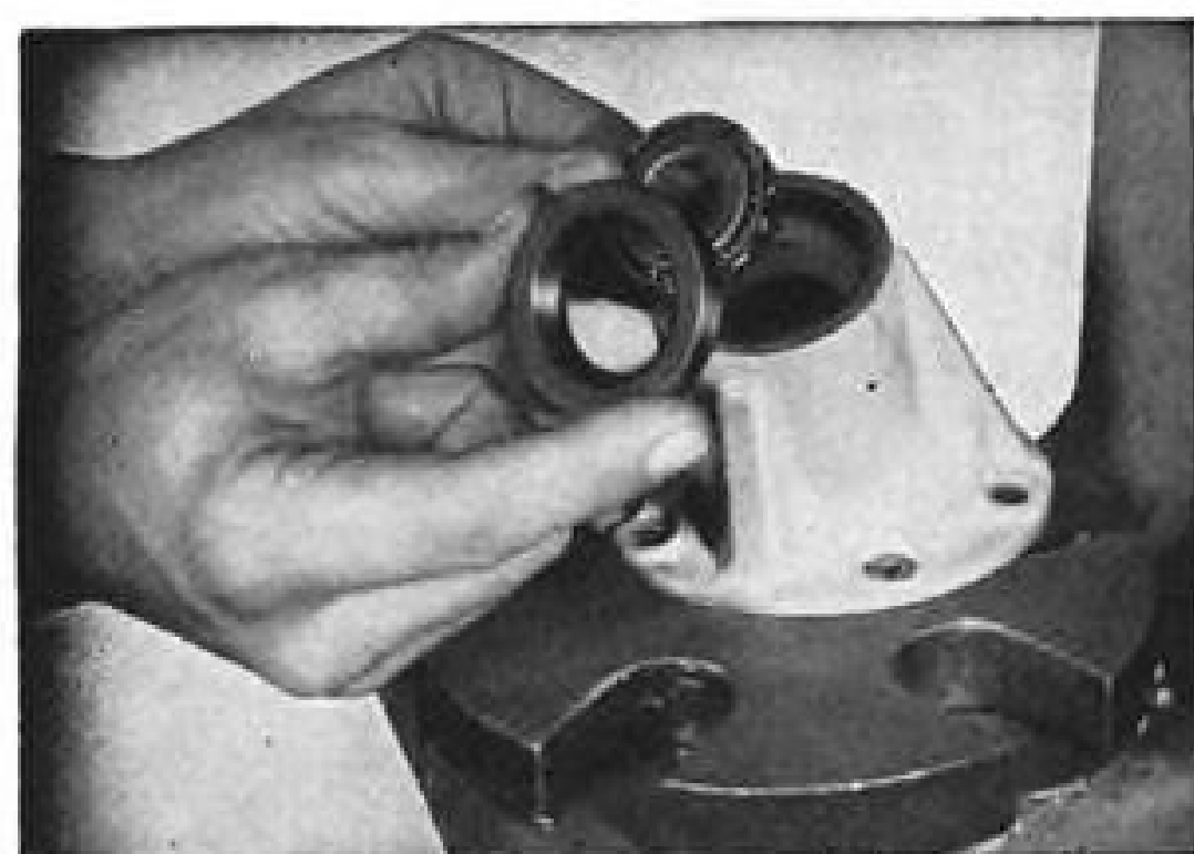
Clipper Seal being installed in the intermediate gear box of the Sikorsky HO5S helicopter to seal oil in, keep abrasives out.
