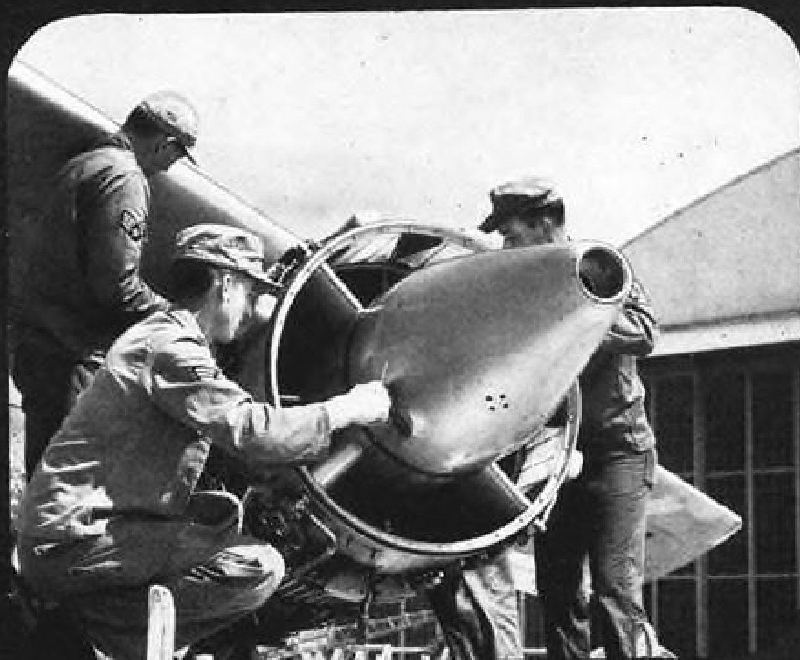
0906 Quick-disconnects of J47 electrical, fuel, and oil lines are completed.
