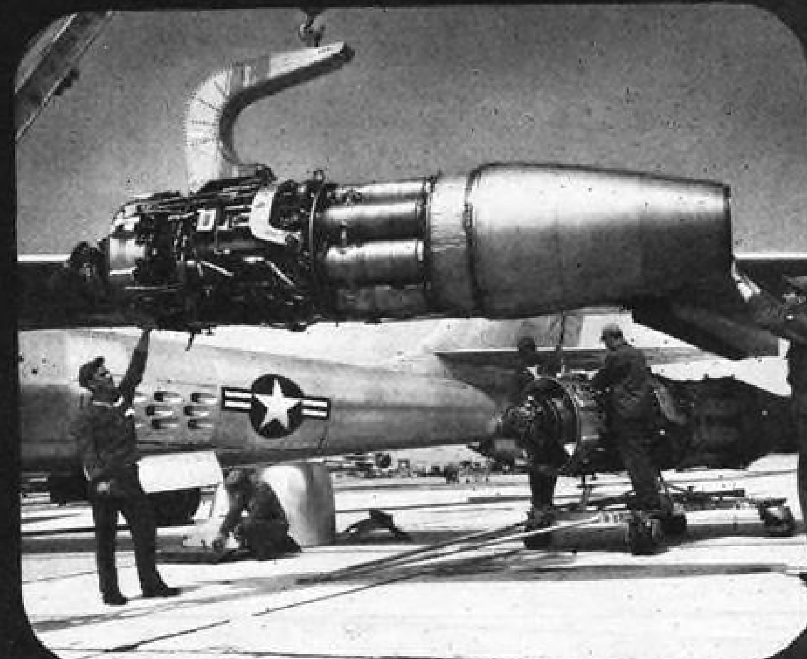
0914 Engine is swung away from wing as new J47 is pulled into position.
