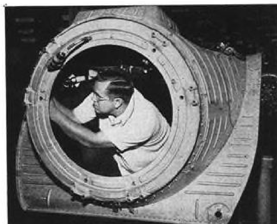
Type 347 or 321 Stainless Steel is utilized in the shroud assembly, installed in the Convair by Rohr Aircraft Corp., Chula Vista, Calif. Note bolt holes for attaching engine. The shroud acts as a firewall between engine and remainder of nacelle which houses hydraulic liquid and oil tanks.
