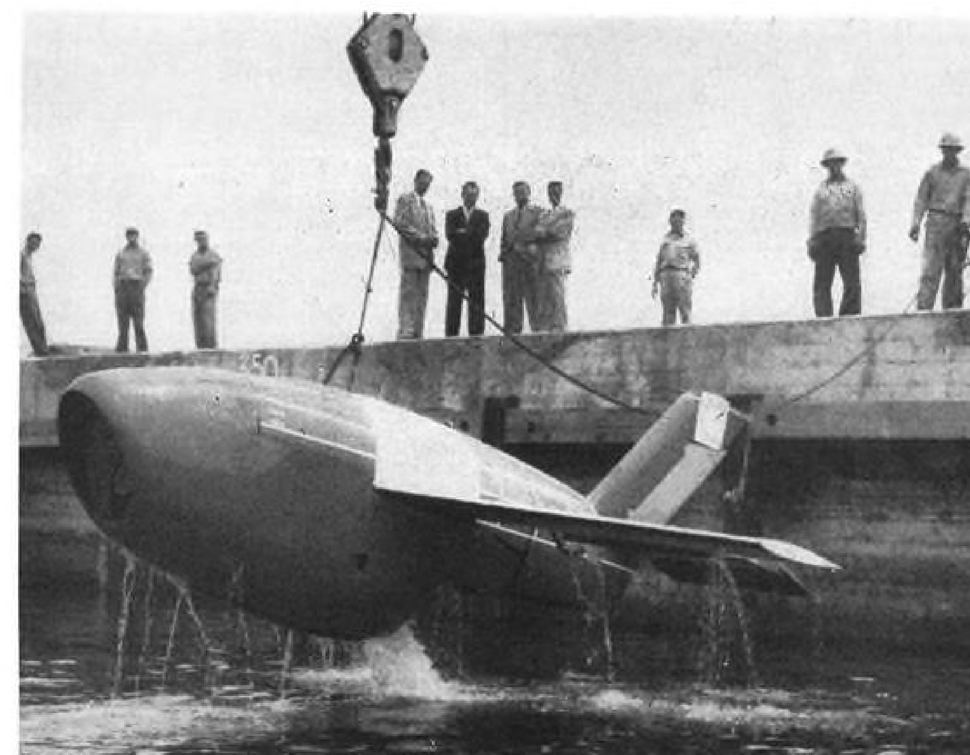
SPEWING SALT WATER , modified Ryan Firebee is regained after one-hour immersion.
