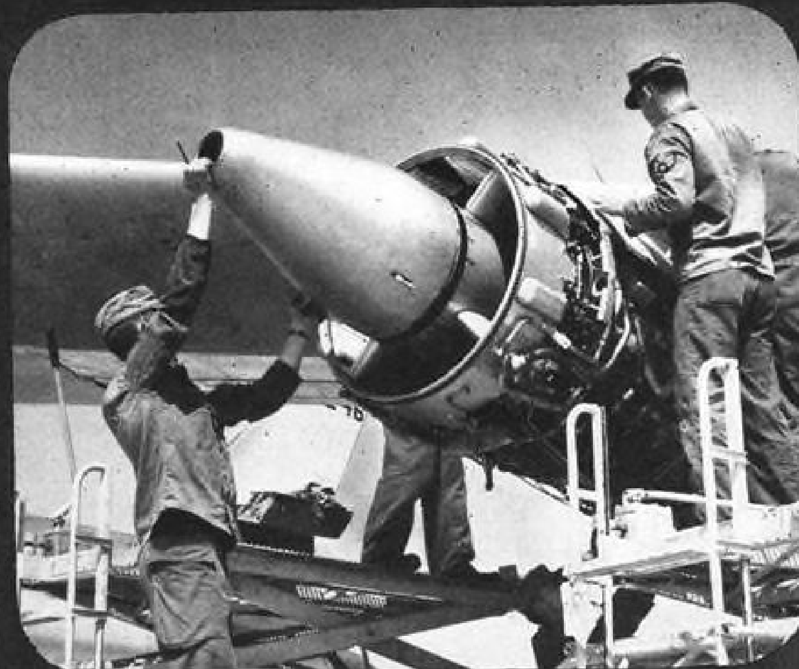
0924 Aluminum "bullet nose" and cowlings are clamped on just before running engine up.
