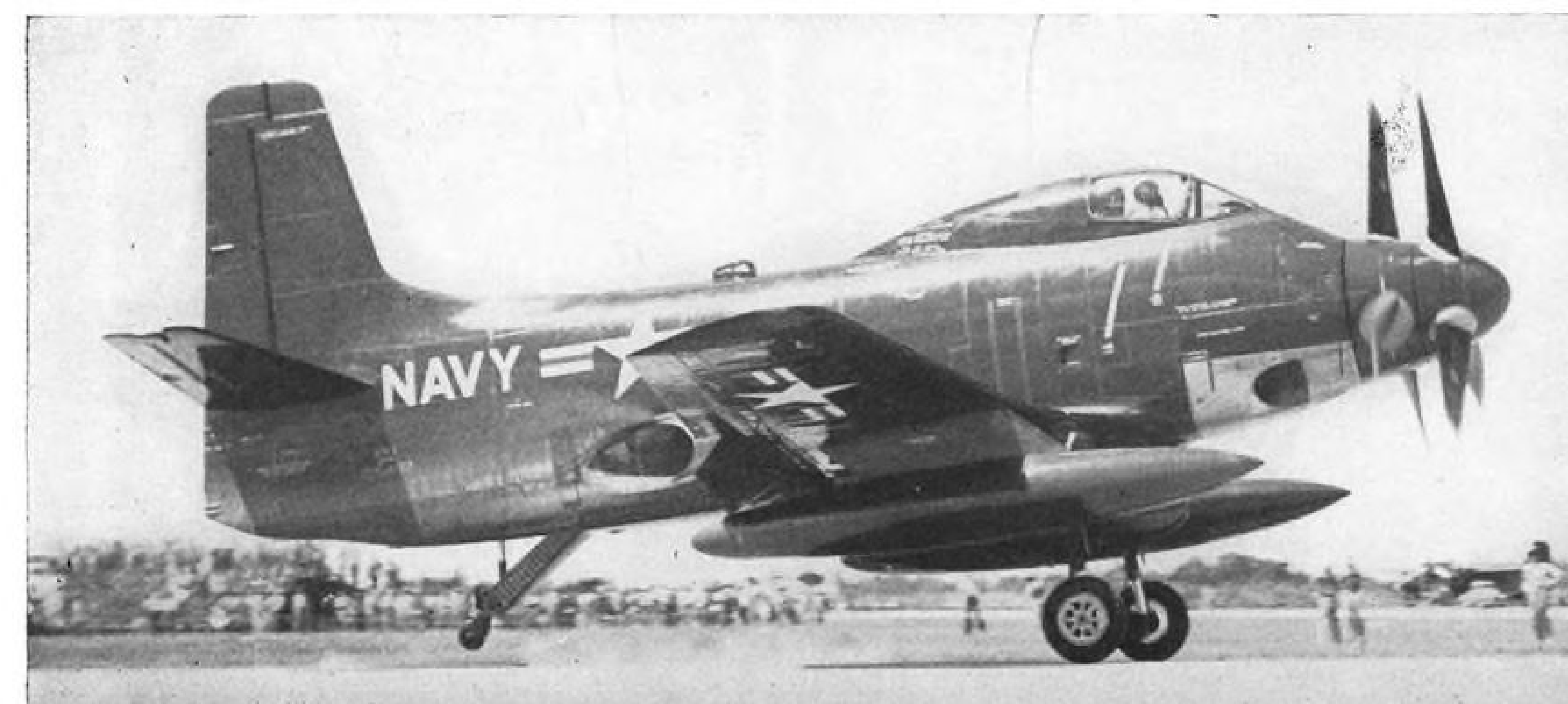
SPEED MARK of 2 hr. 38 min. was set recently for 1,086-mi. distance between Indianapolis, Ind., and Opa Locka, Fla., by this production Douglas A2D-1 Skylark (below). Powered by 5,850-eshp. Allison T40-A-6 turning contra-rotating Aeroproducts props, this and another Skyhawk are used by Allison as testbeds for T40 development. T40s with contraprops also are flying in Convair's R3Y-1 flying boats and are being produced for the new R3Y-2 "bow loader" version.
