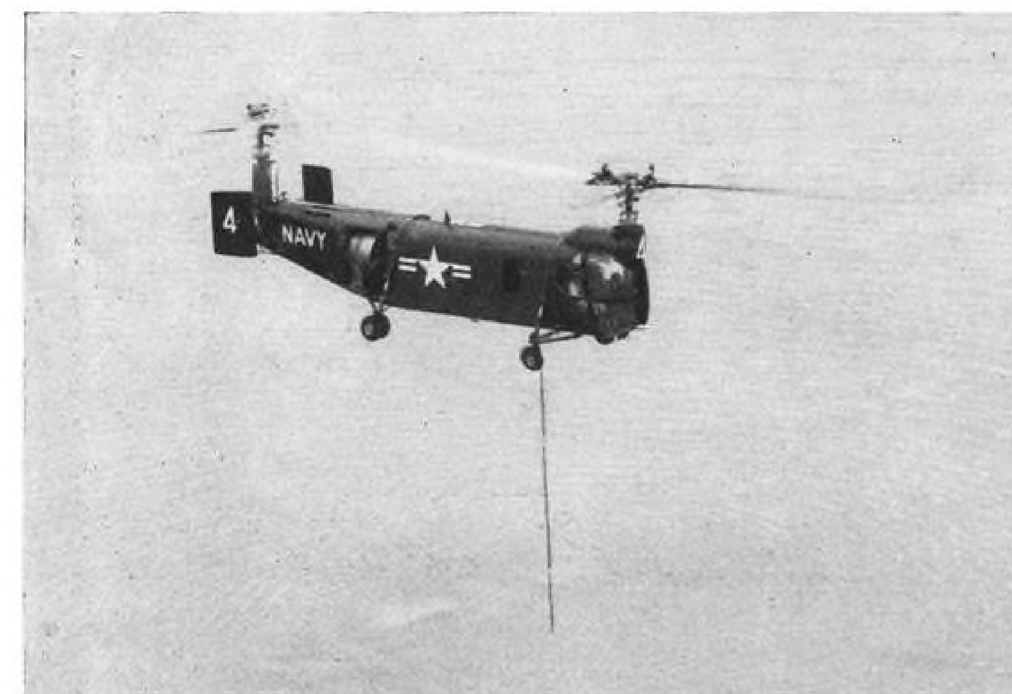
SUB SNOOPING TECHNIQUE using "dipping sonar" to detect underwater craft, is demonstrated by Navy's big Bell HSL-1 tandem-rotor copter. The HSL-1 carries lightweight homing weapons to kill subs located by its detection devices.
