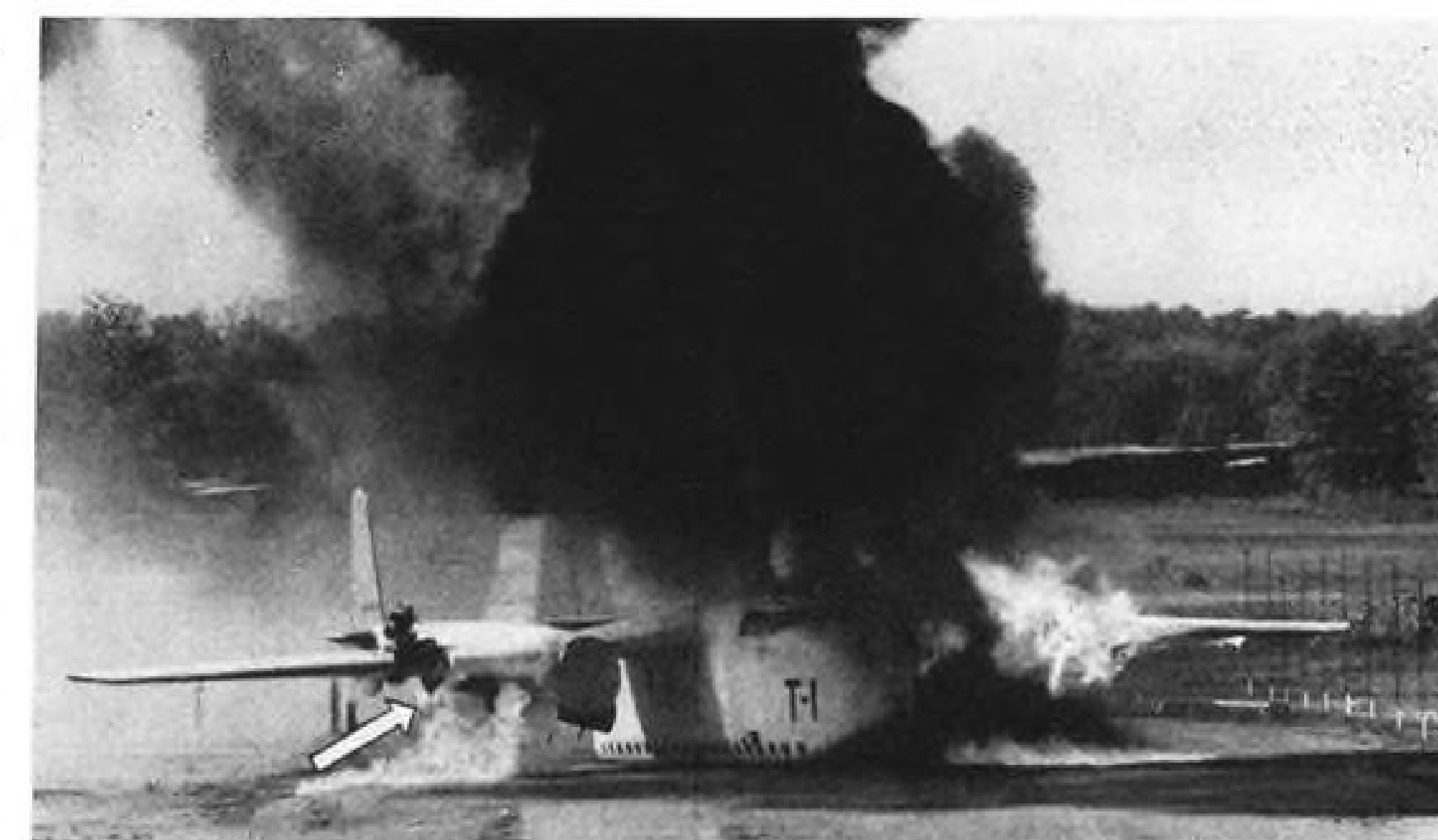
CRASH FIRE RESEARCH PLANE plows through barrier and burns. NACA studies show that fire sources in jet engine (arrow) could be eliminated with . . .
