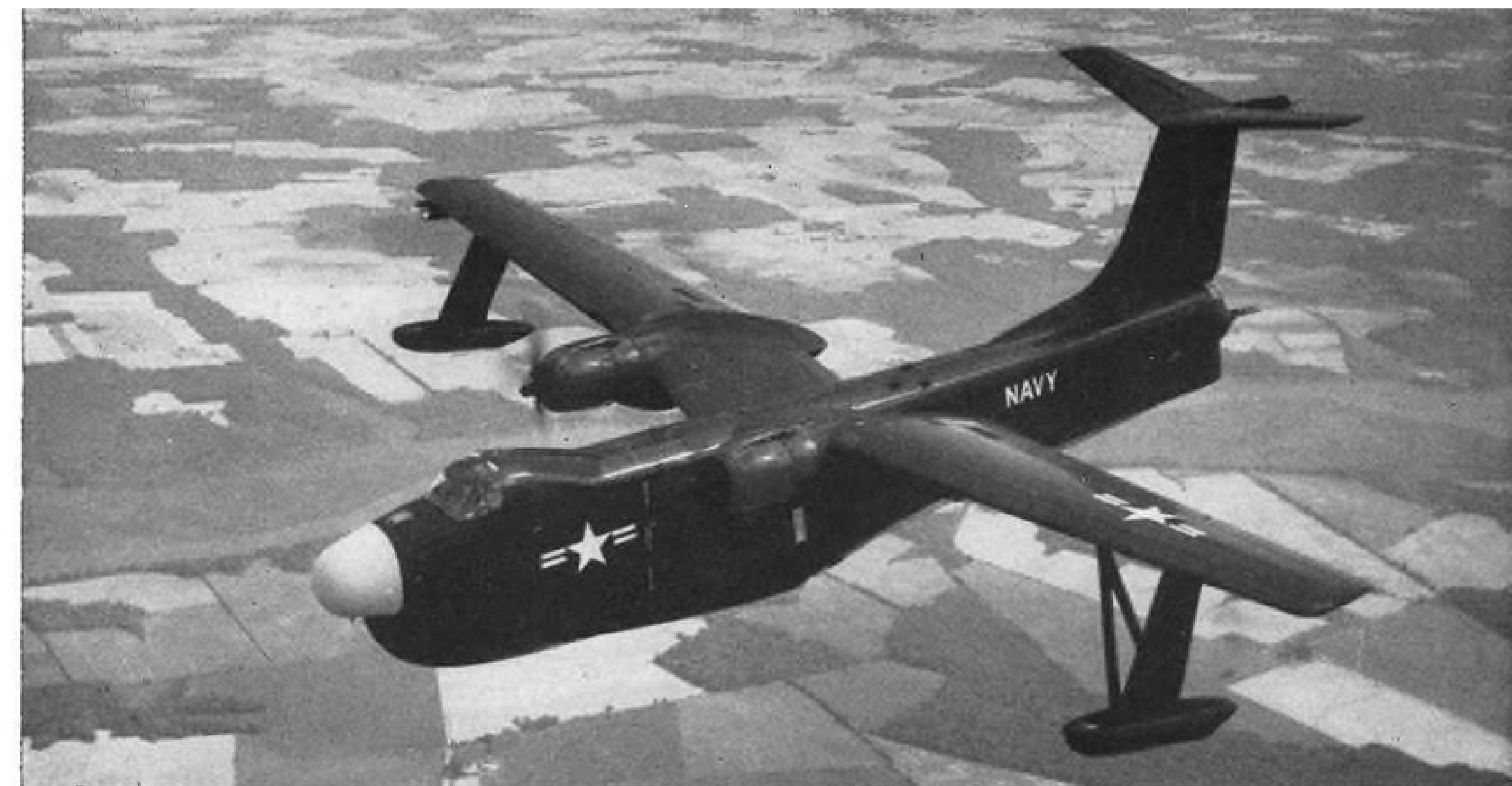
FIRST PRODUCTION Martin P5M-2 Marlin anti-sub flying boat, distinguished from the earlier P5M-1 by its T-tail, has been delivered to the Navy. Packed with electronic gear, the new Marlin has two 3,450-hp. (dry) Wright R3350-32W Turbo Compounds.
