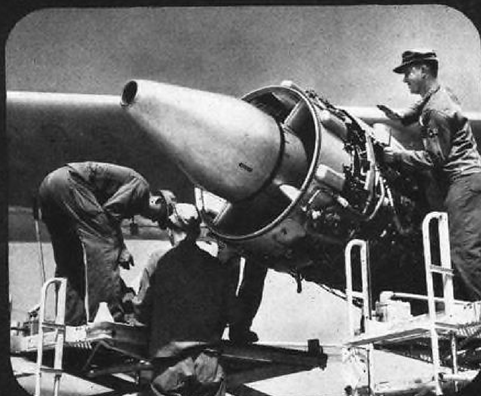
0900 Stepping up on their work stands, line crew removes outboard engine cowlings.
