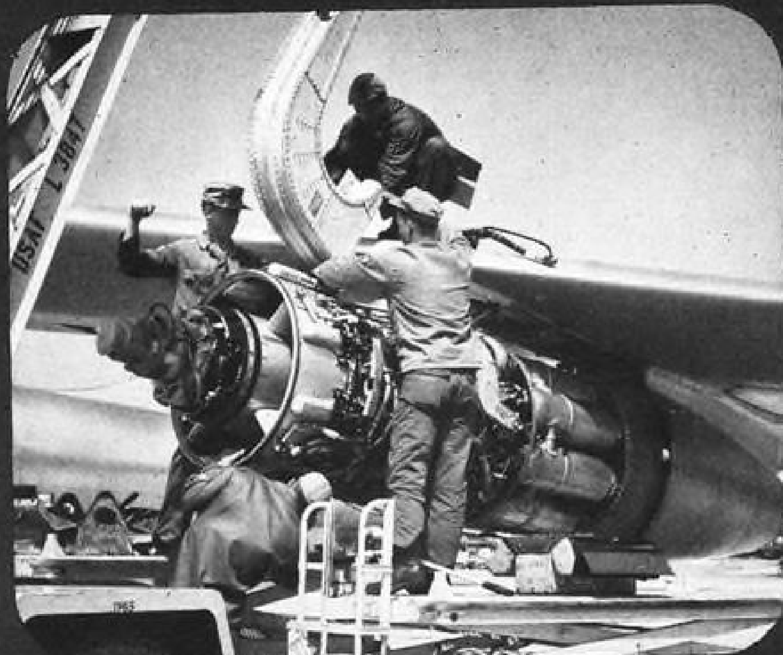
0919 New engine hoisted up while crew installs J47 fuel, oil, and electrical lines.
