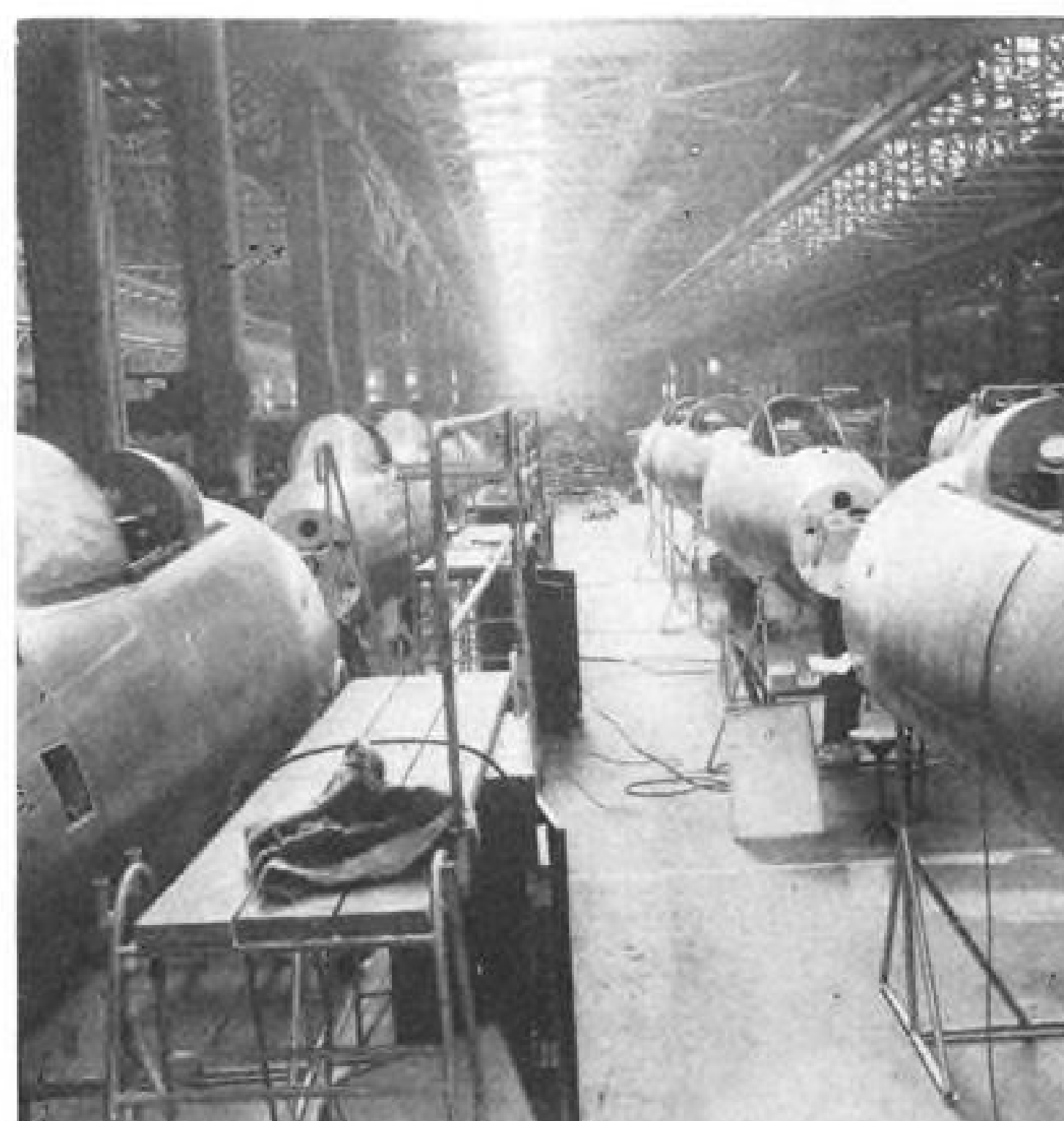
3. SEMI-FINISHED Hunters on production line at Hawker's Blackpool plant wait for other parts to join them.
