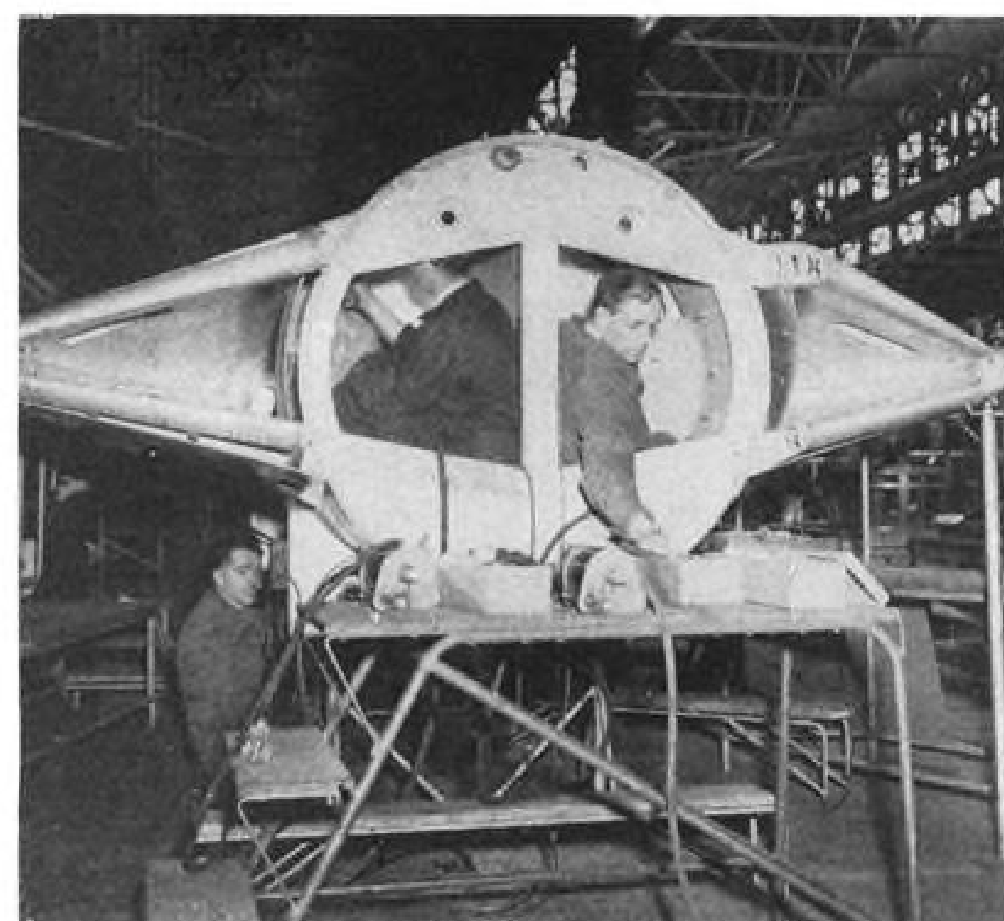
2. FUSELAGE SECTION , like other components, is built as complete unit, including all equipment, wiring, etc. When components come together for final assembly, it is relatively easy to connect structures, tubing, wiring.
