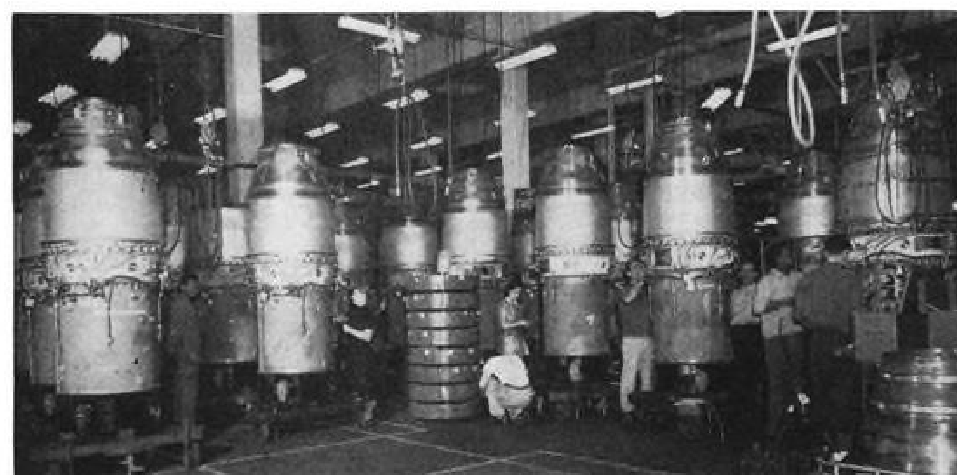
3. AT END OF LINE, engines get finishing touches at Curtiss-Wright's Wood-Ridge plant. The J65 powers the Lockheed XF-104 and five other military aircraft.
