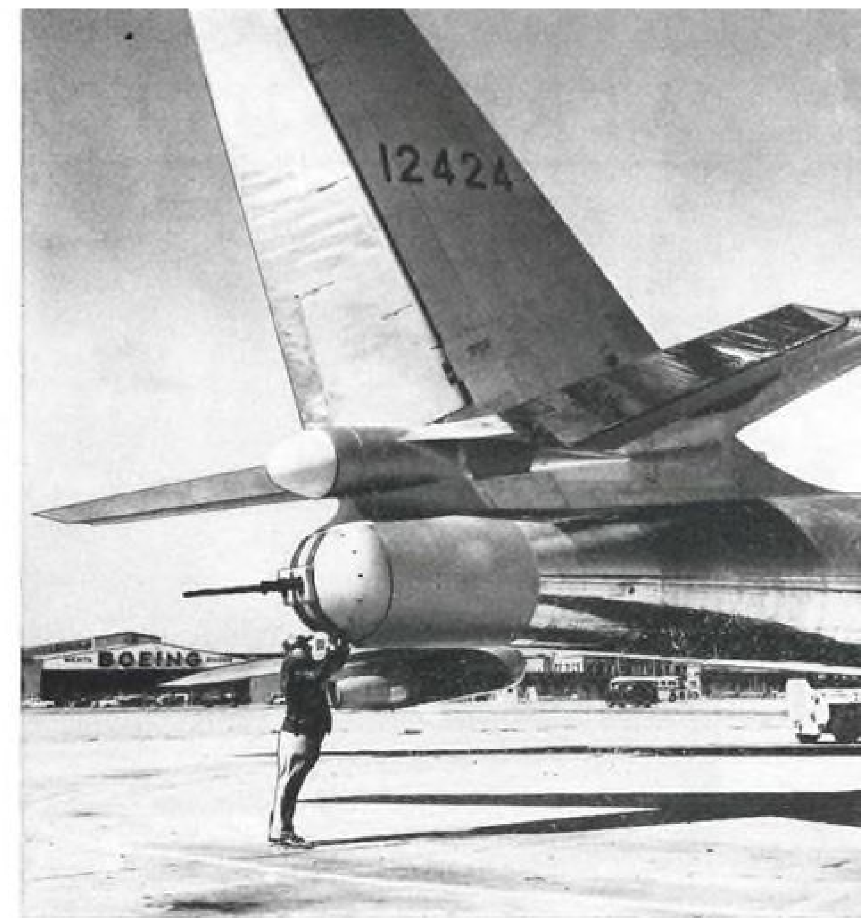
Remote-controlled G-E armament system gives the Boeing B-47E and RB-47E jet bombers a heavyweight punch to the rear. Guided by radar, the 20 mm system can track and hit unseen targets.
