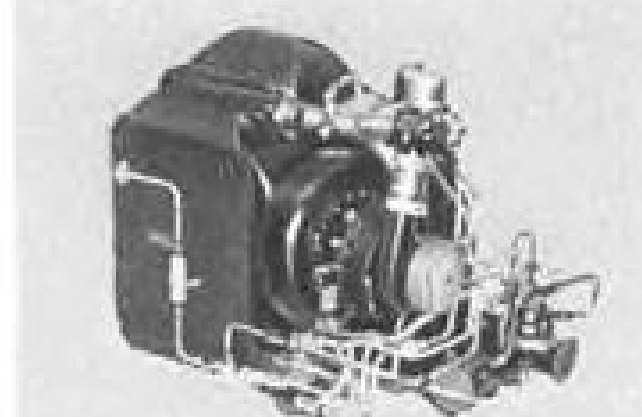
AIR-CYCLE REFRIGERATION PACKAGE BUILT FOR THE 707
