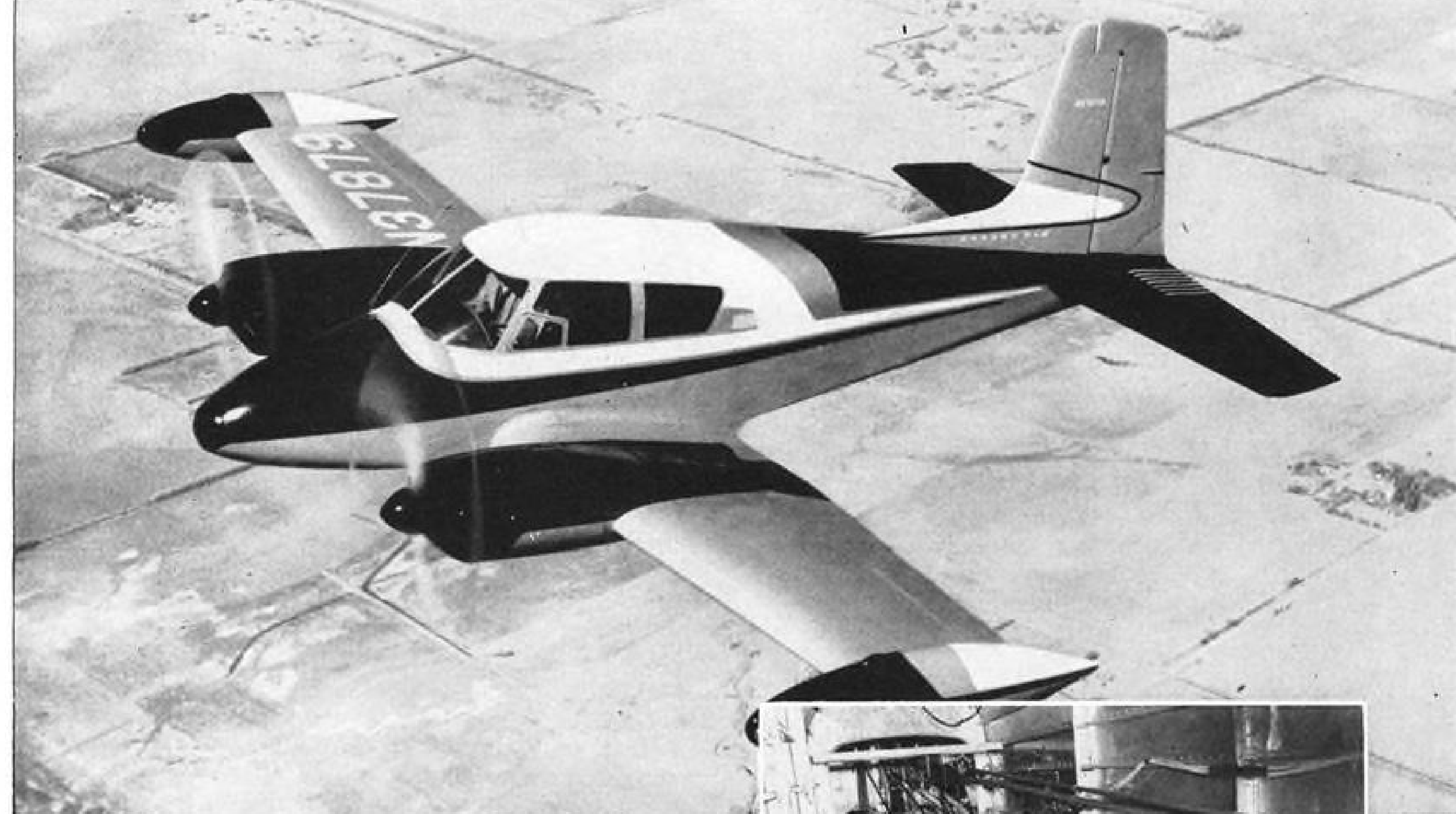
Cessna Model 310 in flight. The new executive plane cruises at 205 m.p.h.; has a range of 1,000 miles.
