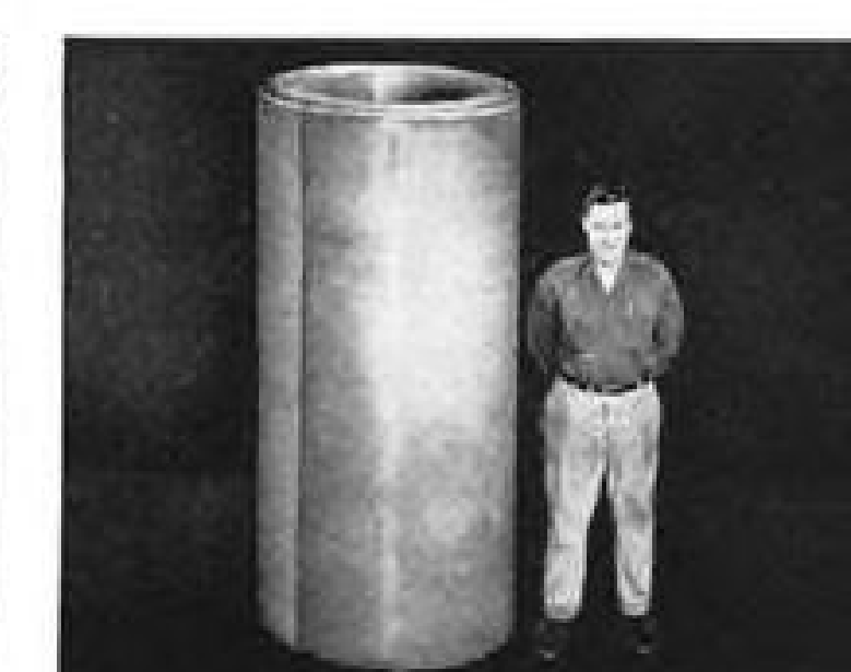
This coil of magnesium sheet started through the 84-inch coil mill as a one-ton rolling ingot.
