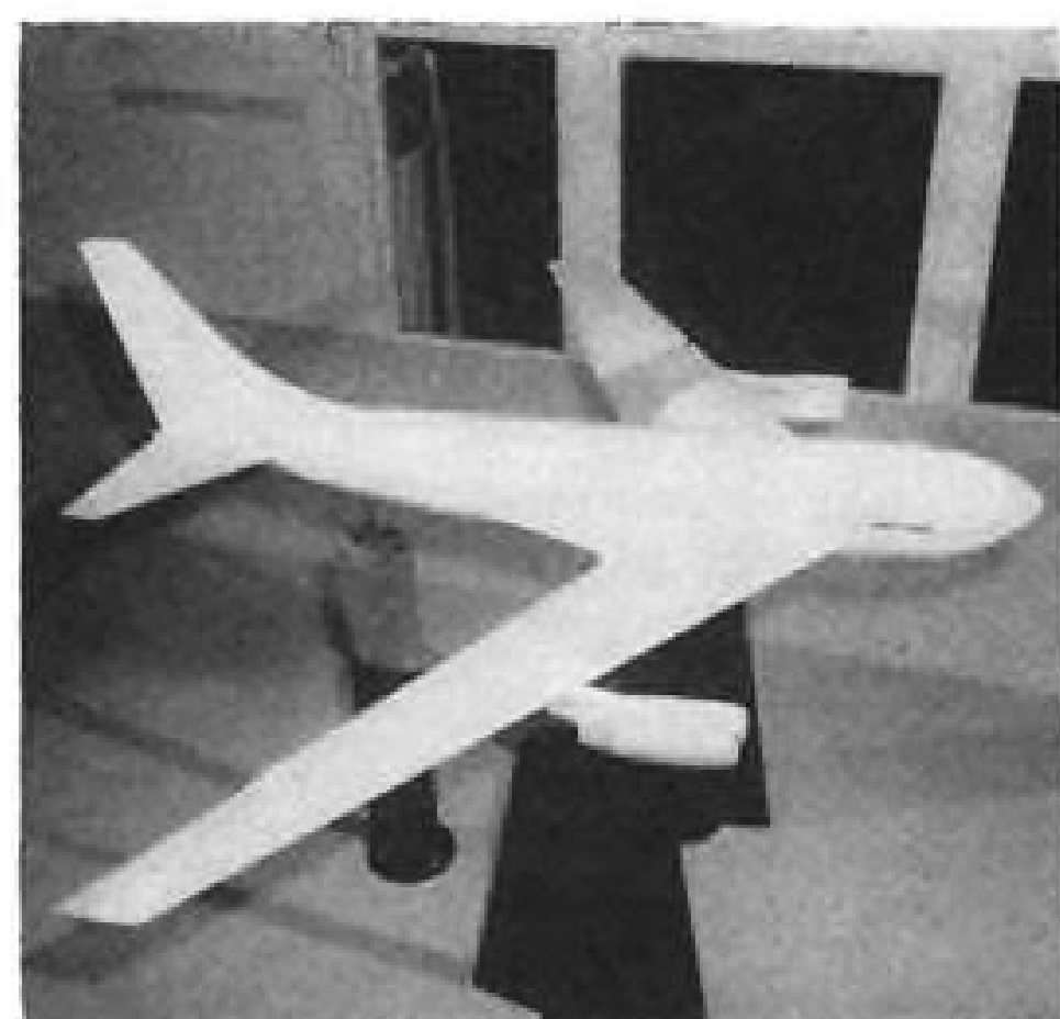
EARLY DESIGN STUDY of the 707, based on B-52, reached windtunnel stage. Note similarity of pods, wing and horizontal tail.
