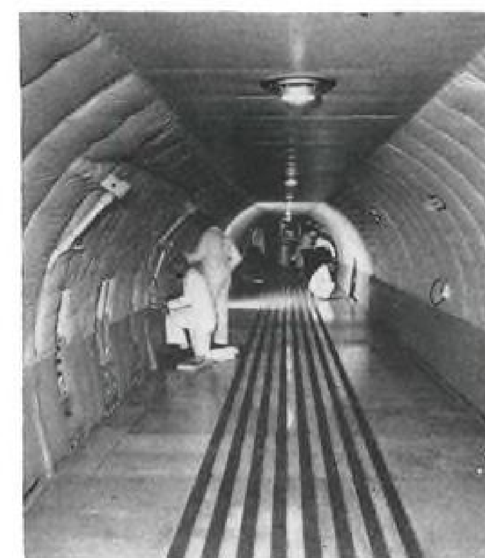
INSIDE THE FUSELAGE of the 707 looking forward. Fuselage cross-section and floor position are arranged to give maximum width at passengers' elbow height.
