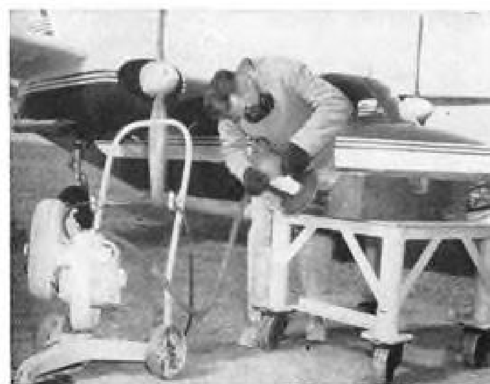
MACHINE sands augmentor tube fairing die used in Aero Commander cowl.
