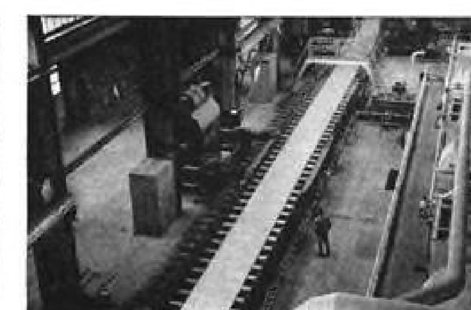
World's first 84-inch magnesium coil mill now rolls sheet and plate in greater lengths and widths.
