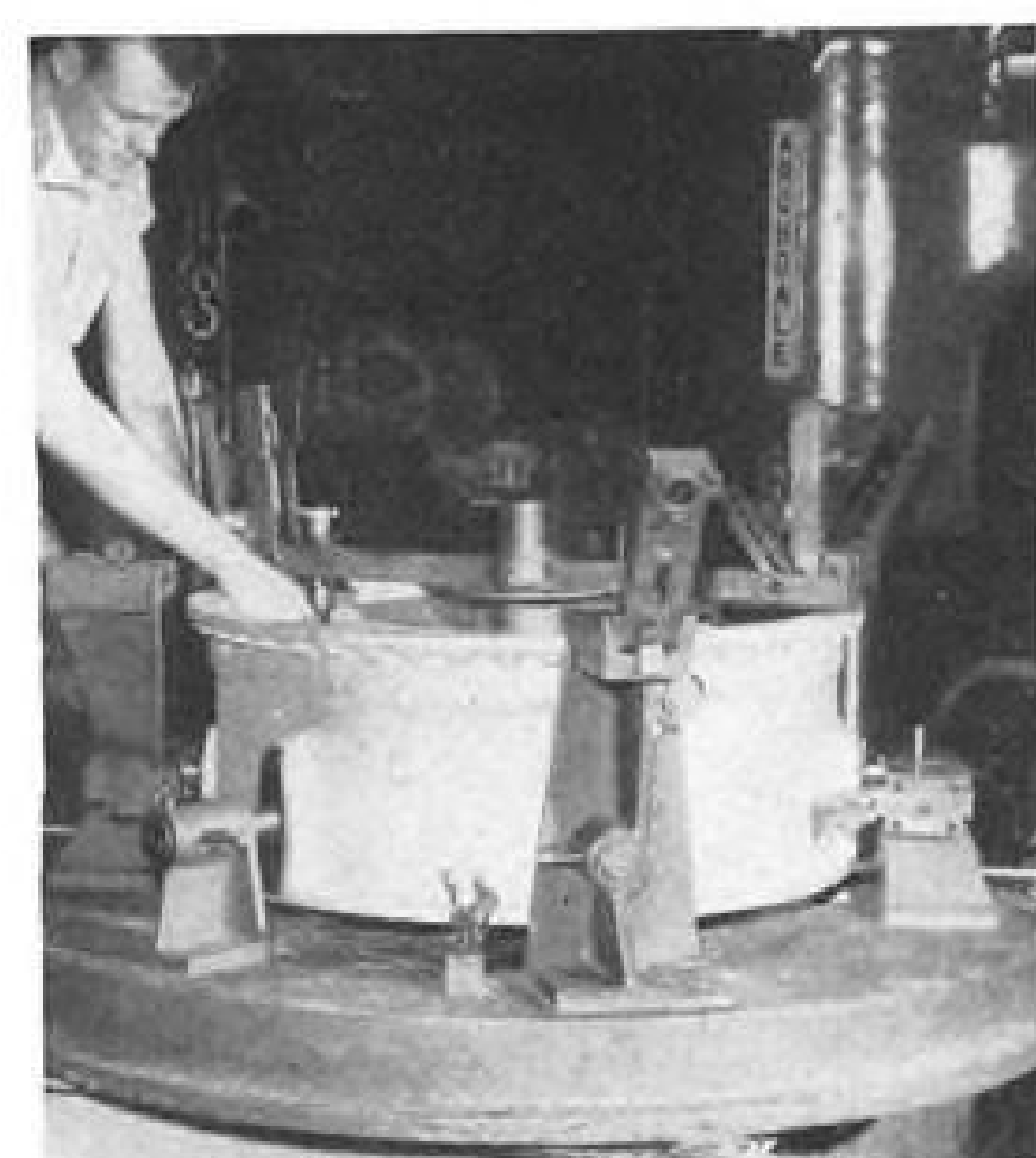
INTAKE CASTING set for operation on Archdale radial drilling machine.
