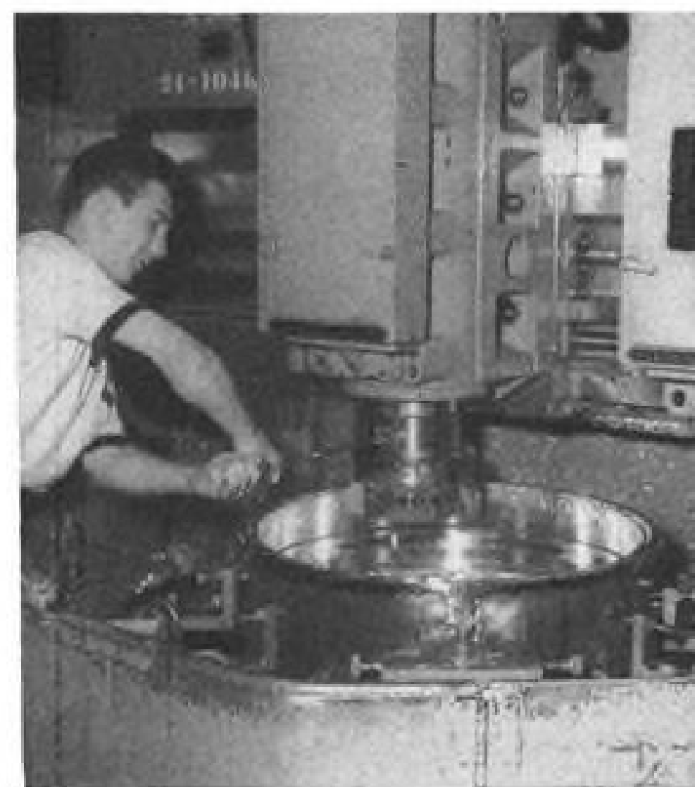
COMPRESSOR CASING has inside surface machined on vertical turret lathe.
