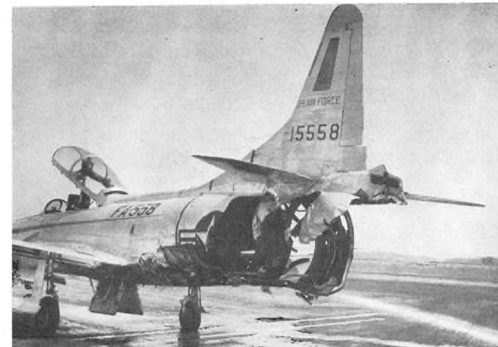
LOCKHEED F-94C aft fuselage is chewed off right up to powerplant turbine wheel.
