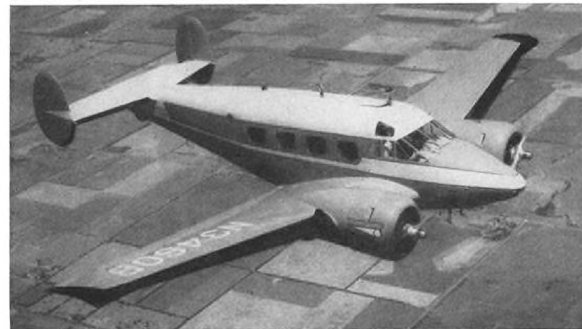
LARGE WINDOWS —four on each side, in place of former three—and deeper fuselage on new 234-mph. Super 18 give improved view, roomier, more comfortable cabin.
